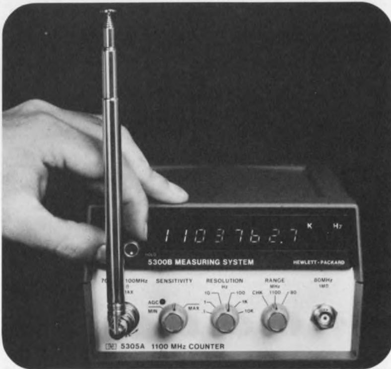
Check its features. The HP 5300B/5305A has the quality, convenience and portability your applications demand. But it doesn't stop there. Snap the 5305A counter module off the 5300B mainframe and in seconds you're ready to snap on any one of seven other modules including a full-range multi-meter. All backed by the full HP guarantee and HP world-wide service.
