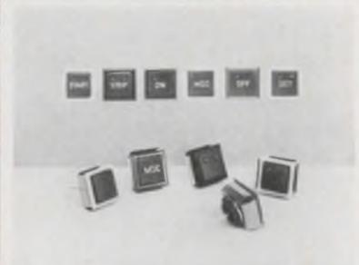
**Touch Activators** for solid-state switch circuits eliminate pushing, pulling, or flipping of switches. No moving parts; high reliability. A mere touch of finger activates switch circuit. Interface with CMOS, TTL, DTL, and HTL. Snap-in panel mounting. Lighted or unlighted. Master Specialties, 1640 Monrovia, Costa Mesa, Calif. 92627.
