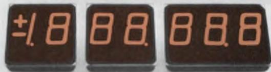
**755 SERIES** High brightness planar gas discharge displays in a 0.550" character. Orange color gives high contrast ratio and allows readability to 40 feet even in high ambient lighting. Designed for interfacing with MOS/LSI, displays have an expected life of 100,000 hours or more.
