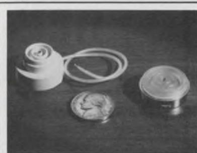
**MINIATURE HIGH VOLTAGE CONNECTORS** with exceptionally low current leakage. High efficiency characteristics sharply reduce size and weight of power supply requirements. At 16KV, current leakage is lower than 10 nanoamperes -54° C to +65° C operating temperature range. SGL ELECTRONICS, Westville, N.J. 08093. Phone: (609) 456-7300
