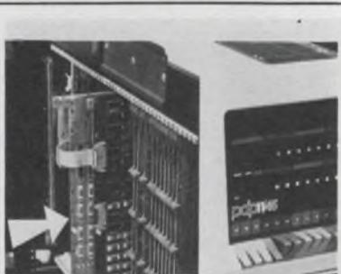
**Cache Buffer for PDP 11/45.** Model 4511 buffers entire 124k main core memory of PDP 11/45, achieving effective MOS speed of 450 nsecs, without 32k MOS limitation. Plug-compatible, bipolar technology, contained on 3 p.c. cards. Installs in minutes. Fabri-Tek, Inc. 5901 S. County Rd. 18, Mpls., MN 55436. (612) 935-8811.
