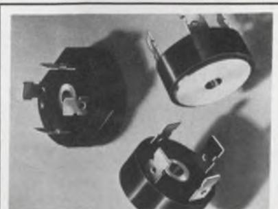
**30 amp bridge rectifiers** for UL applications from Tarzian has exceptionally long creepage path (+1/4"), aluminum base for rapid heat dissipation. 400 Amp surge rating. 50-1000 PIV. Center hole or stud mount cases \$3.42 and up in 25 quan. Sarkes Tarzian, Inc., Semiconductor Div. 415 College Ave., Bloomington, IN 47401, 812-332-1435.
