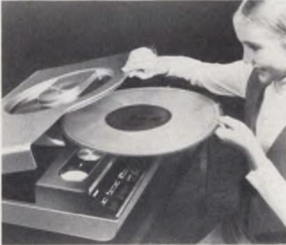
The video disc is inserted in the Philips-MCA playback unit. The system offers such features as slow-down, freeze frame and reverse.
