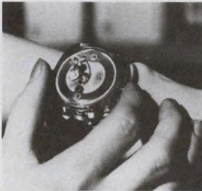
**Citizen alarm's actuator** is this wrist-mounted transmitter. The printed-circuit loop-antenna transmits a coded signal to a grid of receivers. The receivers locate the signal and relate the code to a central dispatcher. Finally the proper help is dispatched to the scene of the emergency.
