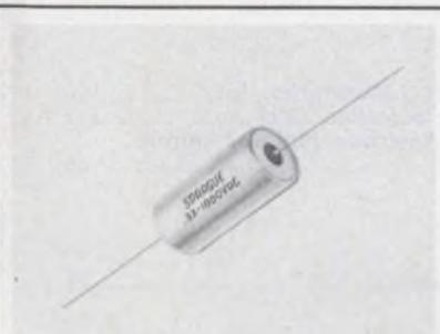
**A natural for SCR snubber applications.** Type 196P Vitamin Q<sup>8</sup> metal-clad paper capacitors for high-current, high-voltage, high-repetition-rate a-c applications. Built to take 600-to-800 volts peak a-c. Write for Bulletin 2110D to Sprague Electric Co., 347 Marshall St., North Adams, MA 01247. (413) 664-4411.
