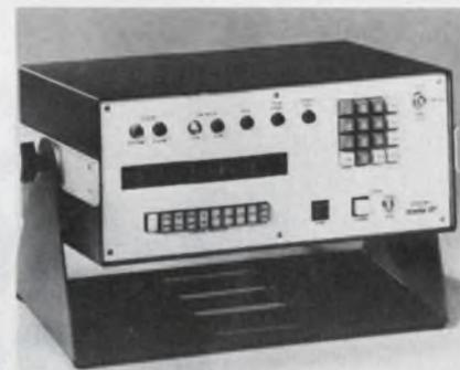
Display panel of the Monitor 101 provides a keyboard (right) for entering numbers into the computer's memory and selector buttons (lower left) for displaying desired data.
