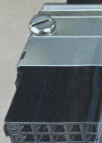
The ribbon is made up of individual coaxial cables, each with a solid center conductor and a foil-wrapped drain wire shield. The drain wire is not spirally wound around the dielectric, but runs parallel with the center conductor. This feature allows the cable to be cut anywhere and yet be consistently and reliably terminated.
