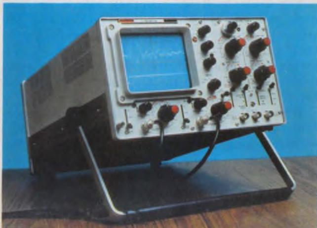
Delayed sweep and mixed sweep operation are two of the key features of Ballantine's 1040A. It is a portable 40-MHz dual-channel scope.
