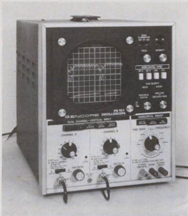
Medium price and performance are available with the PS163 dual-trace scope from Sencore. It features 5-mV sensitivity and less than 2 degrees of phase shift between channels.
