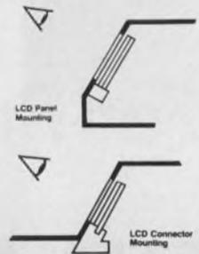
**Connector Mounting** is made with an edge board connector to hold the display and for making electrical hook up.
