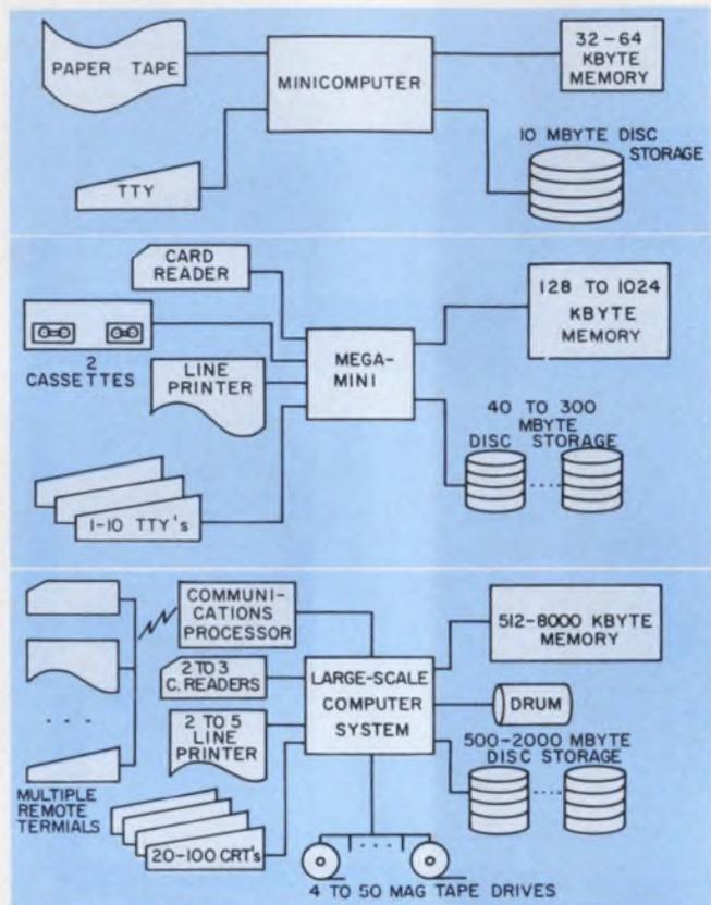
1. Computer systems range from simple minis to large scale mainframes. Newer minis, such as Interdata's Megamini, have less elaborate hardware than mainframe units and fill the gap between large scale processors and simple stand-alone configurations.
