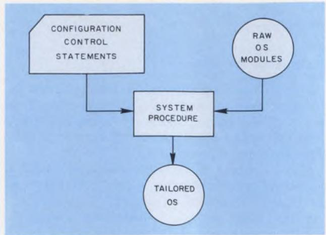
2. To start work with a supermini, the user must do a SYSGEN—in which selected operating system modules are joined to support the particular application.
