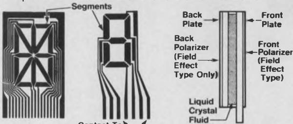
**Flexibility of design** permits LCDs to be scaled up or down to meet product needs. For example, Hamlin makes a display used in a ladies watch that measures only .450" x .575" (11.25 x 41.375 mm), but production facilities permitting, a display could be almost any size. Type of artwork used for creating the display design also provides an inexpensive way to customize with a logo, product illustration, etc.
