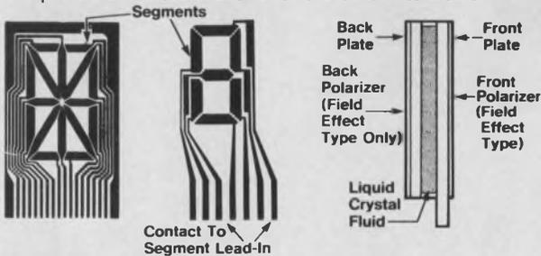
**Flexibility of design** permits LCDs to be scaled up or down to meet product needs. For example, Hamlin makes a display used in a ladies watch that measures only .450" x .575" (11.25 x 41.375 mm), but production facilities permitting, a display could be almost any size. Type of artwork used for creating the display design also provides an inexpensive way to customize with a logo, product illustration, etc.
