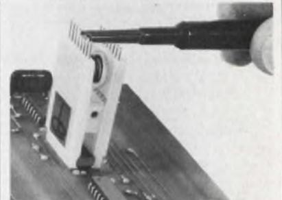
**IC Test Clips: New Lower Prices.** Eleven models of A P Test Clips provide full access to standard and LSI DIP leads . . . solve probe attachment problems . . . remove DIP's damage-free. Typical reduced prices: TC-14: \$5.25 TC-16: \$5.75. TC-24: \$13.85. Gold-plated contacts. Free catalog. A P Products Inc. Box 110-D, Painesville, OH 44077.
