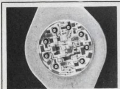
**MSK MODEL 150.** High Voltage—High Current Operation Amplifiers. 1 Amp Output Current.  $\pm 20$  Volt Output. Full Mil Temperature Range. Short Circuit Protected. TO-3 Package. Designed specifically for Synchro Applications. 100 pc. price \$58.00 ea. M.S. KENNEDY CORP. Syracuse, N.Y. (315) 455-7077
