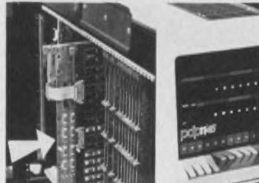
**Cache Buffer for PDP 11/45.** Model 4511 buffers entire 124k main core memory of PDP 11/45, achieving effective MOS speed of 450 nsecs, without 32k MOS limitation. Plug-compatible, bipolar technology, contained on 3 p.c. cards. Installs in minutes. Fabri-Tek, Inc. 5901 S. County Rd. 18, Mpls., MN 55436. (612) 935-8811.
