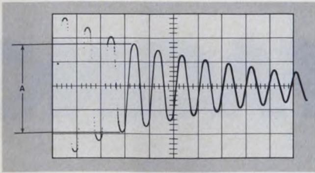
6. To avoid taking a series of exposures to find the writing speed, you can use a damped sinusoid and calculate the results from an equation.
