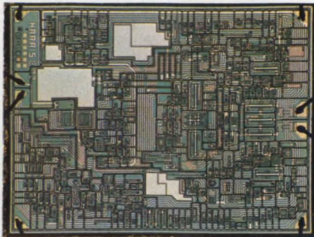
This monolithic chopper-stabilized amplifier, by Harris, has an offset voltage drift of only  $0.2 \mu\text{V}/^\circ\text{C}$ . Open loop gain is  $5 \times 10^8$ , bandwidth is 3 MHz and slew rate is  $2.5 \text{ V}/\mu\text{s}$ .
