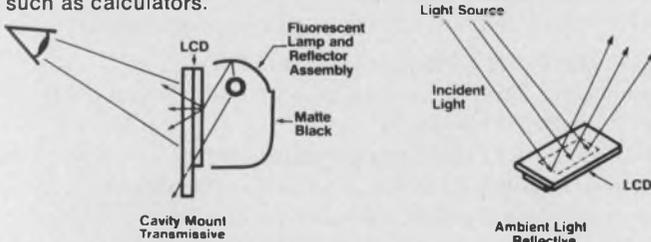
**Ambient lighting** (reflective displays) is the simplest of all arrangements, but the display should be mounted as closely as possible to the panel with minimum recess to receive maximum illumination. For good contrast, a dark background such as a matte black surface on the back plate should be used.
