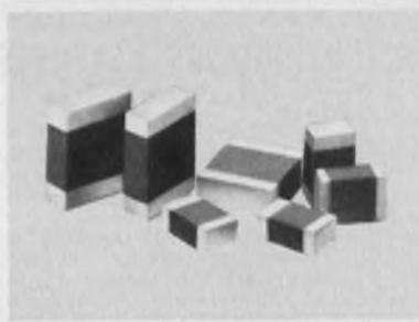
**HIGH Q MULTILAYER CAPACITORS** feature very high quality factors at microwave frequencies. Offered in three standard sizes: .050 x .040, .080 x .050, .125 x .095. Capacitance values from 0.1 pf to 1000 pf with close tolerance and voltages to 1000 VDCW. Johanson/Monolithic Dielectrics Div., Box 6456, Burbank, Ca. 91510, (213) 848-4465.
