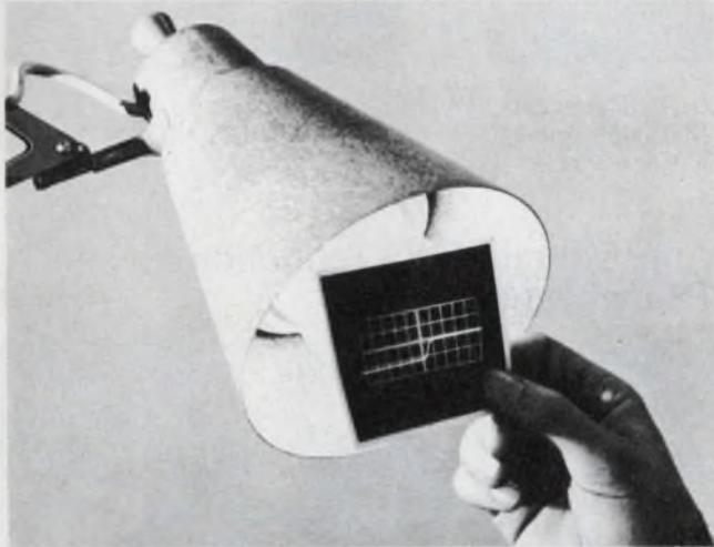
2. In backlighting, the developed film is illuminated from the rear and read by transmitted light, rather than reflected. Some film types can't be backlighted, however.
