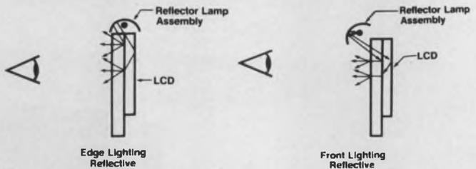
**Front lighting** (reflective design) uses incandescent lamps or a fluorescent (typically 3-watt). It provides the advantage of viewing with ambient light by day and artificial light at night.
