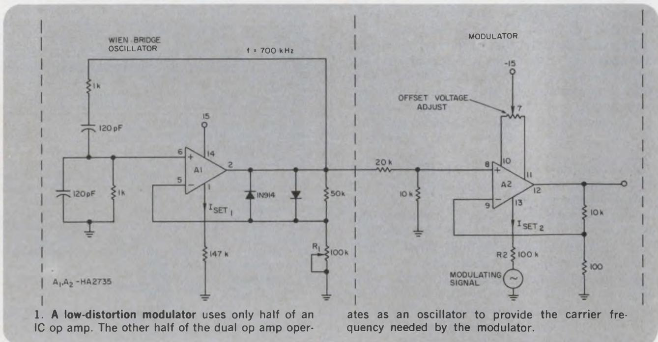
1. A low-distortion modulator uses only half of an IC op amp. The other half of the dual op amp oper-
