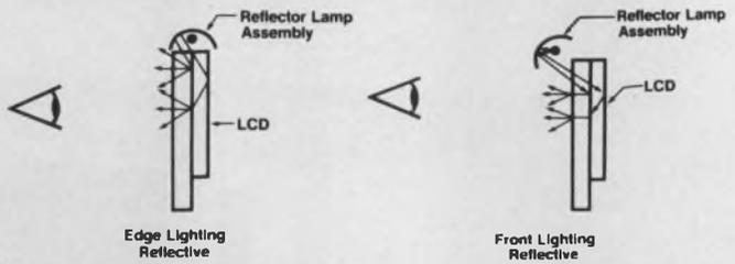
**Front lighting** (reflective design) uses incandescent lamps or a fluorescent (typically 3-watt). It provides the advantage of viewing with ambient light by day and artificial light at night.
