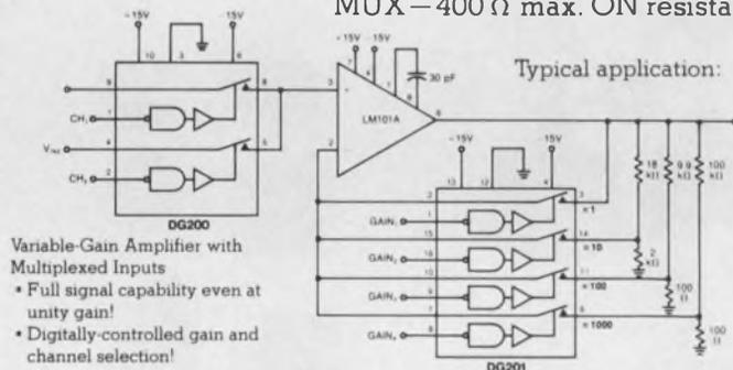
Variable-Gain Amplifier with Multiplexed Inputs
