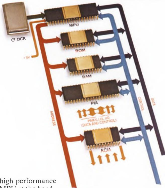
high performance MPU at the head of a modular LSI device series, totally bus compatible and fully compatible with each other.
