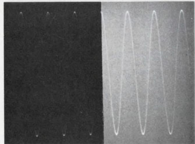
4. Two shots made under identical conditions show the effects of film fogging, that is, pre-exposure of the film. The left trace is hardly legible but appears clear and sharp after the film is fogged (right).
