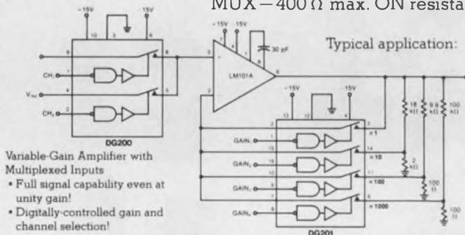
Variable-Gain Amplifier with Multiplexed Inputs
