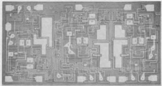
A new dual op amp designed for single-supply operation, Signetics' NE532, uses a Darlington input stage that can be driven slightly below ground ( $-0.3 \text{ V}$ ).
