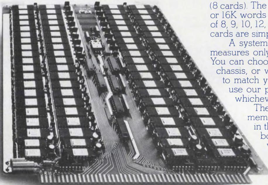
The most compact and most expandable low-cost memory system you'll probably see for years to come is Intel's in-40 dynamic RAM system. It's a true new generation design, available right now in standard models from 16K words to 256 kilobytes or in custom configurations with quick delivery.
