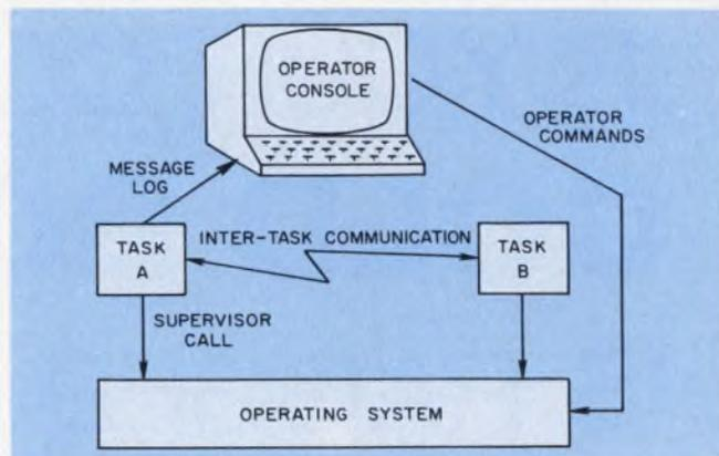
3. To operate successfully in real-time, individual tasks must communicate data with one another and possibly change the order of execution. Contact with the operating system to coordinate these activities is vital.
