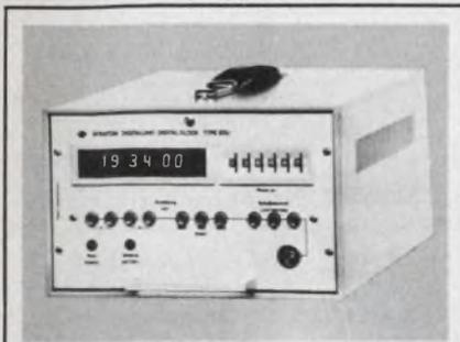
**DIGITAL CLOCK EDU**—High resolution timing unit for frequency standards e.g., our FRT. Accepts external sync. Displays hrs, min, secs, and leap sec. correction. Outputs BCD time data and IPPS timing ref. TTL. Time setting accuracy 500 nano-seconds. Efratom Cal., Inc., 3303 Harbor Blvd., El. Costa Mesa, CA 92626 (714-556-1620)
