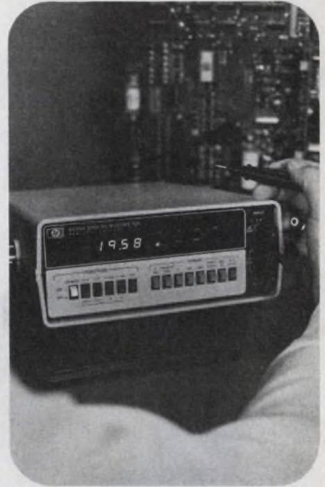
With new touch-hold probe, you can concentrate on your circuit, conveniently hold the measurement, and read the 3435's display after removing the probe. You are confident of measuring at the right point without accidentally shorting the circuit.
