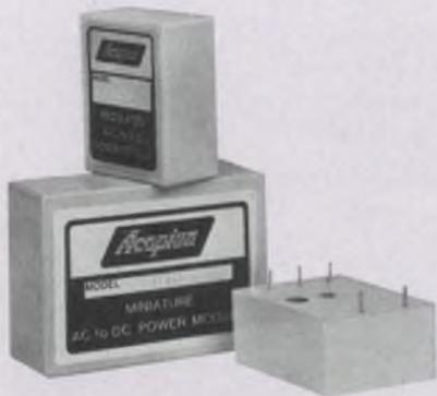
Mount these mini power modules, as small as  $2.3'' \times 1.8'' \times 1.0''$ , directly on printed circuit boards to save space and simplify wiring. Ratings at 5 volts from .250 to 2.5 amps; at  $\pm 15$  volts from .025 to .5 amps. Short circuit protected. Prices start at \$24. Guaranteed 3-day shipment.
