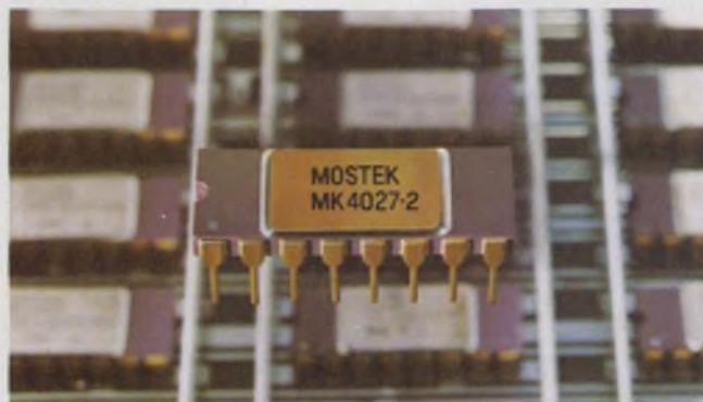
MOSTEK's 16-pin package reduces memory board size 50% over 22-pin packages.
