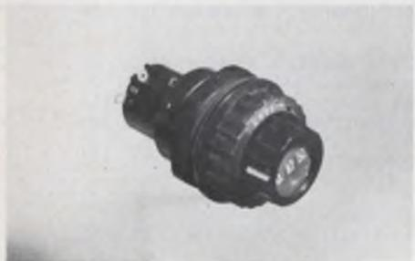
**NEW COMBO I, DIGITAL DIAL/POTENTIOMETER COMBINATION.** Order it with our potentiometer or yours. Dial has precision, gear driven numbers with magnifying lens. Low cost Model 850 potentiometer (pictured), with gold terminals, resistance tolerance  $\pm 5\%$ ; Ind. Linearity  $\pm 25\%$ ; Life expectancy 500,000 shaft revolutions, minimum. ELECTRO TECHNIQUES, INC., 215 Via Del Norte, Ocean-side, CA 92054. (714) 757-7770. TWX: 910-322-1396.
