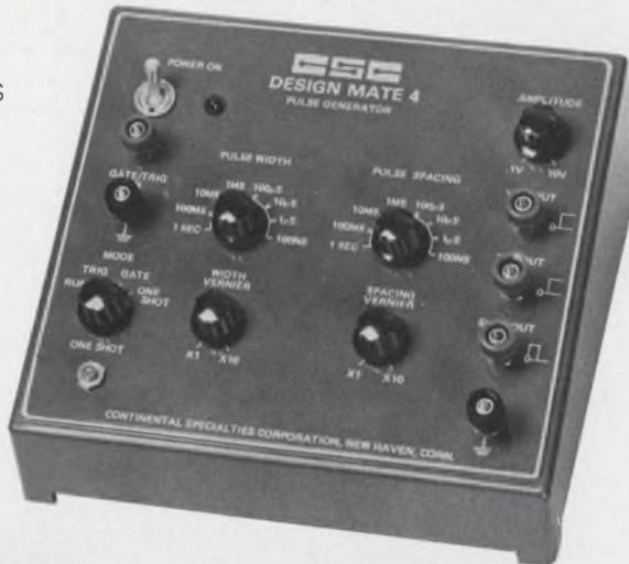
INDEPENDENT CMOS AND TTL OUTPUTS Fan-out to 40 TTL loads
