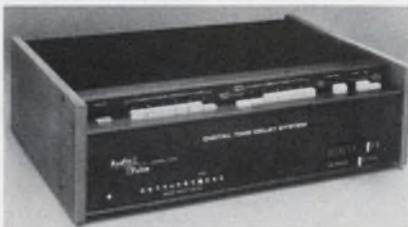
A digital time-delay system using computer technology, by Audio Pulse, expands and varies the sense of acoustic space in a listening room.
