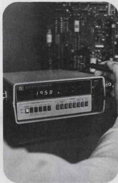
With new touch-hold probe, you can concentrate on your circuit, conveniently hold the measurement, and read the 3435's display after removing the probe. You are confident of measuring at the right point without accidentally shorting the circuit.
