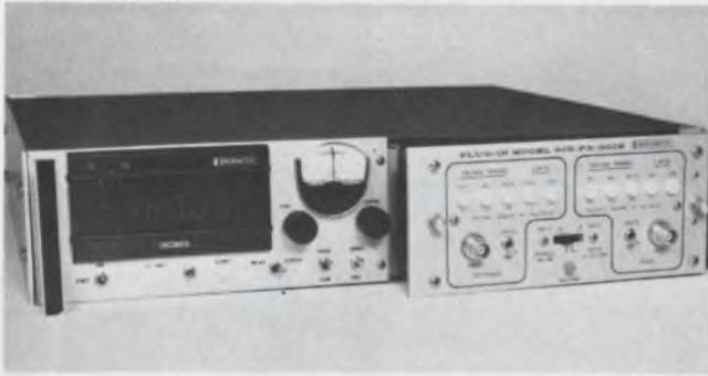
Digital readout of gain, phase and amplitude mark the Series 305, from Dranetz Engineering Laboratories. The autoranging unit works to 700 MHz.
