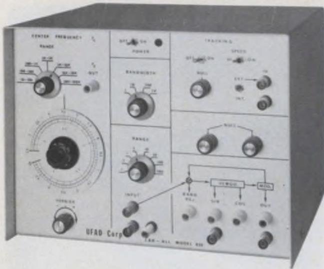
Besides producing network-transfer Nyquist plots on an external scope, the LAB-ALL functions as 10 or 11 other test instruments (UFAD Corp.).
