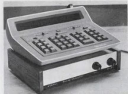
The readouts of a Monroe 1920 calculator are deciphered by a  $\mu$ P to control a 35-word vocabulary in this Wespro talking-calculator system.
