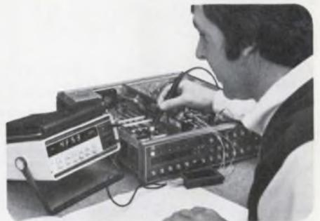
Many of HP's new  $\mu$ P-based instruments and data products utilize the Signature Analysis technique for economical component-level troubleshooting in production and service.
