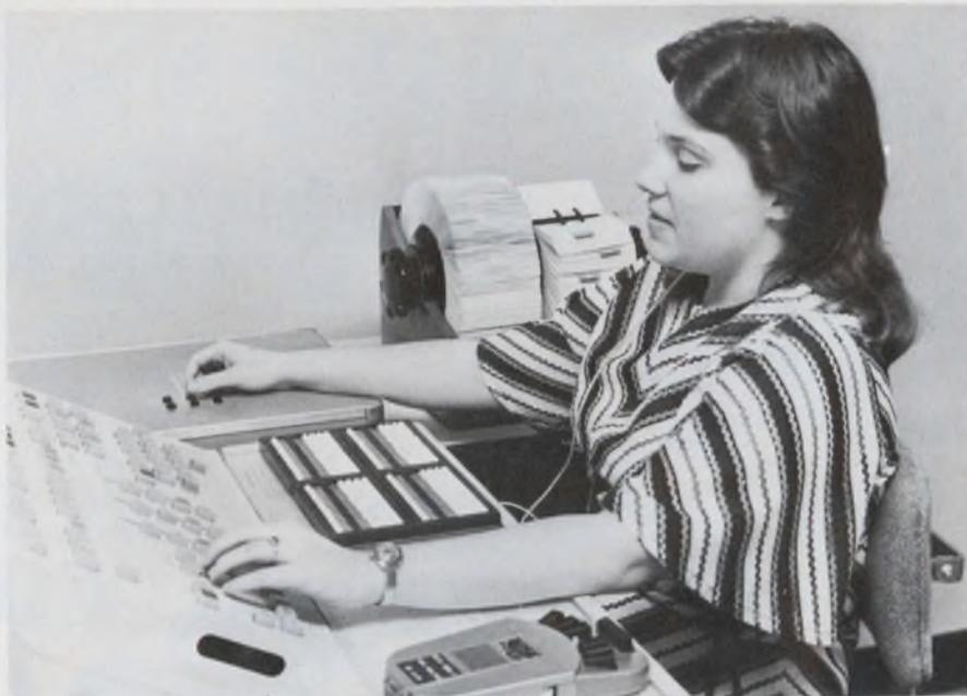
**A system that allows a blind person to work as a long-distance operator** is the outgrowth of a calculator for the blind designed at MIT. Information from 82 switchboard keys is fed to a Motorola 6800, which converts it to 12-character Braille messages at this Little Rock, Arkansas, installation.
