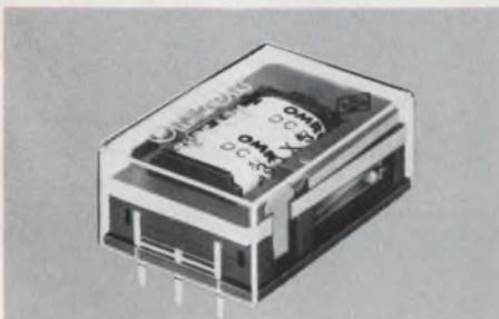
**OMRON LOW PROFILE DRY CIRCUIT RELAY** Reduces contact resistance for stringent low-voltage/low-current circuits, switches up to 3A at 24 VDC. Offers DPDT or 4PDT format, packaged to fit PCBs on 1/2" centers. High reliability, with 100 million mechanical operations (min.) with bifurcated cross bar contacts. Plastic covers can be sealed for wave soldering, with air or nitrogen filling. OMRON ELECTRONICS, INC., 233 South Wacker Drive, Chicago, Ill. 60606 Phone (312) 876-0800.
