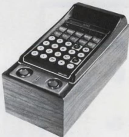
**A Braille readout is provided** on this calculator by the American Foundation for the Blind. It has a variable speed control that enables the user to read as slowly as one digit every four seconds. It sells for \$425.
