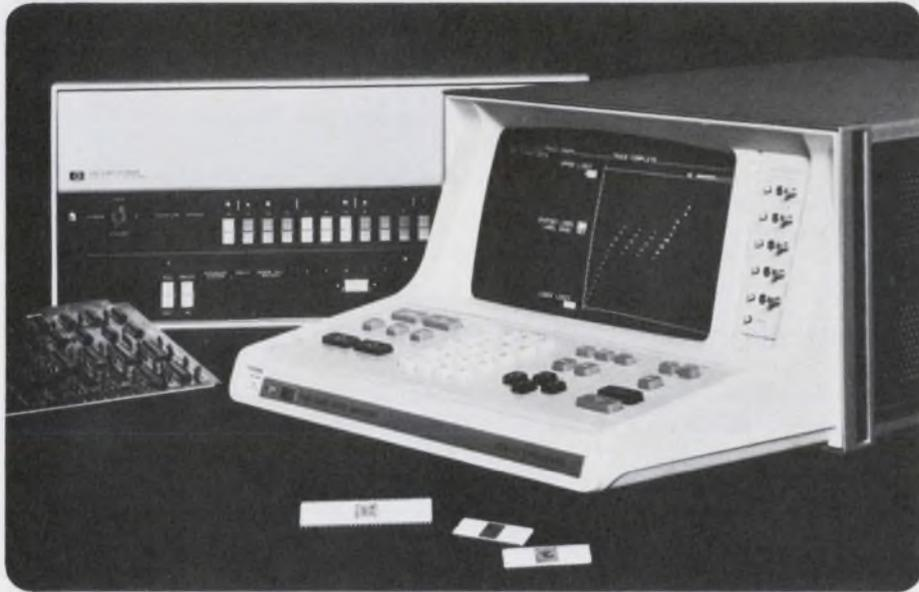
The new HP 1610A logic state analyzer is designed to efficiently test digital systems ranging from the simplest logic circuits to microprocessors and computers. Keystroke retrievable testing and display programs offer such test formats as numerical trace listing, data magnitude versus time graphs, and a comparison between current and stored measurements.
