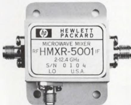
New double balanced mixer is intended for frequency conversion use in electronic surveillance systems, instrumentation and test bench set-ups.
