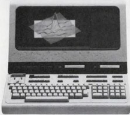
The latest in microprocessor and raster scan technology are combined in Hewlett-Packard's new 2648A Graphics Terminal to produce a high performance, low-cost and bright display terminal that aids the user in many graphic application areas.
