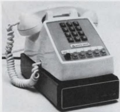
With the 212A modem Bell has anointed the concept of 1200-bps data communications. Users are helped in making the switch from 300 bps since lower-speed circuitry is also included in the unit.
