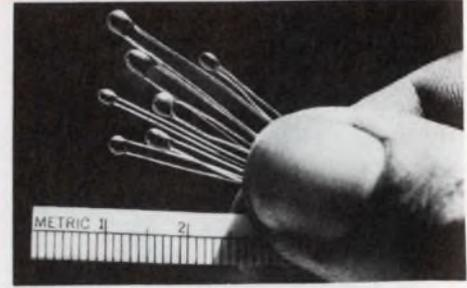
**THERMISTORS** with leads and coating are highly reliable low cost components in small dimensions more compatible with modern circuit design. R @ 25°C 100Ω to 1 meg Ω ±10% to ±1%. CURVE MATCHED INTERCHANGEABLES to ±.25°C. POINT MATCHED INTERCHANGEABLES to ±.2°C. Call or write for HP97 or TI SR52 THERMISTOR LINEARIZATION PROGRAM. WESTERN THERMISTOR CORPORATION, 354 Via Del Monte, Ocean-side, CA 92054. (714) 433-4484.
