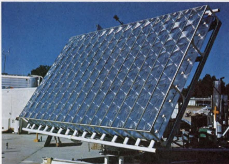
Generating 1000  $W_p$ , this two-axis tracking array uses fresnel lenses to concentrate solar energy 60 times. Lenses are 80% efficient; grooves are turned inward to prevent dirt from accumulating.
