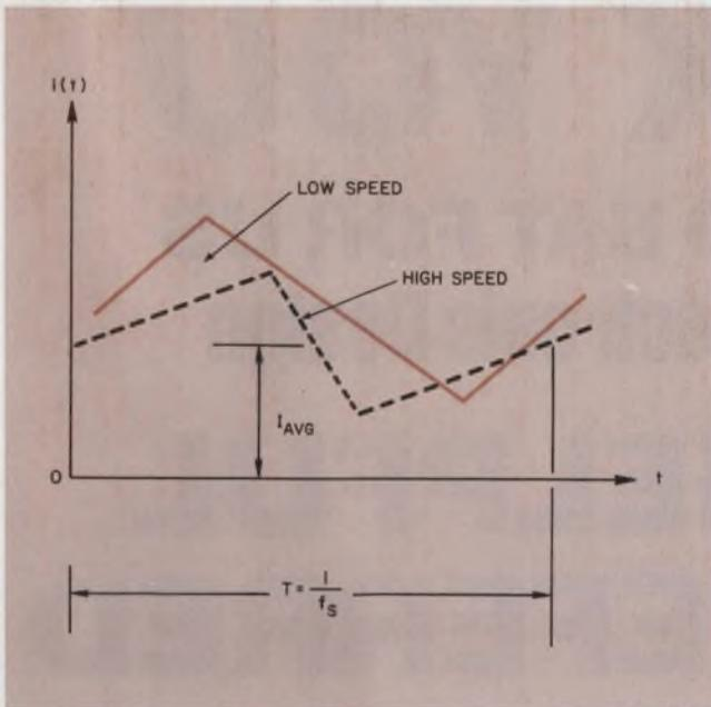
5. **Ripple current in a servo motor is a function of motor speed.** With constant frequency control, ripple current is large at low motor speeds, increasing motor heating. But current must circulate through a motor at all times to prevent a system dead zone.
