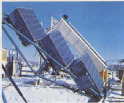
**This two-axis, three-section tracking concentrator** generates 300 W<sub>p</sub>, and uses a solar-powered  $\mu$ P and stepping motors to follow the sun. RCA expects this "fly's eye" concentrator to cost \$1/W<sub>p</sub> in volume quantities.
