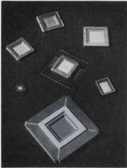
A 68-lead IC-chip carrier, lower center, has been developed by 3-M to be one of the new 50-mil centerline LSI packages being standardized by JEDEC. Chip carriers are also shown.
