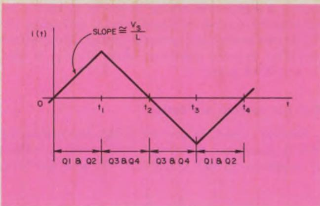
3. Instantaneous current in a servo motor is a triangular waveform whose average value is zero. Pairs of switching transistors in an SSA's power amplifier drive current to the motor through a fixed inductor to generate a triangular waveform.
