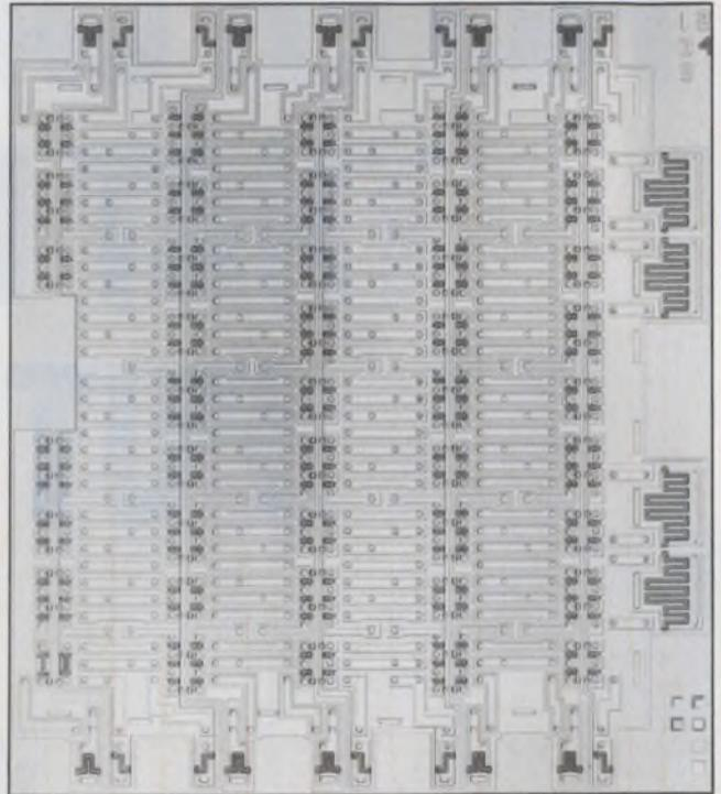
**Typical of uncommitted digital arrays**, this MasterMOS Model S chip contains 106 p-channel and 106 n-channel transistors, 10 medium-power buffers, four large n-channel devices with high-current capability, and one p-channel and one n-channel high-impedance device. The chip is 65 × 74 mils, with pads of 4 × 4 mils.
