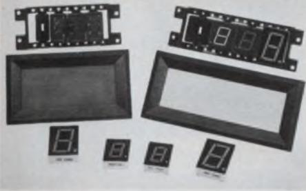
**ATLAS MOUNTING HARDWARE FOR LED DISPLAYS** Series 1750/51 accommodates most mfr's 0.3" to 0.5" character LEDs; Series 1752/53 accepts 0.6" to 1.1" characters. This versatile, unitized plug-in pkg comes complete w/ front bezel containing a hi-contrast, non-glare filter, and self-contained socket assy holding up to 8 displays. Ea. socket accepts up to 18-pin DIP pkg w/ optional .3" or .6" vert. pin row spacing. Avail. immed. IEE, 7740 Lemona Ave., Van Nuys, CA 91405, (213) 787-0311, ext. 268.
