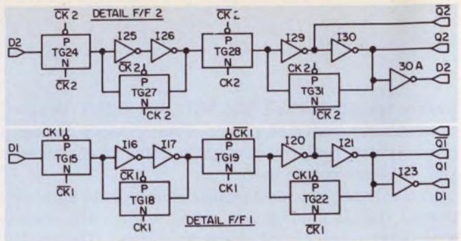
Designing a circuit with an uncommitted array can be broken into three steps. Start with the logic diagram of the circuit (left), which in this example is a four-channel scanner, and then transform the logic diagram into a discrete device diagram (above) so that the metal interconnect patterns can be defined (below).
