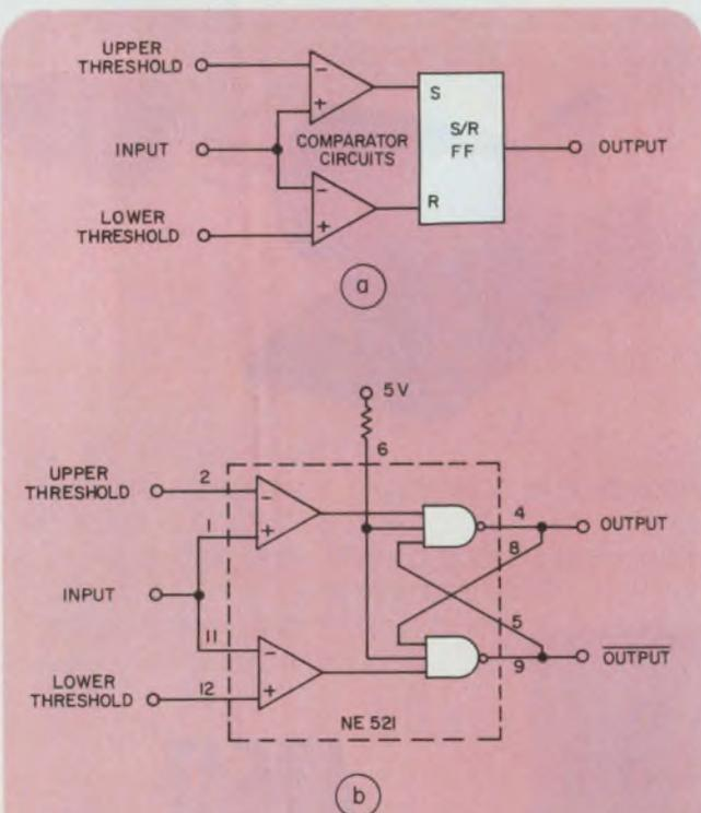
1. A set-reset flip-flop allows hysteresis to be introduced into a comparator circuit. And the threshold levels of the dead band can be set independently of each other.
