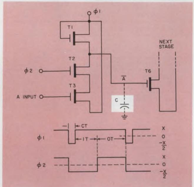
1. In a four-phase inverter, the inherent small capacitance of the next stage's input charges during time  $CT$  of clock  $\phi 1$ . The state of this capacitance is determined, during the input time ( $IT$ ), by the condition of the logic input  $A$ . During the output time ( $OT$ ), the output—the state of  $C$ —transfers to the next stage.
