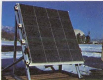
**A nontracking, solar concentrator** uses high-density strips of cells and parabolic reflectors to generate 100 W<sub>p</sub>. (Argonne National Laboratory).
