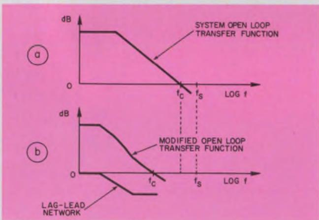
4. Servo-system performance can be modified by a compensation network. The open-loop transfer function (a) indicates an unstable system. A lag-lead network shifts  $f_c$ , the zero-dB crossover frequency, to a lower value, and restores stability to the system as shown in the modified transfer function (b).
