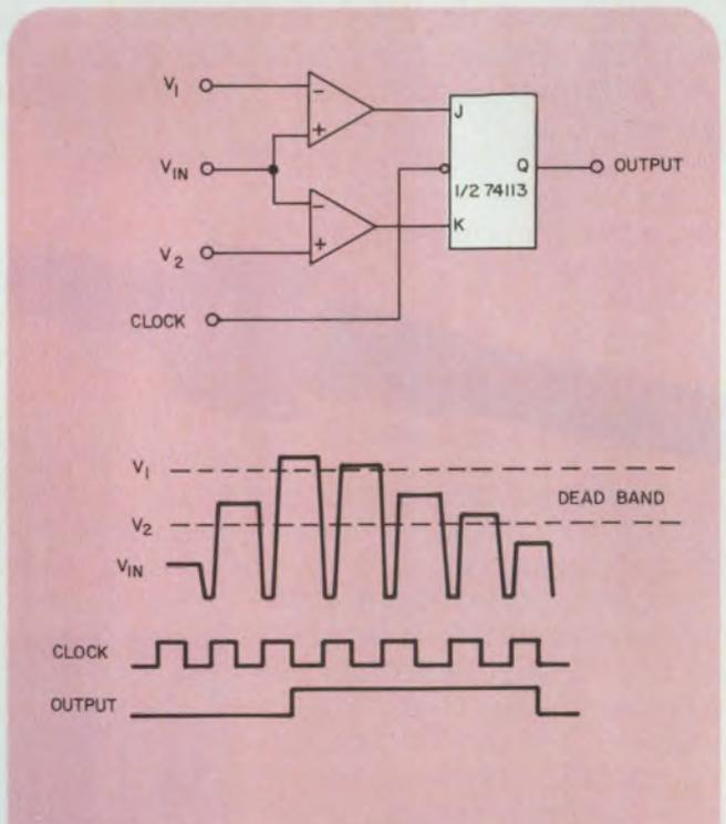
2. A j-k flip-flop following the comparators allows the circuit to be clocked to synchronize input data. In addition to hysteresis from the comparators, clocking helps reduce noise rejection even further.
