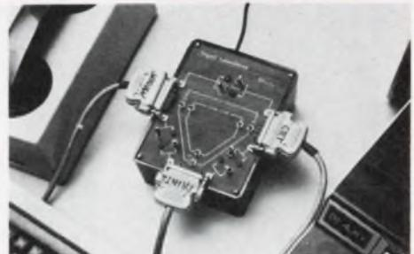
**UNIVERSAL JUNCTION UNIT** . . . for three devices, RS232C or current loop.
