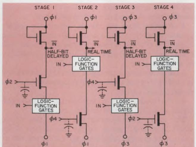
2. Four-phase logic requires the use of four stage configurations. The rules for stage interconnection are relatively simple. Besides, the different stage delays add logic flexibility, and available computer programs can easily obey all the rules consistently.
