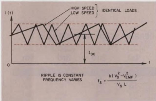
6. **Ripple is constant**, regardless of motor speed with a constant ripple controller. However, frequency variations can lead to instability in position servos.
