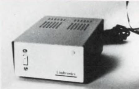
**TRIPLE OUTPUT REGULATED DC SUPPLY** — compact DC supply ideal for micro-processor and memories, Model 477-3 supplies 5V @ 500 ma, +12V @ 100 ma and -5V @ 200 ma regulated outputs, input 110V 60Hz, the unit is enclosed in a compact steel case and complete with AC line cord with fuse. Unit price \$24.00. Lindtronics, P.O. Box 1792, North Brunswick, N.J. 08902.
