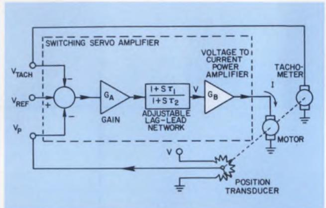
1. A complete servo amplifier is housed in a single switching servo amplifier (SSA) package. Depending on feedback elements, either a position or velocity servo can be built. In the SSA block,  $G_B$  represents not only the power-amplifier stage but also the control electronics section that provides drive signals.
