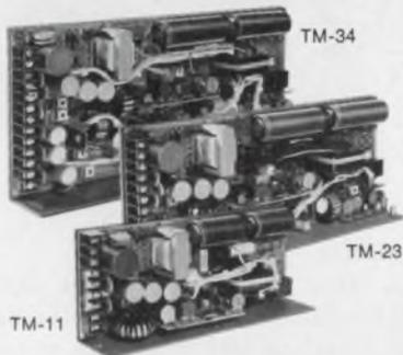
LH's low-cost, single- and multiple-output Tiny-MITE switchers are perfect choices for high-volume OEM computer and terminal applications. TM-11 packs 100 watts in a 9.5" L x 4" W x 2.5" H package. TM-23 packs 150 watts in 12" L x 5" W x 2.8" H. TM-34 packs 175 watts in 13.0" L x 6" W x 2.75" H.
