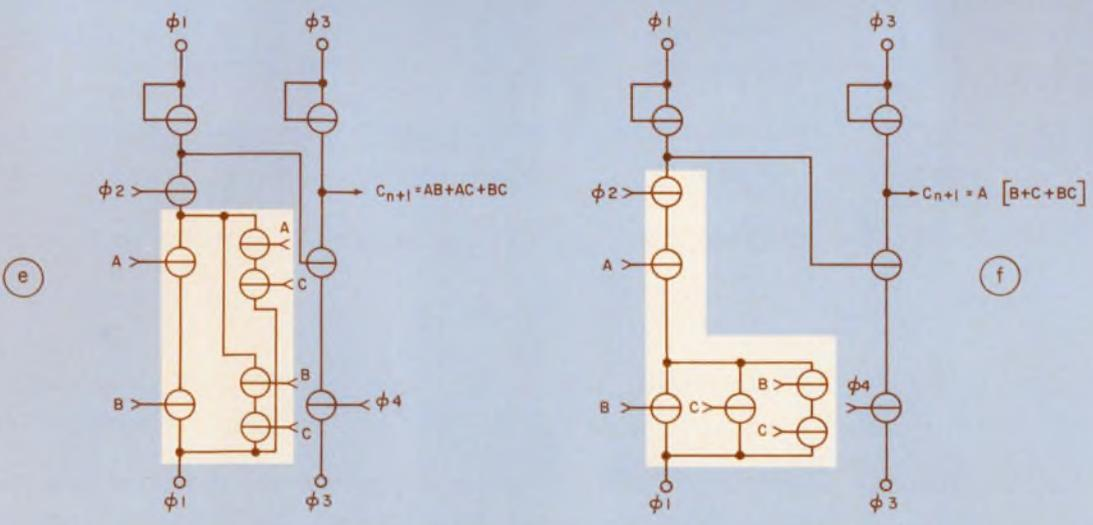
5. A two-bit full-adder design example is taken through the suggested design steps from truth table (a) and Karnaugh map (b) to variations of the design—direct
