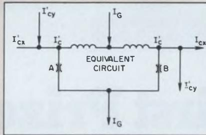
current  $I_G$ , and by two control lines that are inductively coupled to the cell. One control line,  $I_{CX}$ , is at right angles to the word line,  $I_G$ , while the other control line,  $I_{CY}$ , runs in a staircase pattern through a matrix of cells.
