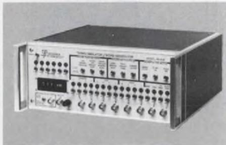
**RS-648 Timing Simulator/Word Generator** is intended for lab use by engineers and technicians who are debugging digital circuitry or for production testing. It provides eight output channels and 16 memory words and is programmable to allow users to simulate exactly the desired timing signals or data transfers needed for device test. From Interface Technology, 852 North Cummings Road, Covina, CA 91724. (213) 966-1718.
