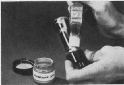
ECCOCOAT® 341 is a moderately conductive surface coating based on silver and epoxy. Pricing is far below that of silver lacquers. Has excellent weathering characteristics and is resistant to salt spray. Can be air dried at room temperature.
