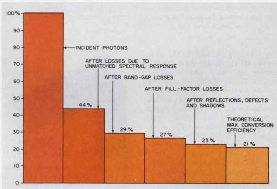
Even the best solar cells won't reach more than 21% conversion efficiency, according to theory. Today's devices range from 8 to 18%.
