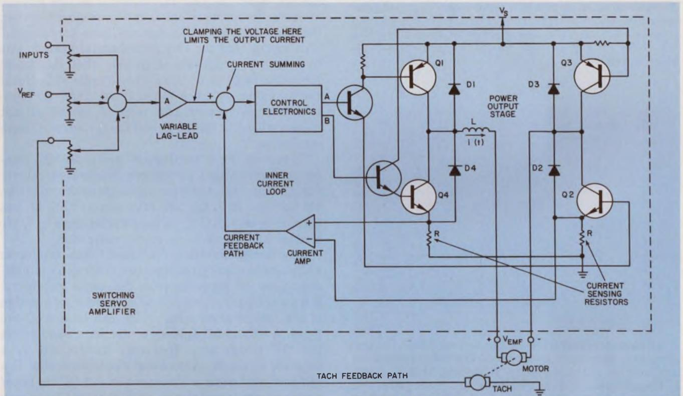
2. Motor drive in an SSA is provided by an "H" bridge. Alternate pairs of switching transistors,  $Q_1$  through  $Q_4$ , allow current to flow in the motor in two directions. An "H" bridge is a current source that senses current flow
