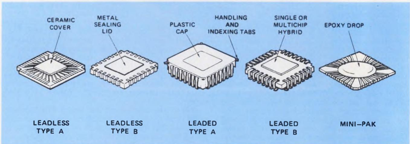
New LSI IC packages proposed by JEDEC have features shown above. One style has leads on 50-mil centers and
