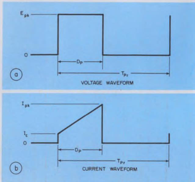
1. A trapezoid of current (a) results when a square wave of voltage (b) is impressed on an inductor. The initial jump of current,  $I_c$ , ramps up to the final value,  $I_{pk}$ , with a slope that depends on coil inductance and resistance.
