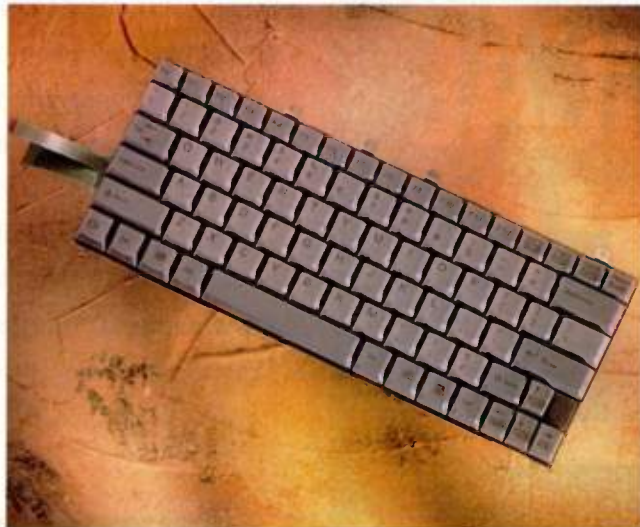
1. The FKB7600 series of 85-key keyboards has a vertical height of just 6.5 mm. However, it retains a 3-mm, full-travel keystroke by employing a gear-link mechanism in the keyswitch.
