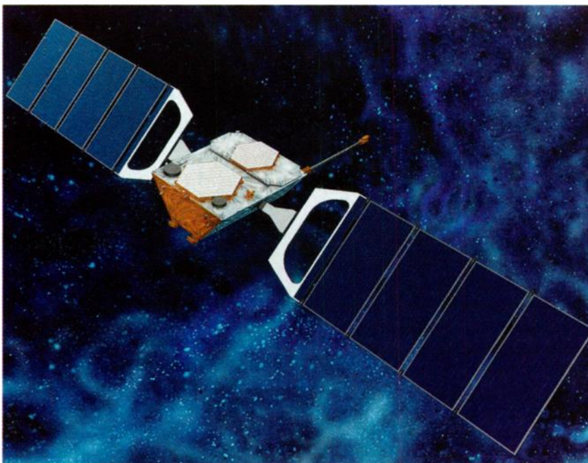
Shaped like a trapezoid, the compact, lightweight Globalstar satellite is a heavyweight when it comes to lifting payloads into orbit. Totalling just 1000 pounds itself, Globalstar can handle payloads of 484 lb. and 36 cubic ft. in volume.
