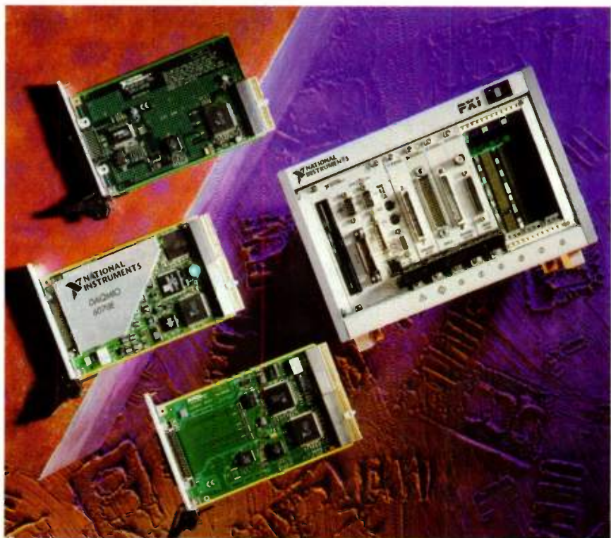
1. The PXI instrumentation architecture is based on the CompactPCI form factor. A basic mainframe holds a controller in from one to three slots and up to seven instrumentation modules.
