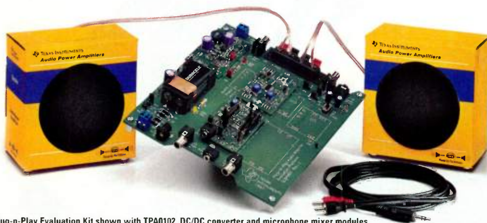
Plug-n-Play Evaluation Kit shown with TPA0102, DC/DC converter and microphone mixer modules
