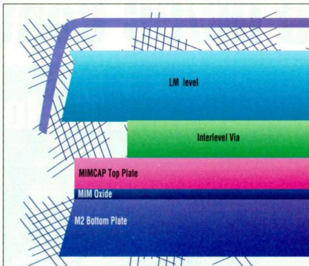
1. This SEM cross-section of a corner of a SiGe HBT shows the MIM/dc capacitor IBM developed for the process.
