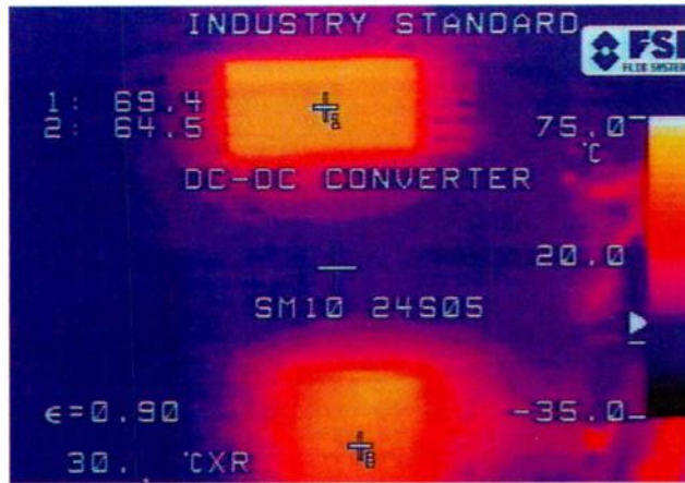
2. The result of this new design for surface-mount dc-dc converters is highly effective thermal dissipation, allowing only a minimal temperature increase between the converter and the card. Furthermore, this rise is consistent, as there are no significant hot spots caused by the convection scheme.
