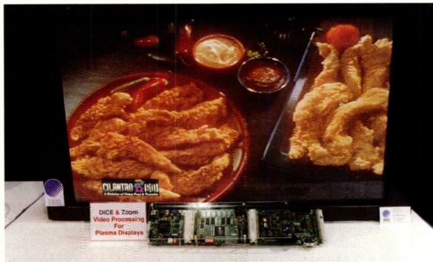
2. Genesis Microchip's HDTV plasma chip set utilizes a Fire Wire interface and offers a potential solution to the problem of digitally interfacing to a TV for digital TV (DTV) applications.
