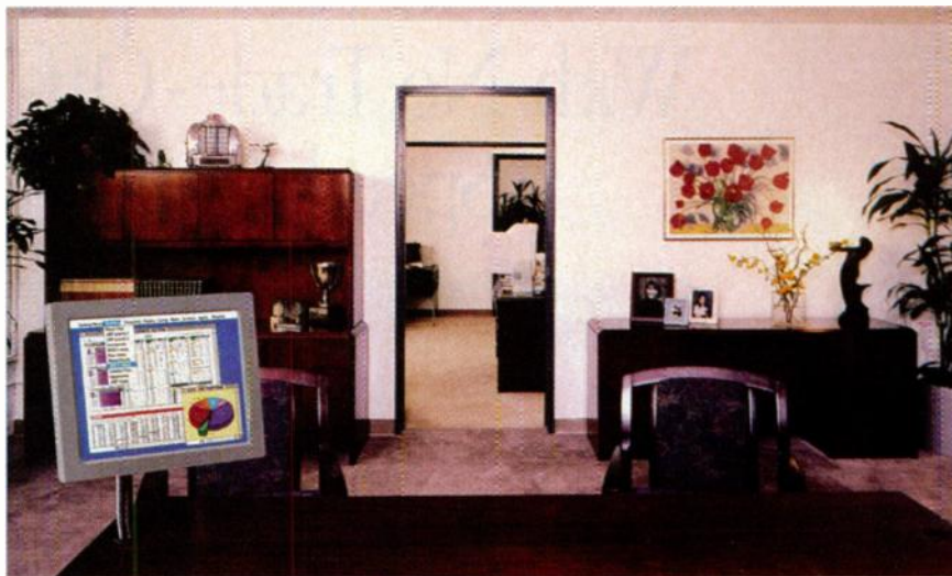
3. Encapsulated color gives NEC's 42-in. 853-by-480-pixel plasma-panel display a brightness of 200 Cd/m 2 . To produce colors, each pixel has a tiny color filter, much like an LCD.
