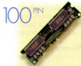
100-pin DIMMs 16-, 8- and 4-MB Unbuffered 32-bit I/O
