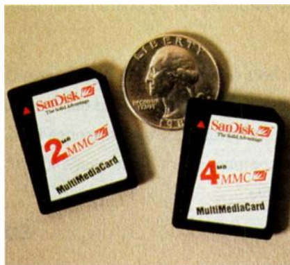
1. A MultiMediaCard (MMC) like these two from SanDisk, is about the size of a postage stamp. A concept developed by Siemens Semiconductor, it's supposed to fill the gap between PC cards and chip cards.
