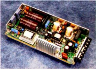
A typical 100 watt single voltage bolt-down power module, Series FAW
