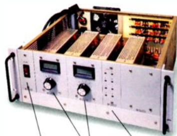
Circuit Breaker 2 DVMs w/selector LEDs
