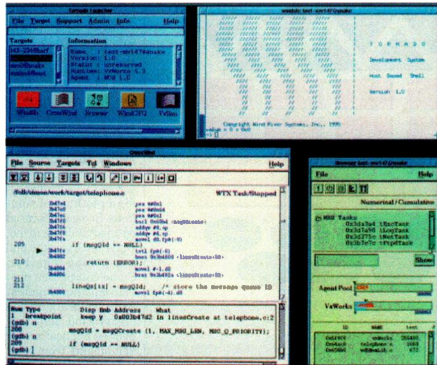
1. Tornado, from WindRiver Systems, is an integrated, cross-development environment for embedded systems. It consists of three major integrated components: a set of Tornado plug-in tools; a set of cross-development tools and utilities; and the VxWorks run-time system that includes the VxWorks real-time operating system, and a range of host/target communications such as Ethernet, a serial port, and an in-circuit emulator (ICE).
