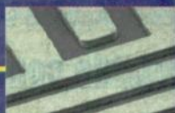
MAGNIFICATION: 1.21KX 5 Micron Conductors 5 Micron Spaces
