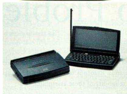
2. The Novatel Minstrel CDPD modem adds wireless Internet access and messaging capabilities to a pocket organizer (a). Palmtop computers can also easily go wireless, using PCMCIA-based modems or embedded modules (b).
