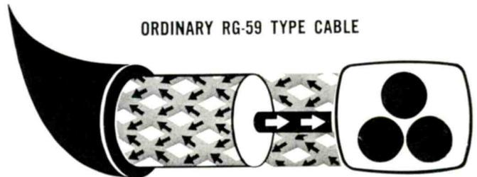
While current in the center conductor flows in a straight line with minimum resistance, to complete the circuit between set and antenna, return current must traverse individual braid strands in a "maze" pattern that creates a resistance loss. In lower grade standard coax with fewer strands, this loss is even greater.
