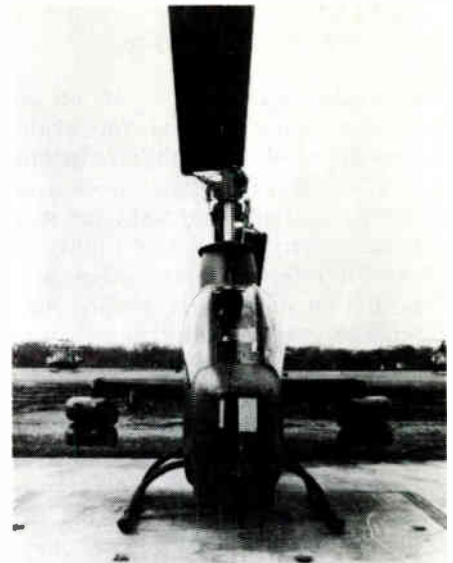
Photo Courtesy Hughes Aircraft Company New sting for the cobra — A HueyCobra attack helicopter with new TOW anti-tank missiles in launcher pods on each side.
