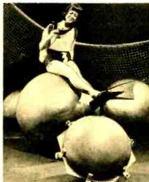
body'd want to send down to probe the mysteries below. They already have proven their worth in an experiment conducted by California U. Serving as bathyspheres for seismometers, the metal globes helped gather valuable data on the origin and propagation of earth tremors in the waters of the Central and South Pacific.
