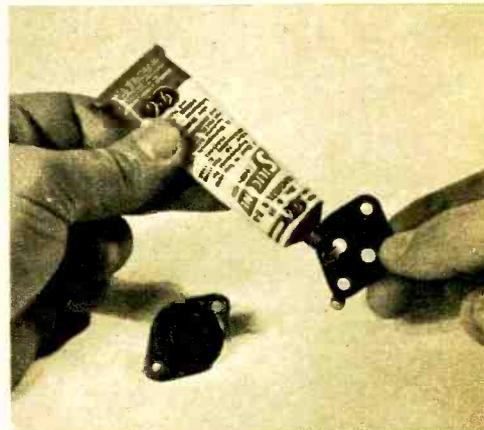
Silicon compound (GC's Silicone is one) can prevent a non-electrical CC. Spreading compound on transistor heat-sink before installing transistor usually will increase heat dissipation markedly.
