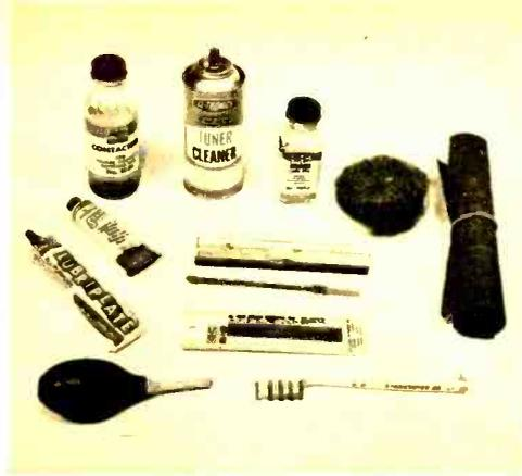
Though some of these cruddy-contact decontaminators are optional, others pretty much are necessities. Among the latter are a solvent, a lubricant, a crocus cloth and fine steel wool.
