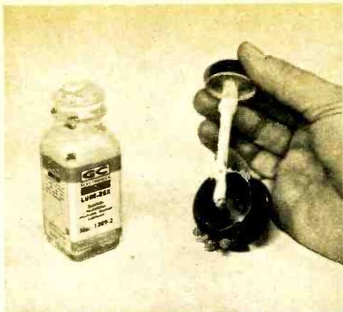
Light lubricant (this is GC's Lube-Rex) applied to wirewound controls reduces electrical noise, prevents oxidation. Control's rear cover must be removed if wirewound element isn't accessible.
