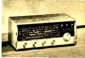
built-in antennas for the long- and short-wave bands, this versatile 5-tube tunes 150 kc through 400 kc and 500 kc through 30 mc in five bands. Other features include a BFO, electrical bandspread and provision for operation on either 117 or 230 V at the flick of a switch. \$99.95. Zenith Sales Corp., 1900 N. Austin Ave., Chicago, Ill. 60639.
