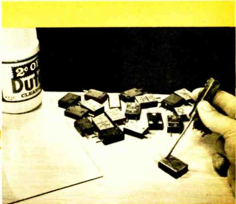
Necessary equipment for raising a crystal's frequency consists of a piece of glass and a can of cleanser. Crystal can be exposed by loosening three screws on case; take case apart slowly and carefully, keeping label side face up.
