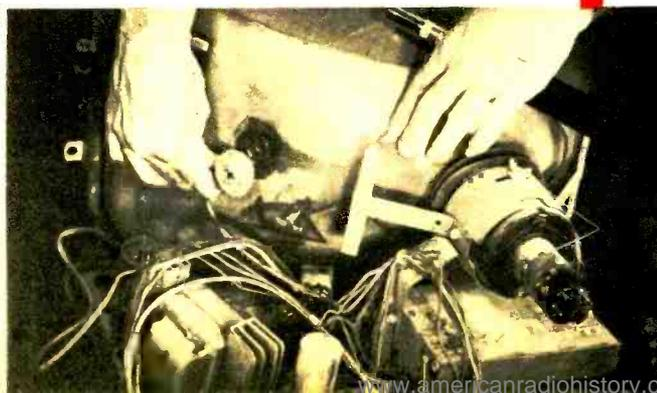
High-voltage anode lead unclips from small well on side of picture tube. Screws or bolts holding tube to chassis also must be removed.
