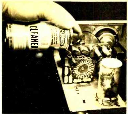
Tuner cleaner is good general-purpose solvent for cleaning all sorts of CCs, including channel-selector switches on CB transceivers. Apply short spray burst to both sides of each switch wafers.
