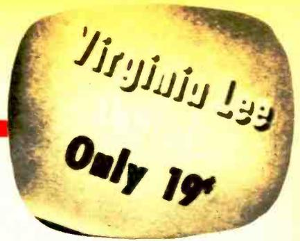
Tilted picture can be righted by rotating yoke and watching mirror. Clean CRT mask and glass before re-installing in front of new pic tube.
