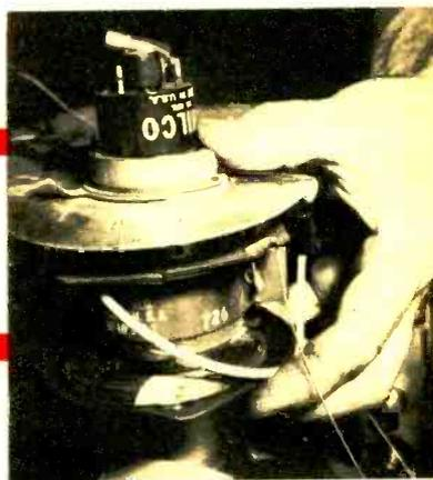
Ion-trap centering devices (if present) and yoke (if mounted on CRT) must be slid off neck of tube. As in other steps, keep track of order in which individual operations are performed since procedure will be reversed during reassembly.
