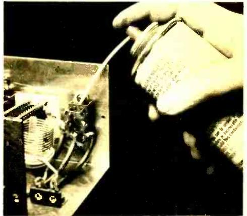
Thin tube fitted over nozzle of solvent-spray can carries spray into concealed contacts inside slide switches, carbon potentiometers. Technique is to insert tube in case opening, then blast away.
