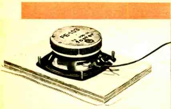
Fig. 6—When the grille-cloth glue dries, trim the excess material to  $\frac{1}{2}$  in., then fold it and glue or staple to the panel edge. Note the large size of the speaker's magnet. At right is completed cabinet ready for installation of the fiberglass wool and the panels.
