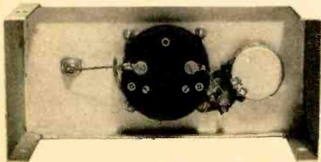
Fig. 6—FSM remote is built in a 2¼ x 2¼ x 5-in. Minibox. Parts placement is not critical. Connect it to Tester with RG174/U coax cable.
