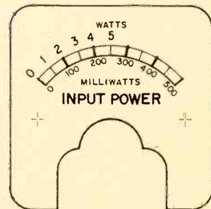
Fig. 6—Meter is calibrated in milliamperes, but if you paste this scale over its scale, you'll be able to read the rig's input power directly.
