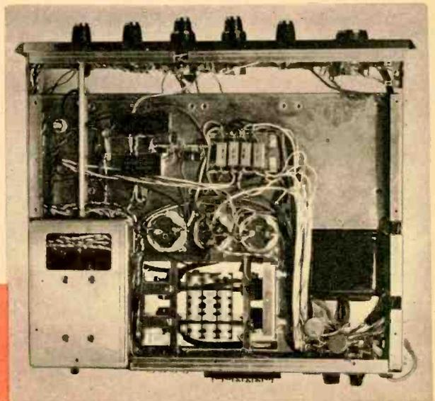
Underside of LK-60 is exceptionally clean. Pre-amps are enclosed in shielded compartment in lower left corner. Input selector switch also is located in compartment and is coupled to the unit's front-panel knob with the extra-long shaft.
