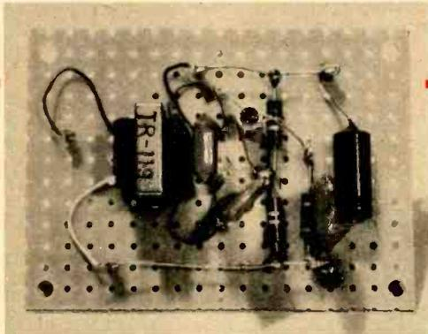
Fig. 3—Modulator is built on a 2 7/16 x 3 3/8-in. piece of perforated board. Drill holes in corners and mating holes in cabinet bottom for mounting.
