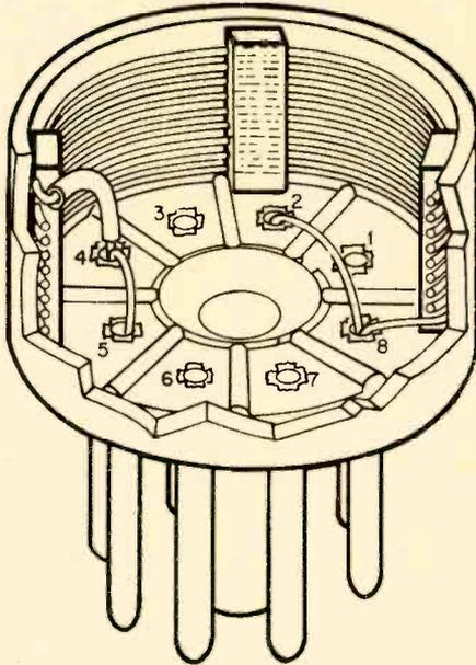
Fig. 4—Pictorial of 20-meter coil. The three diagrams at the right of the schematic in Fig. 2 show pin connections of coils and the jumpers.
