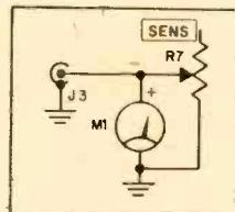
Fig. 5—When S1 is set to "osc" position, power is applied automatically to modulator and oscillator. When plug goes in J1 for audio tests, RF oscillator goes off. Setting S1 to "fsm" removes power from modulator and oscillator and connects antenna to FSM. Schematic of FSM remote indicator is in the box at the right.
