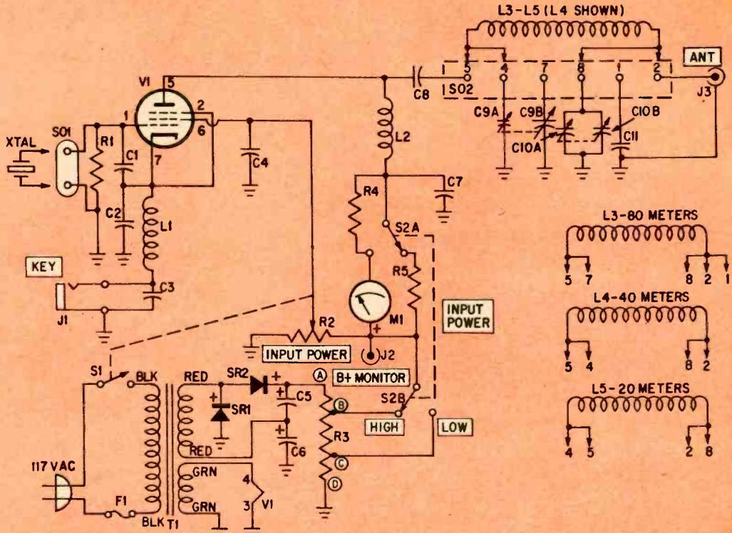
Fig. 2.—Transmitter schematic. S2 determines input power. When it's set to "high" (shown), high B+ is supplied to V1 from tap "B" on R3. When S2 is set to "low," lower B+ is supplied to V1 from tap "C." R2, which establishes V1's screen voltage, is used to vary the input power continuously in both ranges. 80-meter coil, L3, is 33 turns. 40-meter coil, L4, is 17½ turns. 20-meter coil, L5, is 8½ turns. (See Fig. 4.)
