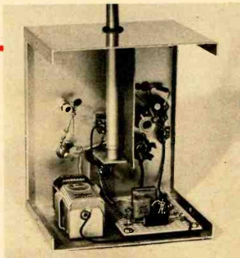
Fig. 2—Antenna hole is  $1\frac{3}{8}$  in. back from front of cabinet. Put grommets between board and bottom of cabinet. Put tape on cabinet under board.
