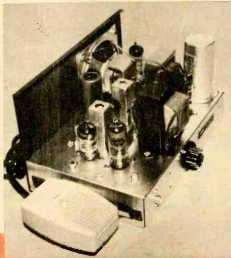
Rear view of GW-12A. Single-channel operation means no tuning capacitor. Octal plug is for AC line cord or for 6/12-VDC vibrator power supply.
