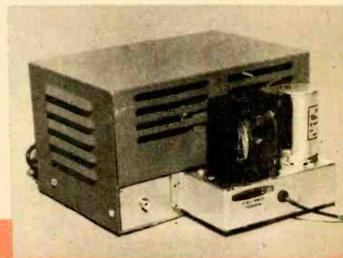
Model GW-12D transceiver includes vibrator power supply for 6 or 12 VDC operation. Supply is bolted to rear of chassis but can be removed.
