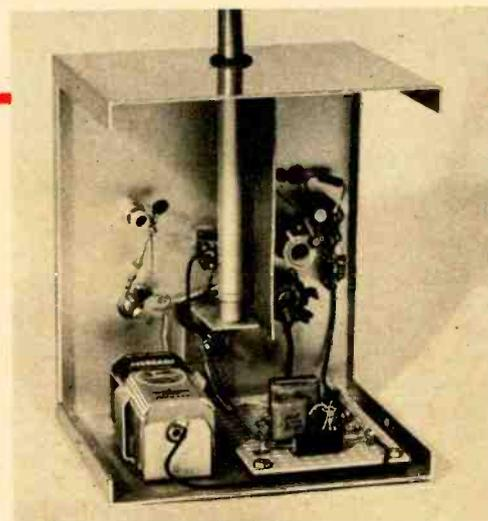
Fig. 2—Antenna hole is 1 3/8 in. back from front of cabinet. Put grommets between board and bottom of cabinet. Put tape on cabinet under board.
