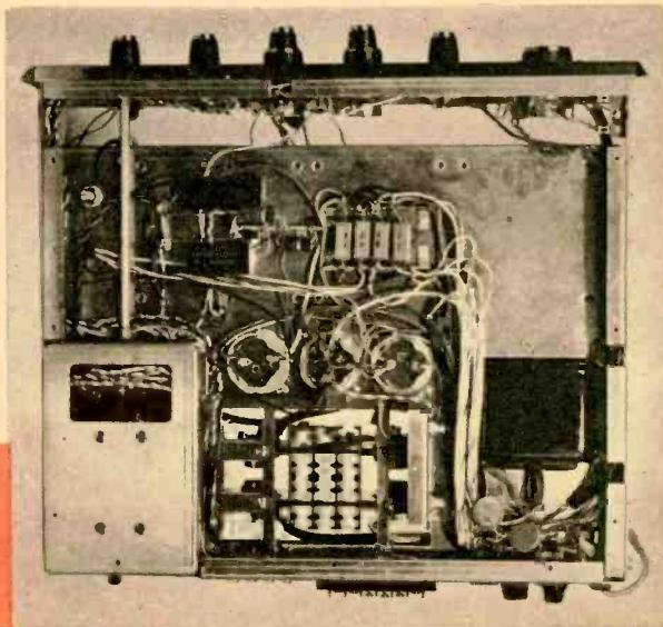
Underside of LK-60 is exceptionally clean. Preamps are enclosed in shielded compartment in lower left corner. Input selector switch also is located in compartment and is coupled to the unit's front-panel knob with the extra-long shaft.
