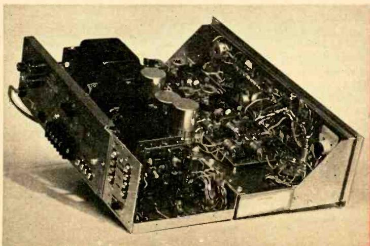
Reason the LK-60 looked so clean under the chassis is because of high parts density on top. However, all circuit boards are supplied precut and tested. Bulk of the work is the interconnecting wiring between boards and switches. Low-level preamp boards are mounted vertically in lower-left corner and are enclosed by a shield cover. Black objects between power transformer and preamps are heat sinks for the output transistors.
