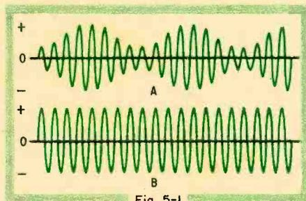
plate-current changes which would correspond precisely to the level of modulation. Not so! While *instantaneous* plate current faithfully would follow the ups and downs of individual cycles of the carrier voltage, *average* plate current would not change with the comparatively slow undulations in overall carrier amplitude that modulation produces. Here's why.
