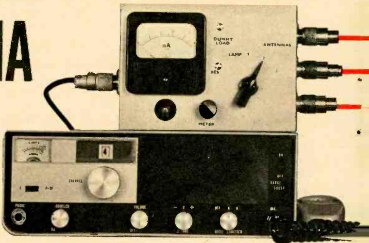
*Twist a switch for your choice of three skyhooks or two dummy loads.*
