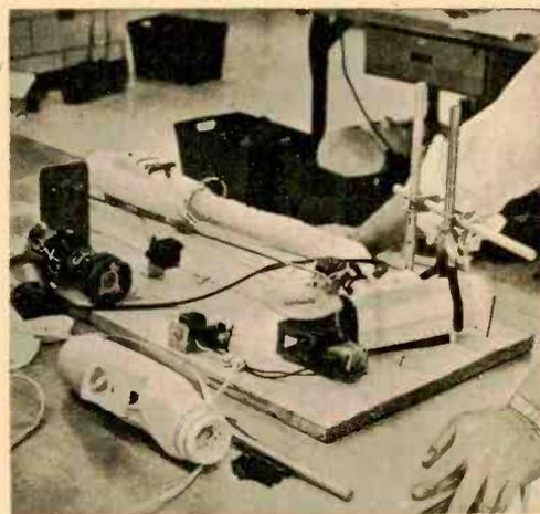
Switch on hair dryer is turned on and off continuously to determine duty cycle. Commercial testers often are not available, so UL makes its own.
