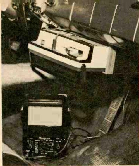
The job is done. The recorder is about 3 in. deeper than the chassis; therefore, operating push buttons, level meter, volume control and speaker will protrude just the right distance. Cement a small magnet on back of mike so it can be held to dash when not in use. To remove recorder for use in home, loosen underchassis screw, disconnect power plug and slide unit out.
