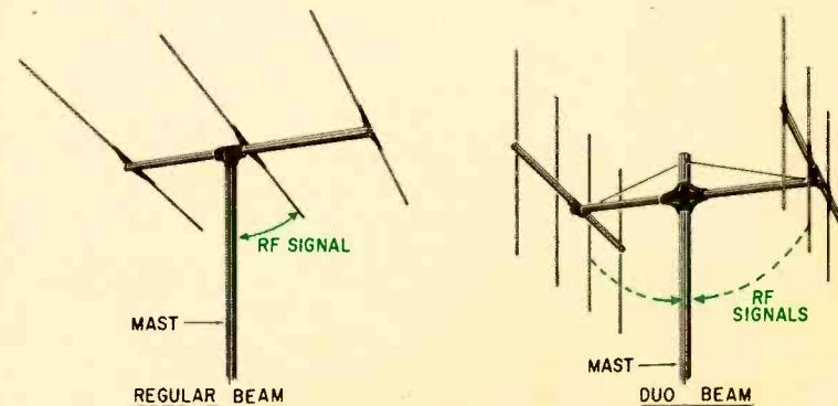
But look at the two-beam arrangement. Sure, soup from two separate antennas strikes the mast. But since the effect is equal on both beams, you can forget about it.
