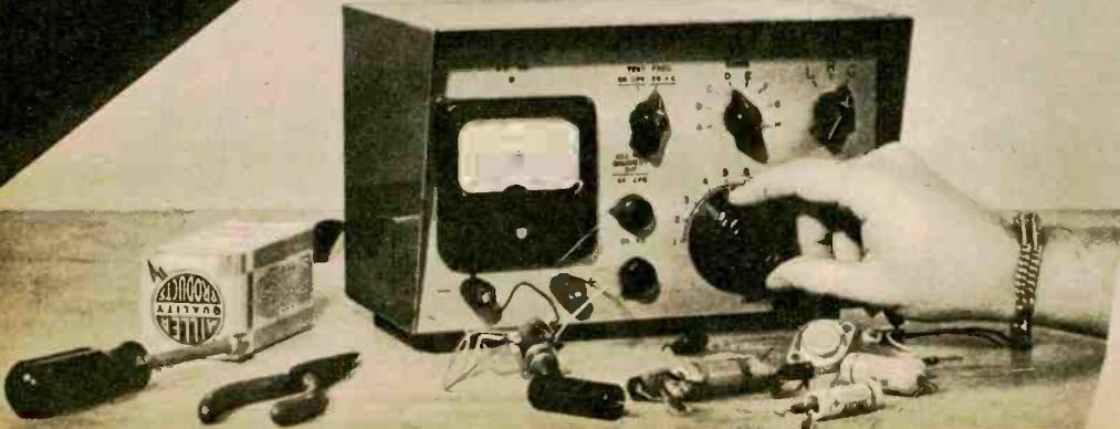
Fig. 1—View down into bridge. Wire selector switches S1, S2 and S3 before mounting them on front panel. Then mount circuit board on bottom of U-section of Minibox with four 1 1/4-in.-long spacers. Connect front-panel controls to circuit board, then install filament transformer T2 and associated components on rear panel. Pictorial of components on rear panel is shown in Fig. 3.
