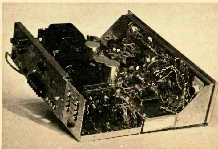
Reason the LK-60 looked so clean under the chassis is because of high parts density on top. However, all circuit boards are supplied prewired and tested. Bulk of the work is the interconnecting wiring between boards and switches. Low-level preamp boards are mounted vertically in lower-left corner and are enclosed by a shield cover. Black objects between power transformer and preamps are heat sinks for the output transistors.
