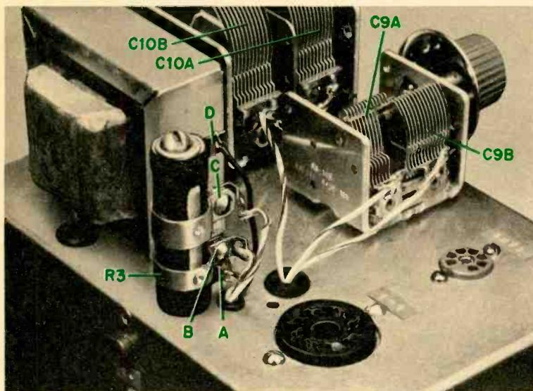
Fig. 3—Closeup of top of chassis shows mounting of B+ voltage-divider power resistor R3. Mount R3 with a  $\frac{1}{4}$ -20 x 2 $\frac{1}{2}$ -in. screw. Slider contact "C" is home brew since only one slider is supplied. Make a cover of perforated aluminum to fit over R3 so you don't touch it. If you did you'd get a nasty shock and burn. Both sections of C10 (top) are connected in parallel. C9A is the smaller section of C9.
