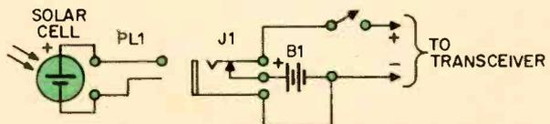
Modification of rig for solar cell operation. Connect cell's positive lead to plug's tip. Be sure to keep polarities straight when connecting battery and lead from switch to the jack.
