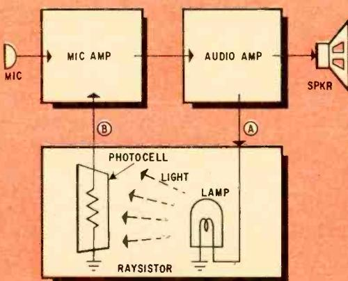
Fig. 2—USL Contact employs a novel speech compressor. Audio, tapped at point A, lights lamp, thus enabling photocell to vary gain at point B.
