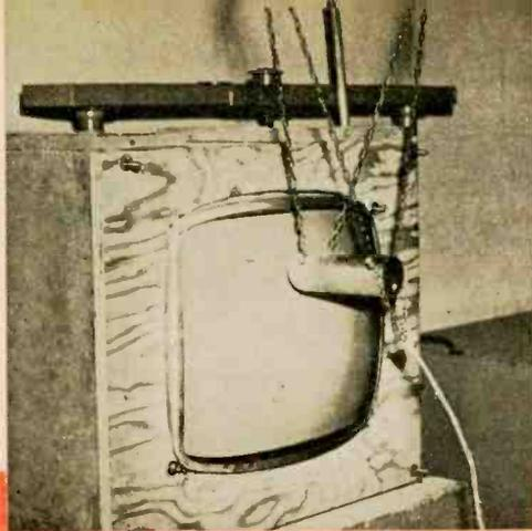
Among most dramatic tests conducted at UL's Melville, N.Y., facility is that for implosion of a TV picture tube. Technician (at left) was forced
