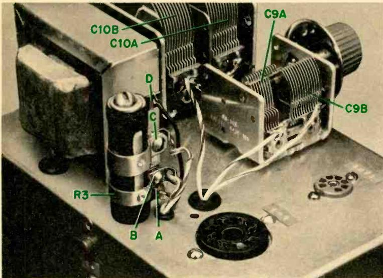
Fig. 3—Closeup of top of chassis shows mounting of B+ voltage-divider power resistor R3. Mount R3 with a ¼-20 x 2½-in. screw. Slider contact "C" is home brew since only one slider is supplied. Make a cover of perforated aluminum to fit over R3 so you don't touch it. If you did you'd get a nasty shock and burn. Both sections of C10 (top) are connected in parallel. C9A is the smaller section of C9.
