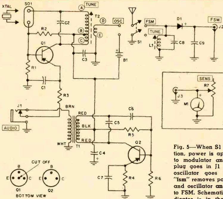
Fig. 5—When S1 is set to "osc" position, power is applied automatically to modulator and oscillator. When plug goes in J1 for audio tests, RF oscillator goes off. Setting S1 to "ism" removes power from modulator and oscillator and connects antenna to FSM. Schematic of FSM remote indicator is in the box at the right.
