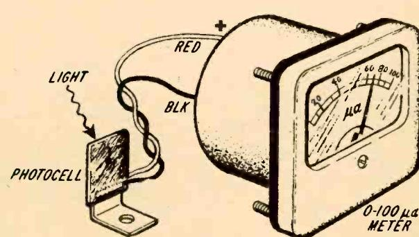
Fig. 3—In diagram of photovoltaic cell at left, holes and electrons are caused by light to cross potential barrier region and combine. Minority carriers which are created pass through the junction and are actually the current developed by the cell. Diagram at the right is of photovoltaic-cell light-level meter.
