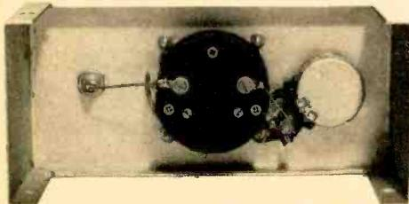
Fig. 6—FSM remote is built in a  $2\frac{1}{4} \times 2\frac{1}{4} \times 5$ -in. Minibox. Parts placement is not critical. Connect it to Tester with RG174/U coax cable.
