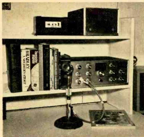
Shack-in-a-pigeonhole gave W2DJJ cause for concern until he tried a little something called a transceiver. Unit next to 24-hour clock on top shelf is power supply, which also houses speaker.
