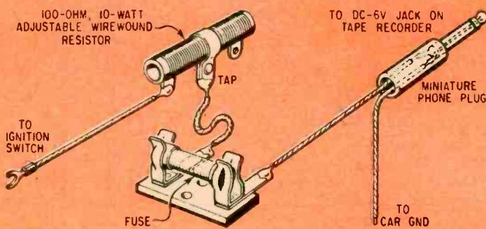
Mount resistor to drop voltage to 6 V on back of chassis. As recorder draws 100 ma. value should be 60 ohms. Use 100-ohm adjustable type and adjust slider with recorder operating to set voltage. Positive lead goes to the sleeve in plug.
