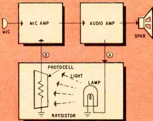
Fig. 2—USL Contact employs a novel speech compressor. Audio, tapped at point A, lights lamp, thus enabling photocell to vary gain at point B.
