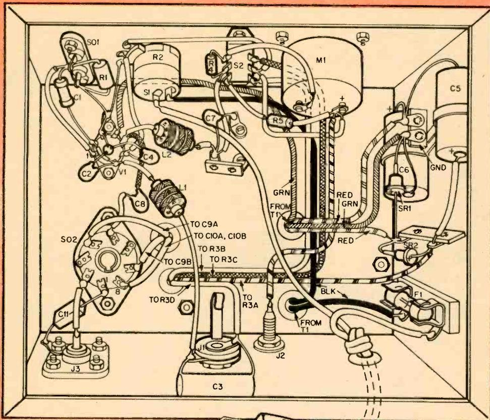
Fig. 1—Underside of transmitter. To layout your chassis, take dimensions from pictorial and multiply by about 2. Arrangement of parts in RF section of transmitter is important; therefore, duplicate our layout as closely as possible. The lugs at the left side of switch S2 are S2A.
