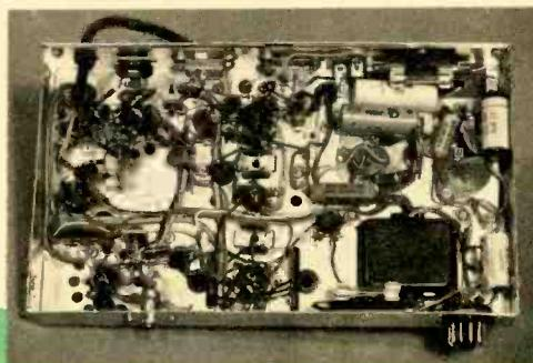
Though it looks crowded, there's room to spare in the underside of the C-540. 117-VAC or 12-VDC power cord fits on connector at lower right.
