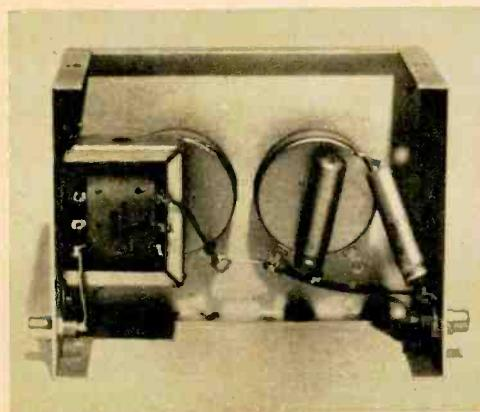
Parts are mounted in main section of 3 x 4 x 5-in. Minibox. R1 is mounted at left, R2 is mounted at right. Output jack is at left, input jack is at right.
