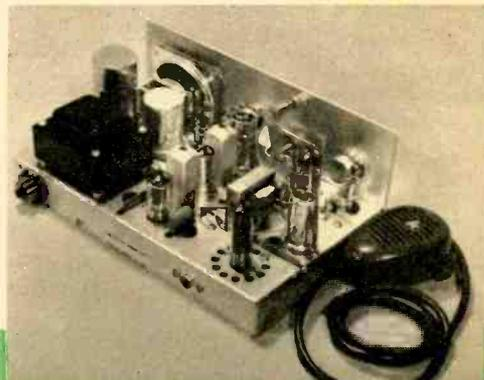
Vibrator on Universal model C-540 is between transformer and speaker. Circuit includes six tubes and has solid-state doubler power supply.
