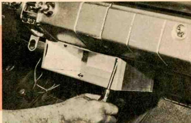
Adjustable wirewound resistor and fuse holder should be mounted on back of chassis. Because resistor will be difficult to get to after unit is mounted, measure the dropped voltage with recorder operating before installing chassis under the dash. Fuse should be a .15 A type 3AG.
