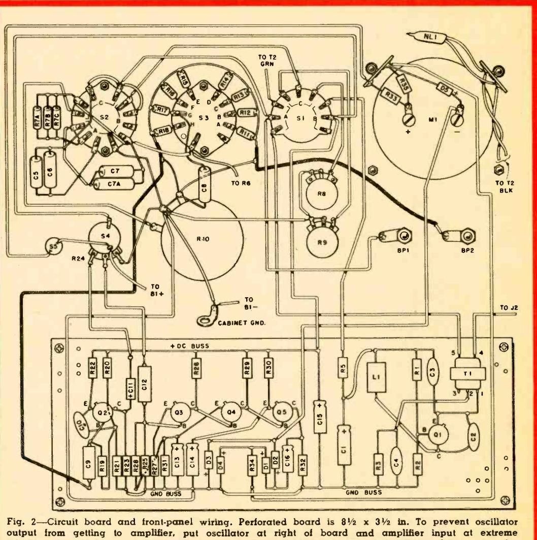
Fig. 2—Circuit board and front-panel wiring. Perforated board is 8 1/2 x 3 1/2 in. To prevent oscillator output from getting to amplifier, put oscillator at right of board and amplifier input at extreme left. Note that shield on wires from BP2 to R11 and from C9 to R18 is grounded at R11 and R18 ends only.
