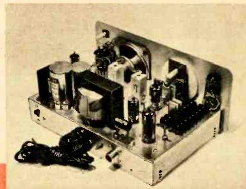
Rear of Comstat 9. Switch at left of rear chassis apron is used to select 5-watt or 100-mw input power. Crystal sockets are at right of chassis.
