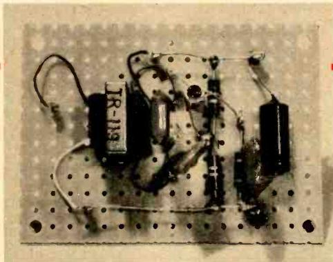
Fig. 3—Modulator is built on a  $2\frac{7}{16} \times 3\frac{3}{8}$ -in. piece of perforated board. Drill holes in corners and mating holes in cabinet bottom for mounting.
