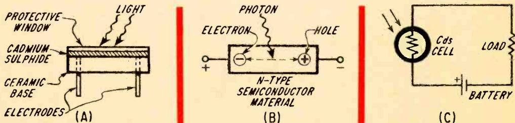
Fig. 1—Diagram A shows photoconductive cell construction. In B, activity of free electrons is increased by light which causes them to be attracted by positive external voltage. Holes left behind are attracted by negative side. This results in a current flow whose magnitude is determined by light intensity.
