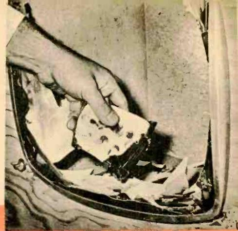
tube approximately  $\frac{1}{2}$ -millisecond before and after the impact; photo at far right depicts technician removing all that remains of the CRT.
