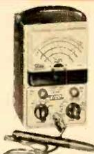
Model 232 Peak-to-Peak VTVM. A must for color or B&W TV and industrial use. 7-non-skip ranges on all 4 functions. With Uni-Probe. \$29.95 kit, \$49.95 wired.
