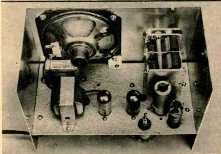
Top of chassis. Output transformer is near speaker. Mount power transformer (with core turned 90 degrees with respect to output transformer) behind it. Transformer T1 is at lower right corner of chassis.
