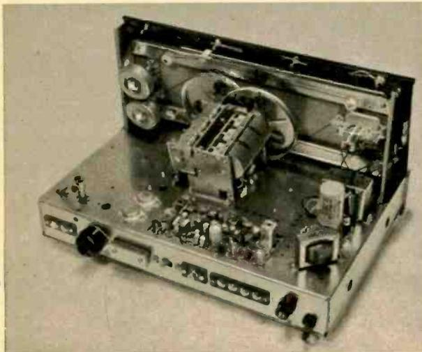
The Lafayette HA-600T receiver has a good deal of circuitry packed on one printed-circuit board. Output transistors are to the left of the board.
