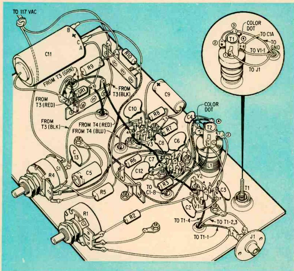
Underside of chassis. Wiring is tight around V1, V2 and V3. Note 12-turn winding (L1) wound over T2. Input transformer T1 is mounted on top of chassis and is shown in detail in inset drawing at the upper right.
