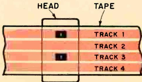
Fig. 5—To prevent crosstalk between tracks, head height must be correct. For example, if head is too low, tracks 1 and 2 will pass over upper gap.
