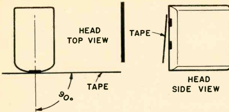
Fig. 6—Contact angle (left) is tangent at which tape contacts head. It should be 90° to head's centerline. Tilt (right) is deviation from parallel between surfaces of tape head and tape. Tape and head should be exactly parallel at contact (it's shown away from head here for illustration purposes).
