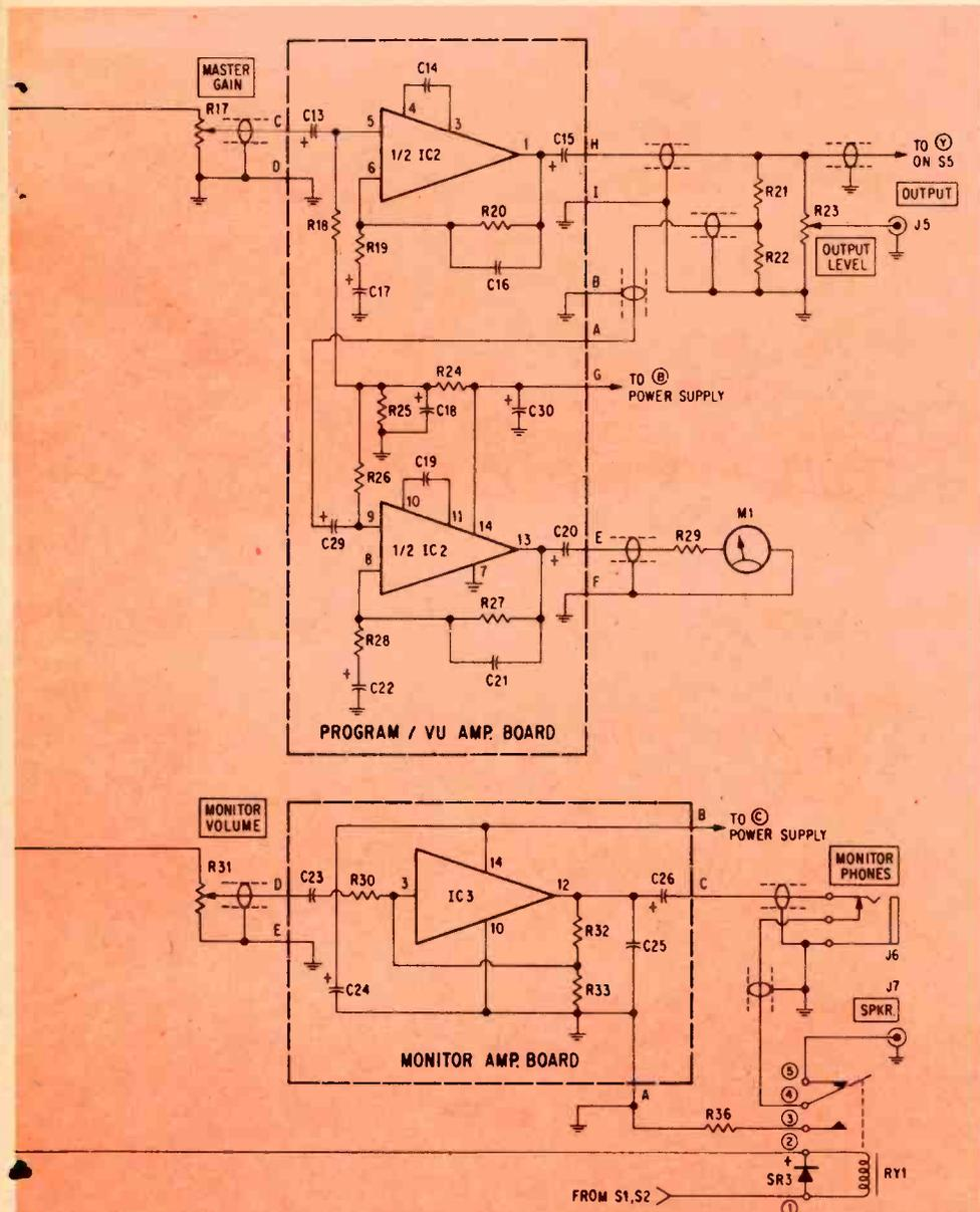
Fig. 5—Console schematic. When cueing a record or tape, switches S3 and S4 are closed and signal is fed via S5 to monitor amp, whose output drives speaker so you cue record or tape. When you turn up either mike gain control, S1 or S2 closes and energizes RY1 to cut out speaker and prevent feedback. Set S5 to the output position and you monitor signal going to wireless broadcaster at J5.
