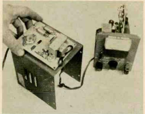
Minikits can often improve existing equipment. Here, Eicocraft power supply is added to power supply for another fixed voltage.
