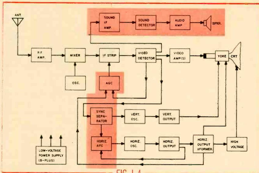
sweep circuit is operating. Even if the high voltage is present, there cannot be a raster unless both horizontal and vertical sweeps are working. Should only the horizontal sweep and high voltage function, the beam is just swept from side to side to form a single horizontal line (i.e. the vertical sweep is not sweeping the beam from top to bottom).
