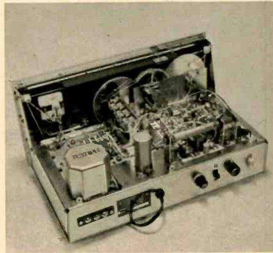
Radio Shack DX-150 has three-gang tuning capacitor and smaller bandspread capacitor to right of it. Power transformer is in lower left corner.
