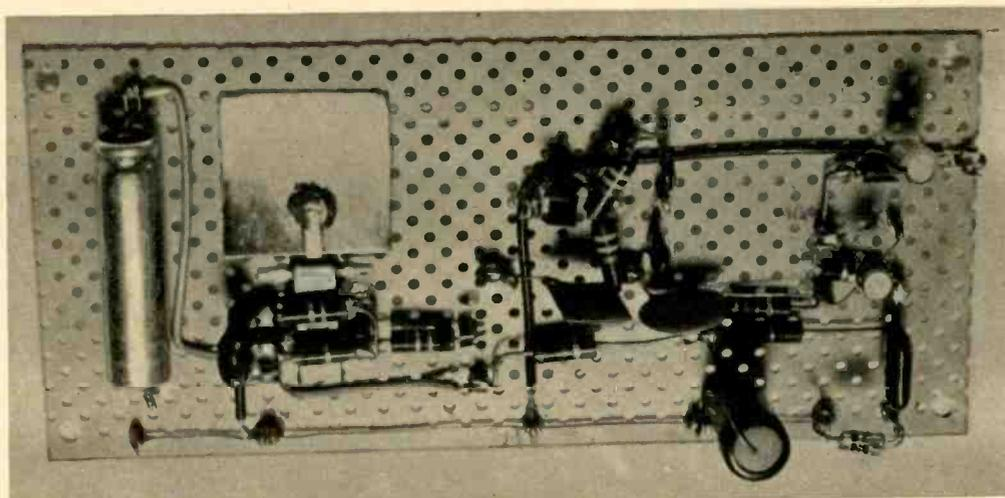
Metal tab is IC's tin heat sink. Note long leads on diodes (lower right) to prevent soldering-heat damage.
