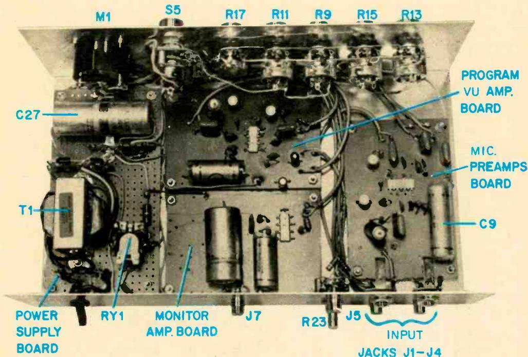
Fig. 4—Photo of inside of console shows part locations. Mount cabinet parts before installing boards.
