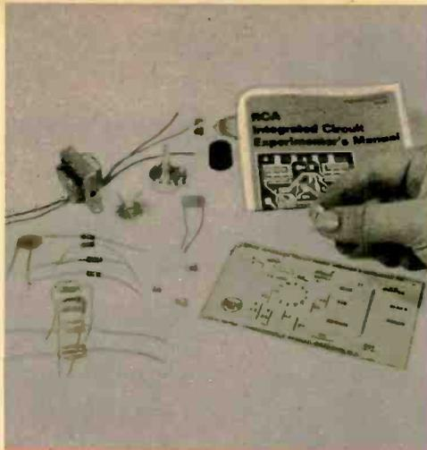
In RCA's IC kit, practically all parts are supplied. Manual discusses both theory and construction in detail. PC board is used.
