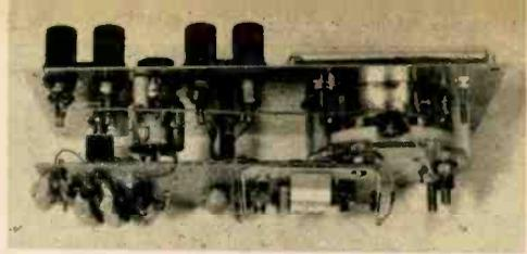
Fig. 1—Note how perforated circuit board is mounted on back of the meter and spaced 1 $\frac{1}{4}$  in. from the panel. Directly behind binding posts is the ground bus which connects to the negative terminal on the meter. Holder is for battery.
