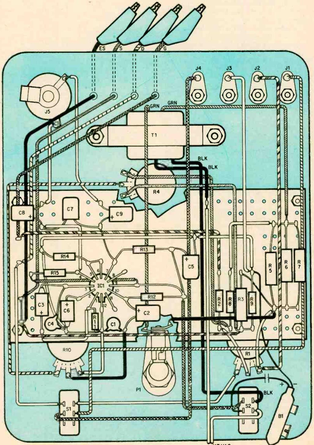
R1, R4 and R10 full counterclockwise. Disconnect the lead from R4 going to the junction of R3 and R9. Set the VOM to measure resistance and connect its test leads to R4's wiper lug and disconnected lead.
