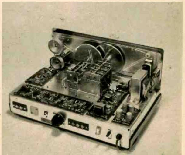
The Allied Model A-2515 receiver has four printed-circuit boards on chassis. Note the three-gang main-tuning and bandspread variable capacitors.
