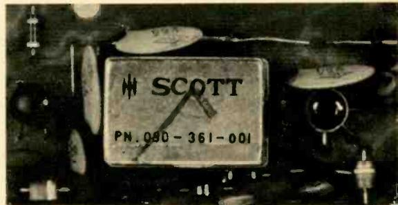
Scott model 342C 100-watt stereo FM receiver is latest component to feature quartz-crystal lattice filter. Factory alignment is said to be permanent. The check mark was put there by factory.
