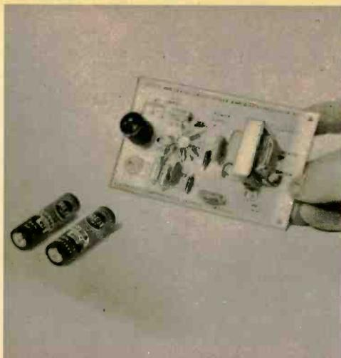
Detailed view of PC board for RCA's IC kit. Circuit operates as audio amplifier or oscillator. You add speaker and batteries.
