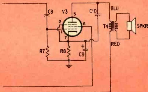
Incoming signals are tuned by T1/C1A and fed to RF amplifier V1. Amplified signal is tuned by T2/C1B and fed to regenerative detector V2. Detected signal (audio) is fed to output stage V3. RF gain control R1 determines volume.
