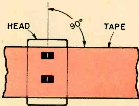
Fig. 4—The azimuth adjustment of the head is correct when the angle between the gap in the head and the edge of the tape is exactly  $90^\circ$ .
