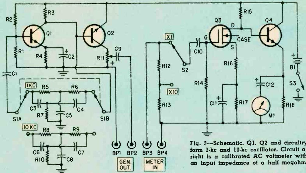
Fig. 3—Schematic. Q1, Q2 and circuitry form 1-kc and 10-kc oscillator. Circuit at right is a calibrated AC voltmeter with an input impedance of a half megohm.
