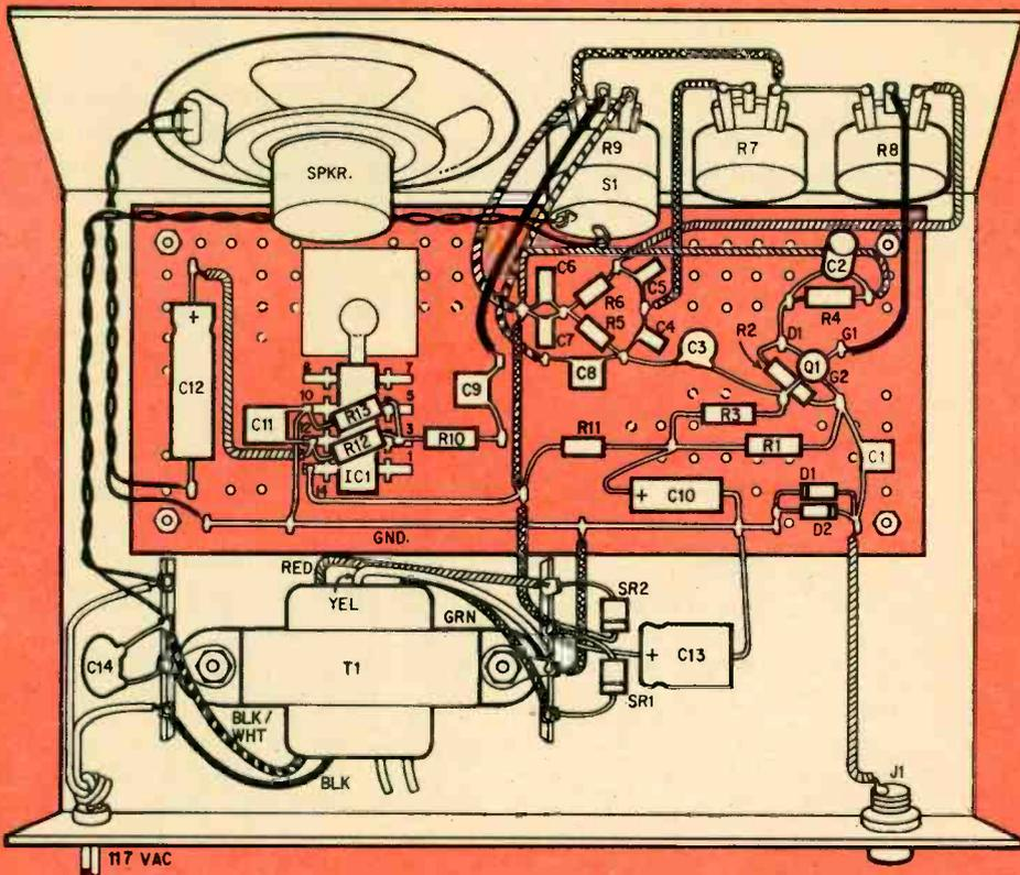
Except for power supply, Q-multiplier is built on a piece of perforated board. Tab on IC1 is heat sink.
