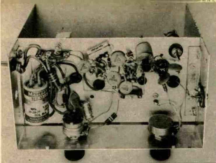
Underside of chassis. Note how the chassis is held in the cabinet with angle strips. If this material is not available, use four angle brackets. Antenna jack (J1) is at right.
