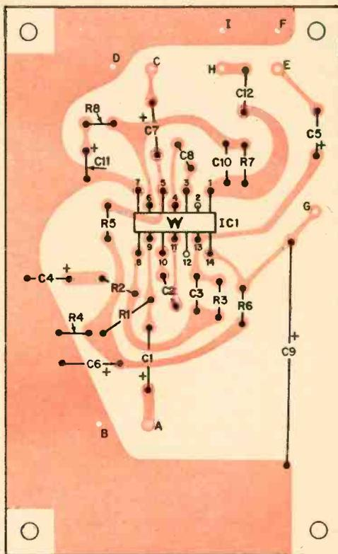
Fig. 1—Below is template for mic.-preamps and program/VU-amp. boards. Trace outline of black areas with carbon paper on foil side of two boards. Part numbers and location for mic.-preamps board is above. Fig. 8 has program/VU-amp. board nos.
