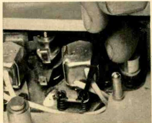
Fig. 8—On same machine azimuth-adjustment screw is at rear of head on the mounting plate. Use demagnetized tools when working around head.
