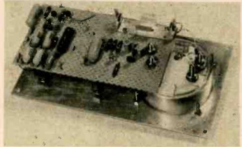
Fig. 2—View of rear of board (above). Author's wiring is on back of board; however, we show it in the pictorial (below) as if it were on top with connections made to flea clips. Use spaghetti insulation on leads that cross and may short.
