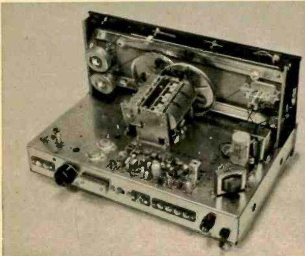
The Lafayette HA-600T receiver has a good deal of circuitry packed on one printed-circuit board. Output transistors are to the left of the board.
