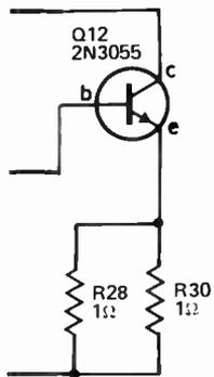
Fig. 3. Circuit diagram of the power supply suitable for one 100 W or two 50 W amplifiers.
