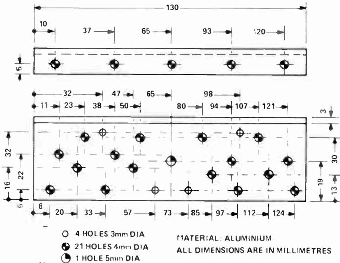
Fig. 8. Heatsink bracket for the 100 W module.
