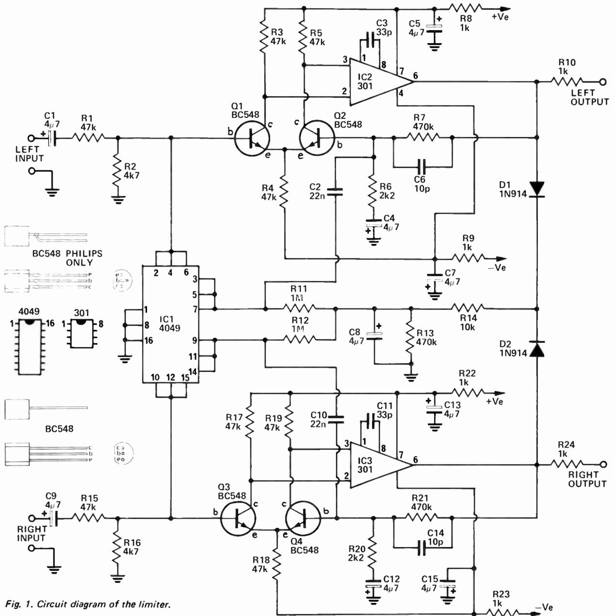
Fig. 1. Circuit diagram of the limiter.
