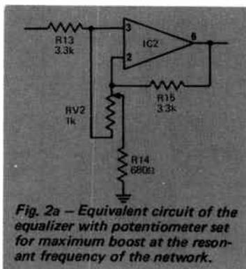
RV2. The voltage on pin 3 (IC2) is therefore equal to the output of the mixer since there is virtually no current through and no voltage drop across R13.
