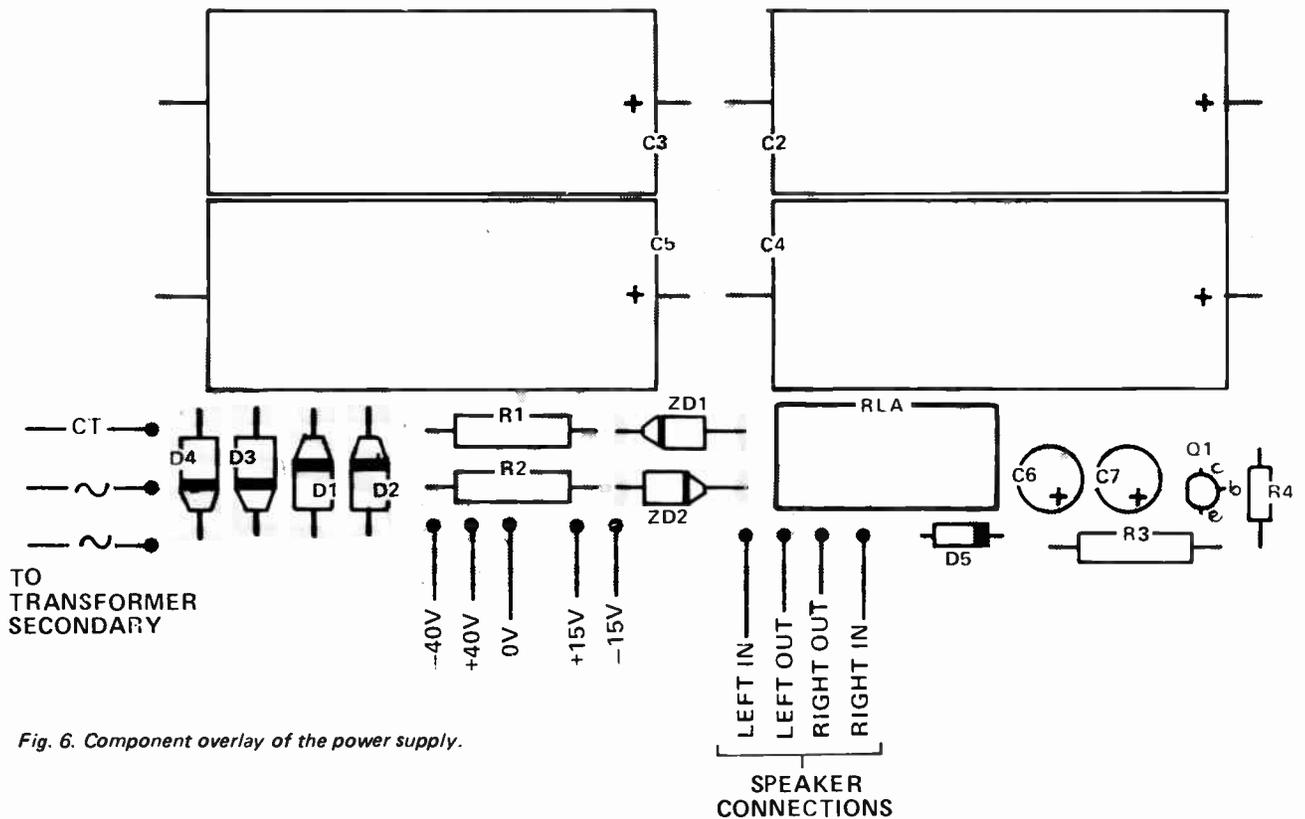
Fig. 6. Component overlay of the power supply.
