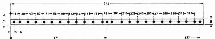
Fig. 9. Drilling details for the potentiometer support
