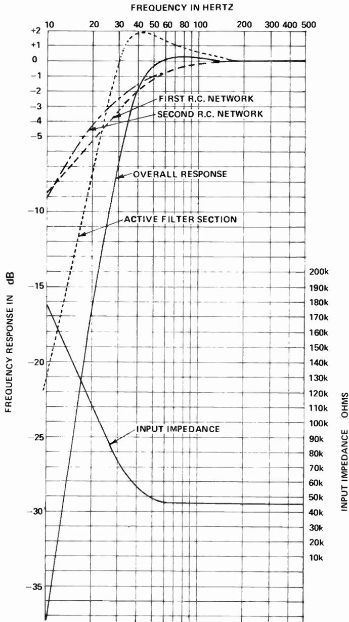
Fig. 4. Characteristics of the rumble filter.
