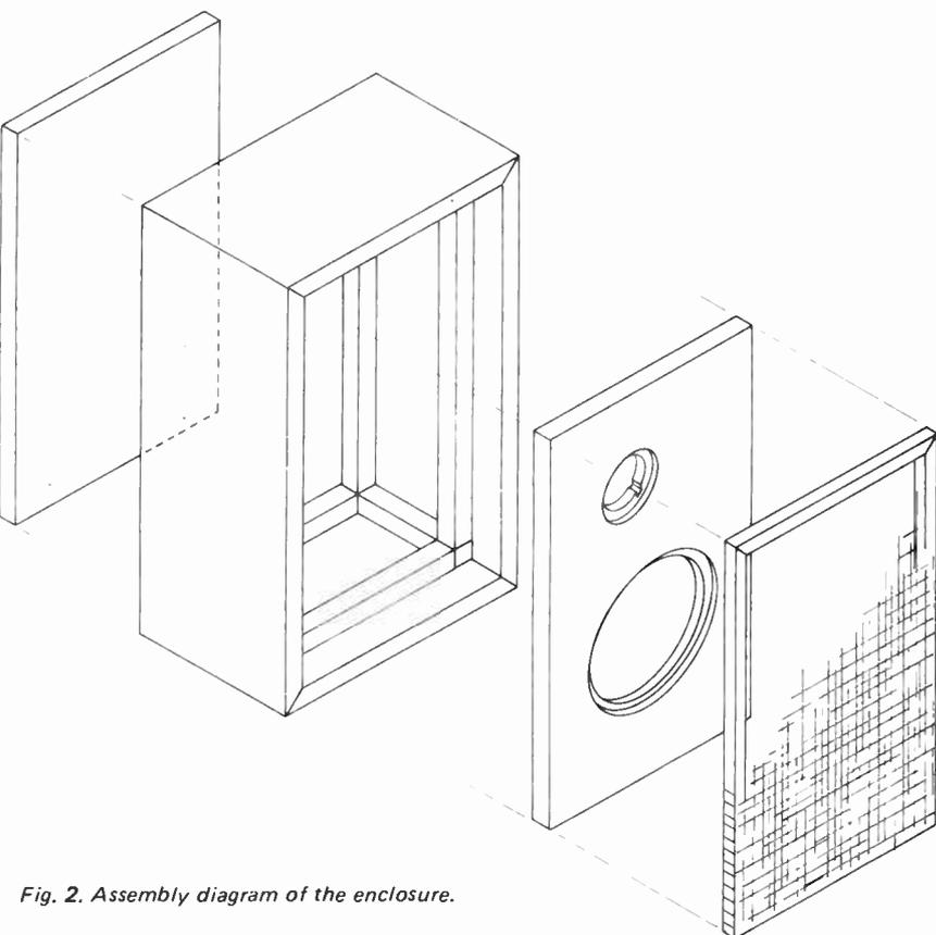
Fig. 2. Assembly diagram of the enclosure.
