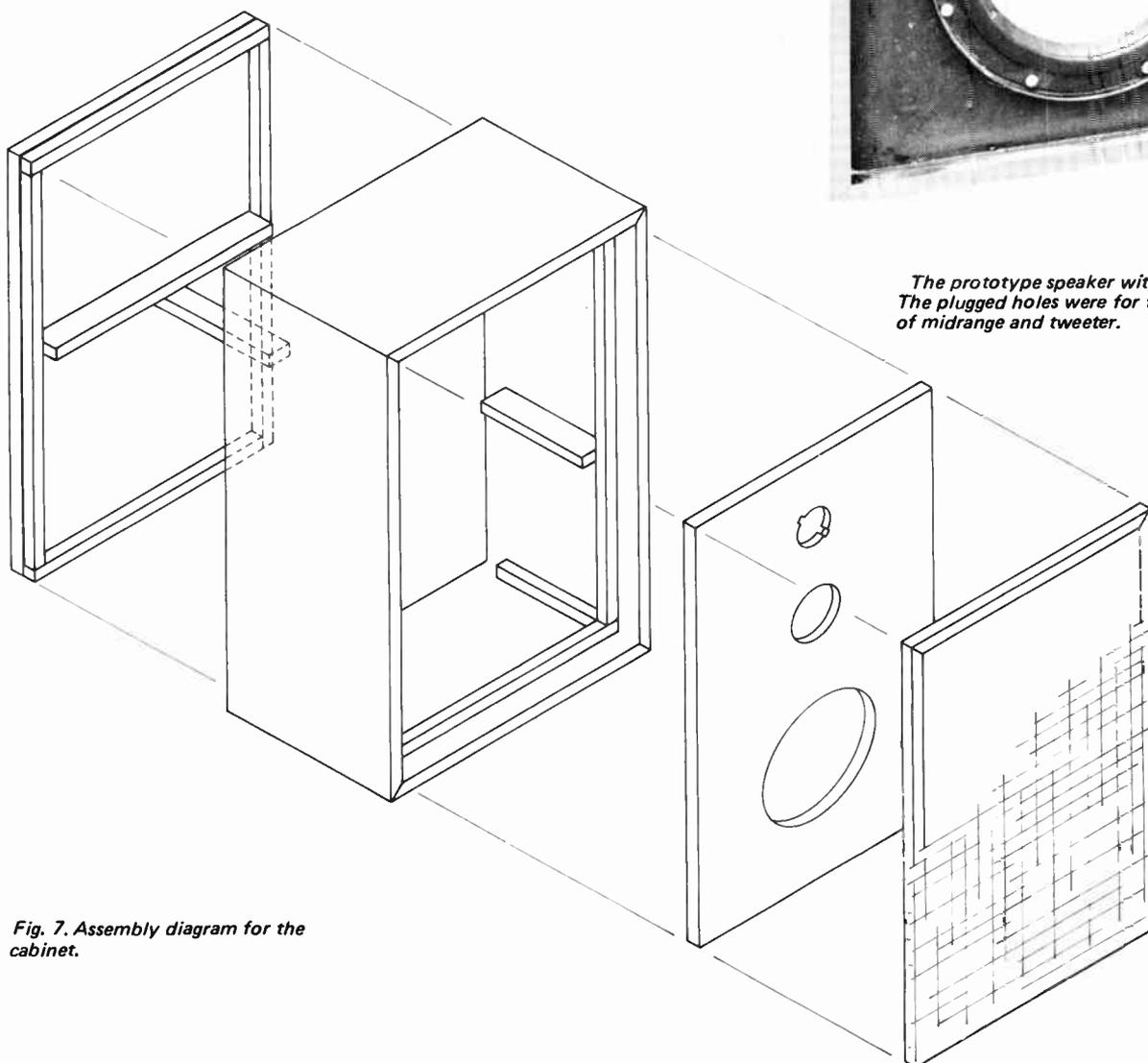
Fig. 7. Assembly diagram for the cabinet.
