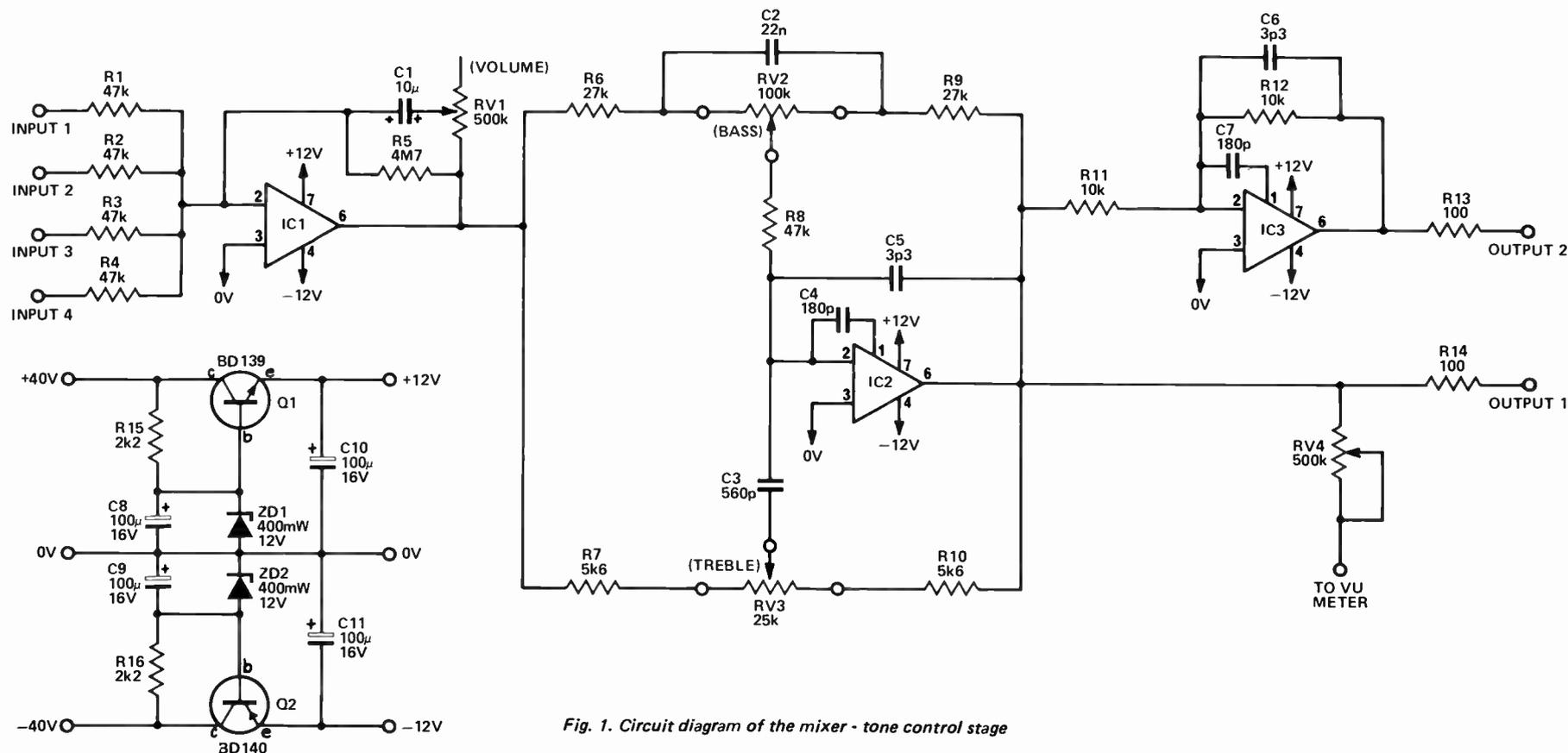
Fig. 1. Circuit diagram of the mixer - tone control stage
