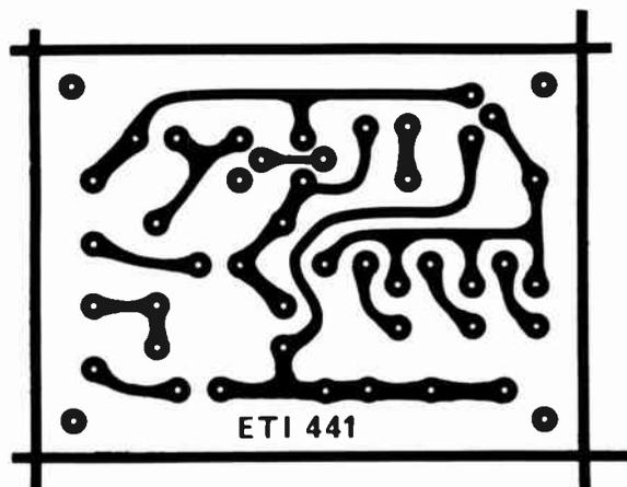
Printed circuit layout. Full size 67 x 49 mm.
