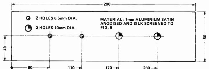
Fig. 9. Dimensions of the front panel.
