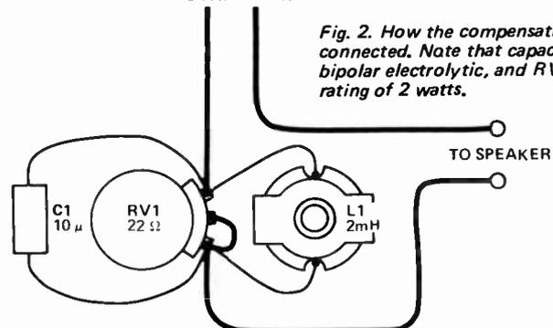
Fig. 2. How the compensation network is connected. Note that capacitor C1 is a bipolar electrolytic, and RV1 has a minimum rating of 2 watts.
