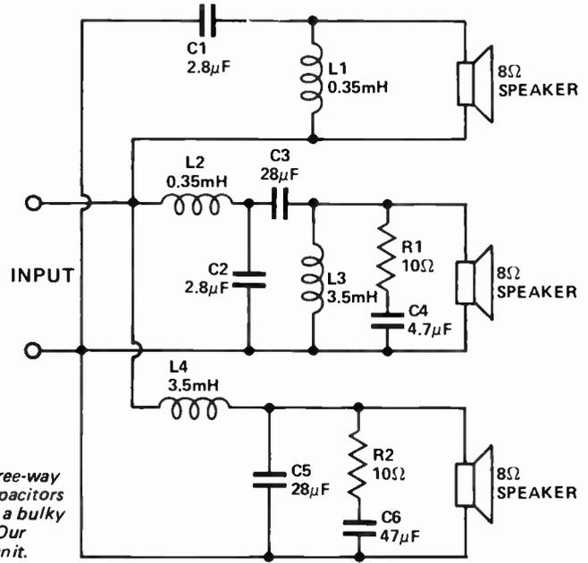
Fig. 1. A conventional three-way crossover system using capacitors and air-cored inductors is a bulky and very expensive unit. Our drawing shows a typical unit.
