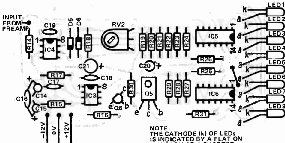
Fig. 6. The component overlay of board A.
