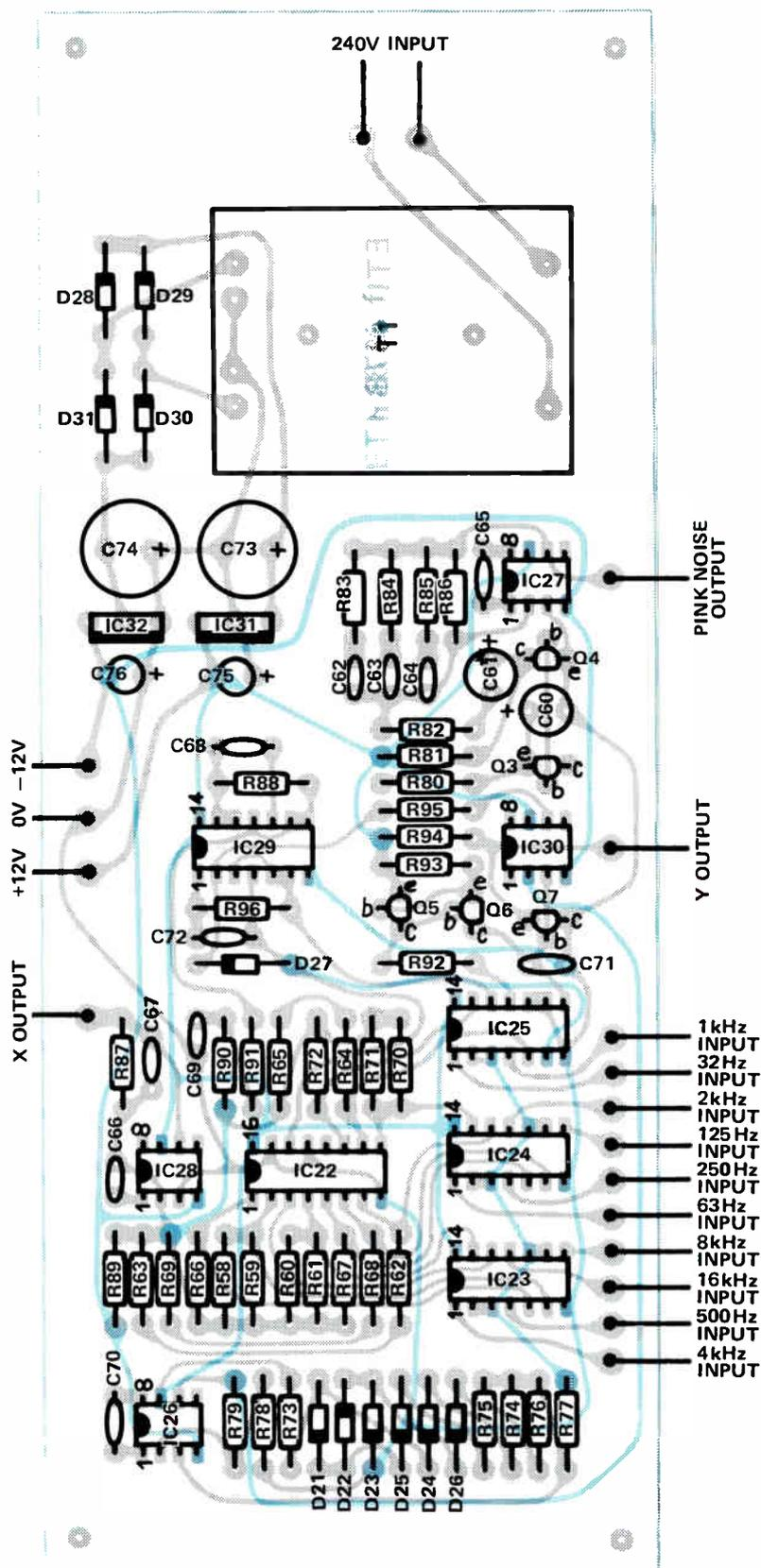
Erratum: Capacitor C75 is shown positioned incorrectly. It should be turned through 180°. A link must also be made between the collector of Q2 and the end of R10 where the -12V track begins on the underside on the board.
