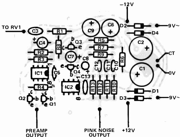
Fig. 5. The component overlay of board B.
