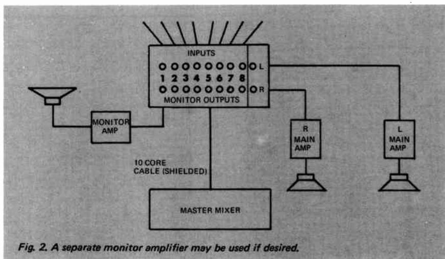
Fig. 2. A separate monitor amplifier may be used if desired.
