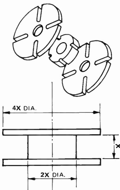
Fig. 6. Dimensions of bobbins used to wind coils L1 to L4. For L1 and L2 'x' = 13 mm, for L3 and L4 'x' = 10 mm.
