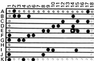
This is the drilling details for the Veroboard version. Do make sure that the breaks required (shown as black dots) are clean, and that no 'whiskers' remain.
