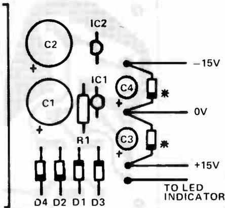
Fig. 4. Changes in the overlay for the low power version.
