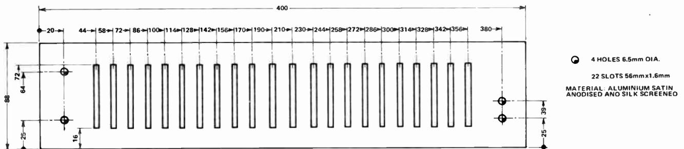
Fig. 8. Metalwork details of the front panel.
