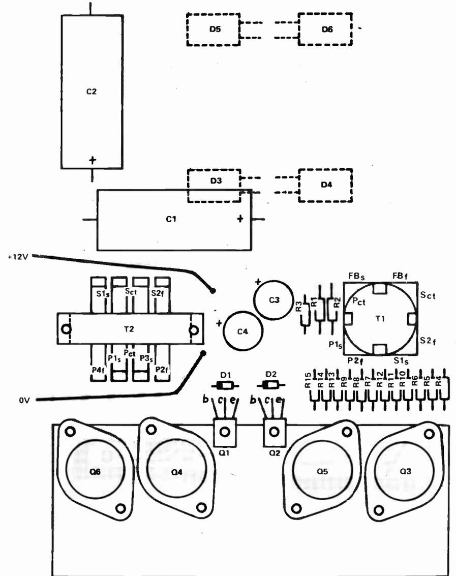
Fig. 4. Component overlay.
