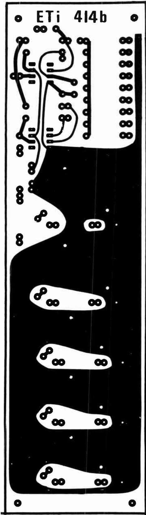
The main mixer and equalizer printed circuit board pattern – shown full size.
