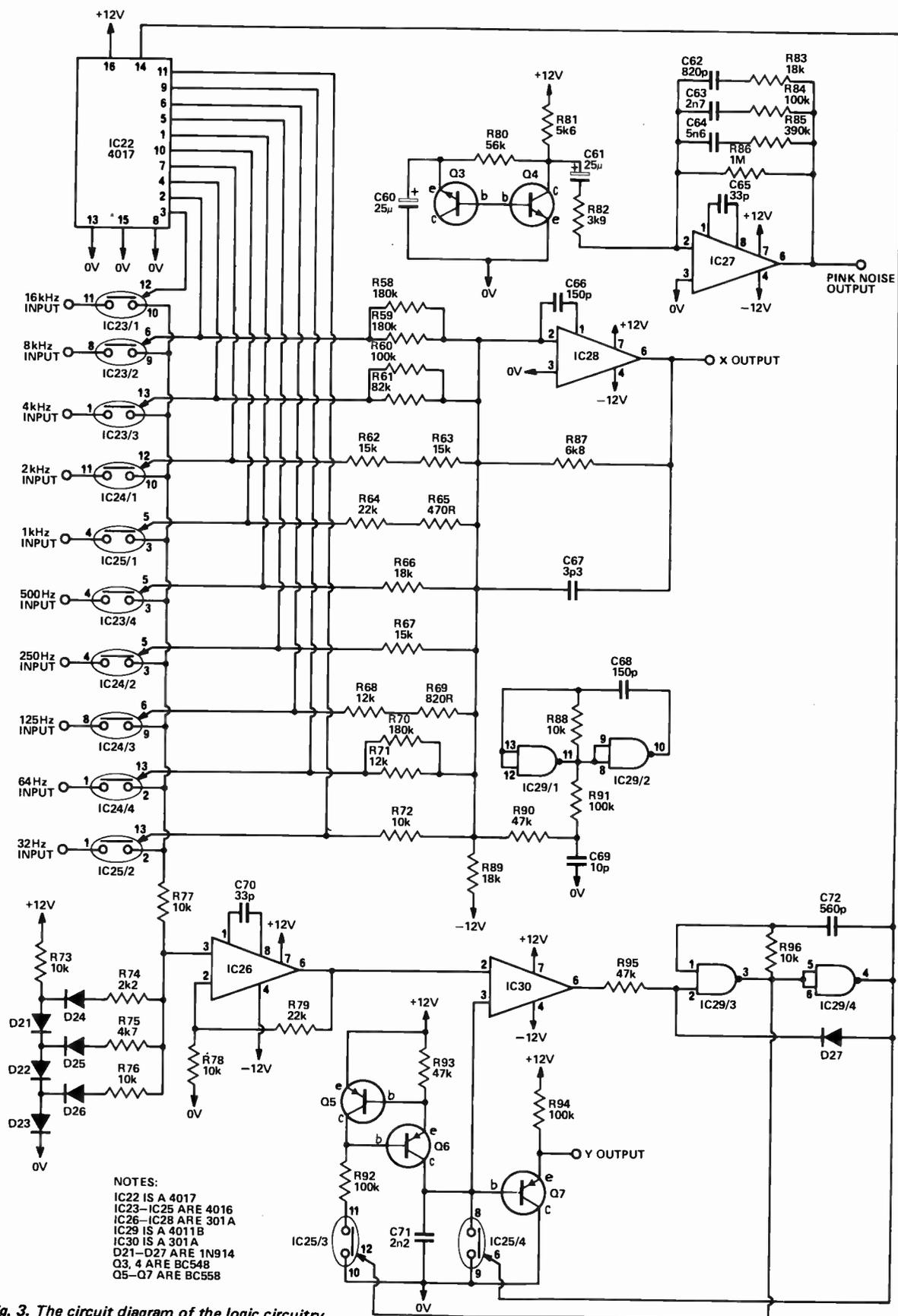
Fig. 3. The circuit diagram of the logic circuitry.
