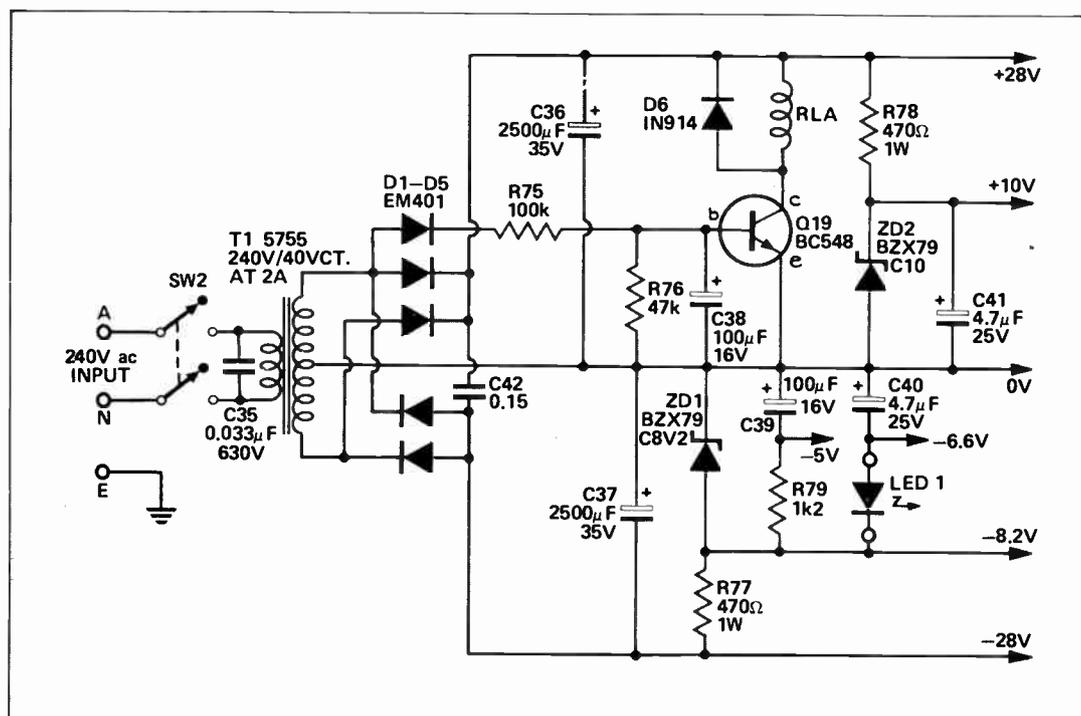
Fig. 2. Power supply for the 25 watt amplifier.
