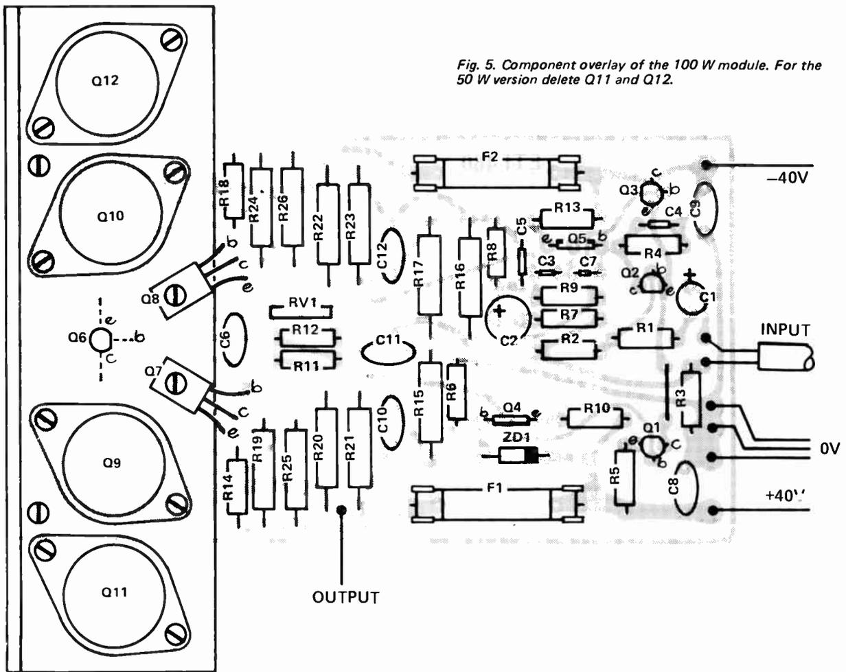
Fig. 5. Component overlay of the 100 W module. For the 50 W version delete Q11 and Q12.
