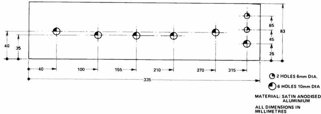
Fig. 8. Front panel details.
