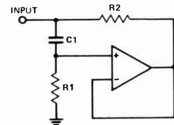
of the network. At either side of resonance the impedance will rise (with a slope dependant on the Q of the network which is 3) due to the uncanceled reactance. This will be inductive above resonance and capacitive below resonance. We can therefore represent the equalizer stage by the equivalent circuit below.
