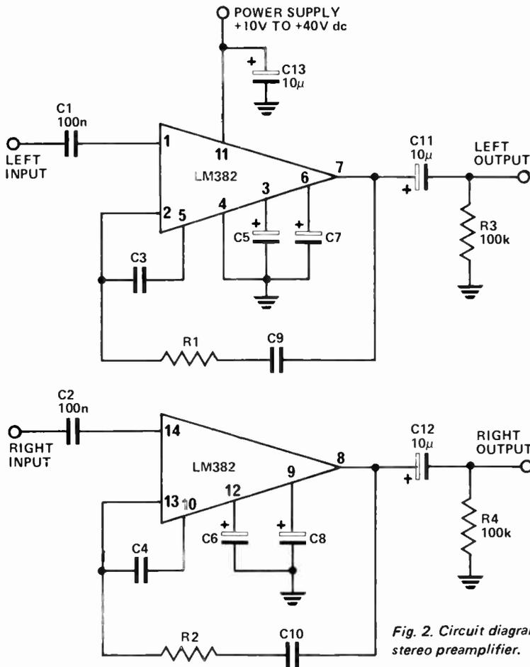
Fig. 2. Circuit diagram of the stereo preamplifier.
