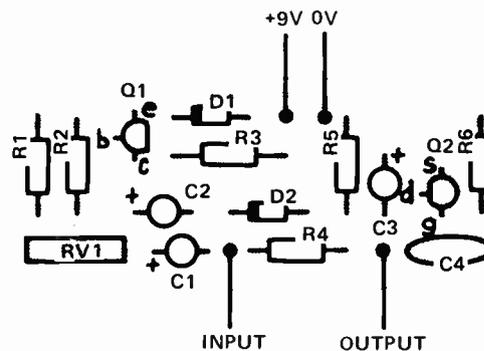
Component layout of printed circuit board version.
