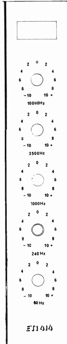
Fig. 5. Equalizer panel escutcheon (actual size 12" x 2 1/4").
