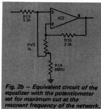
gain of about 15dB. If the slider is at the other end of the potentiometer (Fig 2b) the signal appearing at pin 3 and thus also at pin 2 is about 0.2 of the output of the previous stage due to the voltage division of R13 and the 680Ω. There is still zero current through RV2 and also zero current through R15 since there is no path. The output voltage is therefore the same as that at pin 2, which happens to be about 0.2 times the output of the previous stage. The gain is therefore 0.2 or -13dB.
