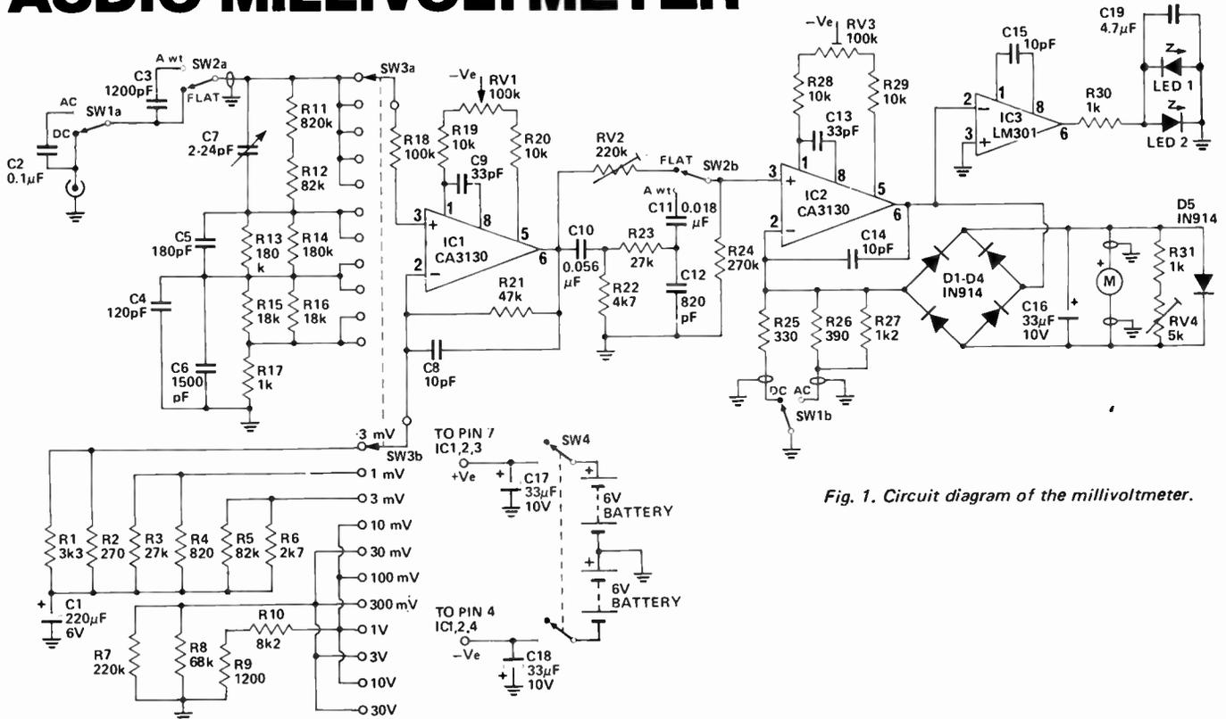
Fig. 1. Circuit diagram of the millivoltmeter.
