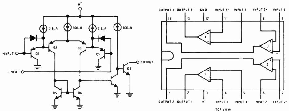
Fig. 3. Internal circuitry and pin corrections of the LM339 IC.
