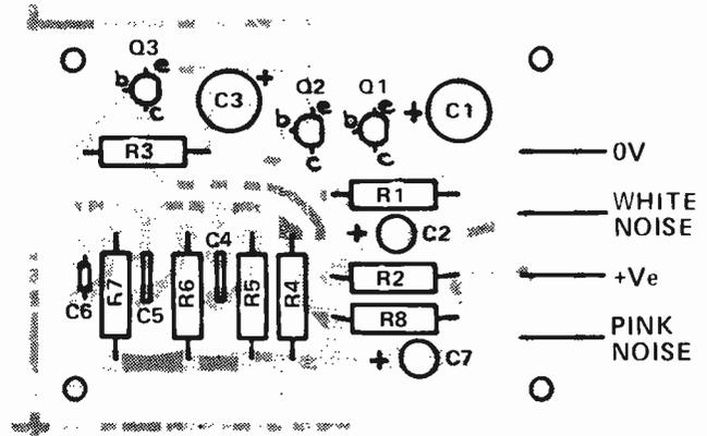
Fig. 2. Component overlay.
