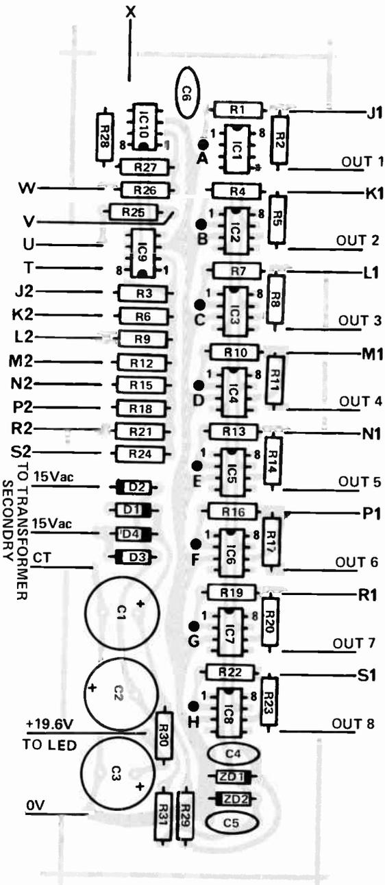
Fig. 7. Component overlay for the mixer/power-supply board.
