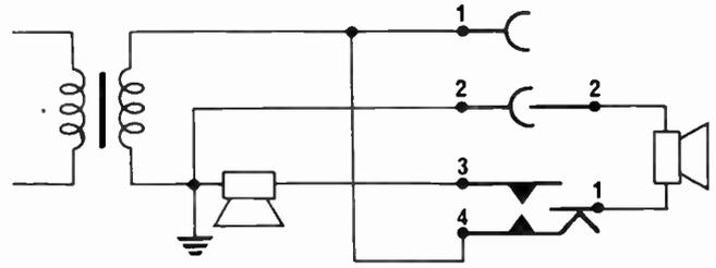
Fig. 1b. With the connector reversed, in position B, the internal speaker is disconnected.
