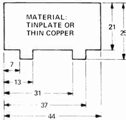
Fig. 4. Heatsink (two required) to be attached to either side of both IC's as shown in main picture.
