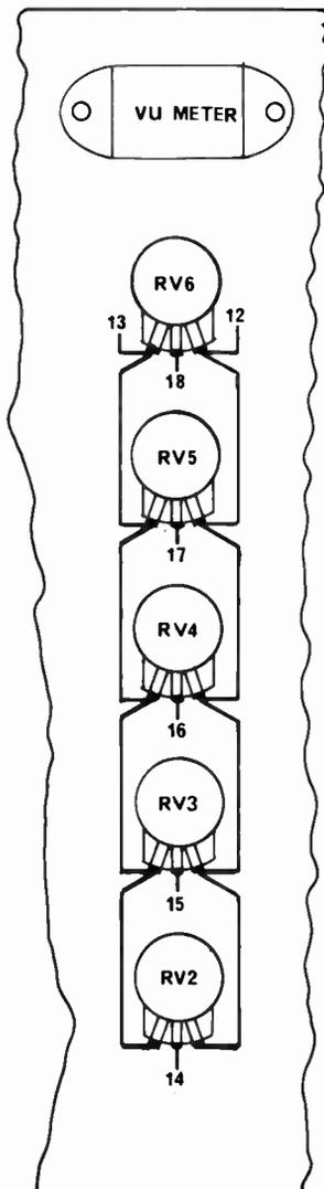
This diagram shows the connections to the potentiometers associated with the equalizers. The numbers correspond one-to-one, to those on the main mixer - equalizer circuit and overlay diagrams.
