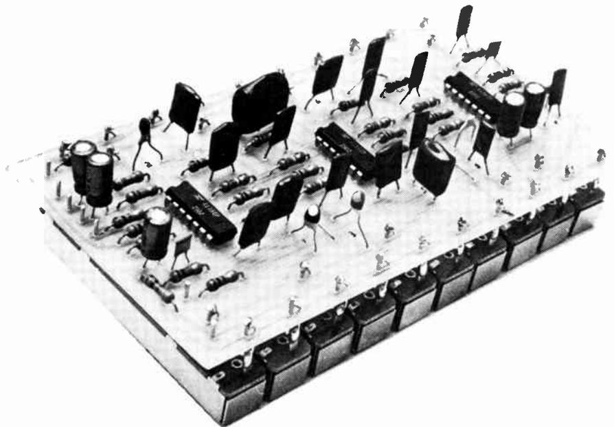
*Photo showing one complete channel, less the volume control, removed from the chassis.*
