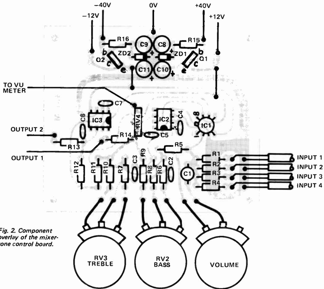
Fig. 2. Component overlay of the mixer-tone control board.
