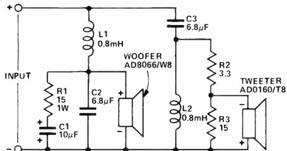
Fig. 3. Circuit diagram of the crossover network. This is the heart of the system and must not be changed if best results are to be obtained.
