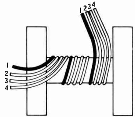
Fig. 6. Diagram showing the start of the quad-filar primary winding of T2. Note that it must be wound this way to reduce power consumption and improve regulation.
