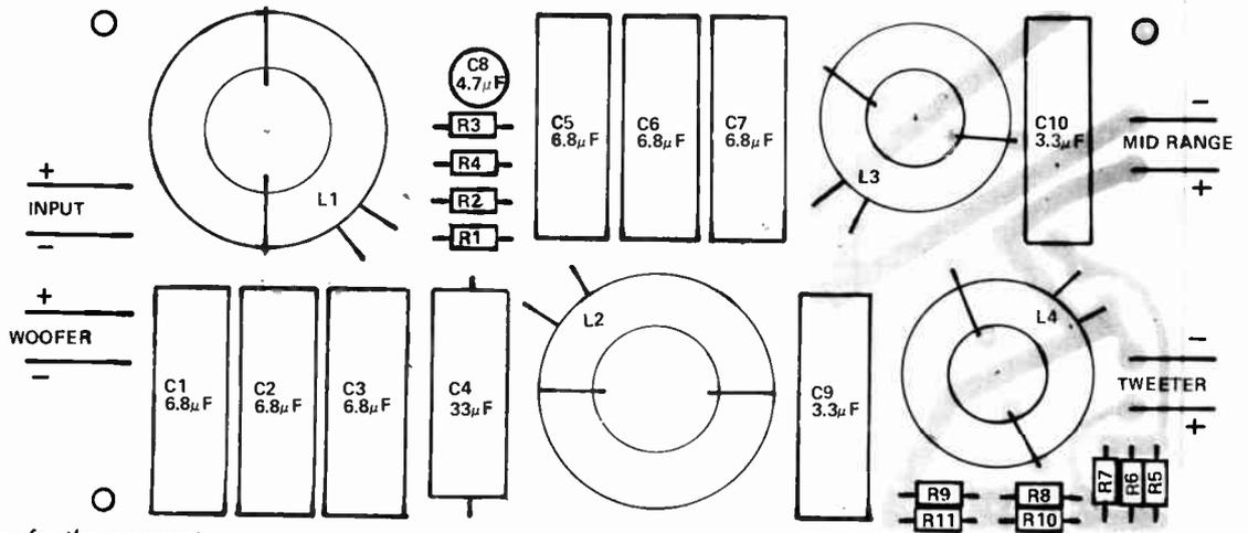
Fig. 4. Component overlay for the crossover.
