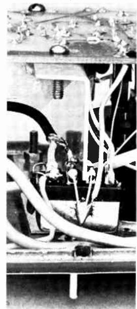
Note how the shield passes between the earthed, centre contacts of the 'A' weight switch.
