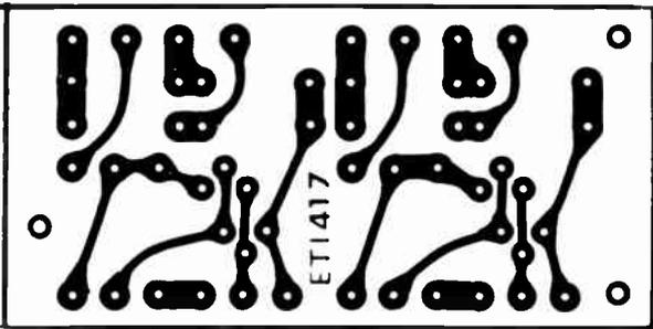
Printed circuit board layout — shown full size.
