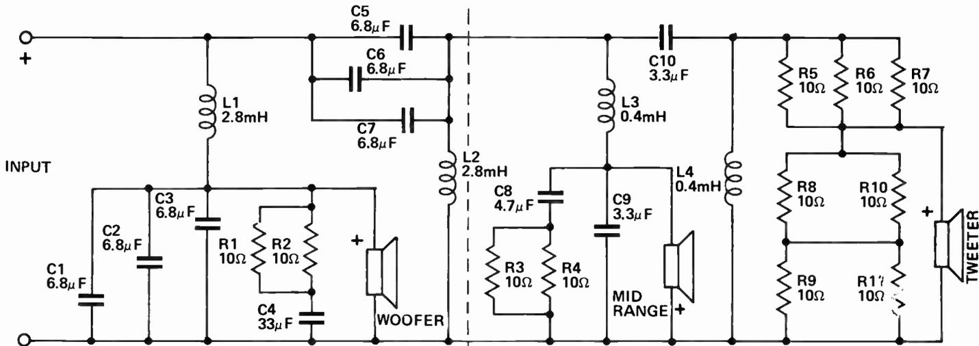
Fig. 3. Circuit diagram of the three way crossover. If crossover amplifier is used only the components to the right of the dotted line are required.
