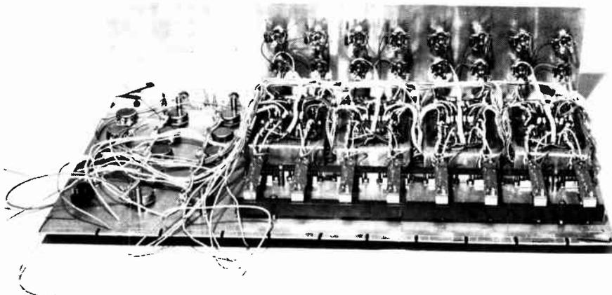
*This photograph was taken during construction of our prototype unit. The four input pre-amps may be seen on the right. Directly in front of the pre-amps are the slide potentiometers used for individual volume controls.*
