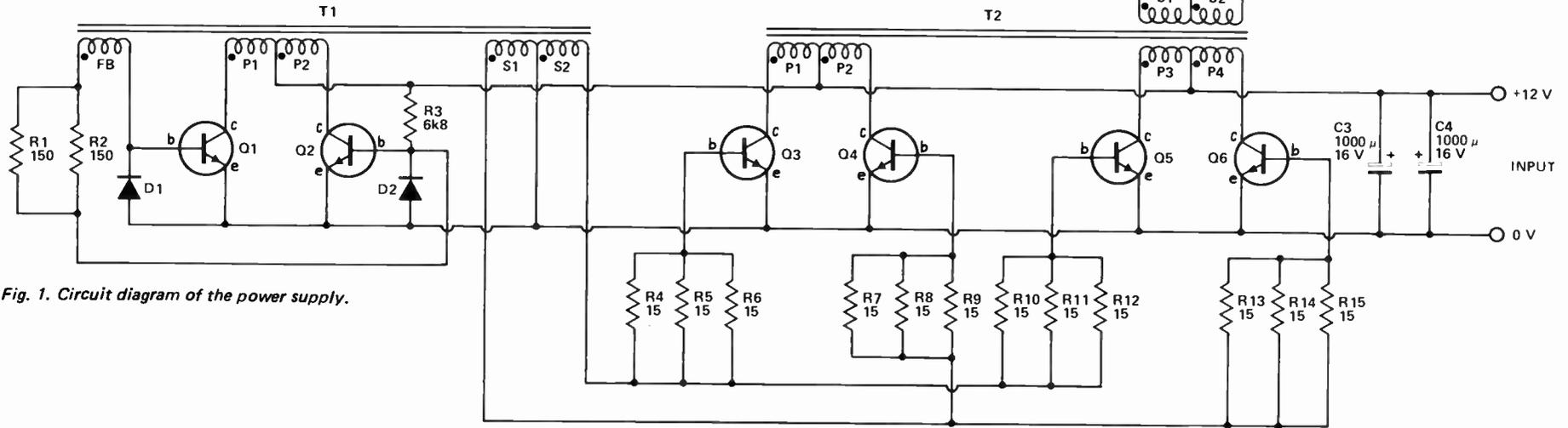
Fig. 1. Circuit diagram of the power supply.
