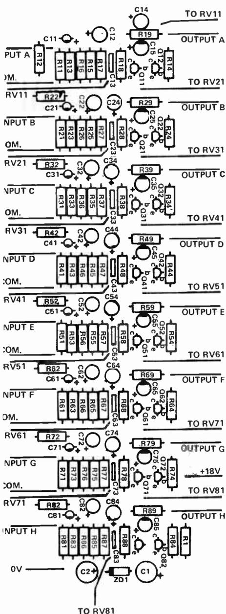
Fig.2. Component overlay for the preamplifier board.
