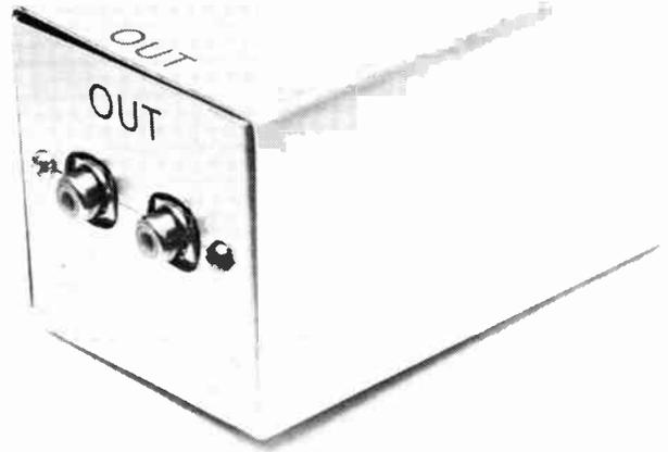
the filter must be situated before the preamplifier. This also poses problems as the signals at this point are very low-level, and there is a danger of introducing hum which would be merely replacing one fault by another.
