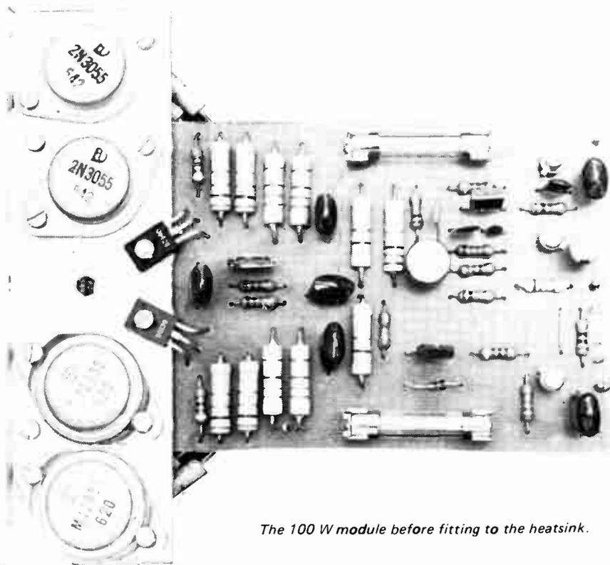
*The 100 W module before fitting to the heatsink.*
