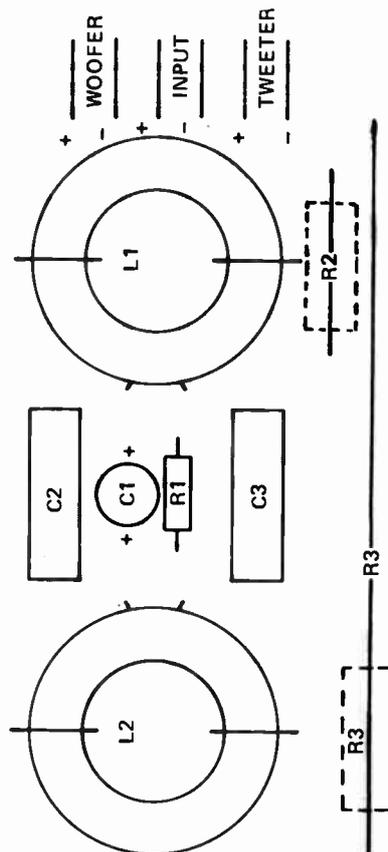
Fig. 6. Component overlay shows how to assemble the crossover network.
