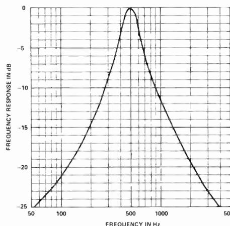
Fig. 1. The frequency response of the 500Hz filter. All other filters follow a similar curve.
