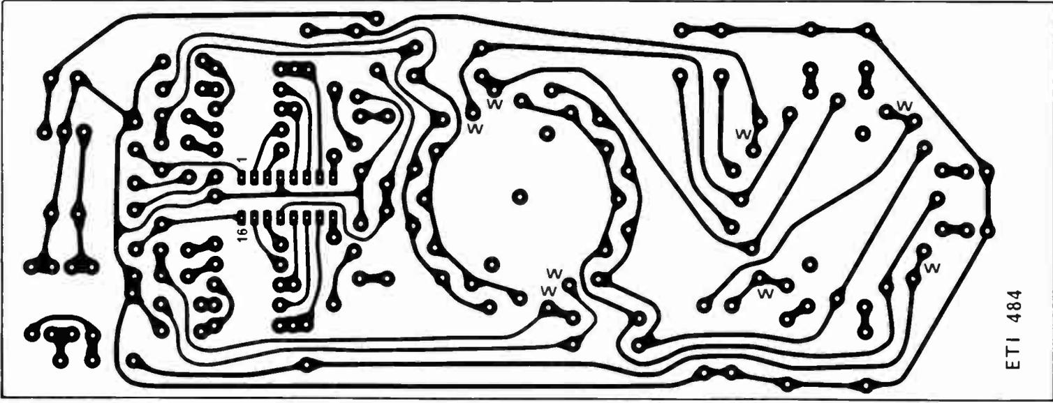
Fig. 5. Printed circuit layout. Full size 200 x 75 mm.
