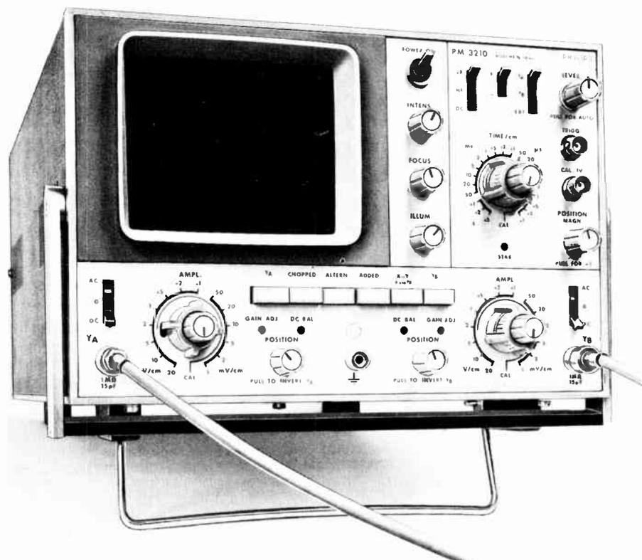
Fig. 13. Front panel of an oscilloscope that represents medium sophistication. The text contains a self test about its controls.
