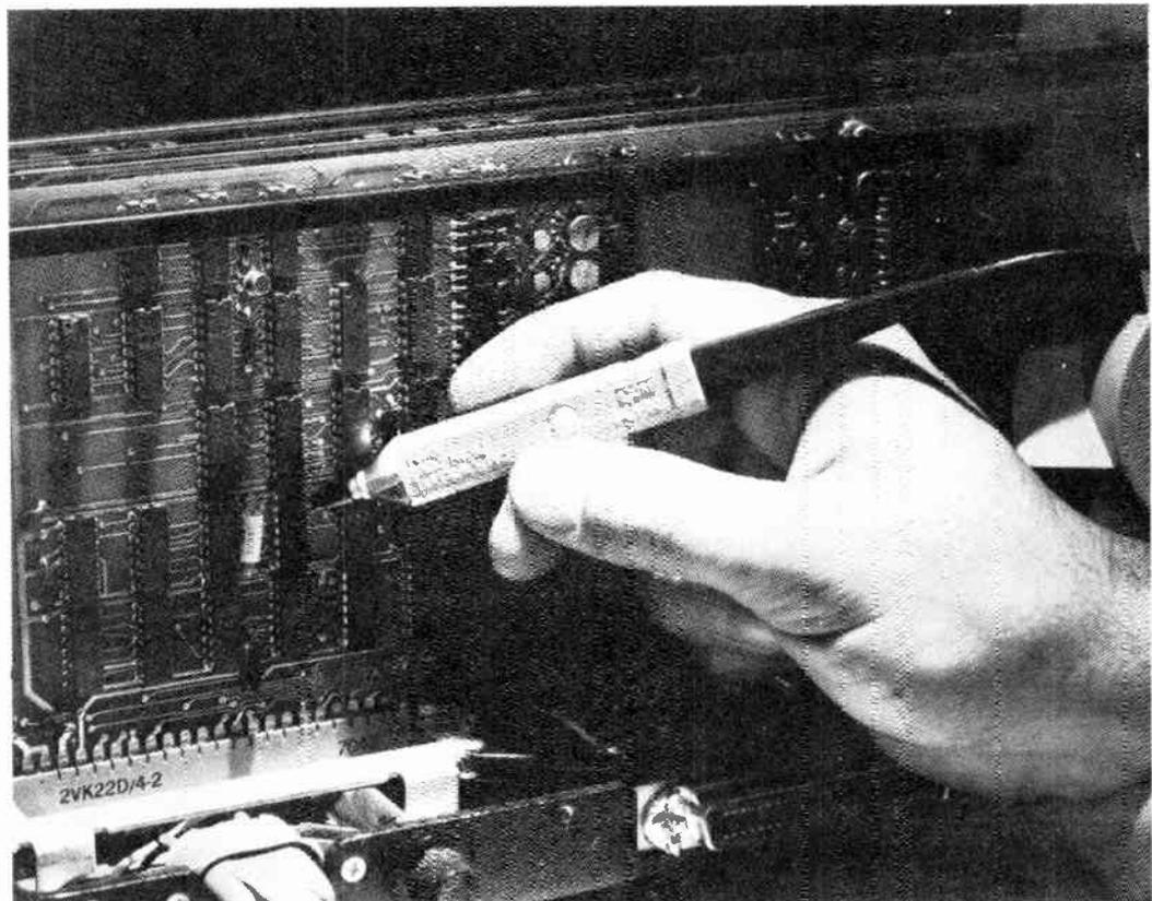
*Fig. 13. Simple logic probe in action.*
