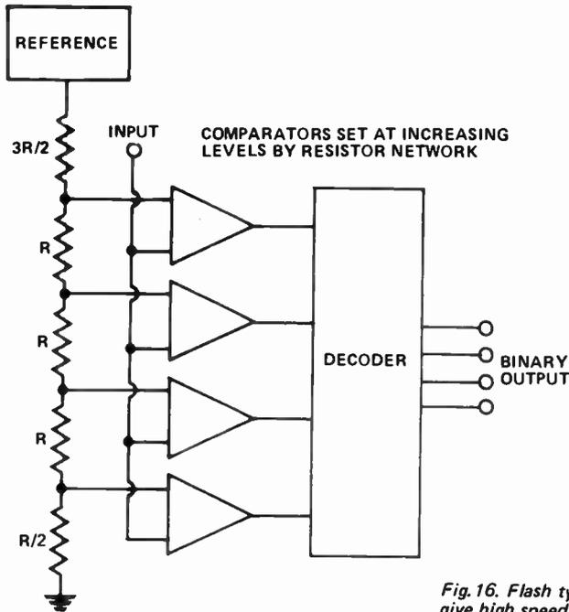
Fig. 16. Flash type converters give high speed A/D conversion.
