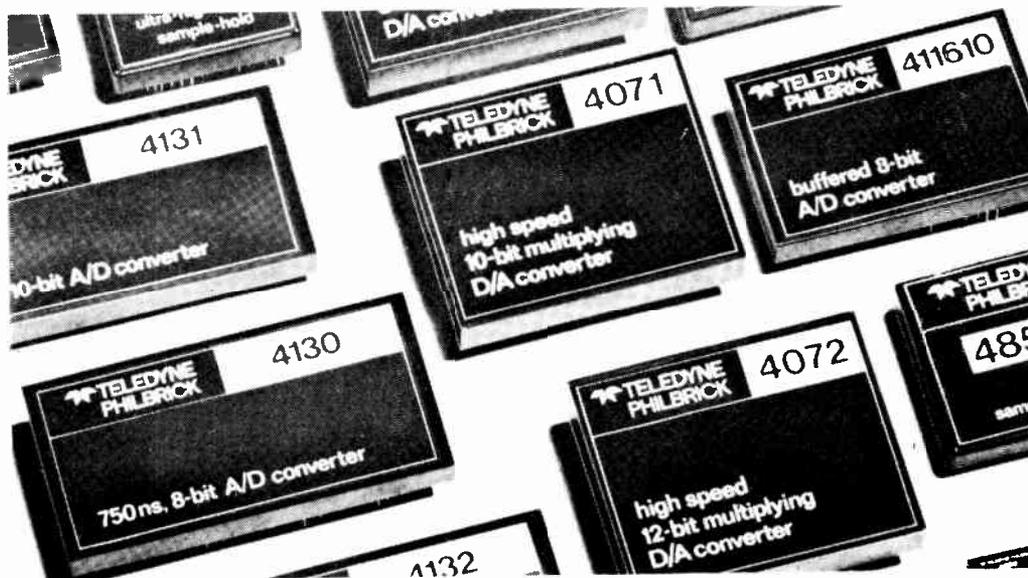
Fig. 1. Typical A/D converters.
