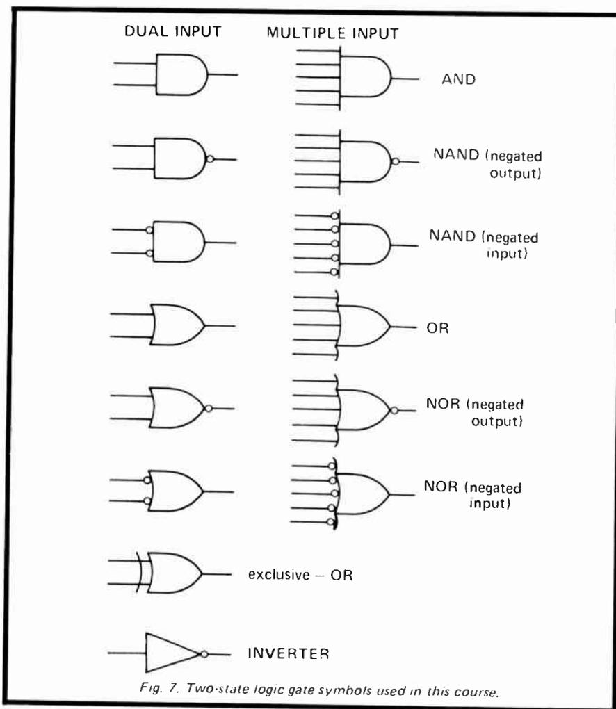
Fig. 7. Two-state logic gate symbols used in this course.
