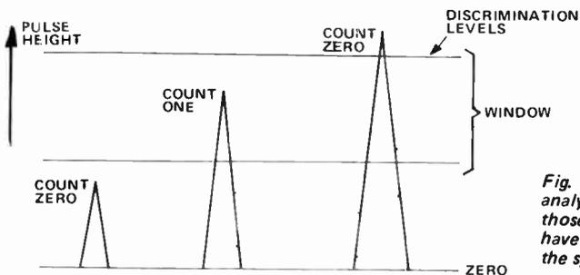
Fig. 15. Pulse-height analysers count only those pulses which have amplitudes within the specified window.
