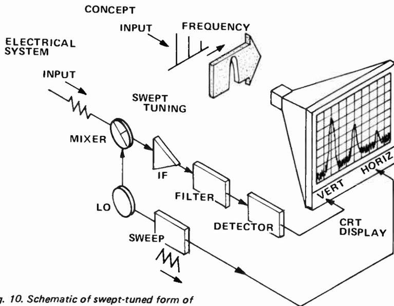
Fig. 10. Schematic of swept-tuned form of spectrum analyser.
