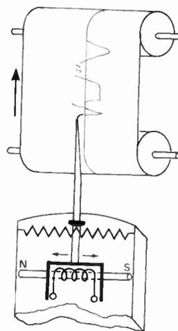
(b) Schematic using linear motor.
