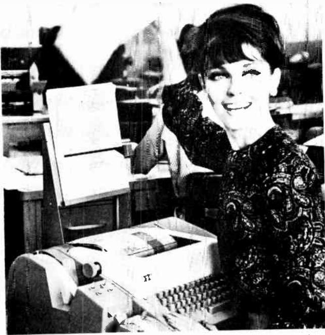
Fig. 3. Keyboard teletype terminals provide hard copy and perforate a paper tape (seen lower left) at the same time. The same facility usually can also print hard copy from a ready made tape.
