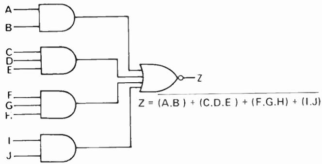
Fig. 13. (a) Logic network for function  $Z = (A \cdot B) + (C \cdot D \cdot E) + (F \cdot G \cdot H) + (I \cdot J)$
