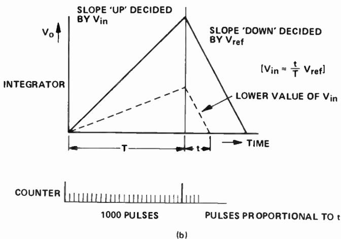
upward ramp counts which, when a 1000 upward limit is used, gives a direct reading of input voltage if the reference voltage is appropriately chosen.
