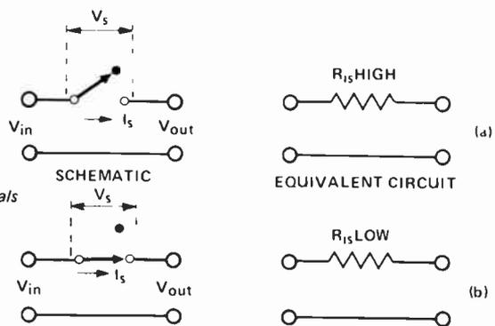
Fig. 4. Switches can handle large power signals with little loss (a) open (b) closed.
