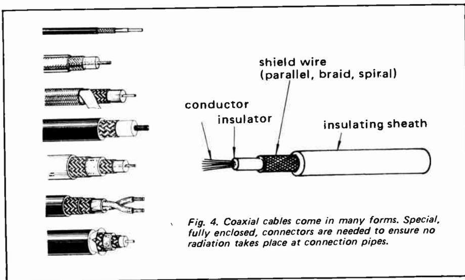
Fig. 4. Coaxial cables come in many forms. Special, fully enclosed, connectors are needed to ensure no radiation takes place at connection pipes.
