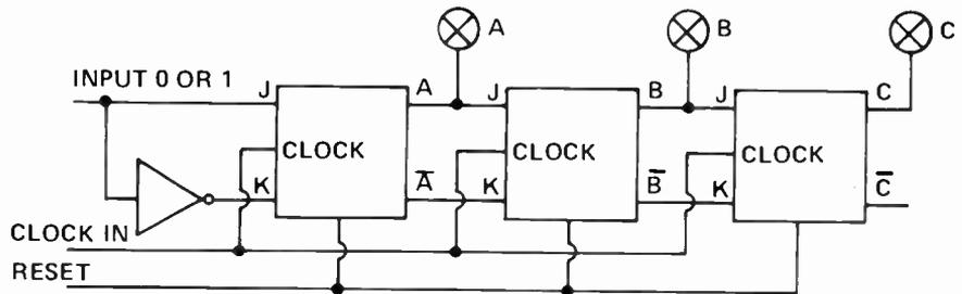
Fig. 6. The shift-register is also built from flip-flops but with different connections to counters. (a) JK type
