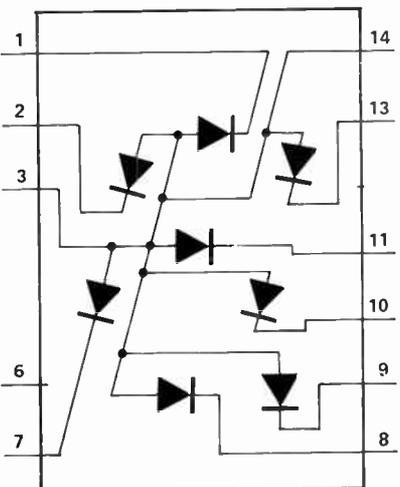
Fig. 12. ABOVE: three seven-segment LED (DL704) displays mounted on a common PC board. LEFT: internal diode positions for a right-hand decimal point seven-segment display module.
