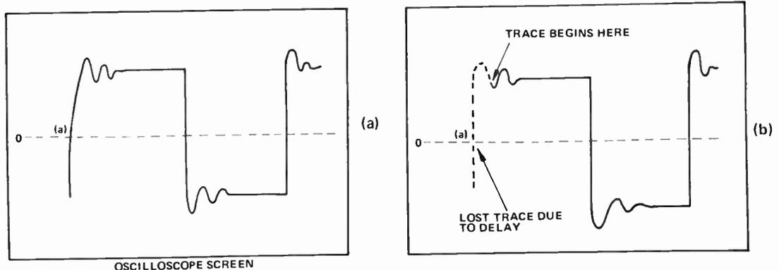
Fig. 7. Inherent trigger delay, if not compensated for, will lose the leading edge of a waveform.
