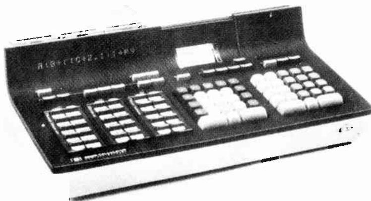
This calculator from Hewlett Packard displays calculations and instructions from the calculator to the user by means of a full alpha-numeric 5 x 7 dot matrix display.
