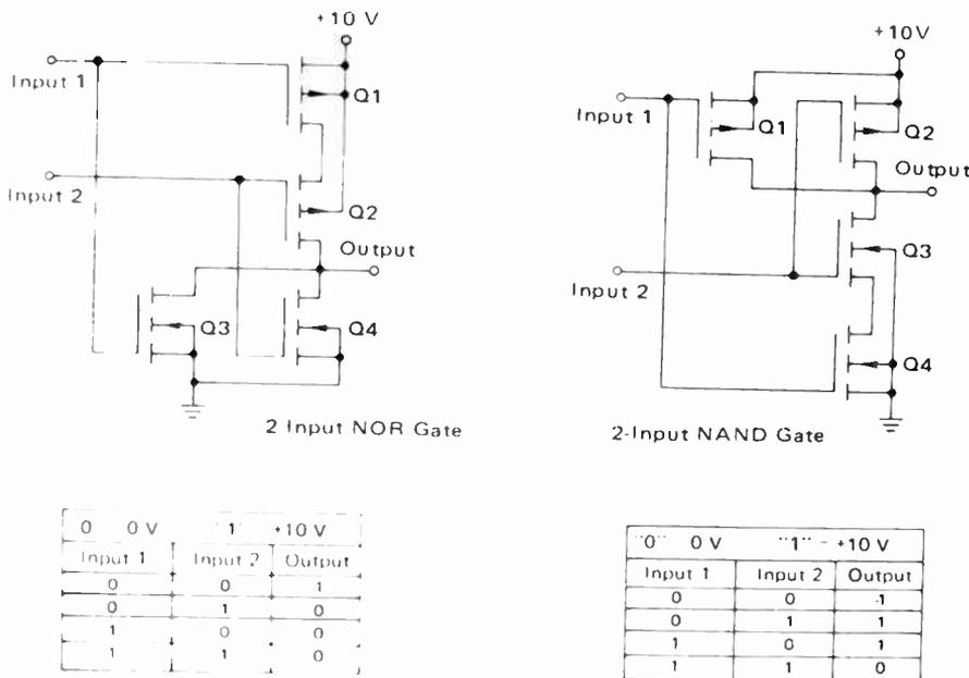
Fig. 9 (a). A CMOS 2-input NOR gate.
