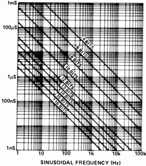
Fig.21. Graph showing relationship between aperture time required, resolution of signal conversion and frequency of sinusoidal signal undergoing conversion.
