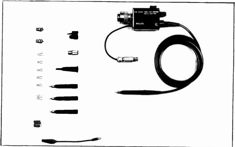
Fig. 15. This FET probe uses active coupling to overcome oscilloscope connection problems.
