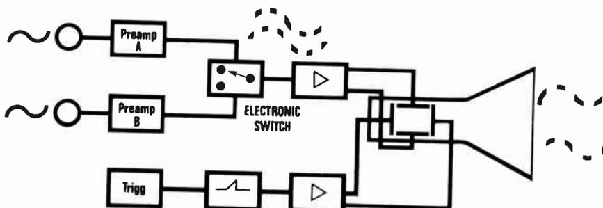
Fig. 10. Electronic-switching enables a single-beam and deflection system to provide dual-trace operation.
