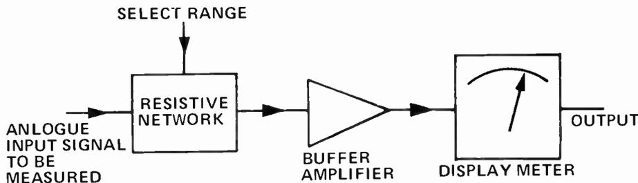
Fig. 1. Schematic representation of analogue multimeter system.
