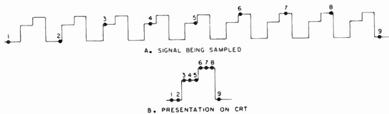
Fig. 5. The sampling oscilloscope builds up the waveform on the screen from sampled values taken from the original.
