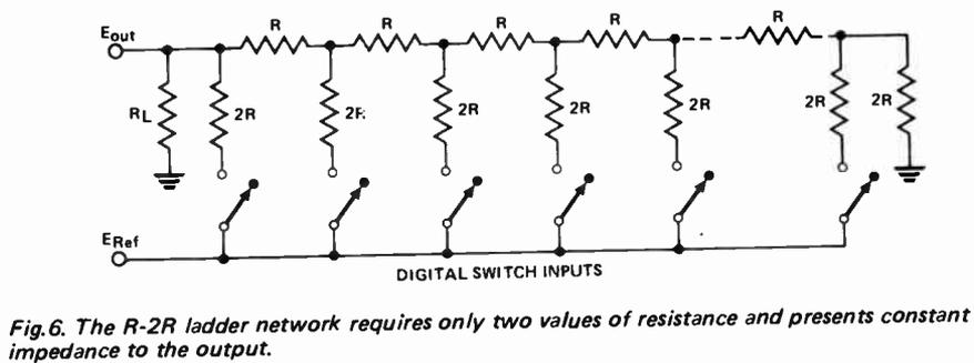
Fig.6. The R-2R ladder network requires only two values of resistance and presents constant impedance to the output.
