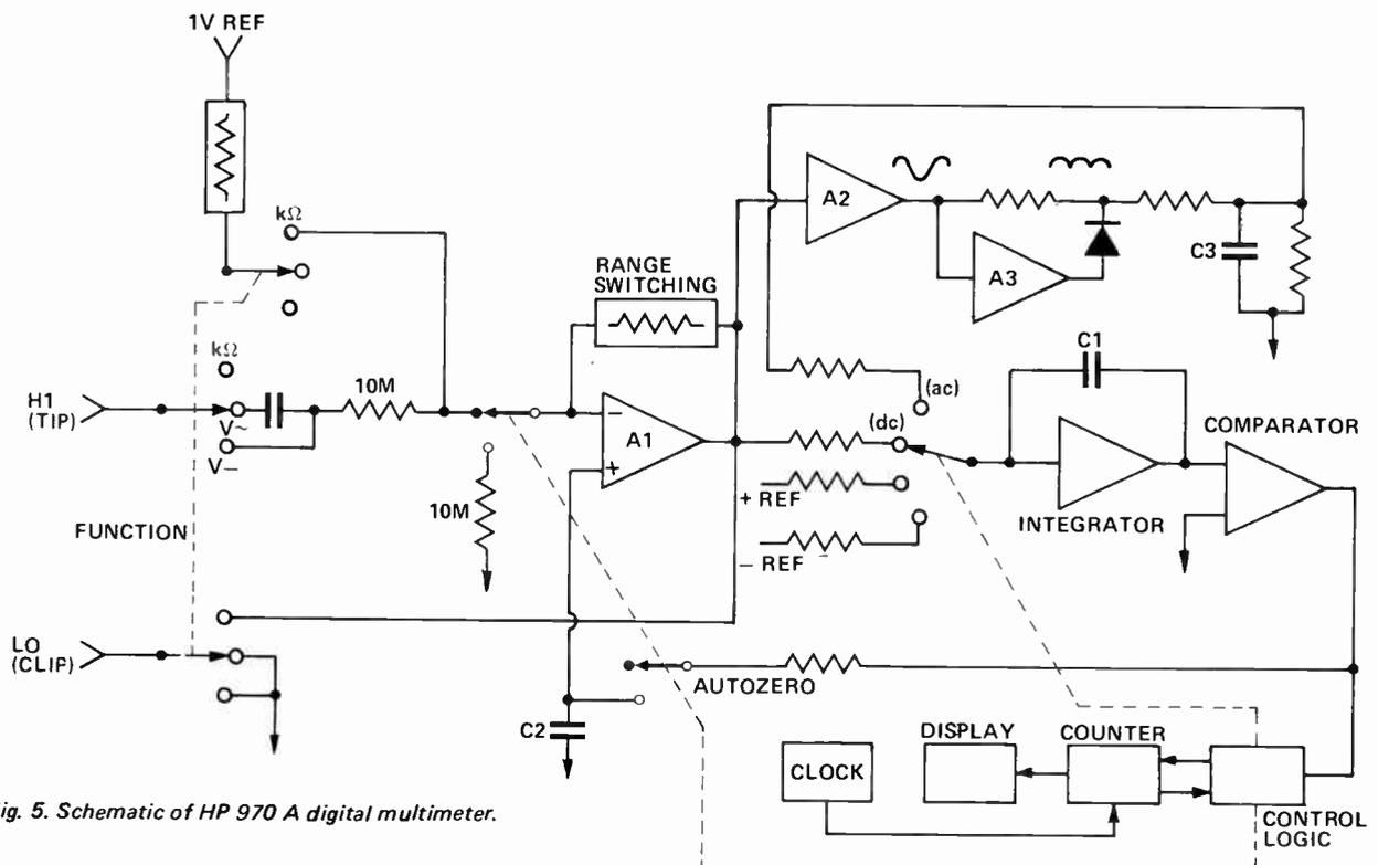
Fig. 5. Schematic of HP 970 A digital multimeter.
