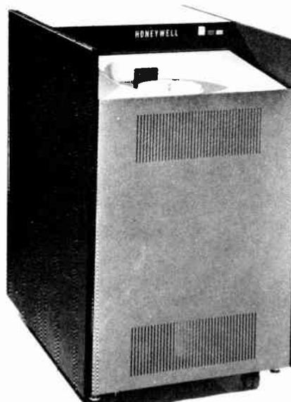
Fig. 16. Honeywell model 4720 moving-head disk storage device.
