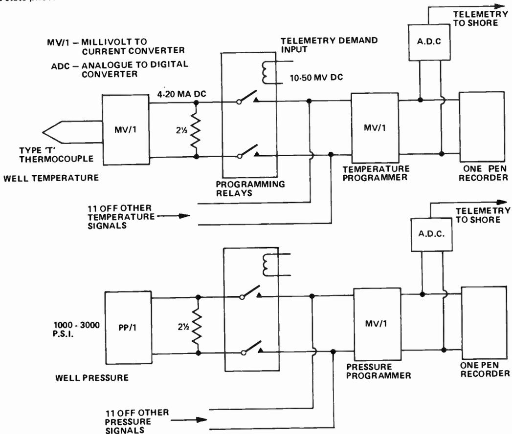
Fig. 8. Process measurement link arrangements used between the oil-well and the off-shore platform. The A/D units send the data to a shore-based computer by digital telemetry links.
