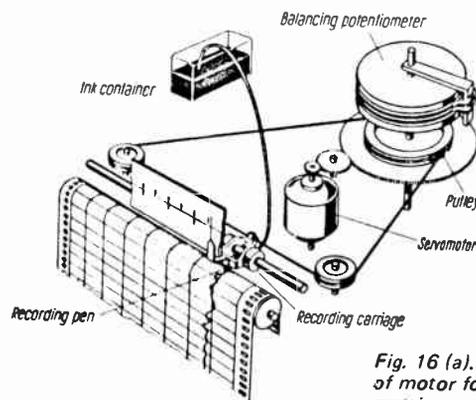
Fig. 16 (a). Arrangement of motor form of potentiometric recorder.
