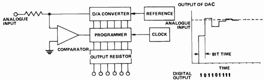
Fig. 19. In the successive approximation A/D converters a DAC is used to convert the incremented digital stage output back to analogue form for comparison with the input.
