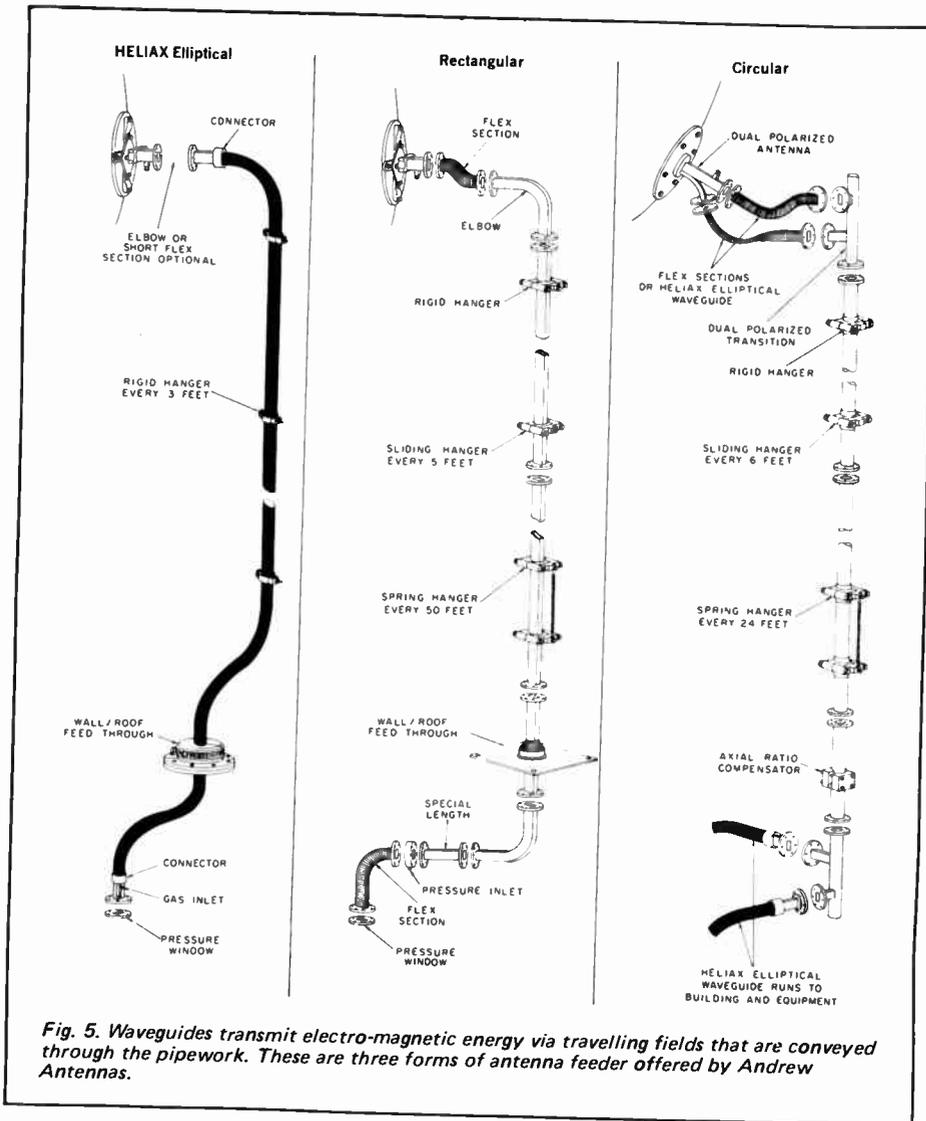
Fig. 5. Waveguides transmit electro-magnetic energy via travelling fields that are conveyed through the pipework. These are three forms of antenna feeder offered by Andrew Antennas.
