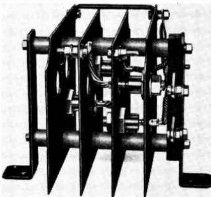
Fig. 1. Power handling stages are easily identified by the heatsink assemblies on which they are mounted — a 35 A, 60 VDC rectifier stack is shown here.
