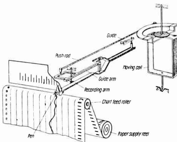
Fig. 13. Special linkages are used to linearize the non-uniform movement produced by a moving coil pen drive.
