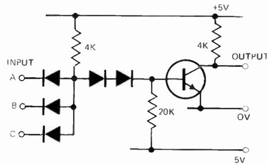
Fig. 3. An early integrated circuit design for a NAND gate in diode-transistor logic – DTL.
