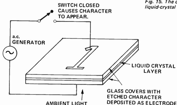
Fig. 15. The construction of a liquid-crystal display.
