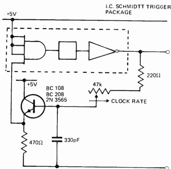
Fig. 18(a) LEFT: A Schmitt trigger combined with a transistor provides an astable multivibrator action.
