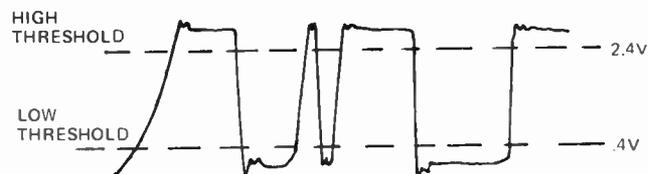
Fig. 5. Typical output signal from TTL, note the transient ringing at each transition.
