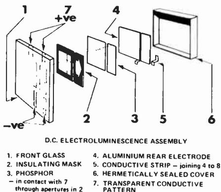
Fig. 5. Schematic of a dcel electroluminescent display panel.
