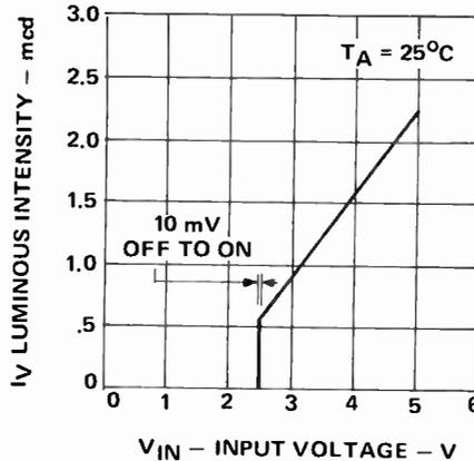
Fig. 10. LEDs with integrated voltage sensing amplifiers turn on when the applied voltage exceeds a built-in value.
