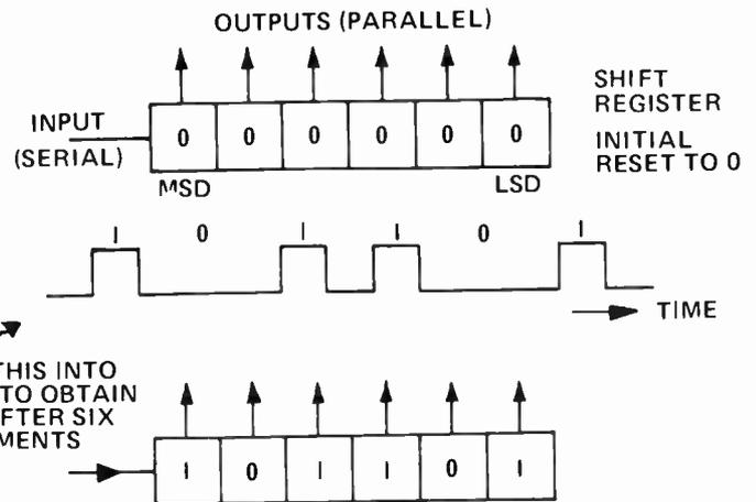
Fig. 8. Registers can provide serial to parallel word conversion, the reverse also applies.
