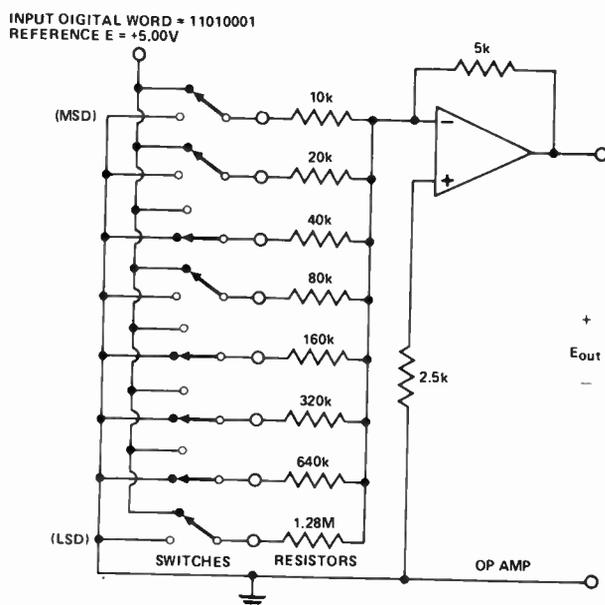
*Fig.4. Switched resistor network of 8-bit, binary weighted D/A converter. 11010001 is being converted.*
