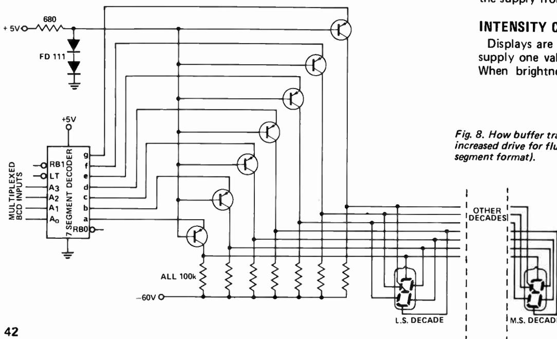
Fig. 8. How buffer transistors are used to obtain increased drive for fluorescent displays (seven-segment format).
