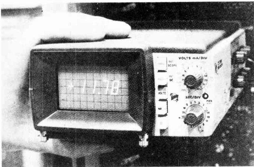
*Fig. 7. The digital multimeter function is combined with a C.R.O. facility in the Tektronix 213 unit.*
