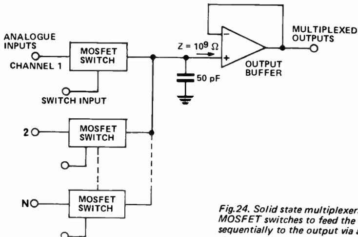
Fig.24. Solid state multiplexers use MOSFET switches to feed the inputs sequentially to the output via a buffer stage.
