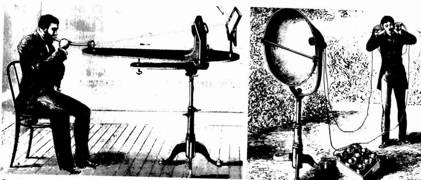
Fig. 6. This Photophone of Bell and Tainter was designed in 1881. Sunlight reflected to the receiver was modulated by acoustic waves vibrating the speaking tube mirror. Detection was with a selenium photo-electric cell driving earphones.
