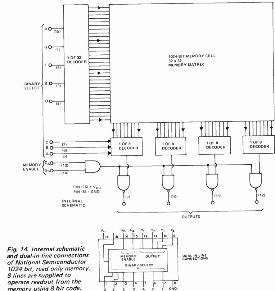
Fig. 14. Internal schematic and dual-in-line connections of National Semiconductor 1024 bit, read only memory. 8 lines are supplied to operate readout from the memory using 8 bit code.
