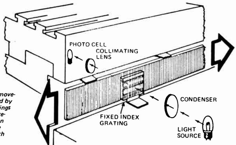
Fig. 3. Accurate measurement of movement is performed by using optical gratings to produce "moire-fringes" which can be counted as the gratings move with respect to each other.
