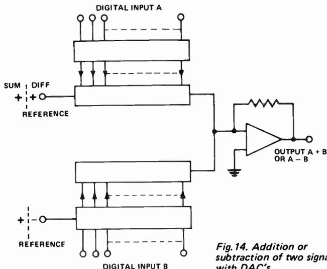
**Fig. 14. Addition or subtraction of two signals with DAC's.**
