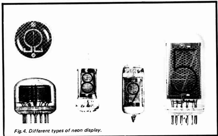
Fig.4. Different types of neon display.
