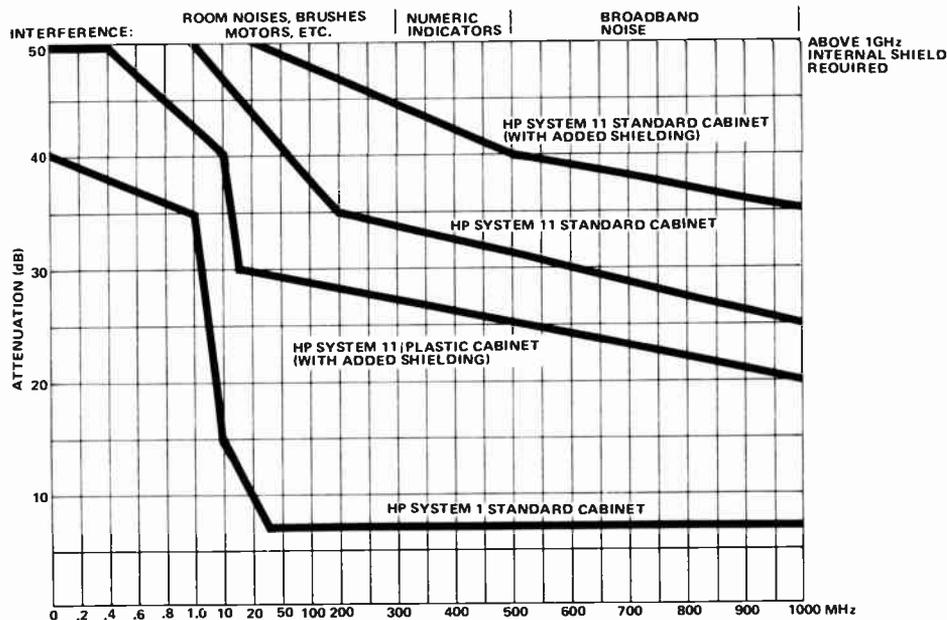
Fig. 15. Shielding of RF energy by various designs of enclosure used for H.P. instruments. The actual value of a particular unit depends upon the need for holes and shafts through the panels.
