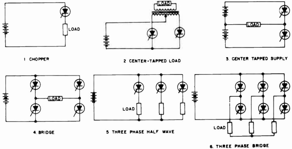
Fig. 10. Various inverter configurations using SCR switches. Triggering methods have been omitted for clarity.
