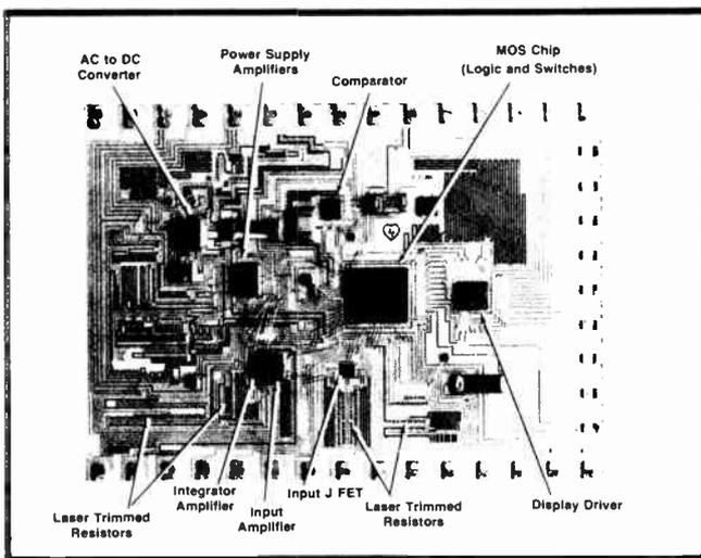
*Fig. 6(b). Thin-film hybrid of HP 970A carries much of the analogue circuit on its 28 x 38 mm substrate.*
