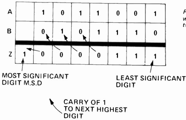
Fig.14. Addition of two binary numbers proceeds with a carry as for decimal arithmetic but with only two states 0, 1 in each digit.
