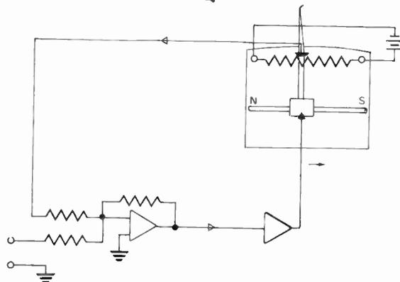
(c) Circuit schematic of potentiometric method (simplified).
