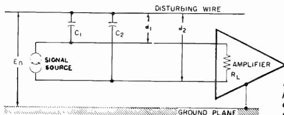
Fig. 13. Common-mode pick-up of noise is balanced out by the differential system.
