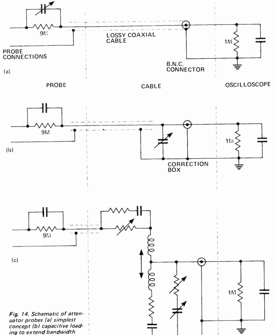
Fig. 14. Schematic of attenuator probes (a) simplest concept (b) capacitive loading to extend bandwidth (c) inductive.
