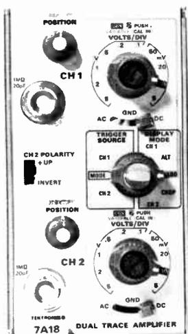
Fig. 11. Example of dual-trace plug-in showing the basic controls.
