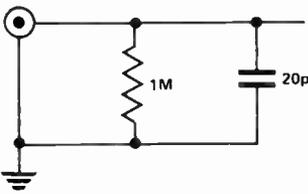
Fig. 12. Most oscilloscopes have this input equivalent circuit. Although the values seem insignificant, at high frequencies they become dominant requiring the use of special probes.
