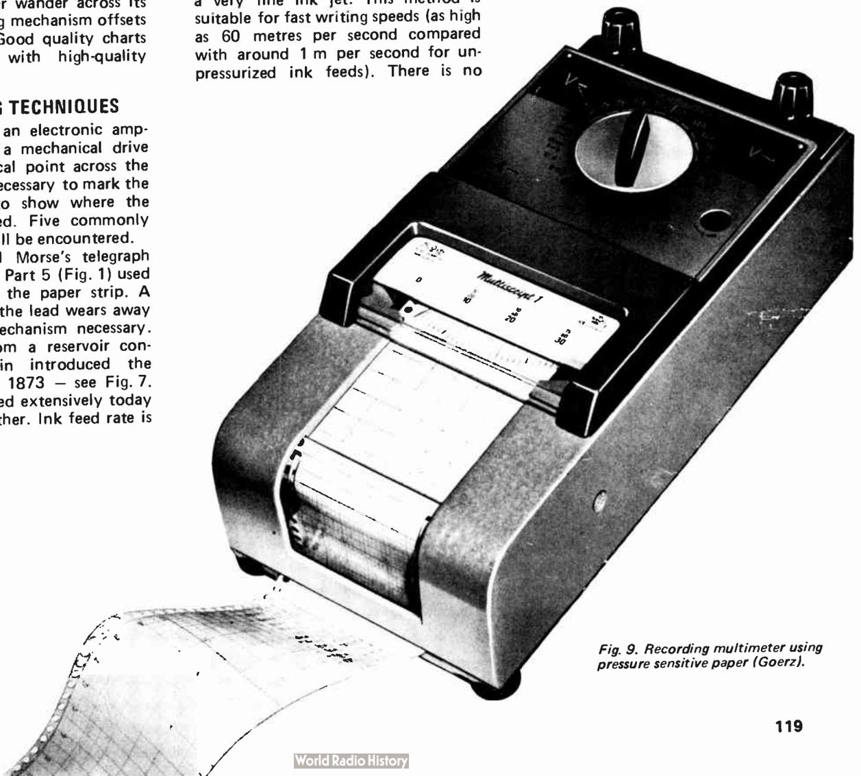
Fig. 9. Recording multimeter using pressure sensitive paper (Goerz).
