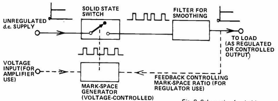
Fig. 8. Schematic of switching regulator or controller (see text).
