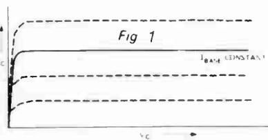
First, let's see how a constant current source works. Transistor Q1 and associated components provide the constant current source for the probe. Figure 1 shows the collector characteristics of a typical silicon transistor. They show that, if you hold the base current constant, the collector current will
