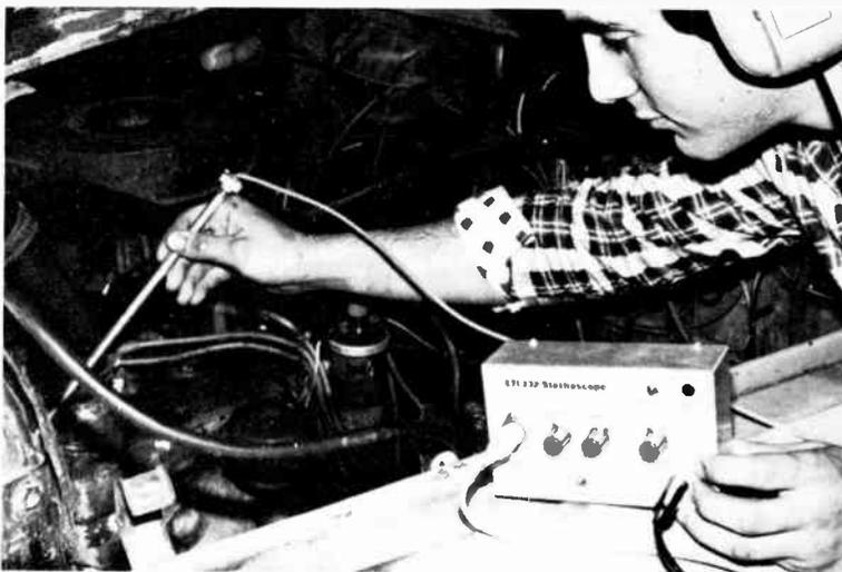
Using the stethoscope to listen to the water pump in a car engine.
