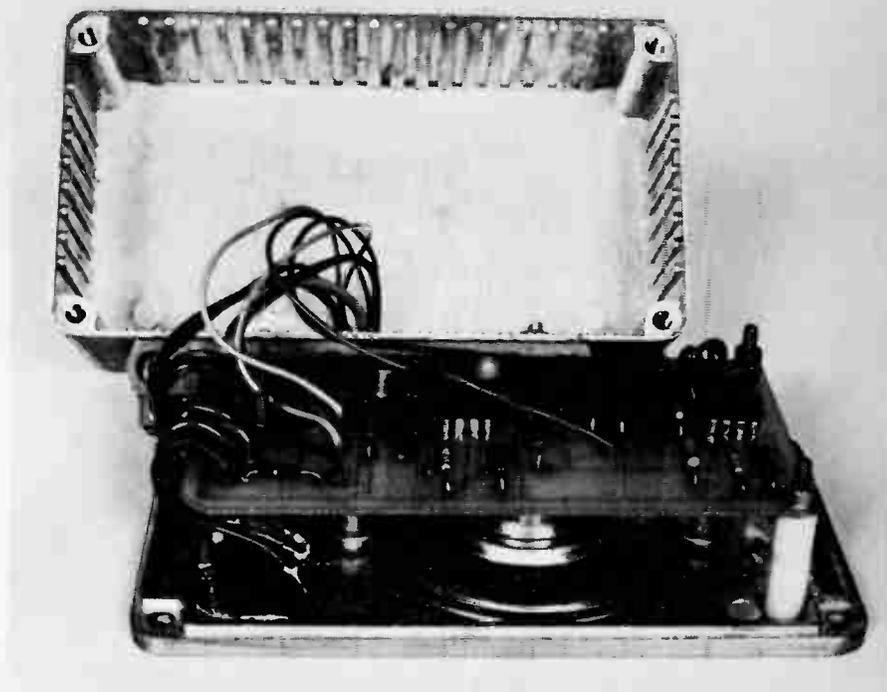
Our unit was assembled into a diecast box using standoff pillars to support the pc board. If you use an 8 ohm or 16 ohm speaker with a series resistor, the value of the resistor can be varied to alter the speaker volume. With a high impedance speaker, a suitable value resistor may be inserted in series to lower the volume. Try 100 ohms as a start.
