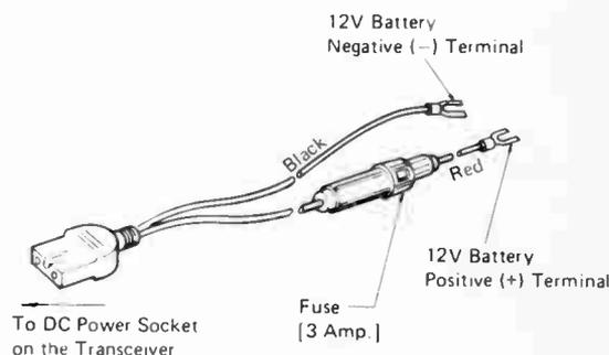
Before making any power connections, determine whether the vehicle, boat, etc, has a negative or positive earth electrical system. Reverse connection could damage or destroy the transceiver circuitry. The red power lead connects to the '+' (positive) side of the electrical system and the black lead to the vehicle '-' (negative) side of the electrical system.
