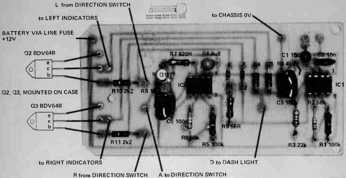
Component overlay and external component connections.
