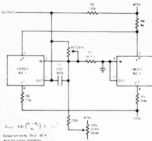
\*The 0.01 in the above equation is in units of  $\text{V}/^{\circ}\text{K}$  or  $\text{V}/^{\circ}\text{C}$  and is a result of the basic  $0.01 \text{ V}/^{\circ}\text{K}$  sensitivity of the transducer
