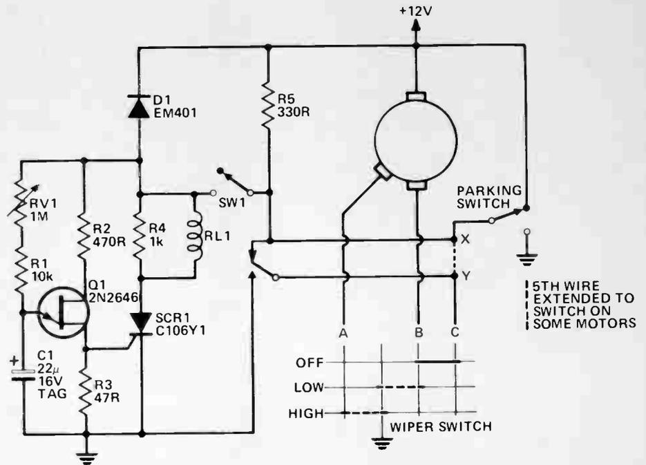
Fig. 2. The ETI319B Vari-Wiper circuit using relay output for use with permanent magnet motors.
