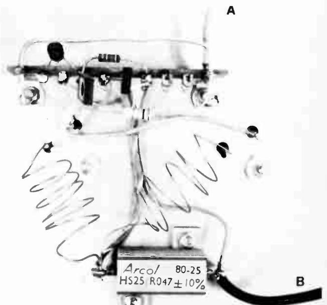
Construction of the light globe substitute circuit. Layout is not critical.
