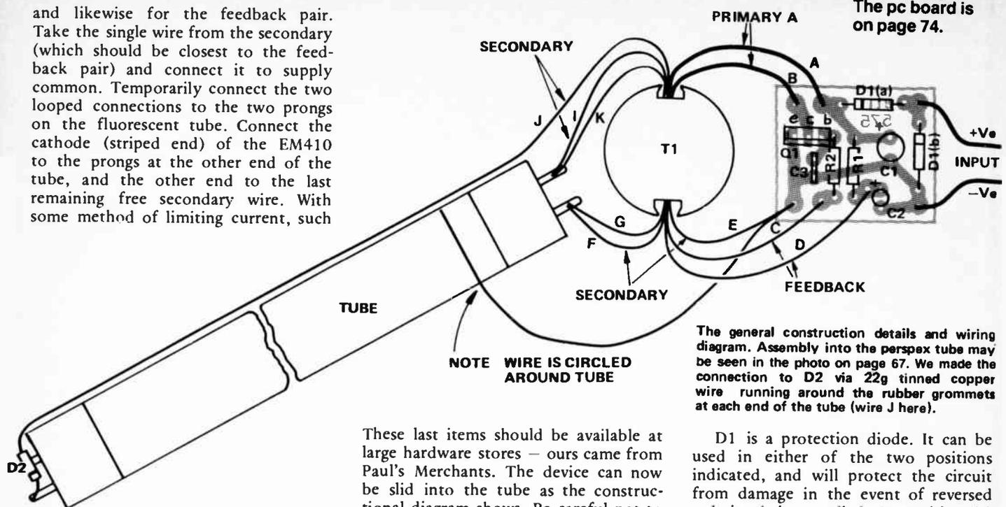
The general construction details and wiring diagram. Assembly into the perspex tube may be seen in the photo on page 67. We made the connection to D2 via 22g tinned copper wire running around the rubber grommets at each end of the tube (wire J here).
