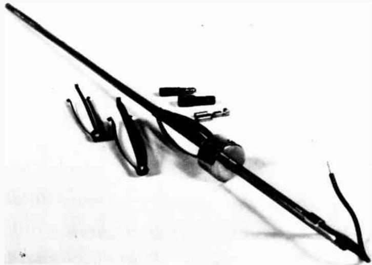
The V.D.O. dipstick probe with its associated parts. Full assembly details are given on page 33.
