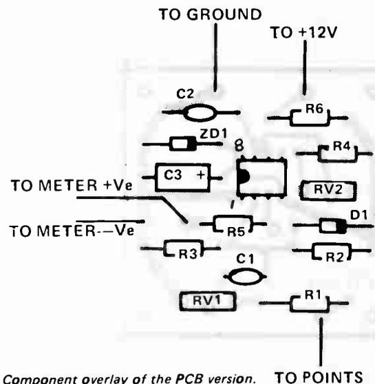
Fig. 3. Component overlay of the PCB version.
