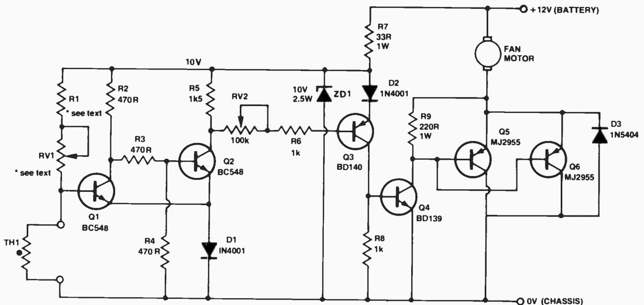
thermistor controls a Schmitt trigger (Q1 and Q2) which drives several power transistors (Q5 and Q6), connected in series with the fan motor, via two intermediate stages (Q3 and Q4).
