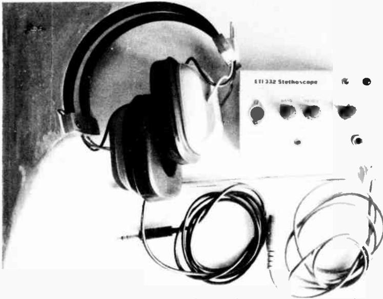
Completed stethoscope, ready for action! The probe here was made from a crystal eartip, a length of 10 mm tubing being pushed over the ear plug.
