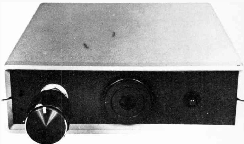
one range will be necessary so the switch and three unused trim pots can be left out. The unit can be set to any rev limit, say 6000 revs, to indicate when you're coming close to over-revving the engine. The actual limit depends on the particular engine in your vehicle.
