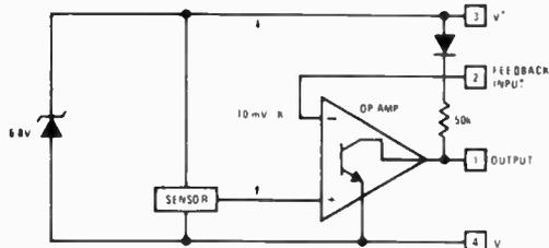
Internal block diagram of the LM3911.
