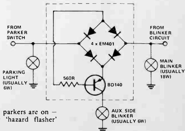
here which he then fitted into a plastic pill bottle (useful things) and inserted into the wiring at each side of his car.
