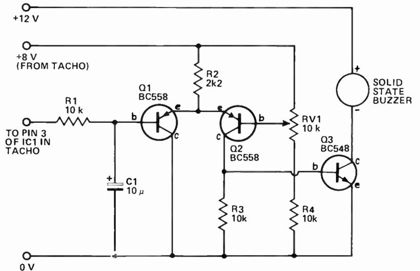
Circuit diagram of add-on unit – note that a connection must be made from the +ve side of the solid-state buzzer to the +12 volts.
