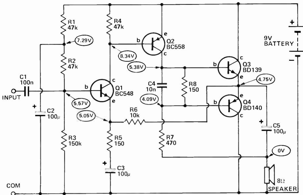
Fig. 1. Circuit diagram of the amplifier.
