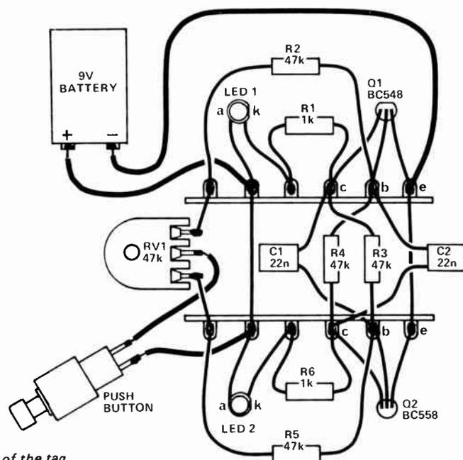
Fig. 1. Layout of the tag strip version.
