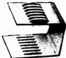
This is a typical heatsink for small power transistors. (20 mm x 20 mm). It can easily be bolted on to the rear of the transistor – heat sinks such as this may be bought from most component suppliers – or made up from a short strip of copper or aluminium.
