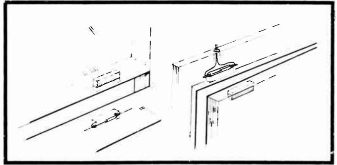
Set the reed switch into the window frame and the magnet in to the moving part.
