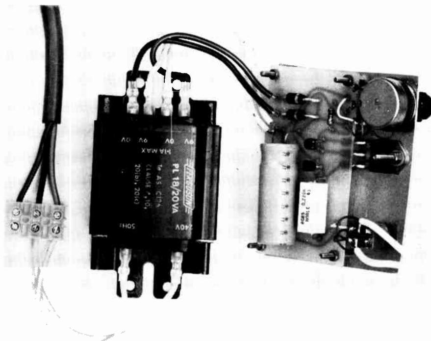
within this specification are the requirements that the mains input connections be shielded, that they be on the opposite side of the transformer from the output, that specially heavy insulation be used (in that the primary winding is kept right away from the secondary winding) – and so on.
