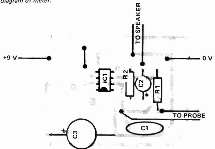
Component overlay of PCB unit.
