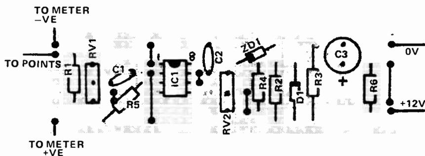
Fig. 5. Component overlay for the Veroboard version.
