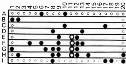
Drilling details of Veroboard.
