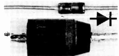
Two diodes, black band (top) and white band (bottom) indicate the cathode (-ve) end of the component Bands correspond to bar on symbol in circuit diagrams.
