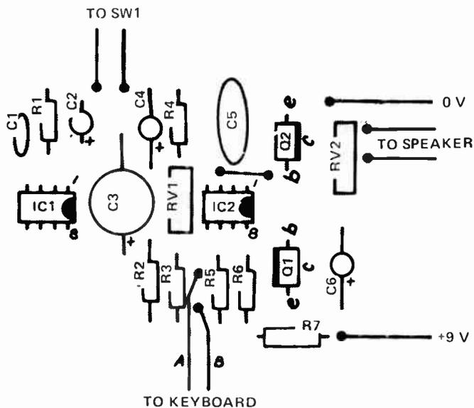
Component overlay for printed circuit board version.
