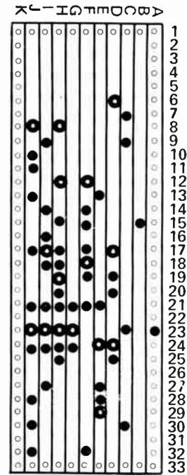
*This is how the components are mounted on the Veroboard version. Note particularly that two alternative positions are shown for resistor R1 – the position chosen depends upon whether 'under alarm' or 'over alarm' operation is required. Similar comments apply to the pc board version shown on the right.*
