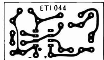
Fig. 5. Printed-circuit board layout (copper side). Full size of this board is 50mm x 30mm.
