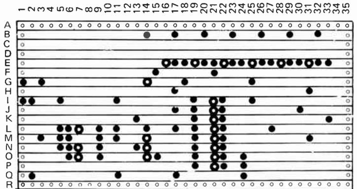
Fig. 4. Cut the Veroboard track in the places indicated by the pads with holes. The other dots are where soldered connections are made.
