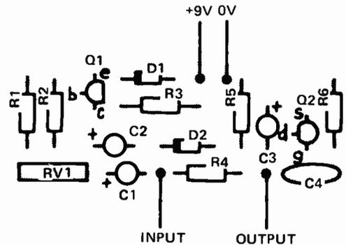
Component layout of printed circuit board version.
