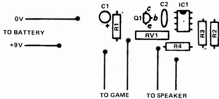
Here's how the components are located in the printed circuit board version of the game.
