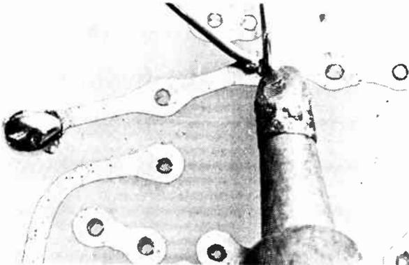
Fig.9. Apply the soldering iron to the joint so that the track and component wire are heated together for about two seconds, then apply the solder to the joint — NOT to the soldering iron tip.
