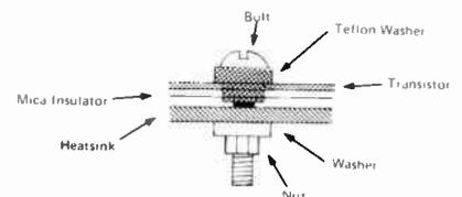
These two drawings show how the heatsink attached to Q2 may be insulated. Note that the transistor should be mounted tight against the heatsink to increase thermal conductivity.
