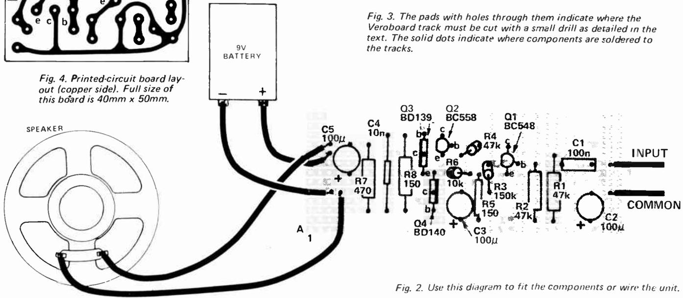
Fig. 2. Use this diagram to fit the components or wire the unit.
