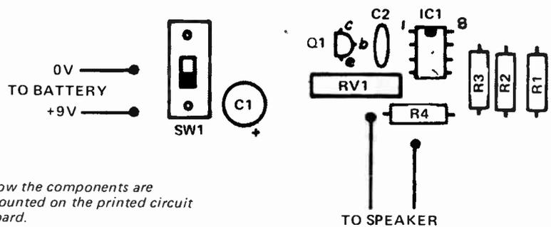
How the components are mounted on the printed circuit board.
