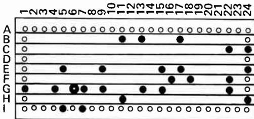
Fig. 5 Cut the Veroboard track in the place indicated by the pad with the hole. The other dots are where soldered connections are made.
