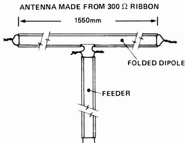
*Fig.1. This simple folded dipole may be constructed from a short length of 300 ohm ribbon tied in position or tacked to suitable pieces of wood or hardboard.*
