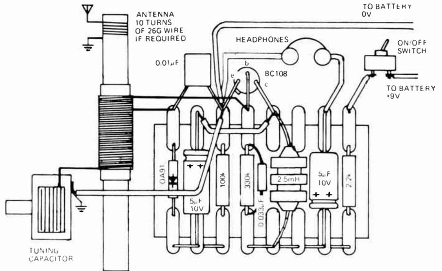
*Tag Strips – construction is quick, cheap and simple. However the method is only really suitable for small scale projects as inter-tag wiring will otherwise be extensive and tedious. The method also wastes space. (Circuit shown is of a single transistor reflex receiver first published in our December 1971 issue).*
