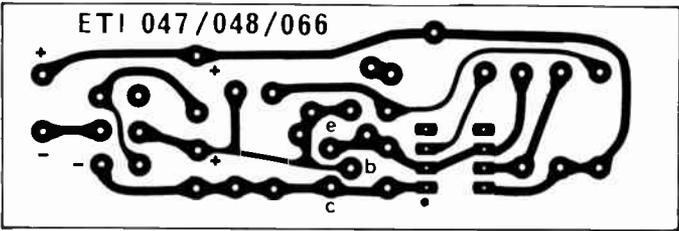
The PCB used in this project is also applicable in projects 047, 048 and 066. It is an ETI general purpose 555 PCB.
