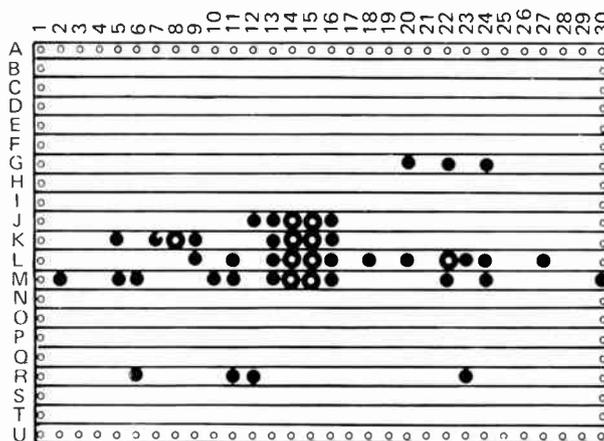
Fig. 2. The pads with holes through them indicate where the Veroboard track must be cut with a small drill as detailed in the text. The solid dots indicate where components are soldered to the tracks.
