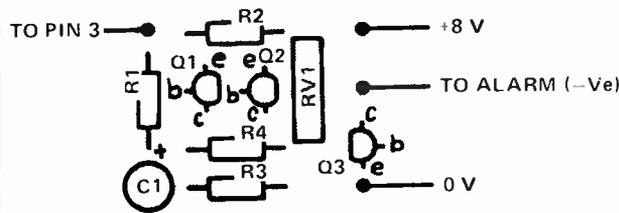
The printed circuit component overlay. Make sure all transistors are installed in the correct position corresponding to the overlay.
