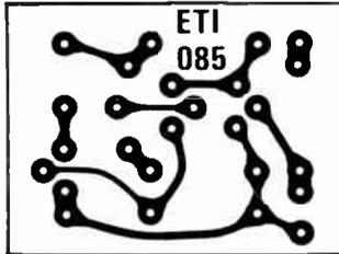
Printed circuit board layout – full size.
