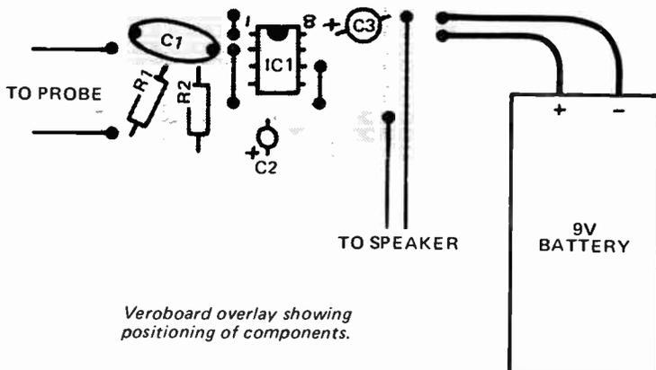
Veroboard overlay showing positioning of components.
