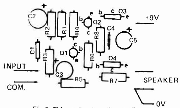
Fig. 5. This overlay shows how to fit components to the printed-circuit board.
