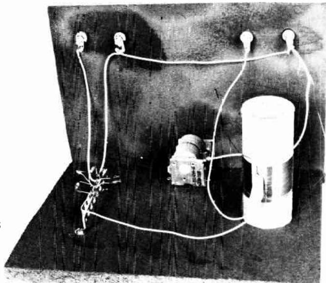
*RIGHT: Rear view of the crystal set showing placement of components and interconnections. The dial on the front panel was cut from cardboard and lettered with rub-down lettering (see opposite page).*
