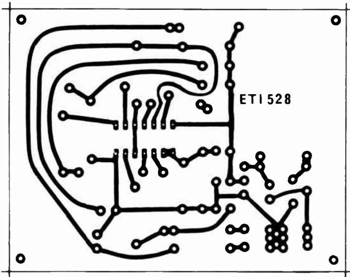
Printed circuit board layout. Full size is 90 mm by 70 mm.
