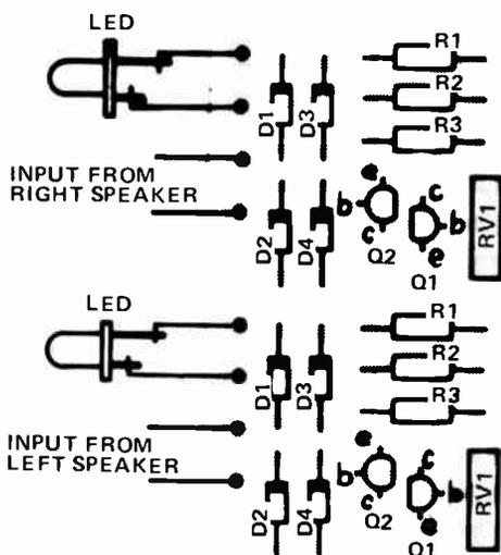
Fig. 2. This is the component overlay of the printed circuit version. Note that the board contains two separate but identical circuits.
