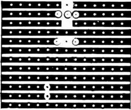
*Veroboard – board has copper tracks bonded to non-component side. Breaks are cut where necessary. Component leads are soldered to tracks on copper side of board.*
