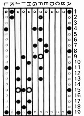
Drilling details for Veroboard of over-rev alarm. Dots mean solder points while hollow circle indicates a hole cutting the copper track.
