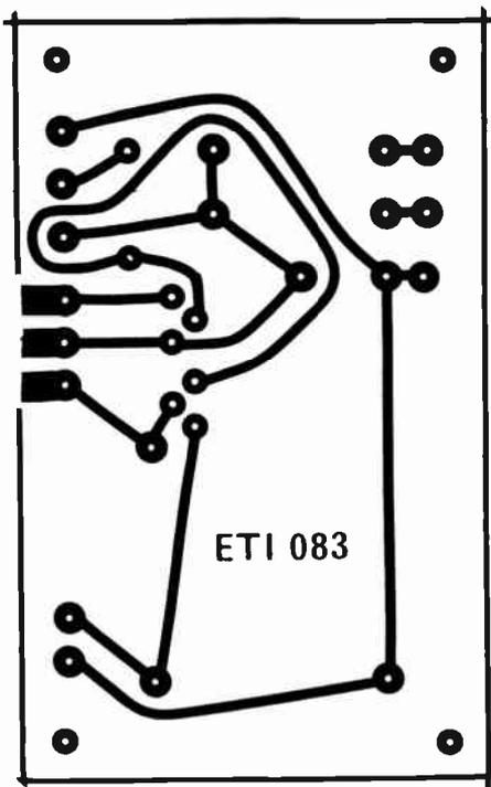
Printed circuit board pattern (shown here full size).
