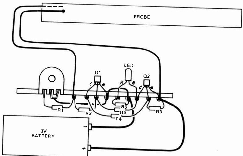
*Component arrangement. Note connections of transistors. The probe shown here is made from a small section of double sided PC board. One wire (dotted) leads to the obscured side, the other (solid) connects to the uppermost side.*
