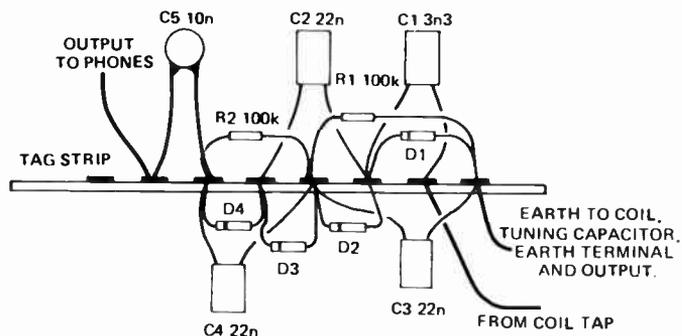
As with the simple crystal set, we mounted the components for the voltage-multiplier crystal set on an eight-lug tag strip. We have supplied a drawing as it is clearer than a photo in this instance.
