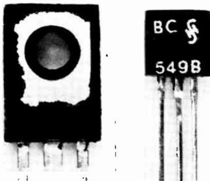
Two transistors. To the left is BD140. Note metal backing for heat dissipation. Right a BC549, Philips type with bent centre lead, which has different pin configurations than other transistors of the same type. Check in the back of this book for connections.
