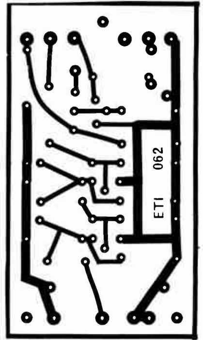
Fig 3. Printed circuit board layout for the tuner. Full size 90mm x 50mm.
