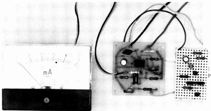
*The components for the over-rev alarm are mounted on the board seen on the right of the main tachometer board.*
