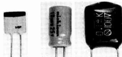
Three types of capacitors, (left) ceramic, (middle) electrolytic, and polyester (right).
