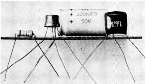
When components are fitted to a board the leads should be splayed, as shown, to keep them in position prior to soldering. Position components so that values and voltage ratings may be seen. This facilitates later servicing.
