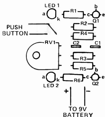
Fig. 2. Layout of the printed-circuit board version.
