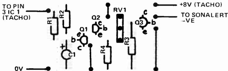
Veroboard component overlay. Note polarity of transistors and the capacitor.
