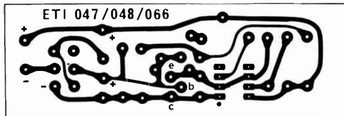
*Printed Circuit board pattern – such patterns are usually shown full-size. The black strips are the inter-connecting tracks between components and are formed by etching away the rest of the copper – see main text for full description.*
