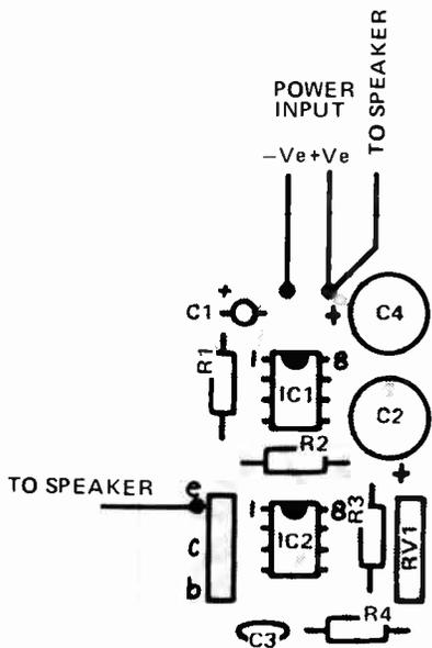
Component overlay. Note polarity of electrolytic capacitors and 555 IC's.
