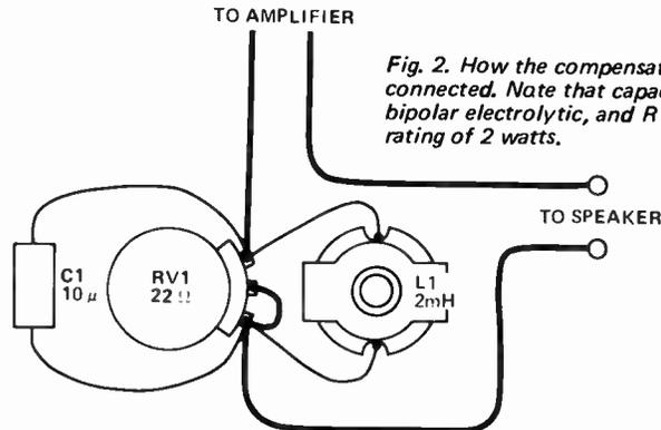
Fig. 2. How the compensation network is connected. Note that capacitor C1 is a bipolar electrolytic, and RV1 has a minimum rating of 2 watts.
