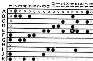
This is the drilling details for the Veroboard version. Do make sure that the breaks required (shown as black dots) are clean, and that no 'whiskers' remain.
