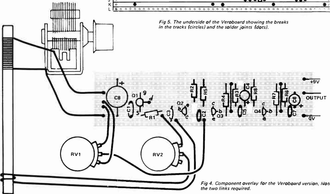
Fig 4. Component overlay for the Veroboard version. Note the two links required.
