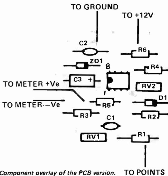
Fig. 3. Component overlay of the PCB version.
