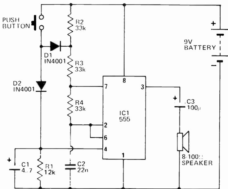
Fig. 3. Circuit diagram of the two-tone doorbell.
