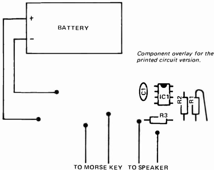
Component overlay for the printed circuit version.
