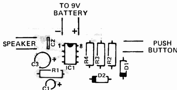
Fig. 4. This overlay shows how to fit components to the printed-circuit board.
