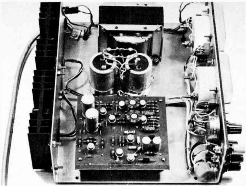
is compared against the voltage set by RV1 by operational amplifier IC3. The output of IC3 controls the series regulator configuration, and hence the output voltage. The action of IC3 is to keep the two voltages at its input at the same level. Thus, the output voltage will be four times the input voltage, and virtually independent of load current.
