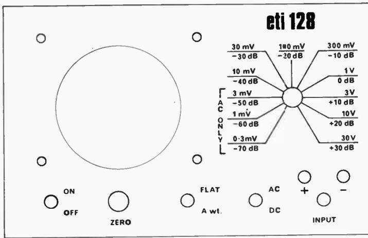
Fig. 6. Front panel artwork. Full size 189 x 121 mm.
