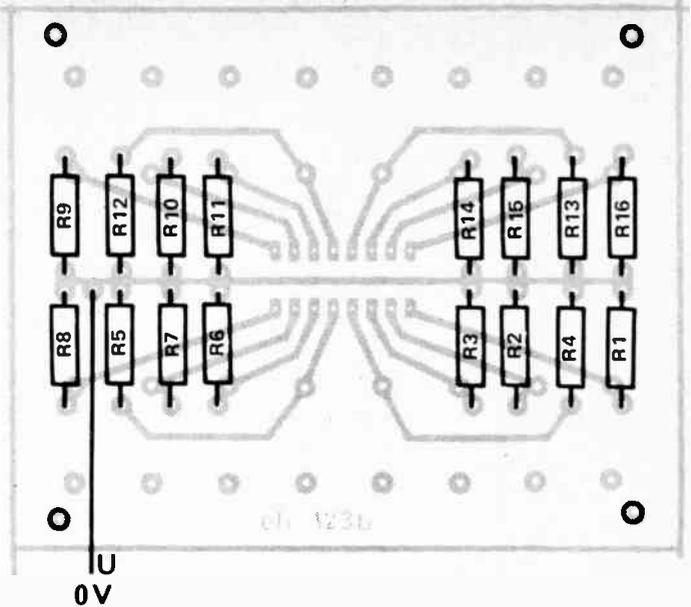
Fig. 3. Component overlay for the copper side of board ETI-123b.
