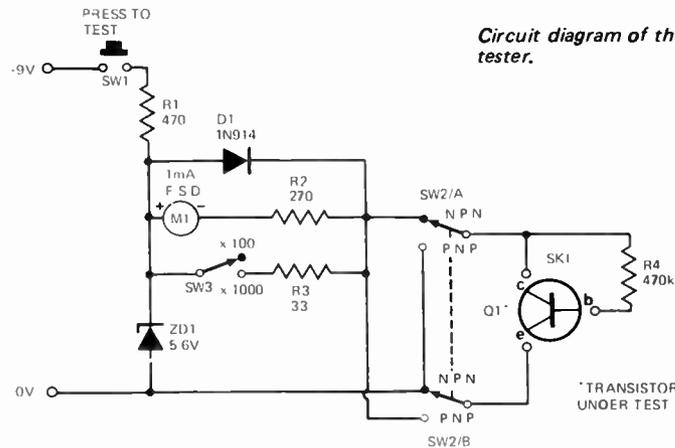
Circuit diagram of the ETI transistor tester.
