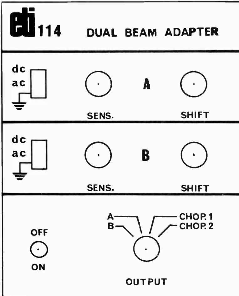
Fig.5. Artwork for front panel of the adaptor.
