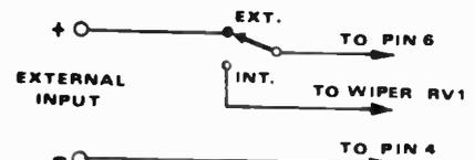
Fig. 2. Circuit modifications for externally programming positive rail (see text).
