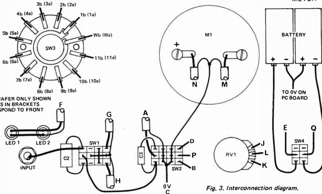
Fig. 3. Interconnection diagram.
