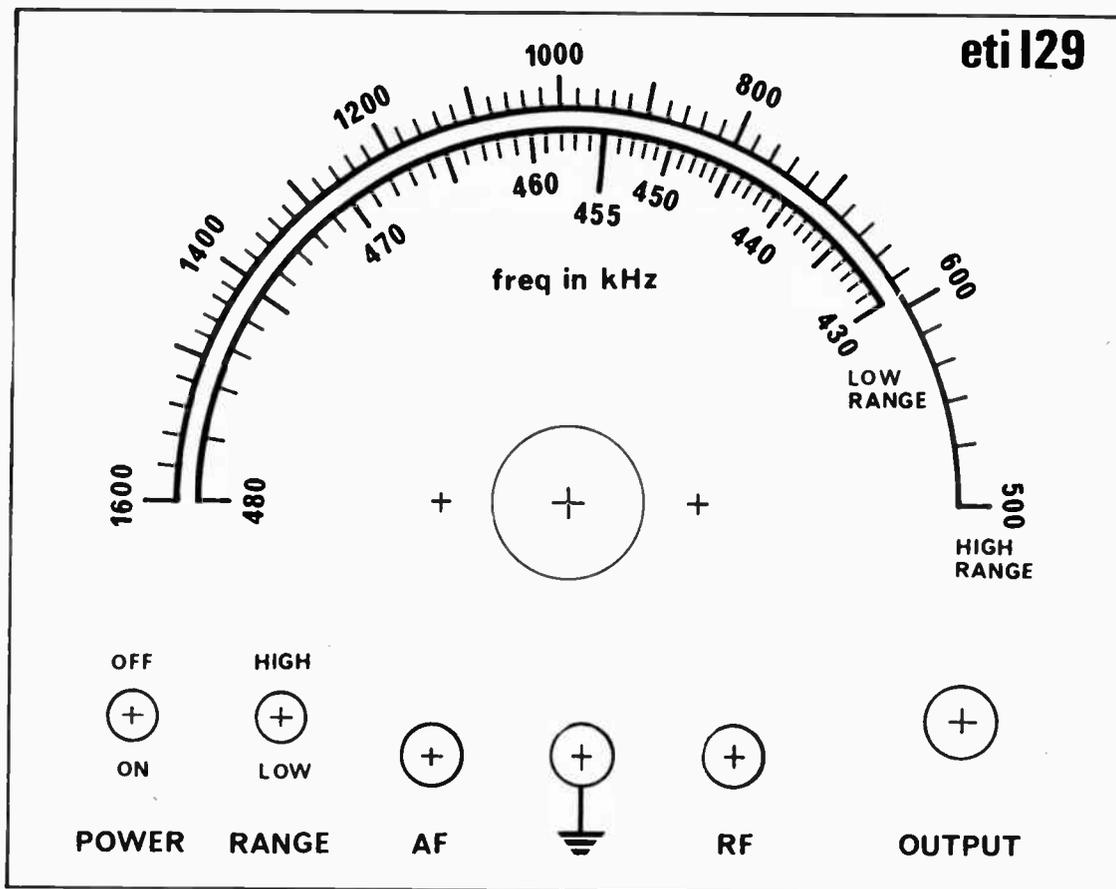
Fig. 4. Front panel artwork. Full size 148 x 116 mm.
