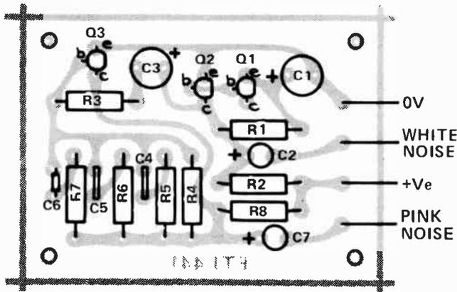
Fig. 2. Component overlay.
