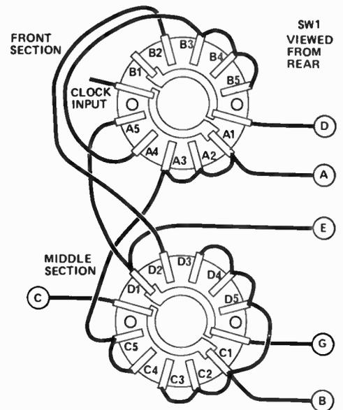
Fig. 3. Wiring of the range switch.
