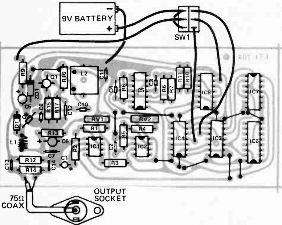
Fig.3. Component overlay.
