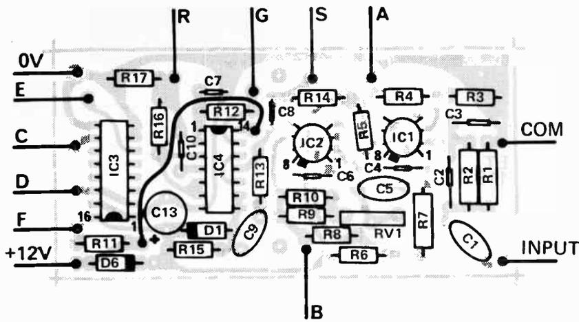
Fig. 2. Component overlay.
