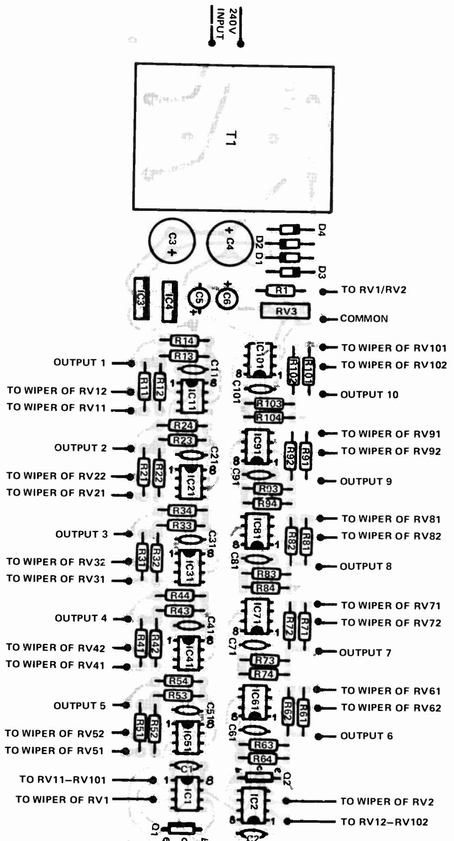
Fig. 2. Component overlay for the controller board, ETI588C.
