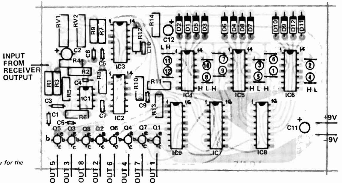
Fig. 7. Component overlay for the decoder.
