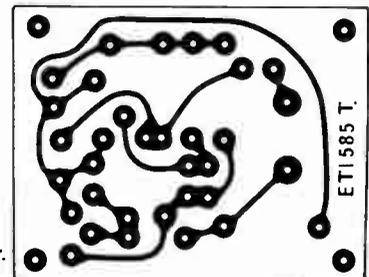
Fig. 7. Printed circuit board of transmitter.
