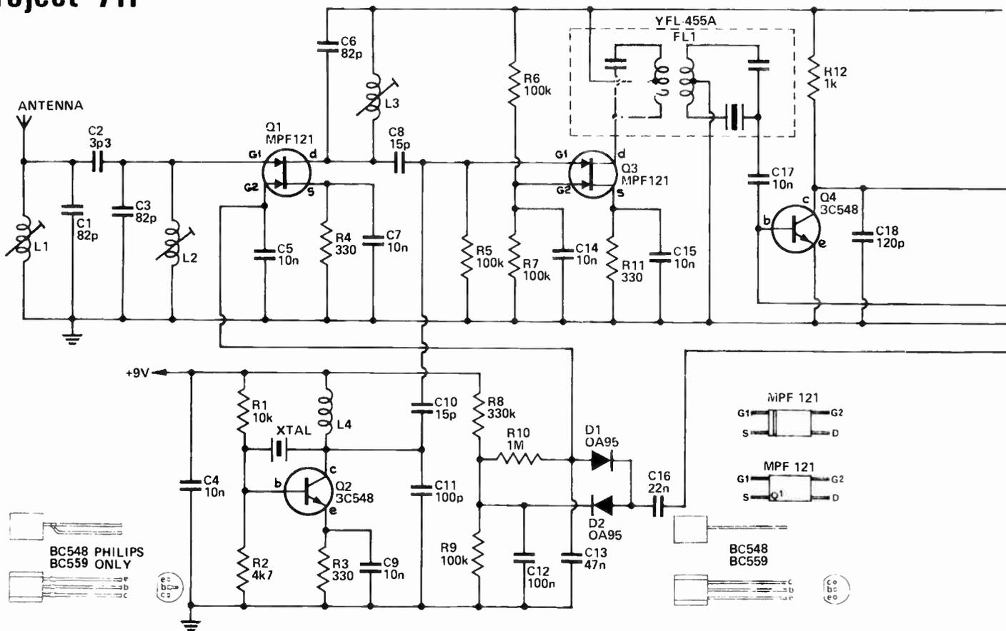
Fig. 3. Circuit diagram of the receiver.
