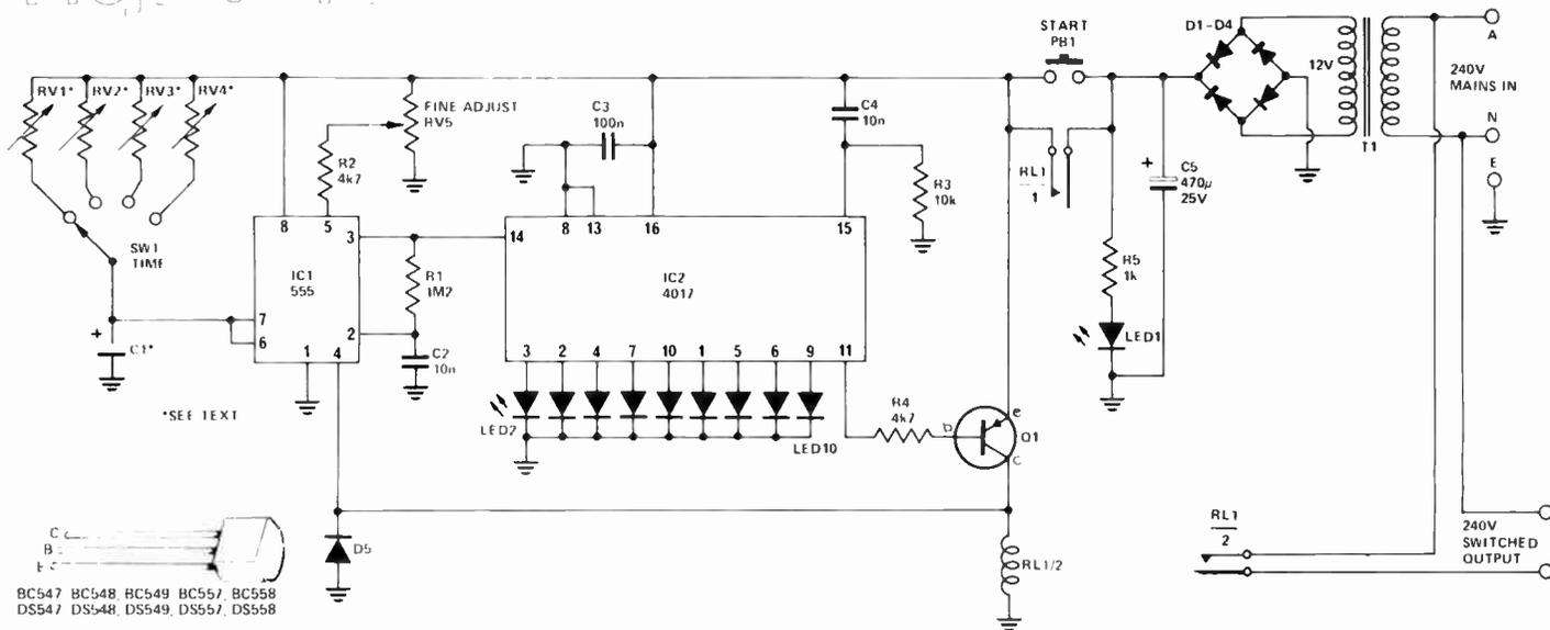
timing period can be increased ten fold. The unused decoded outputs can then be connected to a column of LEDs which will give an indication of elapsed time.
