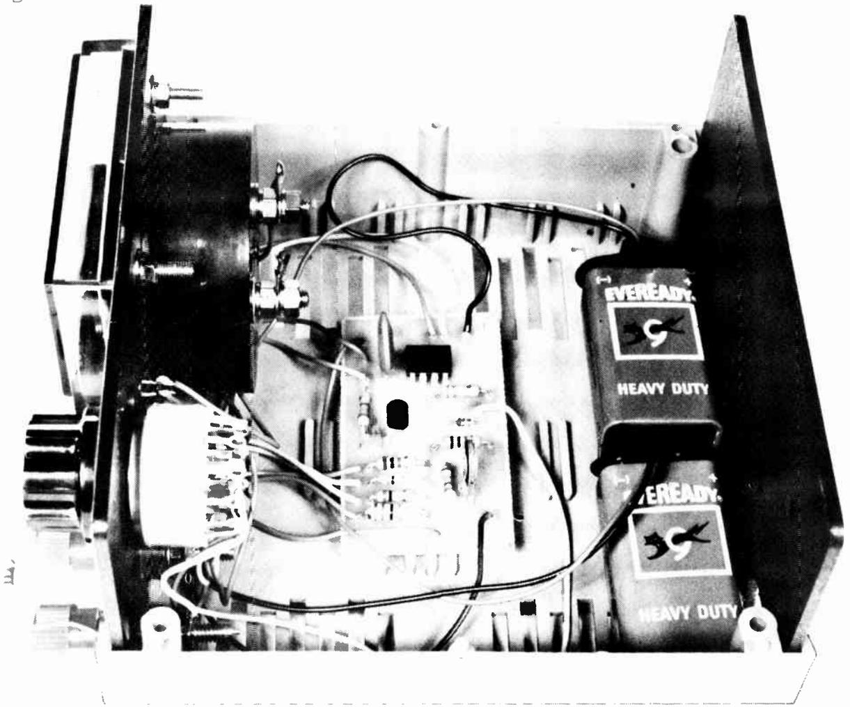
741 as it has been selected for its low input current. The overall accuracy of the instrument is determined by the tolerance of the range resistors (R3 to R6) and the accuracy of the meter. If 1% or 2% resistors are used the accuracy
