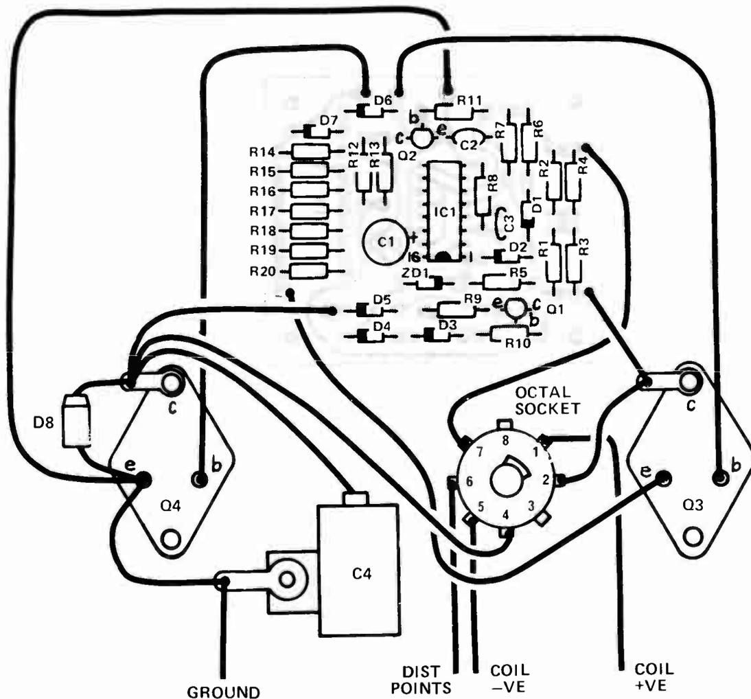
Fig. 2. Overlay and wiring diagram.
