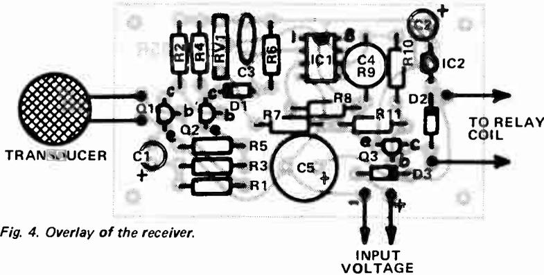
Fig. 4. Overlay of the receiver.
