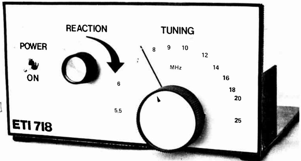
APART FROM THE very early sets, which were based upon coherers and other devices you never hear of today, the first radios were very straightforward designs totally unlike today's sophisticated superhets. The early Tuned Radio Frequency (TRF) sets were simply a tuning circuit with some gain and a detector circuit, but later designs used positive feedback, in the form of reaction, to increase the performance. It is still possible to get a lot of fun from sets of this type.
