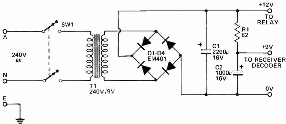
Fig. 3. Circuit diagram of the power supply for the complete receiver decoder. ETI 711P
