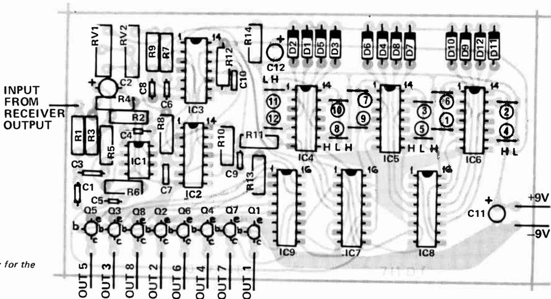
Fig. 7. Component overlay for the decoder.
