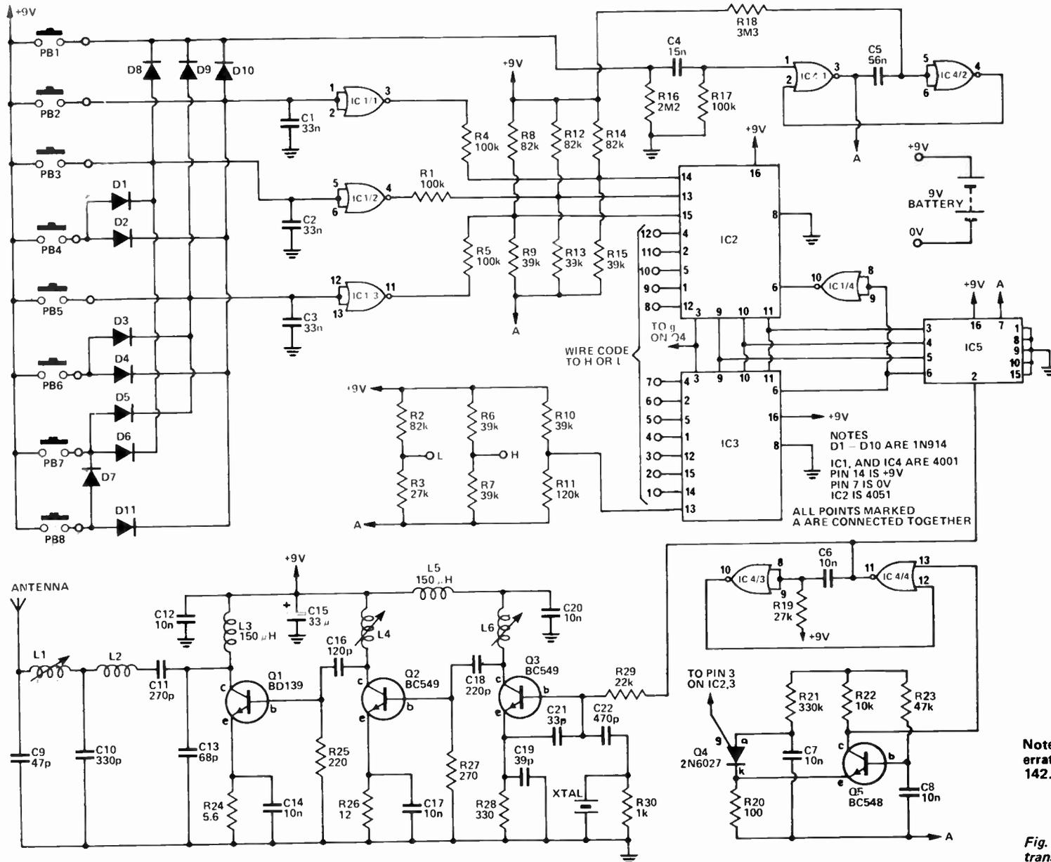
Fig. 1. Circuit diagram of the complete transmitter
