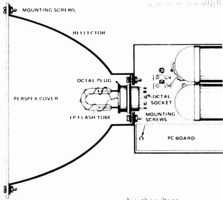
**How the strobe tube works**
