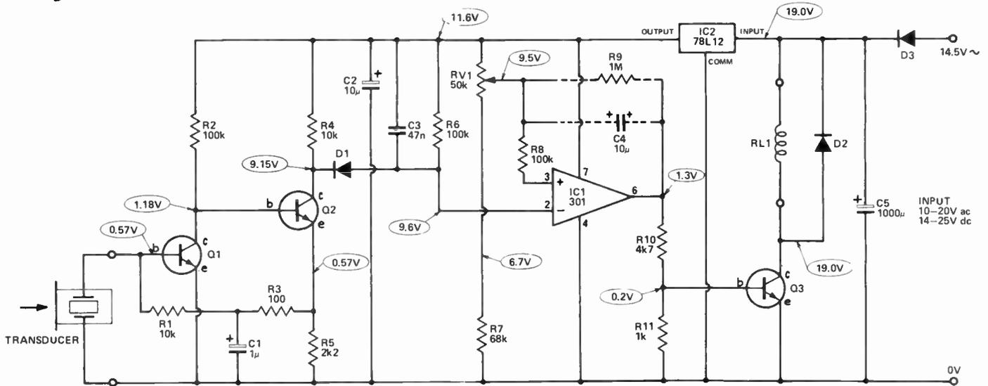
Fig. 1. Circuit diagram of the receiver.
