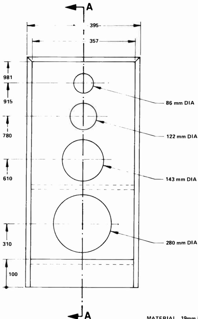
Complete cutting and assembly details for the four-way loudspeaker box. It is important that all joints be well sealed.
