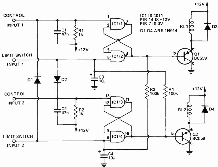
Fig. 2. Circuit diagram of the double-control relay drive circuit. ETI 711C
