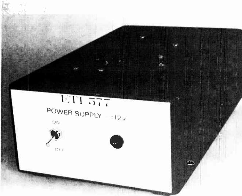
Our prototype was housed in a diecast box to match that used for our Series 4000 moving-coil cartridge preamp, although any suitable box may be used if the power supply is intended for another application. Scotchcal front panels should be available from kit suppliers or separately from Radio Despatch Service in Sydney.
