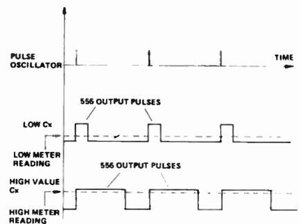
The unknown capacitance,  $C_x$ , determines the width of the output pulses from the 555 monostable. The meter integrates these pulses to produce a reading which is directly proportional to the unknown capacitor's value.
