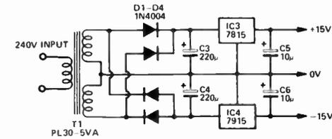
Fig. 5. The circuit diagram of the control desk.
