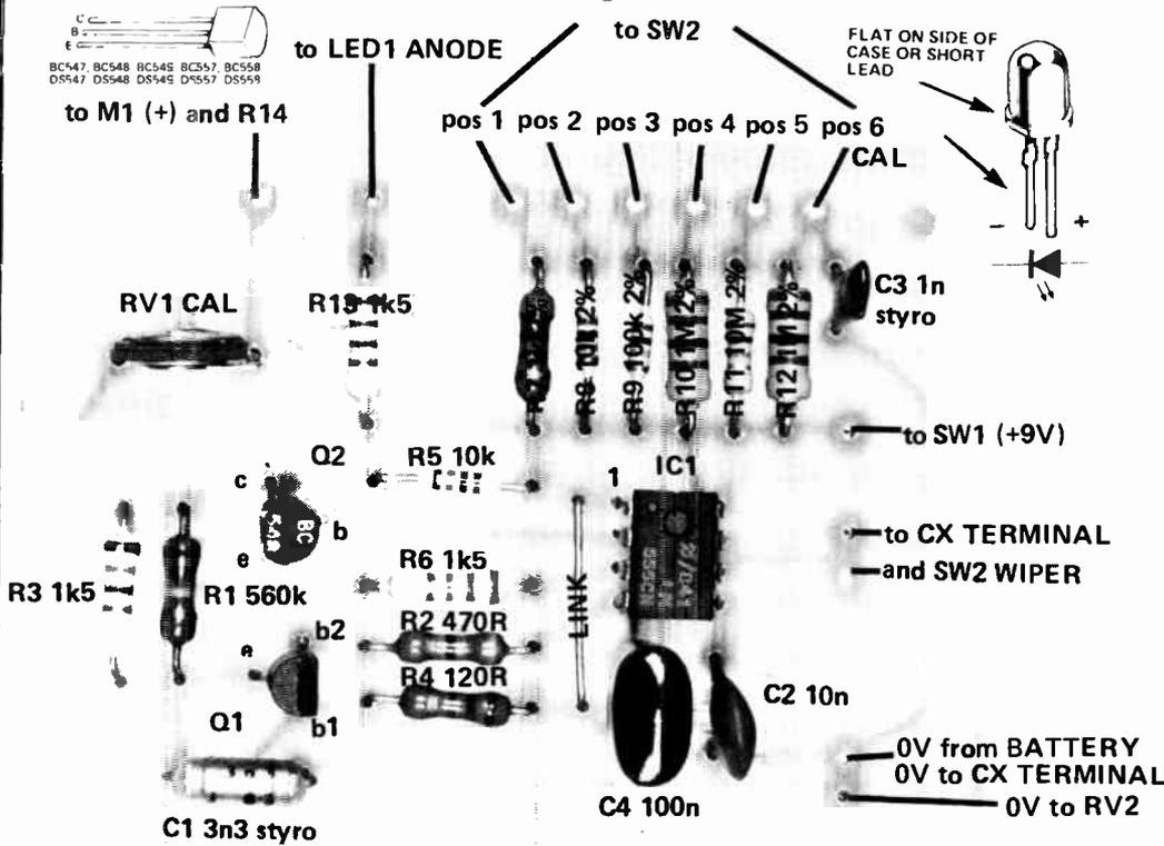
meter will thus be directly proportional to the ratio of the time the output pulse is on to the time it is off, resulting in a linear relationship of capacitance to meter reading. A low value of capacitance connected to the 'CX' terminals will produce a short duration pulse and thus a low meter reading; a high value of capacitance will produce a long duration pulse and a high meter reading, as illustrated on the accompanying diagram.
