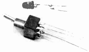
Above: The switches and LEDs have lengths of wire soldered on to them so that they can be inserted into the pcb before being attached to the front panel. They can then be soldered in place. This procedure ensures that there is no strain on the joints. Below: the completed unit. Full details of metalwork will be given in a later article, in which we will describe how to use this preamp with two of the ETI 470 60W units to build a high-performance, low cost stereo amplifier.
