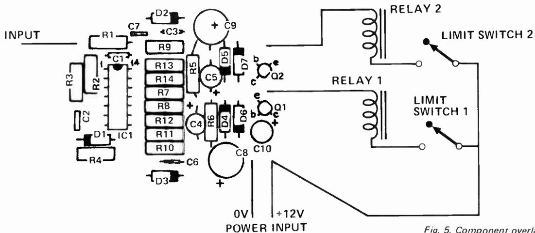
Fig. 5. Component overlay and interconnection diagram for the single-control relay driver. ETI 711B
