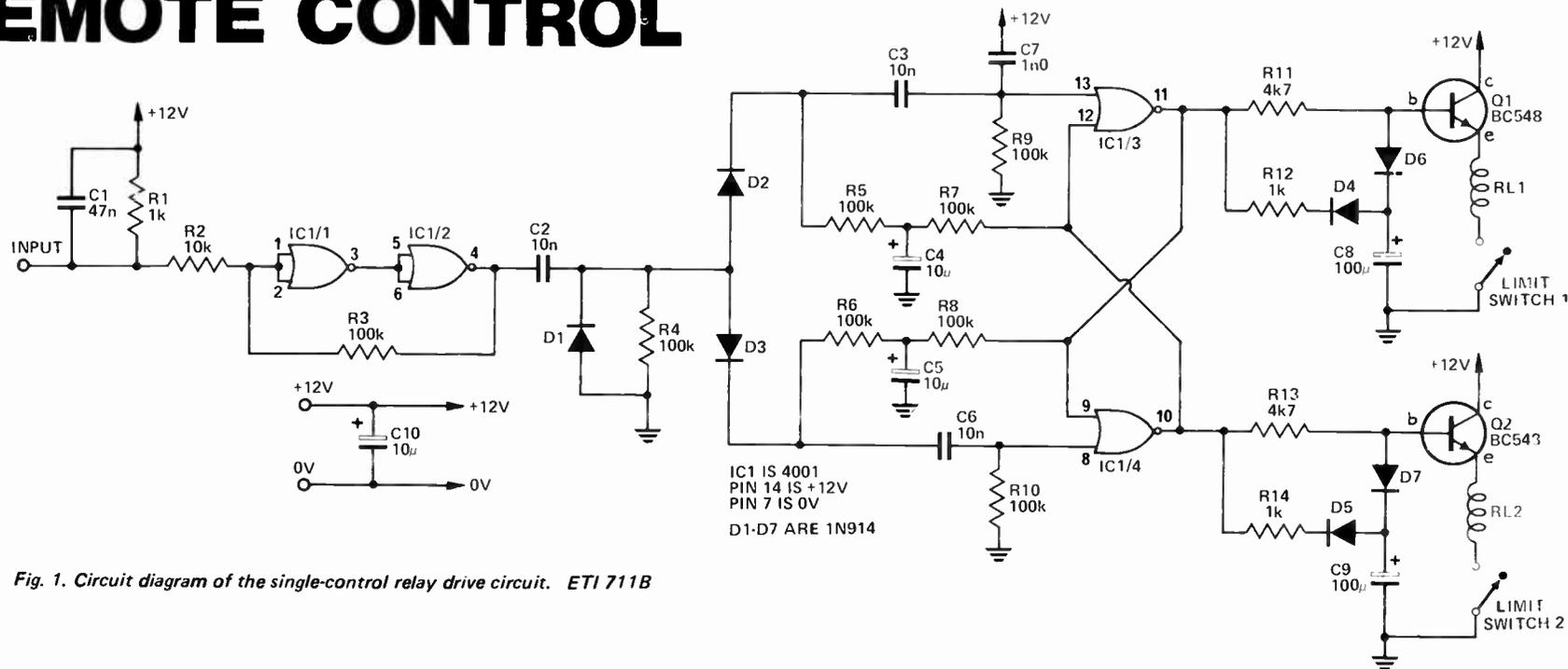
Fig. 1. Circuit diagram of the single-control relay drive circuit. ETI 711B
