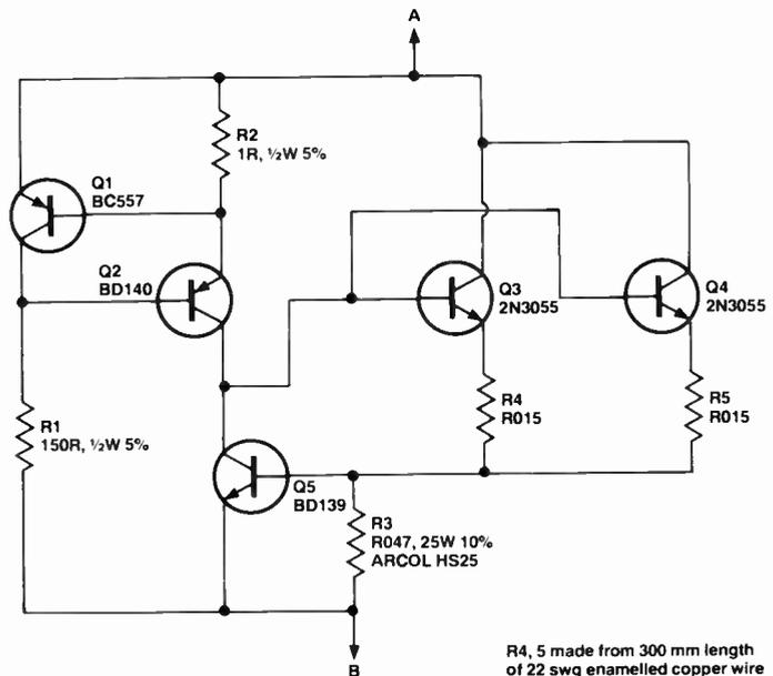
R4, 5 made from 300 mm length of 22 swg enamelled copper wire
