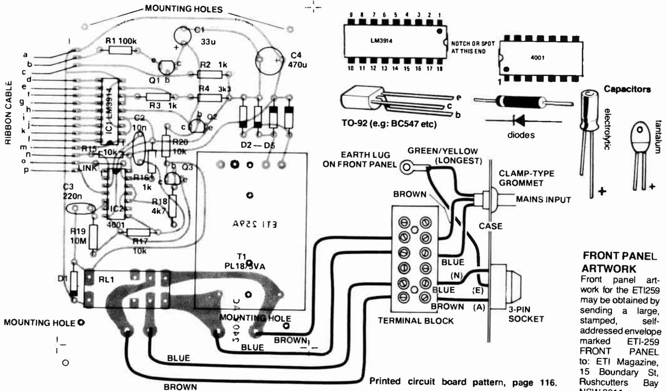
point. Now mount the piezoelectric buzzer and solder its leads in place, as shown on the overlay. Attach knobs to the shafts of SW2 and RV1 last of all.
