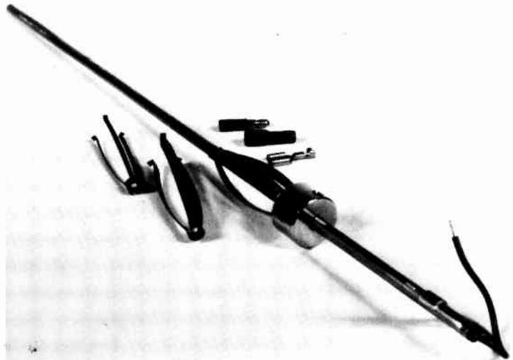
The V.D.O. dipstick probe with its associated parts. Full assembly details are given on page 27.
