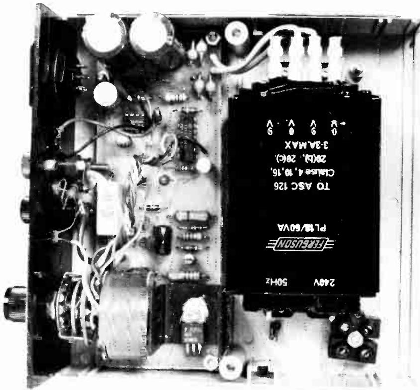
Internal view of the project, showing general placement of components. Mains wiring has been removed for the sake of clarity.
