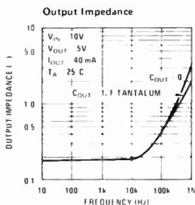
Figure 1. Output impedance characteristic of a three-terminal regulator.
