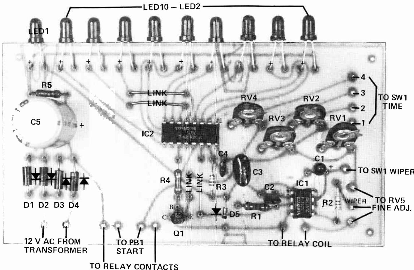
with the timer will determine the type of relay you use. This unit is capable of driving quite large relays, however, we used a commonly available Omron type having contacts rated at 10 amps.
