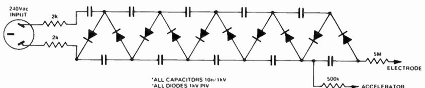
Figure 3. Circuit of a commercial negative ion generator.
