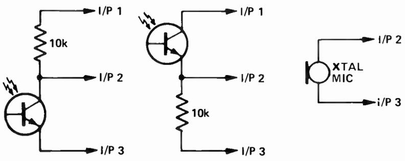
Use phototransistors, type FPT100 or TIL78 or similar
