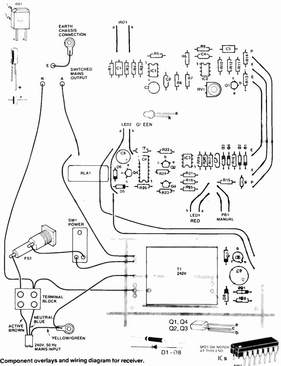
Component overlays and wiring diagram for receiver.
