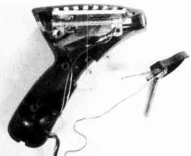
Modified hand controller with connection to both ends of resistance wire.
