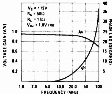
As the device is direct-coupled, dc levels will be maintained between input and output.
