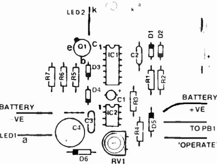
Component overlay for transmitter.
