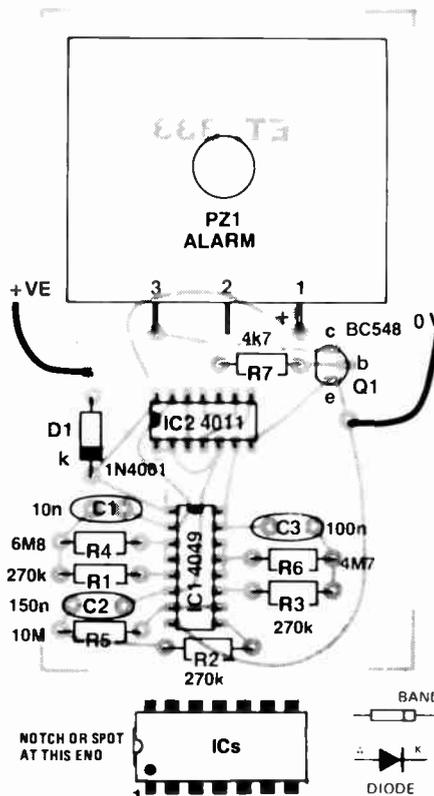
insert the transistor, Q1. Take care to get it the right way round, otherwise the alarm won't work at all and you may destroy the transistor when you first apply power.
