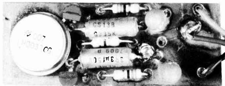
The completed pc board, prior to assembly in the probe housing (pcb pattern is on page 116).
