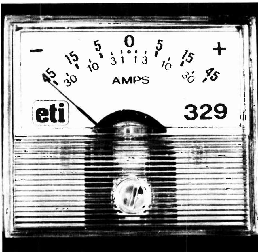
ponents and features a centre-zero scale employing either a centre-zero meter or conventional meter movement. It may be installed in 12 V or 24 V systems and incorporates reverse-polarity protection in case you connect it the wrong way round or try to destroy it by some devious automotive electrical fault. (I recently had the unpleasant experience of momentarily disconnecting a wire on my car which resulted in the *instant obliteration* of every semiconductor in the vehicle.)
