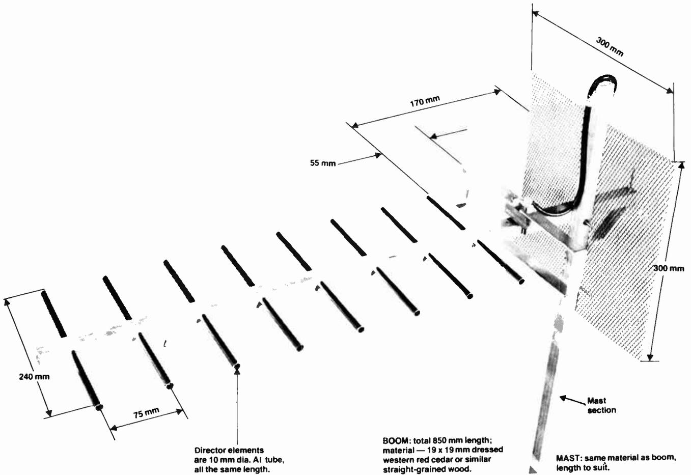
General construction. Note that a metal mast may be used instead of the wooden one.
