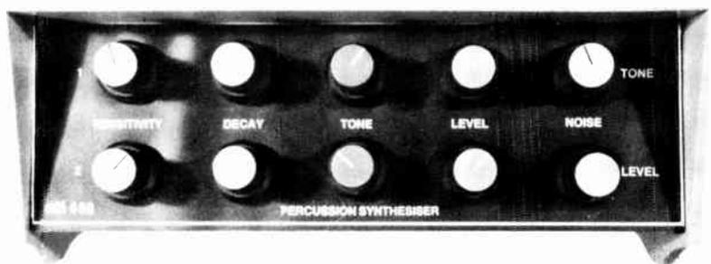
We housed our project in a light but sturdy ABS plastic case and attached a Scotchcal label to the front panel — artwork for this panel and for the pc board is reproduced on page 130. The two 'transducer' inputs, the output and supply input are located on the rear panel. Small speakers serve as input transducers and are mounted in separate small boxes.
