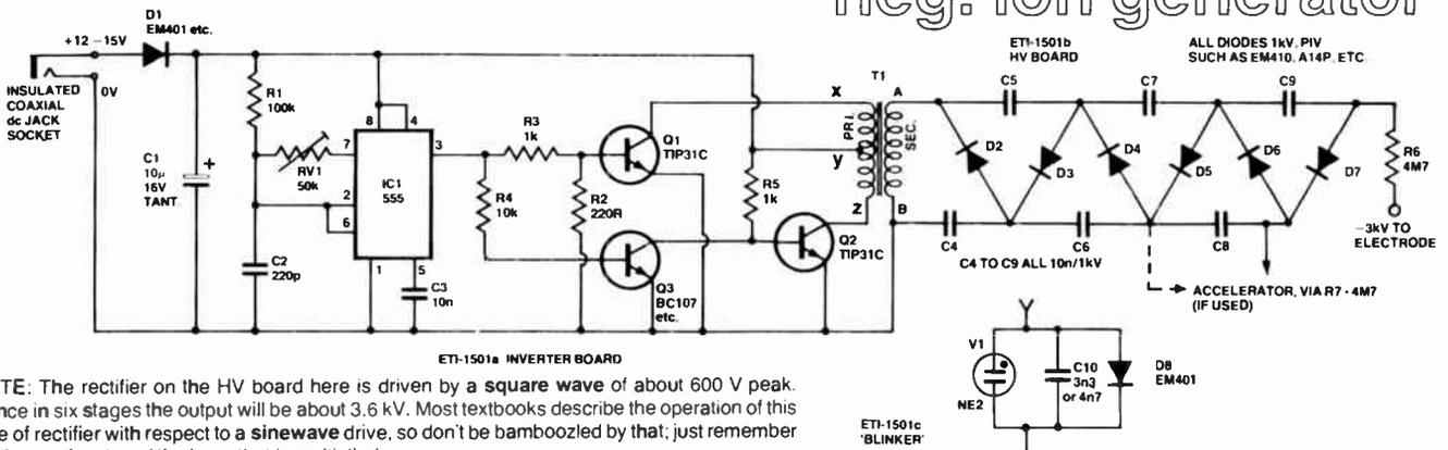
NOTE: The rectifier on the HV board here is driven by a square wave of about 600 V peak. Hence in six stages the output will be about 3.6 kV. Most textbooks describe the operation of this type of rectifier with respect to a sine wave drive, so don't be bamboozled by that; just remember it's the peak value of the input that is multiplied.
