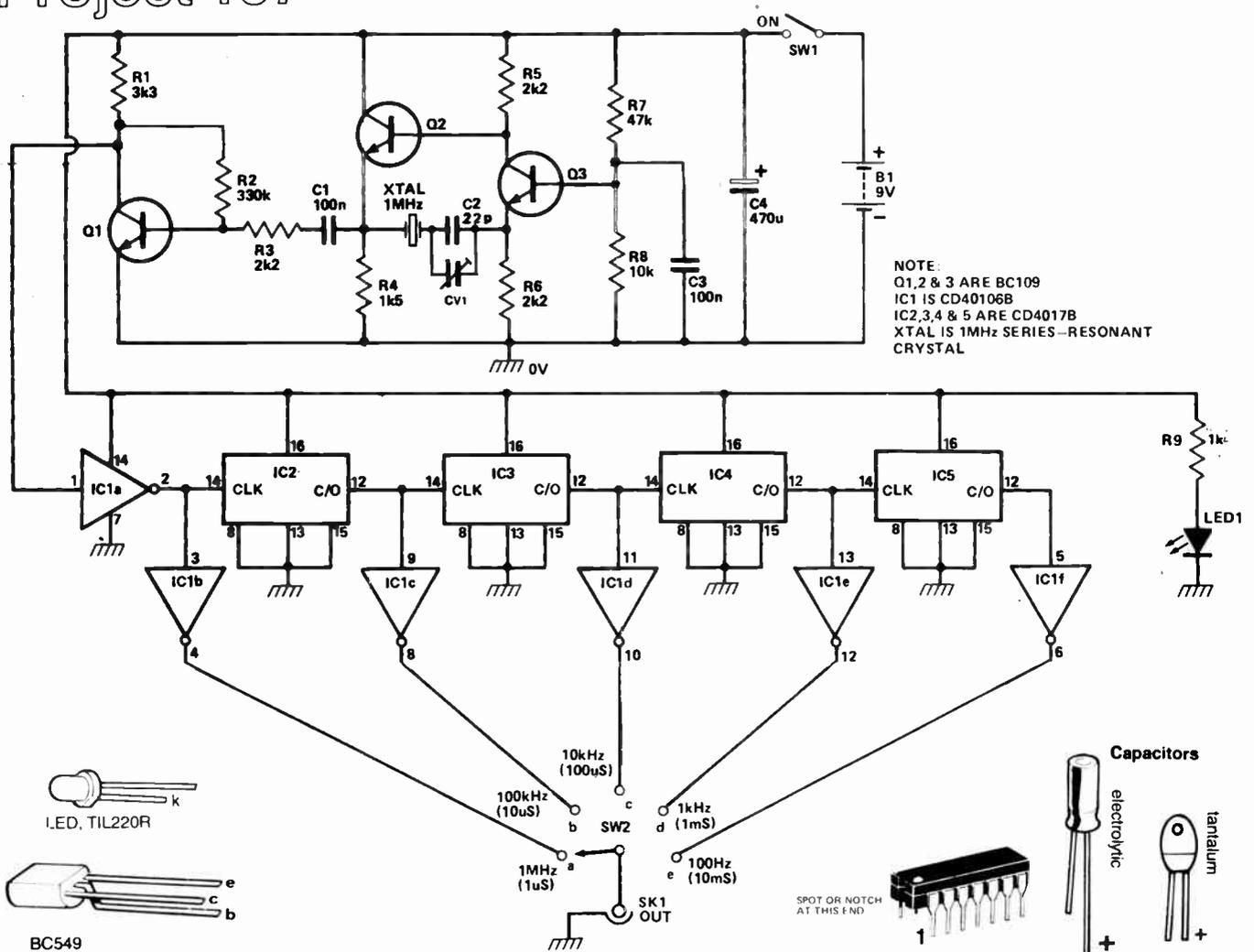
4017s). The first Schmitt inverter provides 1 MHz output, which is buffered by another Schmitt inverter to provide the 1 MHz output to the output selector switch. The output of each decade divider stage is also buffered by a Schmitt inverter to provide, respectively, the 100 kHz, 10 kHz, 1 kHz and 100 Hz outputs to SW2.
