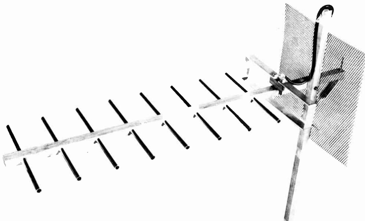
To make this antenna you'll need two metres of 10 mm dia. aluminium tube, one metre of 25 x 3 mm aluminium strip, a 300 mm square of Multimesh, one metre or more of 19 x 19 mm dressed western red cedar, plus some nuts and bolts. We bought the lot for about \$7!
