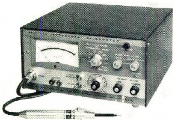
Fig. 3. Sensitive gaussmeter by Bell measures small fields.
