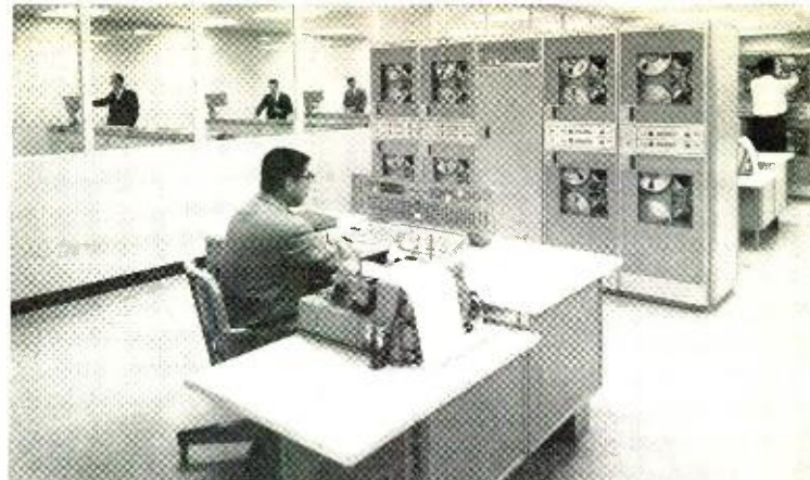
The computer control console (foreground) and the memory tape storage units that are utilized in the ERMA system discussed.
