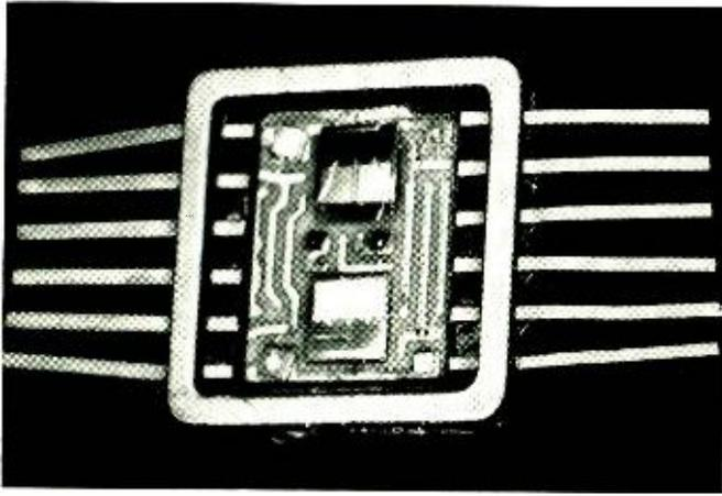
Fig. 9. Typical example of a hybrid circuit made by General Instrument Corp. Eight separate chips are used on this unit.
