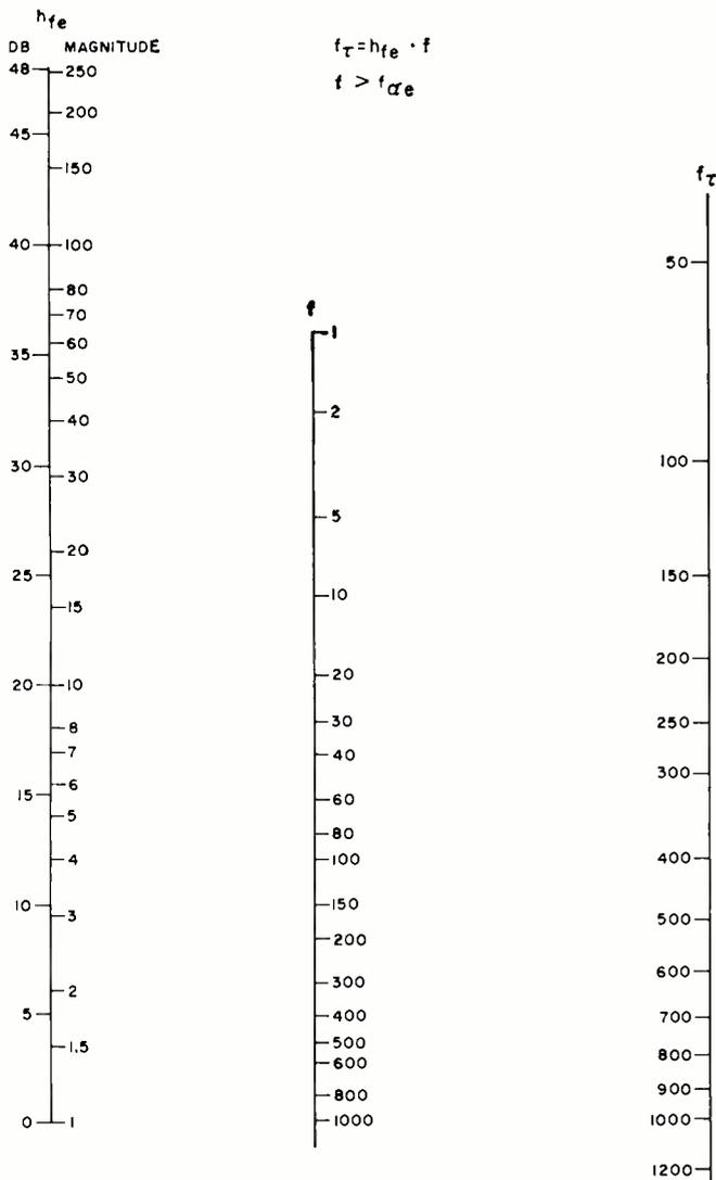
Fig. 5. Nomogram shows the relationship between gain-bandwidth product ( $f_{\tau}$ ) value of  $h_{fe}$  at 1 kc. in db or magnitude, and common-emitter, current-gain cut-off frequency ( $f_{\alpha e}$ ).
