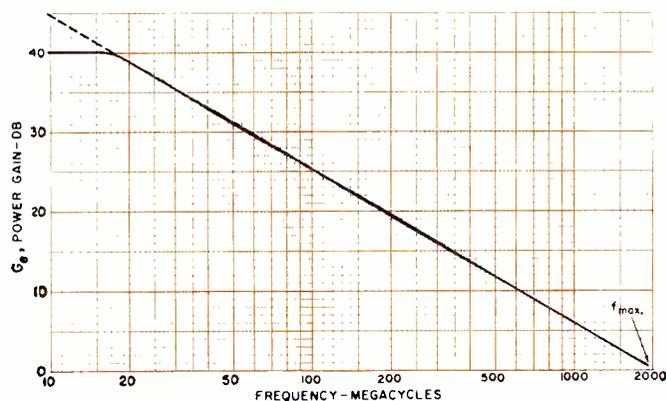
Fig. 2. Power gain vs frequency for a particular transistor.
