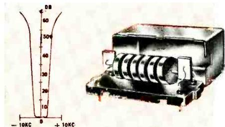
With CB channels only 10 Kc apart, selectivity is important! In the HB-500, ultra-sharp selectivity is achieved by means of a true mechanical bandpass filter in the 455 Kc IF section. At 10 Kc on either side of the center frequency, the filter provides 60 db of attenuation — an extremely high rejection ratio that assures complete adjacent channel rejection!
