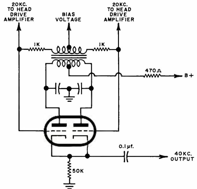
Fig. 6. Push-pull oscillator has unbypassed cathode which "follows" most positive grid, thereby acting as a doubler.
