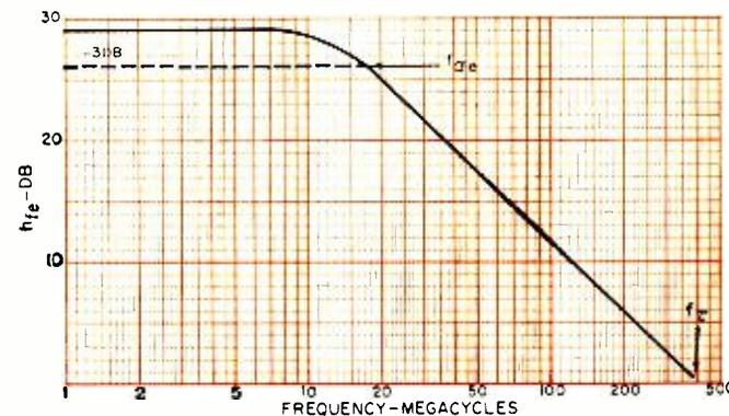
Fig. 3. Current gain vs frequency for a typical transistor.
