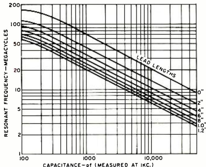
Fig. 5. Resonant frequency of some typical capacitors as a function of their lead length (22-gauge wire is assumed).
