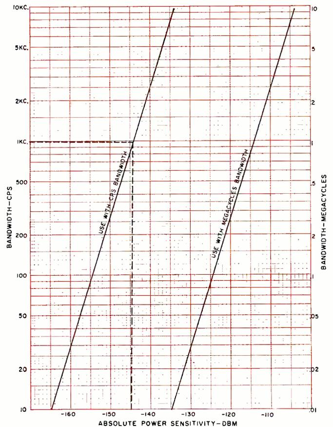
Fig. 1. Absolute power sensitivity of perfect amplifier for various amounts of bandwidth at about room temperature (300°K).
