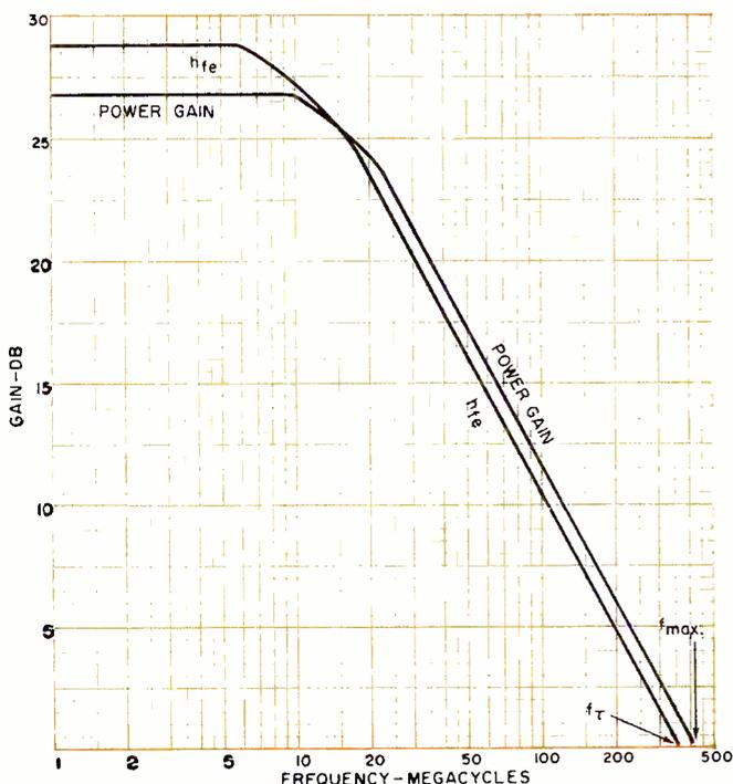
of the three common transistor high-frequency response parameters, let's examine the interrelationship among them and methods of converting from one specification to another.
