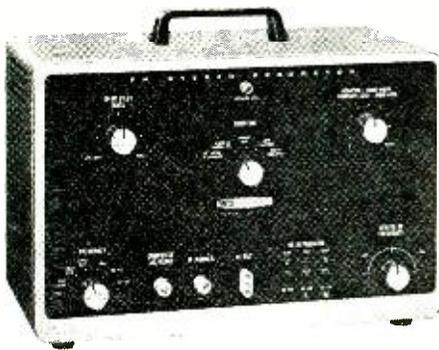
( $\pm 2$  cps) pilot signal, adjustable in level from to 10%, is provided to check the lock-in range of stereo receivers.
