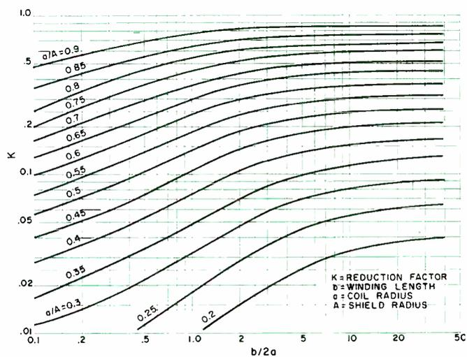
Fig. 2. Curves for determination of decrease in inductance produced by coil shield.  $K \times 100\%$  is amount of inductance reduction. For a square shield, A is .6 of the length of one side. Coil must be single layer for this graph to apply.
