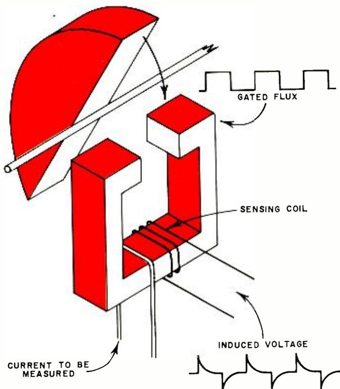
Fig. 1. Magnetic flux being gated by spinning "shutter."
