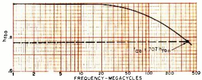
Fig. 4. Common-base current gain for a typical transistor.
