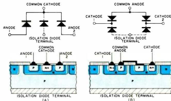
Fig. 6. (A) Construction of a common-cathode pair of diodes. (B) Construction of a pair of diodes having a common anode.
