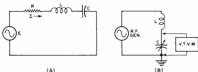
Fig. 2. (A) Amount of series resistance determines "Q" of series-resonant circuit. (B) Basic circuit of "Q" meter.
