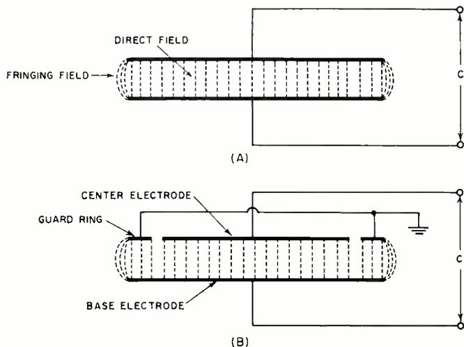
Fig. 2. (A) Effect of fringing lines of force on parallel-plate capacitor electrodes. (B) Guard ring reduces fringing.
