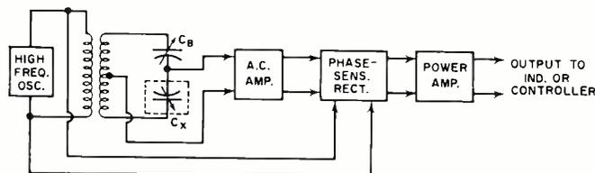
Fig. 4. This high-frequency, bridge-type transducer circuit is commonly used with some types of capacitive instrumentation.
