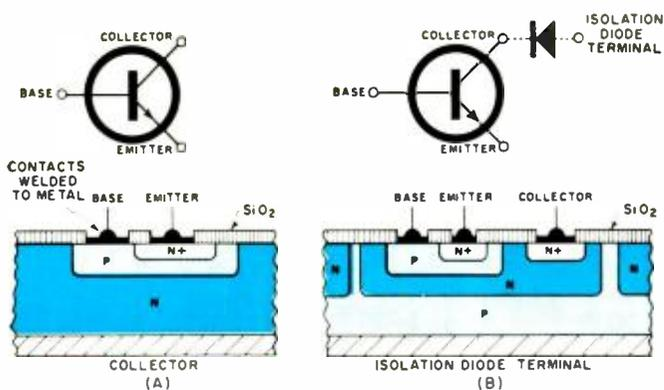
Fig. 5. (A) Construction of a conventional planar transistor. (B) Construction of an integrated circuit planar transistor.
