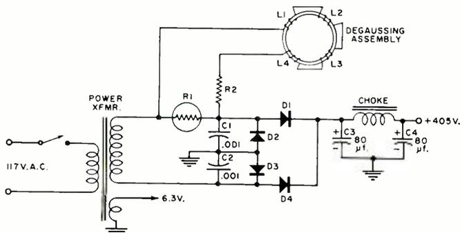
Fig. 2. Current through degaussing coils depends on warm-up resistance of thermistor  $R1$  and voltage-dependent resistor  $R2$ .
