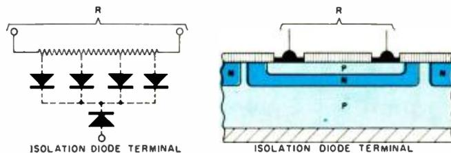
Fig. 7. How a monolithic circuit diffused resistor is made.
