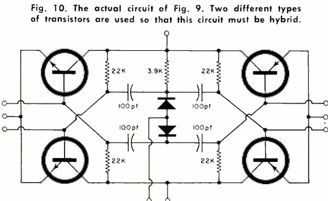
Fig. 10. The actual circuit of Fig. 9. Two different types of transistors are used so that this circuit must be hybrid.
