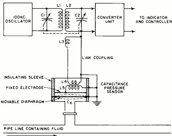
Fig. 5. This capacitance-type liquid pressure transducer is designed to operate with frequency-modulated carrier system.
