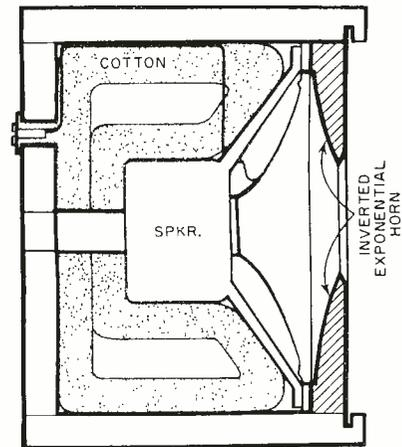
at 75 cps, and more rapidly to 15% at 50 cps. However, the output falls off rapidly below 90 cps, so that there is no boominess or muddiness from frequency components too low for the speaker to reproduce. Its output is clean throughout its useful range and drops to inaudible levels at lower frequencies.
