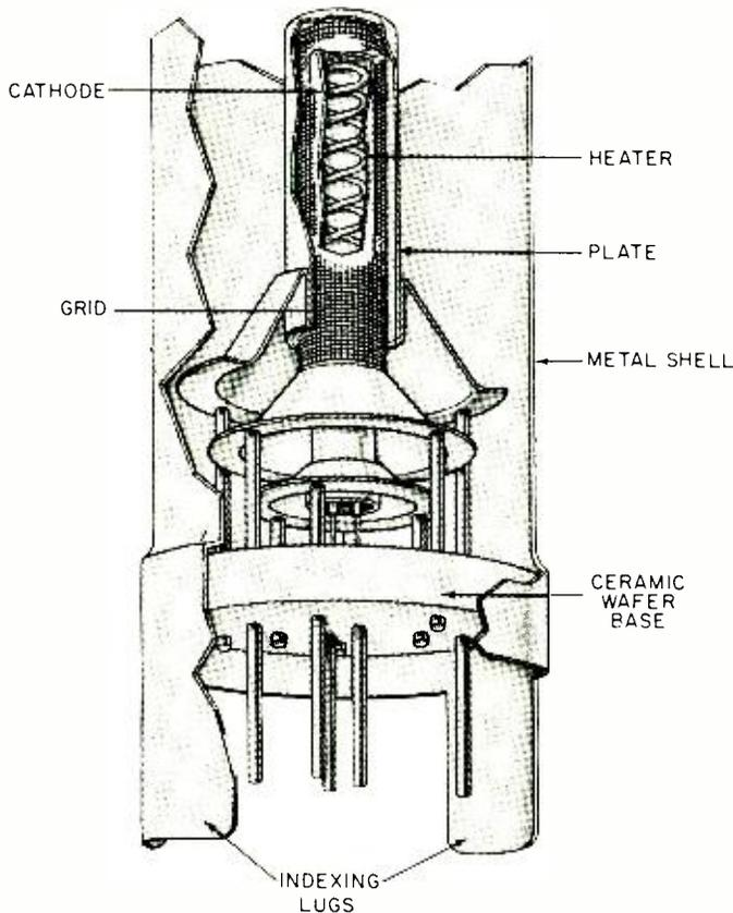
Fig. 1. Cutaway view of a typical nuvistor miniature tube.
