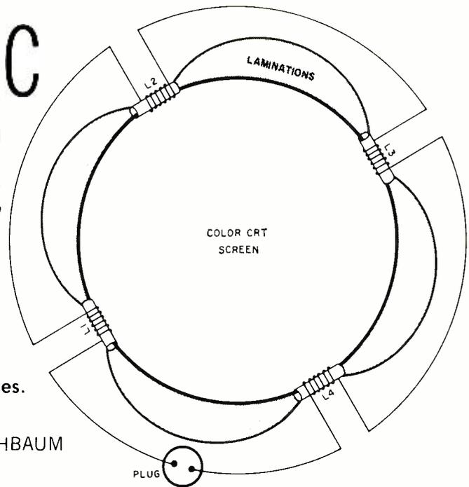
Fig. 1. The steel-laminated ring with associated coil mounts around the color tube to act as a permanent degaussing coil.
