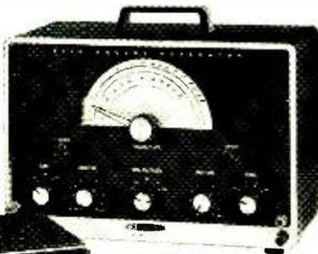
**Professional Sine-Square Wave Generator IG-82 . . . \$51.95**—Ideal for any application in service and general laboratory work. Less than .25% sine wave distortion. Less than .15 microsecond square wave rise time. Sine & square wave output available simultaneously. Covers 20 cps to 1 mc in 5 bands. Features exact frequency calibrating system for proper dial tracking. 13 lbs.
