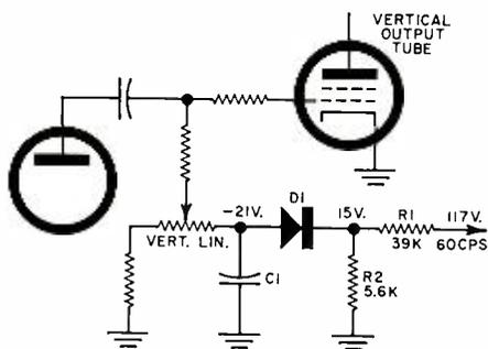
from the diode is filtered by *C1*, and applied to the vertical output tube control grid through the linearity control and its associated resistors.
