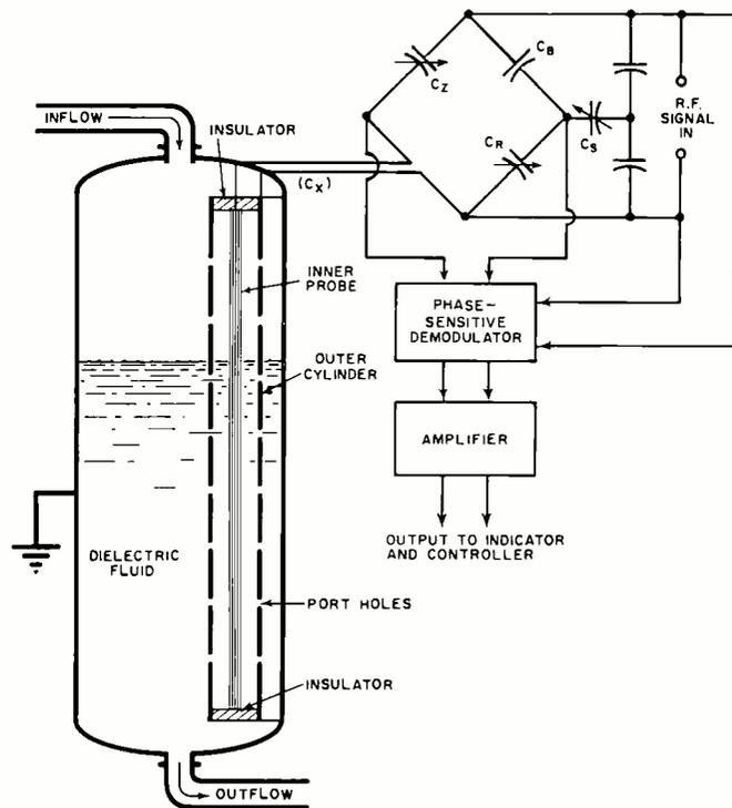
Fig. 6. Capacitance transducer system used as level measurement for tanks of various types of nonconducting liquids.
