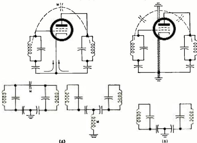
(and hence degree of magnetic and electrostatic coupling to the shield), resistivity of the shield material, and the relationship between shield length and diameter, coil length and diameter, and the relationship between coil and shield. The effect is that of adding a resistance in series with the coil and its resistance, and since "Q" is a ratio of  $X_L/R$ , "Q" is reduced as  $R$  is increased.
