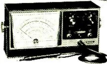
**Deluxe "Service Bench" Vacuum Tube Voltmeter IM-13 . . . \$32.95**—Measures AC volts (RMS), DC volts, resistance & db. Separate 1.5 & 5 volt AC scales for high accuracy; "gimbal" mounting bracket for easy bench, shelf or wall mounting; meter tilts to any angle for best viewing; smooth vernier action zero & ohms adjust controls; large, easy-to-read 6" 200 UA meter; and single AC/Ohms/DC test probe. 7 lbs. Assembled IMW-13 . . . \$49.95.
