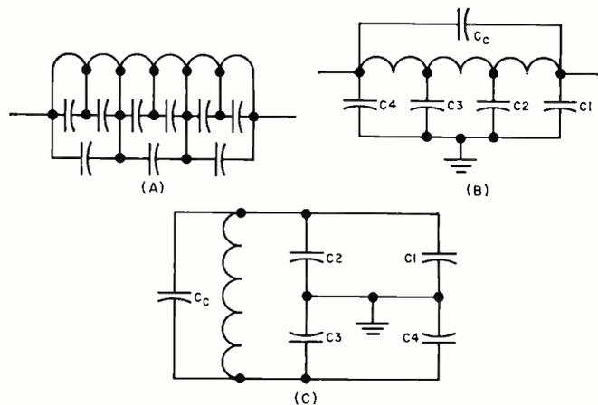
Fig. 4. (A) Capacitance between individual turns of a coil. (B) Effect of capacitance between coil and ground (C1 and C4 are bypass capacitors). (C) Equivalent circuit of (B) showing effect of capacitors on the resonant frequency of the coil.
