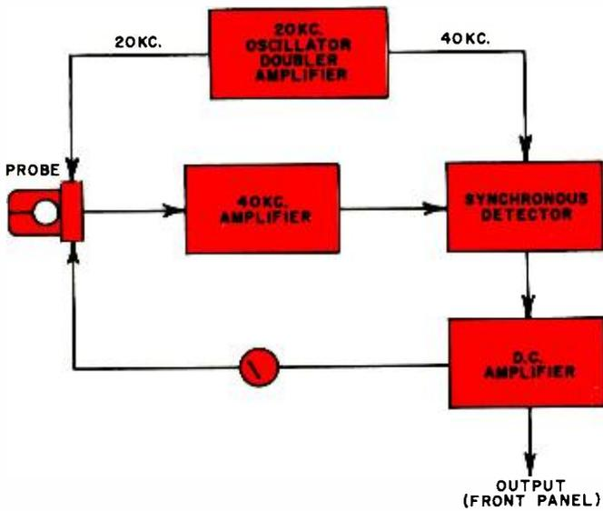
Fig. 3. Simplified block diagram of d.c. current probe circuits.
