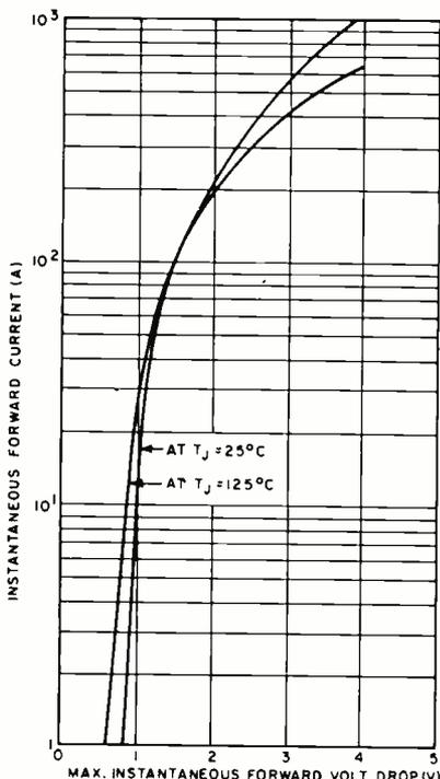
Fig. 1. Forward voltage drops for various currents for two junction temperatures, +25 and +125°C.
