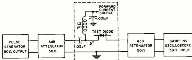
Fig. 2. Test circuit used to measure reverse recovery time.
