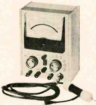
THE industry's first broadband FET voltmeter is the Model SSVM-1 by Data Instruments. The new device has extremely high input impedance and can make measurements over a very wide frequency range. Input impedance on d.c. is greater than 100 megohms, and on a.c. it is about 15 megohms shunted by 2 pF.
