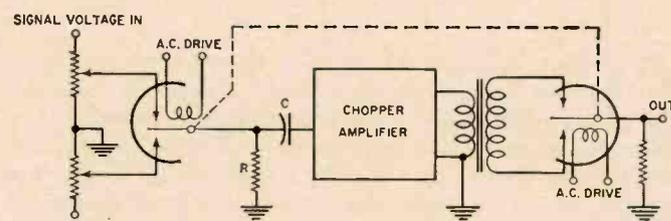
Fig. 9. Comparison circuit measures difference in d.c. values.
