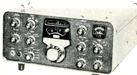
operation, a "Switch-Board" coil and band-switch assembly, and a new automatic level control circuit for wide variation in speech level.
