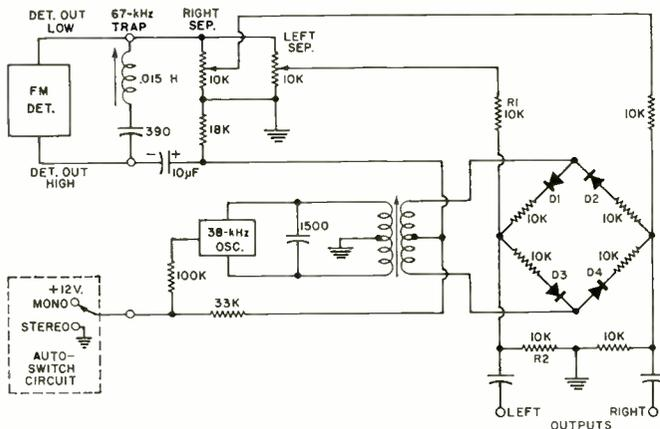
Fig. 1. Simplified circuit of the multiplex demodulator.
