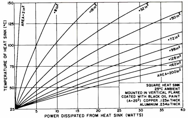
Fig. 3. Power-dissipation characteristics of square heat sinks.
