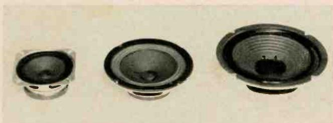
Typical 4", 6", and 8" high-compliance speakers are shown. The free-air resonances are 60, 50, and 30 Hz, respectively. Speakers of this type are characterized by heavy magnets, very flexible cone surrounds, long-throw voice coils, and low cone resonance. Such speakers are readily available from most speaker manufacturers and as private-label brands from some of the larger electronics parts dealers. Speaker sizes range from approximately 4" all the way up to 15".
