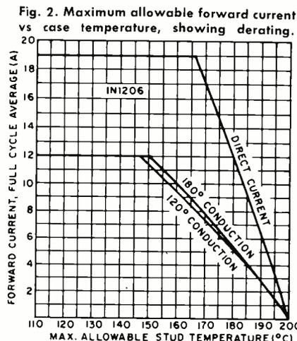
Fig. 2. Maximum allowable forward current vs case temperature, showing derating.
