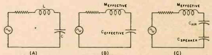
Fig. 1. (A) A series-resonant electrical circuit. (B) A simplified electro-mechanical equivalent circuit for loudspeaker in free air. (C) Simplified equivalent circuit of speaker in sealed box.
