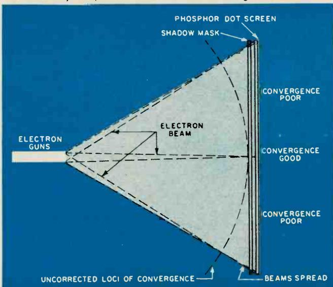
coincidence of the three electron beams near the center of the picture-tube active-screen area. This static convergence is achieved by adjusting the fields of three permanent magnets, each controlling one electron beam as illustrated in Fig. 1. The final convergence of the three beams, however, requires a fourth motion, and this is produced by the blue lateral magnet which permits static adjustment of the blue beam in the horizontal direction. This allows all three beams to converge exactly.
