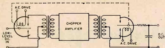
Fig. 7. Amplifier with d.p.d.t. chopper for full-wave demodulation.
