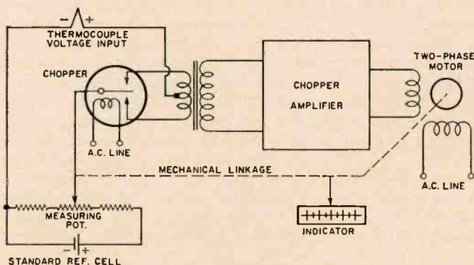
Fig. 10. Electronic null-balance temperature recorder circuit.
