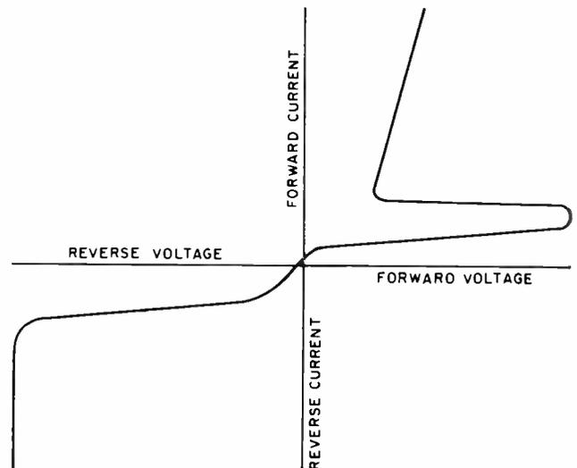
Fig. 5. Typical four-layer diode characteristics are shown.
