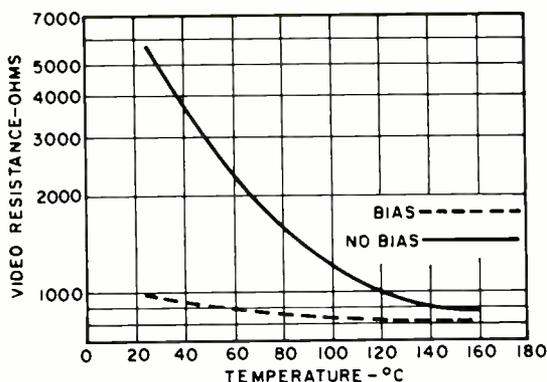
Fig. 4. High-temperature characteristics of 1N630 diodes.
