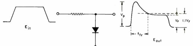
Fig. 4. Switching diode forward transient characteristics.
