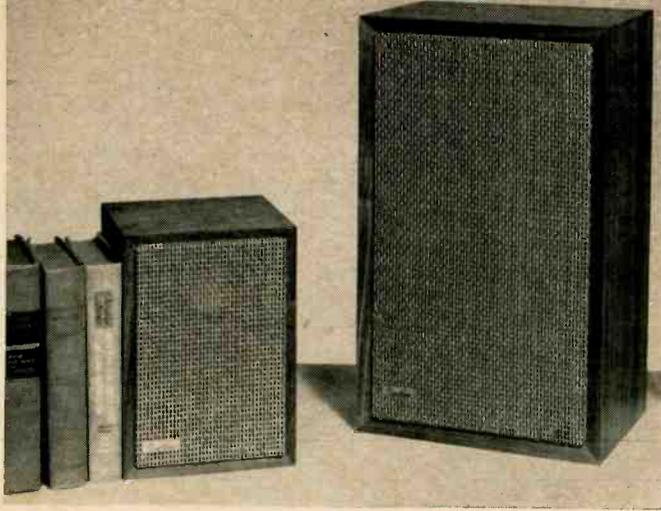
Finished speaker systems using high-compliance drivers and completely sealed enclosures are quite compact. The smaller unit shown measures only 10 1/2" x 7 1/2" x 7" and includes a 4" woofer and 2" tweeter. The larger unit measures 19" x 11 1/2" x 8 1/2" and includes an 8" woofer along with a 3 1/2" tweeter.
