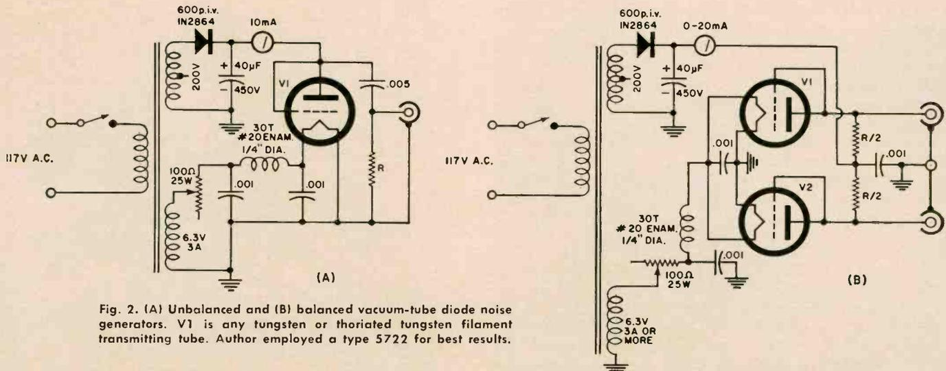
Fig. 2. (A) Unbalanced and (B) balanced vacuum-tube diode noise generators. V1 is any tungsten or thoriated tungsten filament transmitting tube. Author employed a type 5722 for best results.
