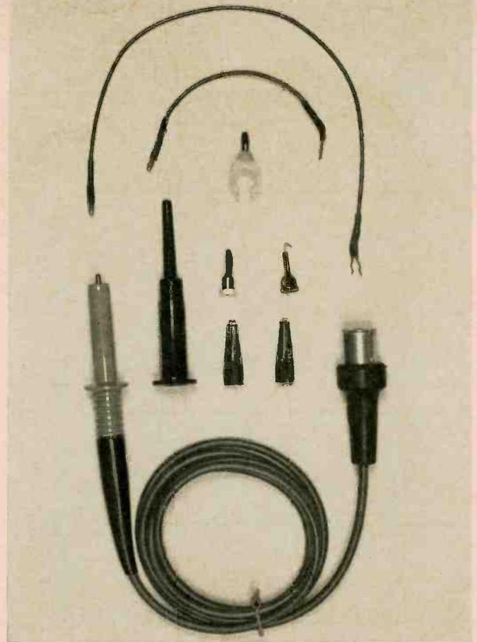
Fig. 2. Some probes come with a variety of interchangeable tips.
