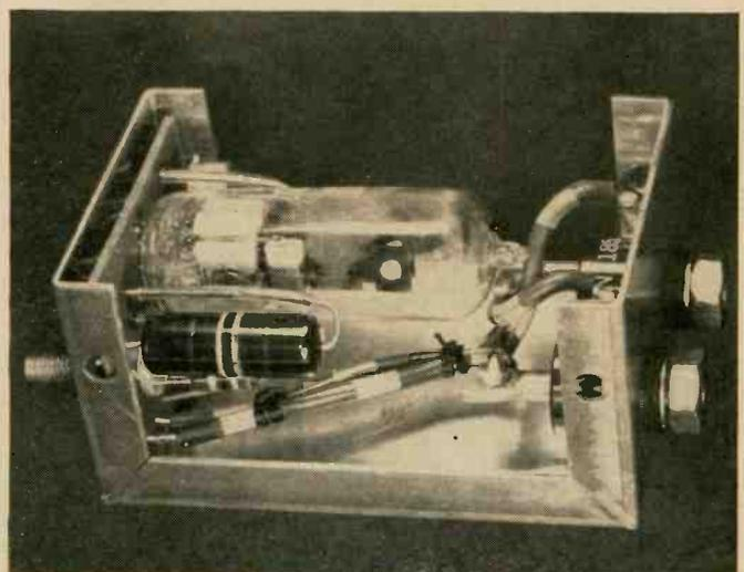
Connect the battery side of the circuit to the "B" terminal and the ammeter side of the circuit to the "A" terminal. If there is any doubt that you have found the right conductor, turn on a light (the door or dome light will do), then break or open the circuit. The light should extinguish.
