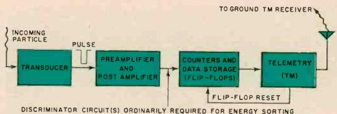
Fig. 3. Signal flow of typical radiation-measuring experiment.
