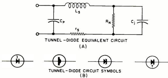
Fig. 2. Tunnel-diode equivalent circuit and circuit symbols.
