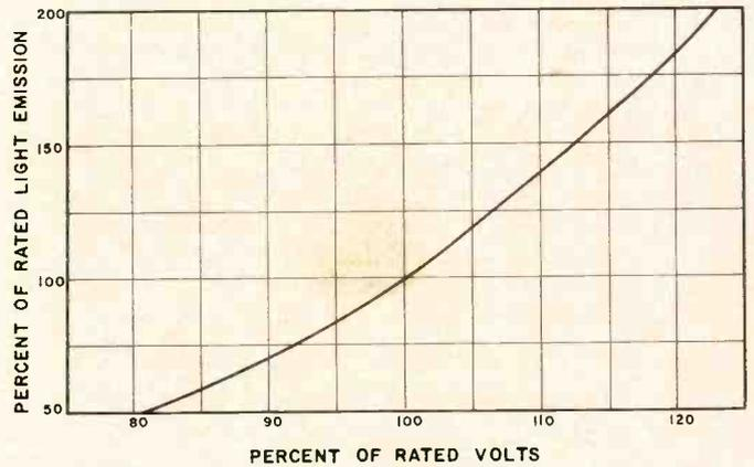
Fig. 2. Variations in light output for various voltages.
