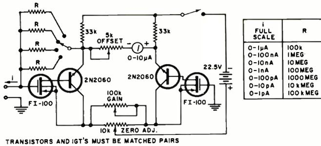
Fig. 4. Circuit of extremely sensitive d.c. picoammeter.
