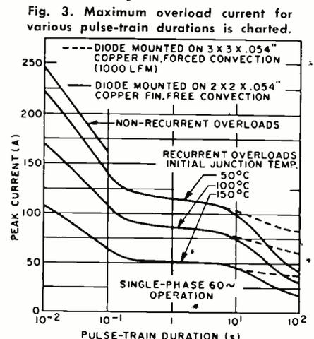
Fig. 3. Maximum overload current for various pulse-train durations is charted.
