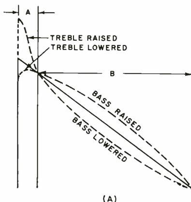
Fig. 2. (A) Effects of varying the bass and treble frequency controls. Crossover point is usually about 1000 Hz. (B) Clipped saw-tooth due to amplifier overload is easily recognized using a saw-tooth. (C) Ringing is caused by amplifier instability.
