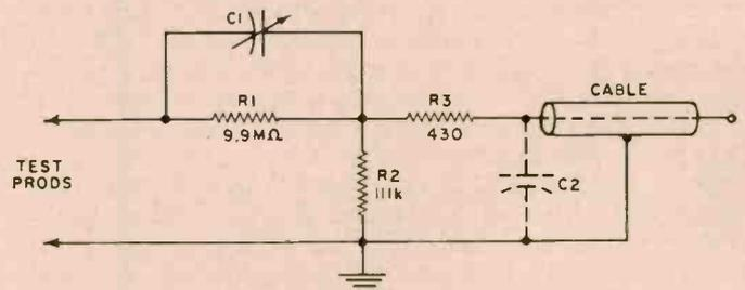
Fig. 3. A typical  $100\times$  attenuator probe uses a small variable capacitor to compensate for coaxial cable capacitance present.
