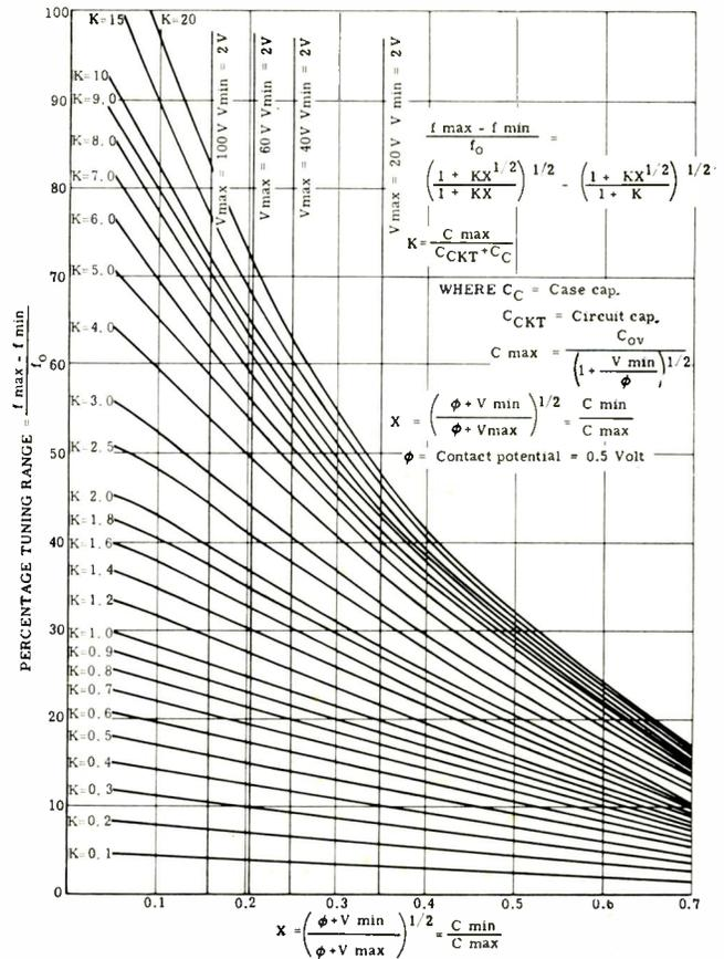
Fig. 2. Percentage resonant circuit tuning range.
