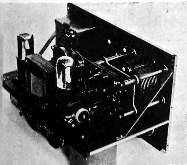
Interior of generator, using switching scheme of Fig. 3
