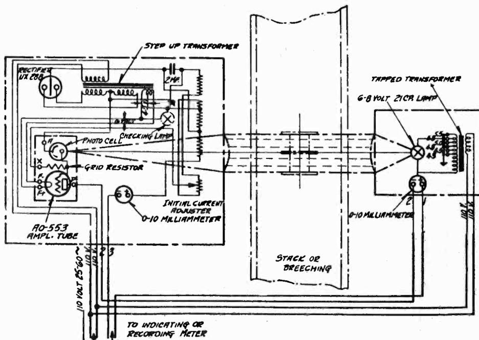
This sketch shows the operating parts of a standard electric smoke indicator as installed in a number of plant smoke-stacks by engineers of the Westinghouse company. A beam of light is projected across the smoke passage, and onto a photo-cell
