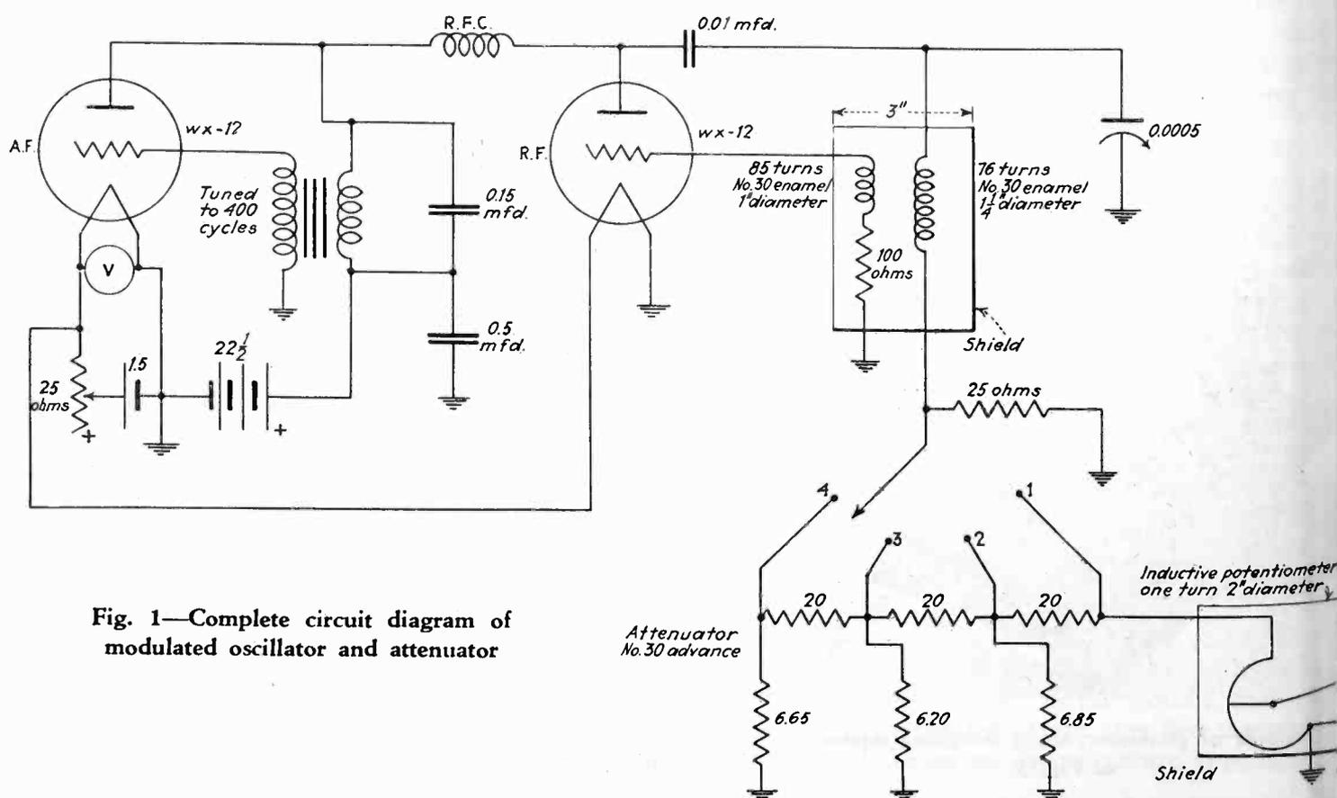
Fig. 1—Complete circuit diagram of modulated oscillator and attenuator
