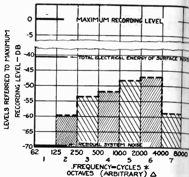
Fig. 3—Electrical energy analysis of disc surface noise
