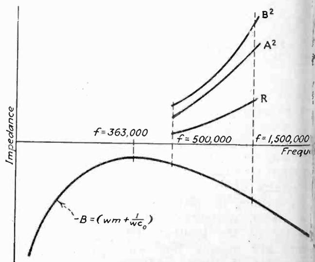
Fig. 6—Characteristics of the new pre-selector circuit
