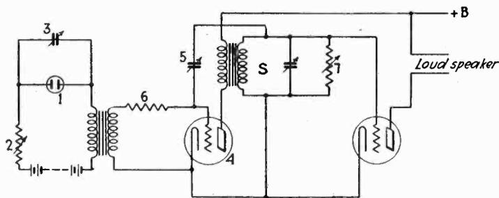
Fig. 1—Circuit to illustrate theory of producing damped oscillations or "Hallformanten"
