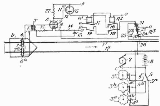
**Railway traffic control.** Direct current is periodically supplied to a track-rail, the train carries a vacuum tube receiving circuit system in which an amplifier tube is coupled by resistance to a following tube which operates a relay controlling the train. L. L. Nettleton, assigned to the Union Switch & Signal Company. No. 1,772,781.
