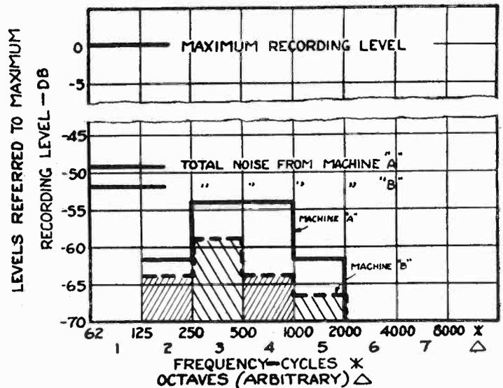
Fig. 5—Annoyance analysis of disc turntable mechanical vibration
