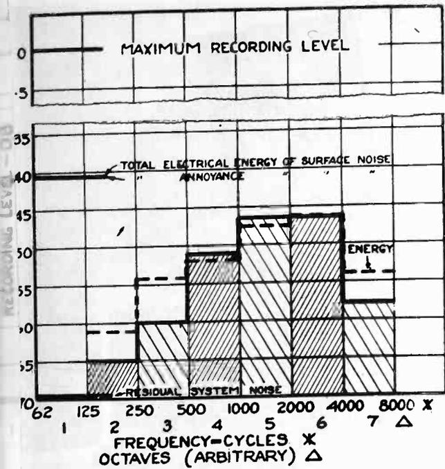
Fig. 4—Electrical energy and annoyance analysis of disc surface noise
