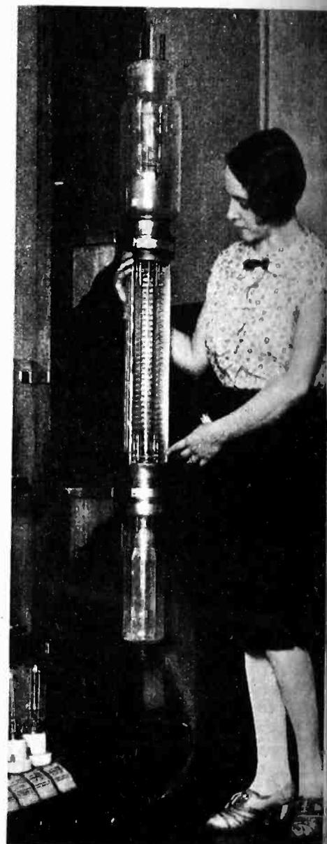
One of the 200-kw. tubes installed in the new KDKA station, near Saxenburg, Pa.
