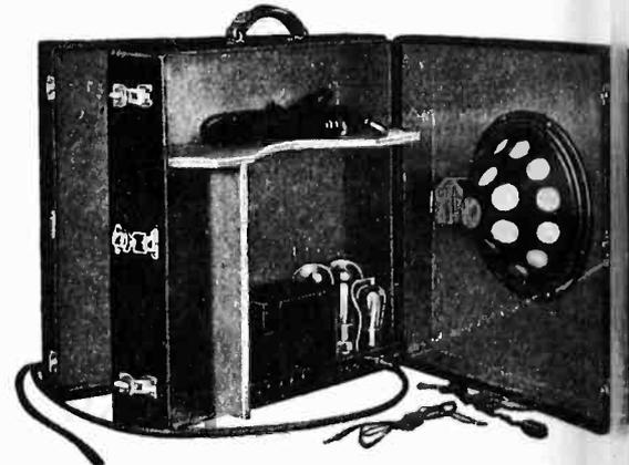
Amplifier unit designed by QRS-DeVore Corporation, Chicago. One 224, one 250 and one 281 tube are used. The speaker section may be removed from the case
