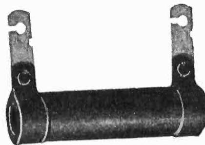
ture-proof enamel. Contact bands and soldering lugs are of Monel metal. The lugs are solder-dipped for easy connection. All parts expand equally under load. The overall length of the unit is 2 inches, with a maximum outside diameter of  $\frac{5}{8}$  inches. It is made with resistance ratings from 10,000 to 250,000 ohms.—*Electronics, Sept., 1930.*
