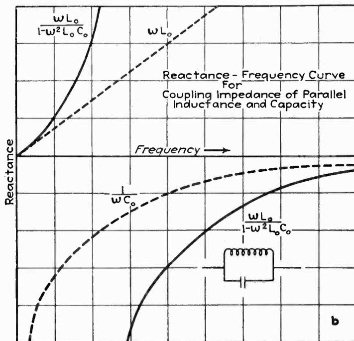
Fig. 2—Reactance-frequency curves for series- and parallel-tuned circuits
