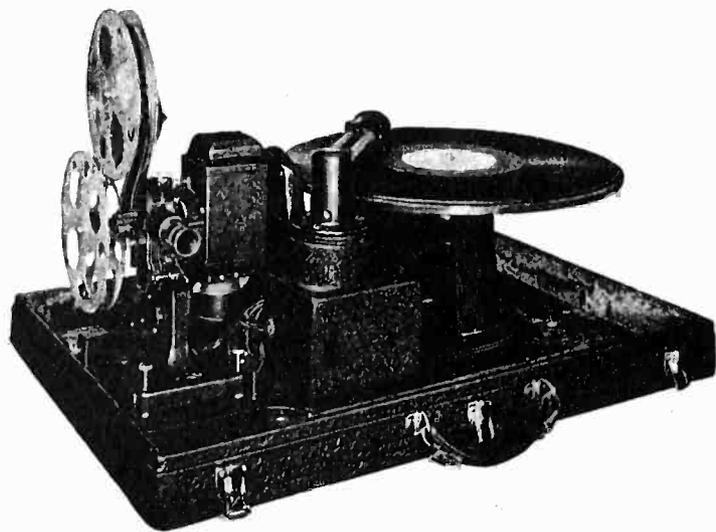
The turntable and 16 mm. projector unit are integral in this portable unit manufactured by the QRS-DeVry Corporation, Chicago
