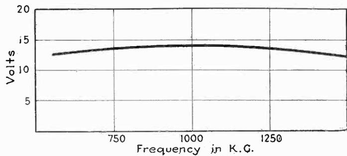
Fig. 2—Output characteristics of signal generator (right)
