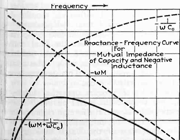
Fig. 4—Reactance-frequency curve for mutual impedance of capacity and negative inductance
