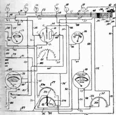
**Testing equipment.** A patent device, involving the testing of vacuum tubes by means of apparatus arranged to vary the grid potential and thereby vary the mutual conductance and the plate potential to increase the resistance, etc., all contained in a cabinet. J. H. Miller, assigned to General Electric Instrument Company, Schenectady, N. Y. No. 1,771,504.
