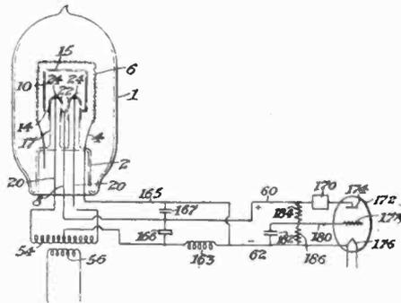
**Rectifier and voltage regulator.** Two patents granted to T. E. Foulke and assigned to General Electric Vapor Lamp Company, Hoboken, N. J., dealing with a combination of a gaseous rectifier and a voltage regulator in a single envelope. Nos. 1,772,562 and 1,772,603.
