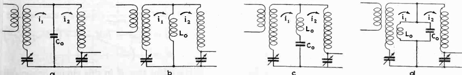
Fig. 1—Various coupling impedances for two tuned circuits. A common impedance that is capacitive is shown in (a). Circuit (b) will produce separations depending on  $R$  and its change with frequency. Circuits (c) and (d) combine inductive and capacitive coupling
