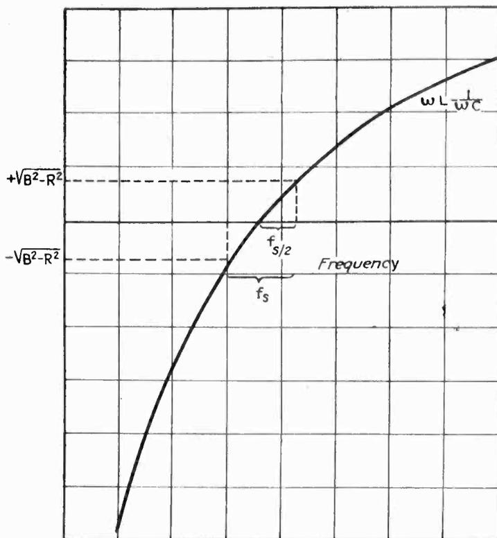
Fig. 5—Reactance-frequency curve of tuned circuit
