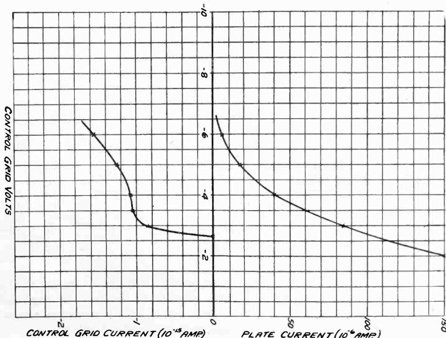
Right: Characteristics of the low-grid current tube
