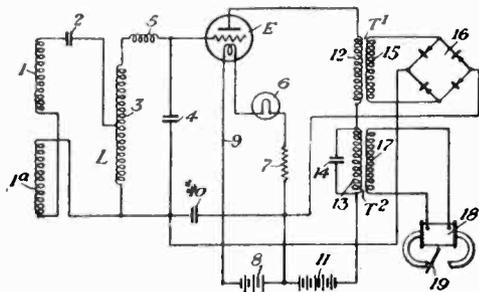
**Train control apparatus.** Vacuum tube circuit to be carried by a train capable of picking up electrical energy from the trackway and thereby controlling the train. G. W. Baughman, assigned to the Union Switch & Signal Co. No. 1,772,796.
