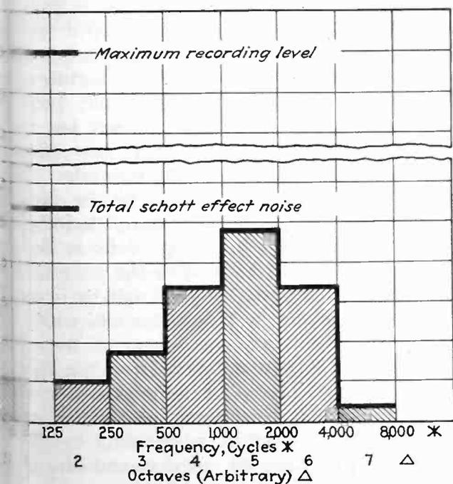
4—Annoyance analysis of photo-electric cell due to Schott effect
