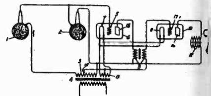
**Illumination control.** Two light sensitive cells, normally balanced and arranged that when substantially equal amounts of light fall upon the series of lamps is lit. H. C. Sletten, assigned to G. E. Co. No. 1,775,577.
