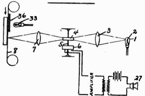
**Sound-record film and apparatus.** Variations on a film corresponding to sound wave variations, with opaque, straight edge borders upon opposite sides of the sound record. J. R. Balsley, assigned to Fox Case Corp. No. 1,776,058.
