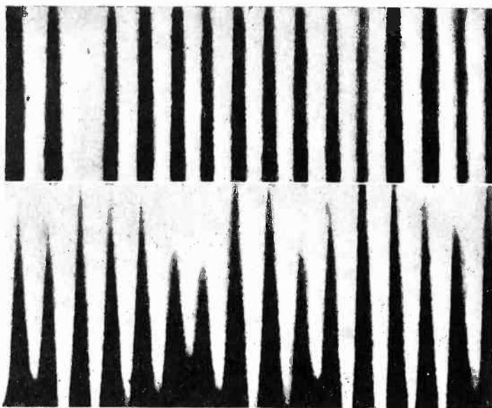
Fig. 2—Photomicrograph of a typical variable density sound track (at top) and variable area (at bottom). These two sound tracks are recordings of the same sounds
