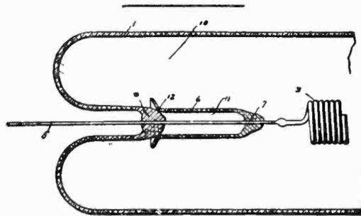
**Method of fixing electrodes in glass tubes.** A separate heat-conducting member sealed to the stem of an electrode. F. B. Hale, one-half assigned to W. C. Brumfield, San Francisco. No. 1,775,198.
