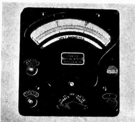
moulded Bakelite. All instruments are magnetically shielded. Accuracy is within one per cent of full scale value. The prices range from \$40.25 to \$53.25.—*Electronics, October, 1930.*
