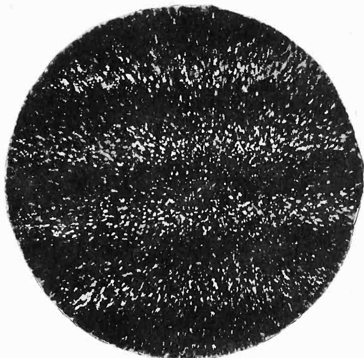
Fig. 1—Photomicrograph of sound track on positive stock. A magnification of 250 times shows grains and grain clumps
