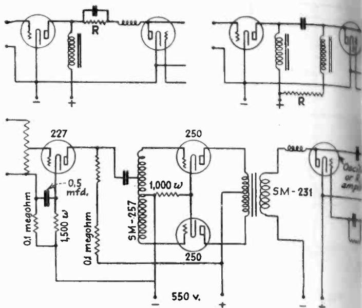
Fig. 5—Circuits adapted for high modulation
