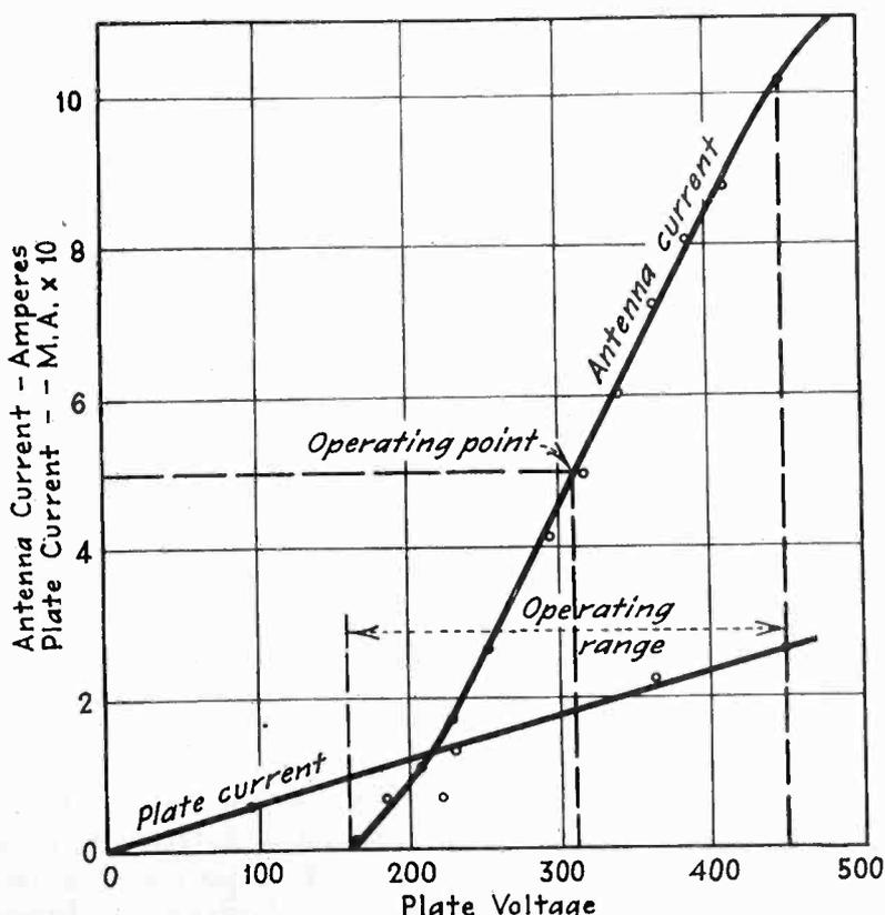
power input to the tube increases by a factor of 1.5 during complete modulation. Therefore the r.f. power increases by a like amount, or the r.f. current by a factor of  $\sqrt{1.5}$ , or 1.224. The r.f. current in either tank or antenna circuit, should increase 22.4 per cent when modulating 100 per cent.
