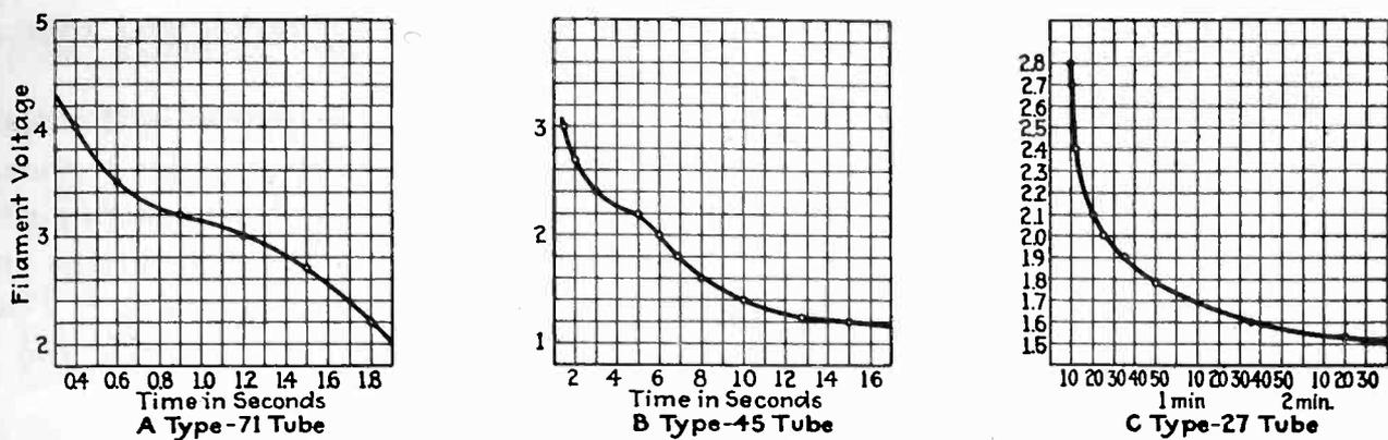
Fig. 7—Typical time-delay curves for three types of tubes covering usual range for delay action
