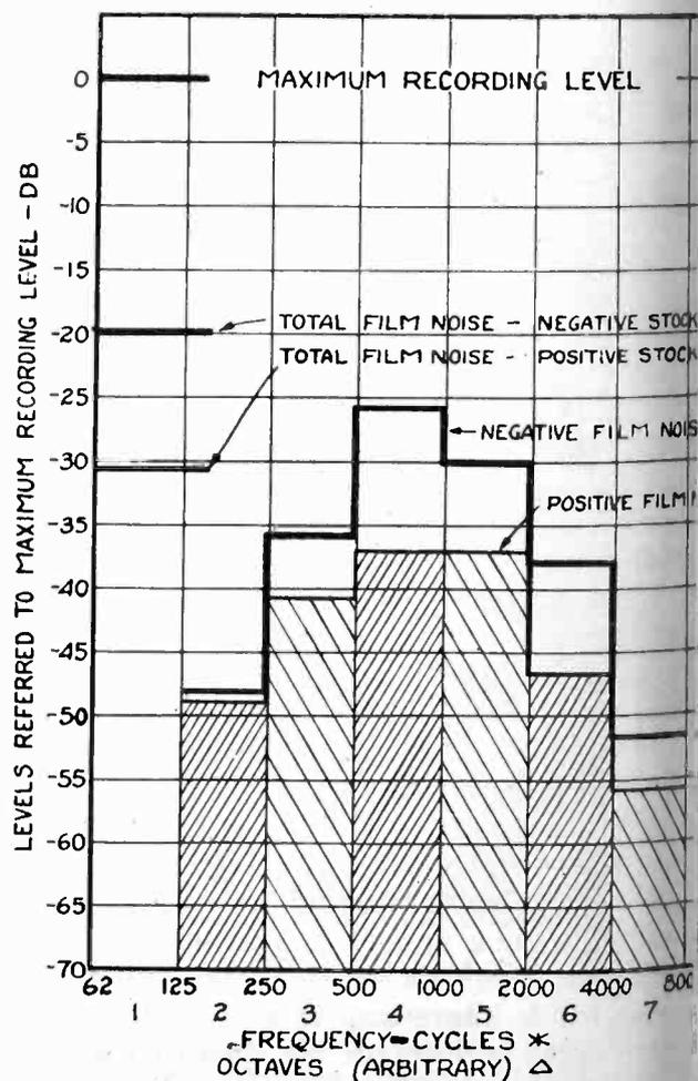
Fig. 3—Annoyance analysis of total film reproduction noise, comparative measurements for negative and positive stock are shown
