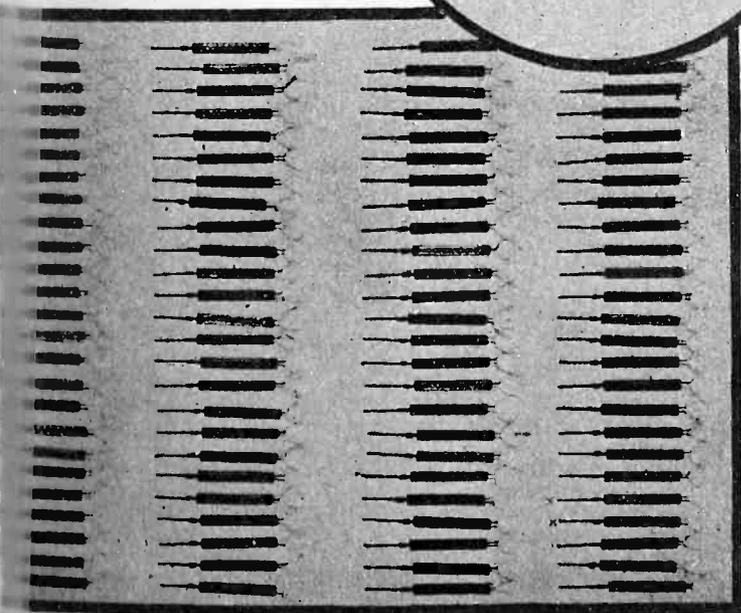
X-ray picture of tray of 100 radio-tube cathodes in Raytheon laboratory. Defectives are marked with an X
