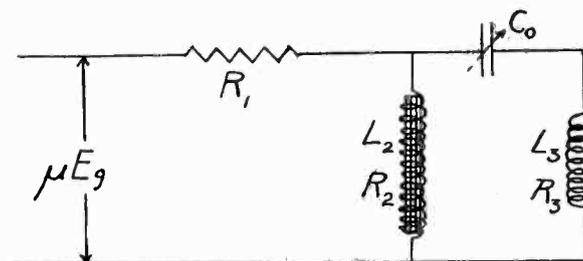
Circuit arrangement for condenser coupled tune amplifier, and its equivalent electrical circuit
