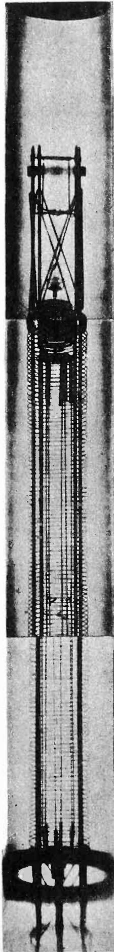
An X-ray photo, made in three sections, of a 100-kw. tube
