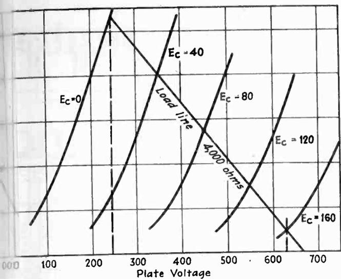
Fig. 2—Characteristics of power tube of the 250 type
