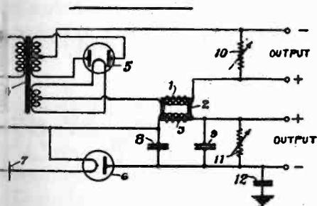
**Amplifier-filter circuit.** Combination of two double wave rectifiers to pre-attenuation of the core of a filter. Humphrey Andrews, London, England. No. 1,774,822.
