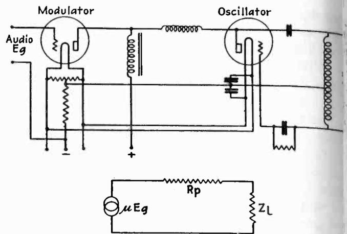
Fig. 1—Conventional diagram and simple equivalent of modulator-oscillator system
