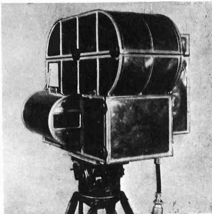
Fig. 5—Rear view of light-weight camera cover designed to overcome camera noise during recording
