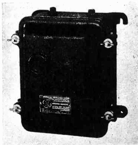
same case. It is made, as so far announced, only for alternating current circuits. This new relay makes possible a great number of outdoor photo-cell applications, such as alarms in outdoor garage ramps, outdoor counting operations, etc.—*Electronics, October, 1930.*
