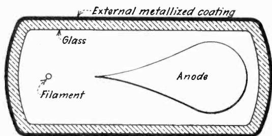
Above: Cross-section of gridless tube
