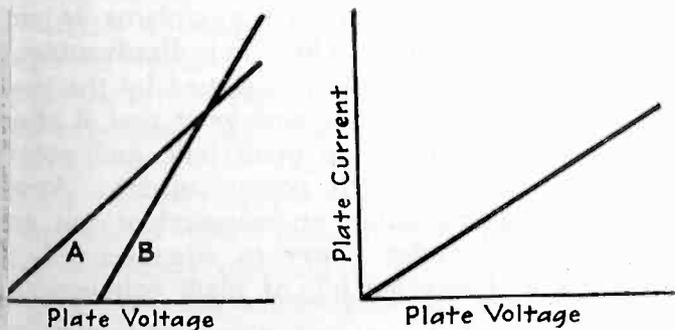
Above: Fig. 3—Relation between plate voltage, plate current, and antenna current in distortionless system
