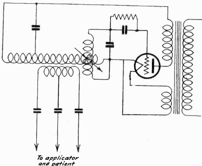
Electronic tube employed as both rectifier and oscillator
