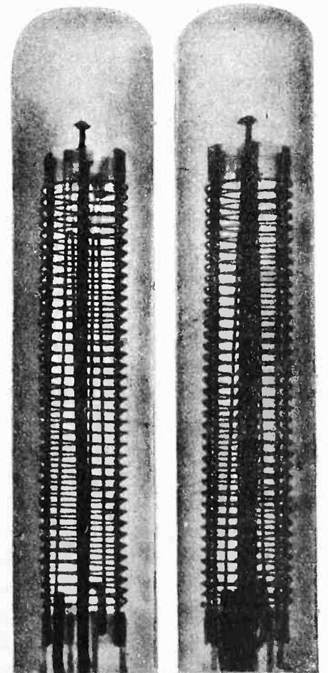
Two shadowgraphs of grids in UV-207 (20 kw.) tubes made by X-rays
