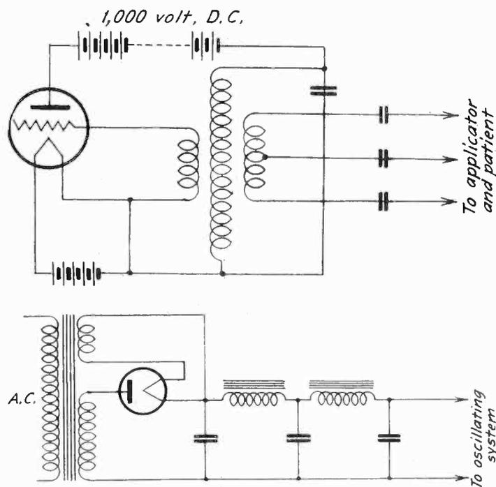
Above—Circuit of simple electronic-tube device for surgical cutting and coagulating
