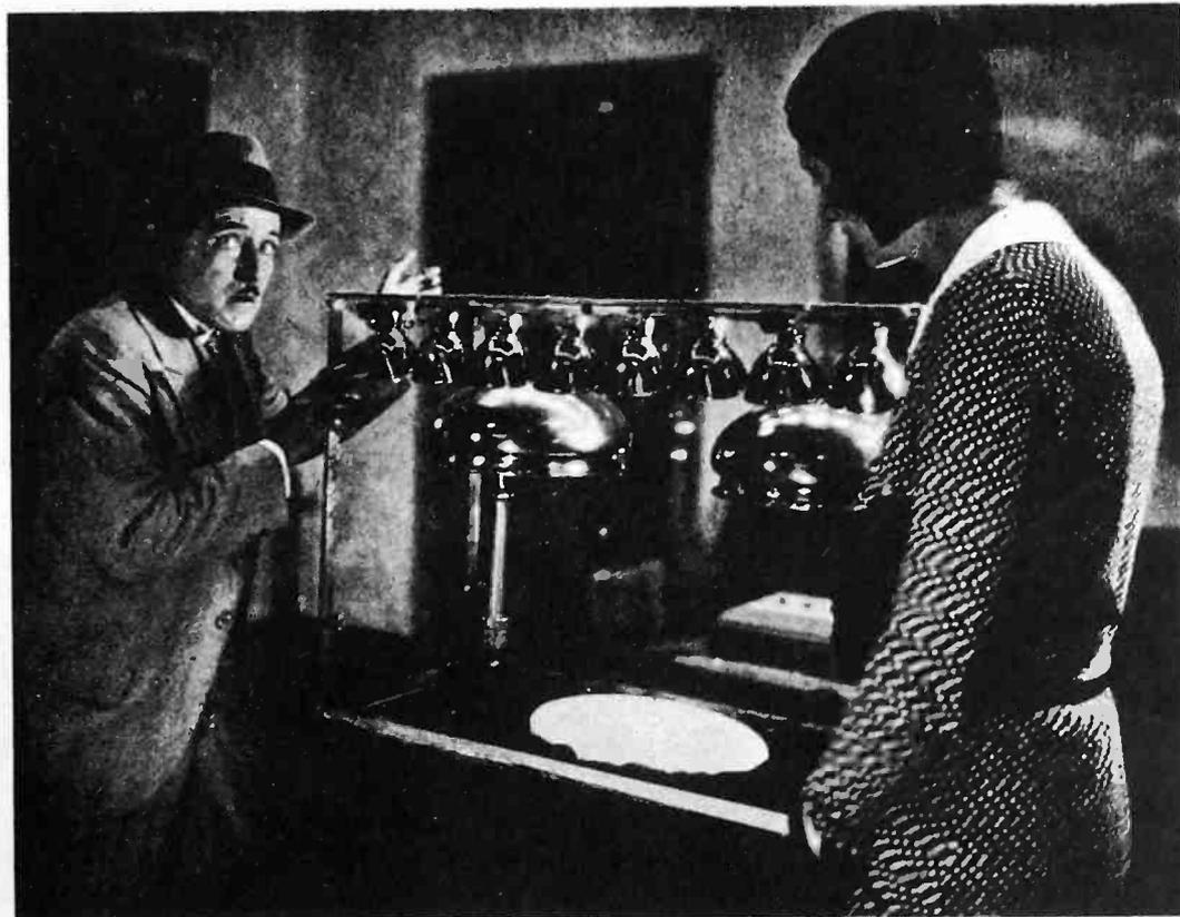
This new and scientific burglar alarm uses a grid-glow tube as a silent and invisible electric watchman. The tube when adjusted in the apparatus is so sensitive that the presence of a human being at a predetermined distance operates an alarm relay
