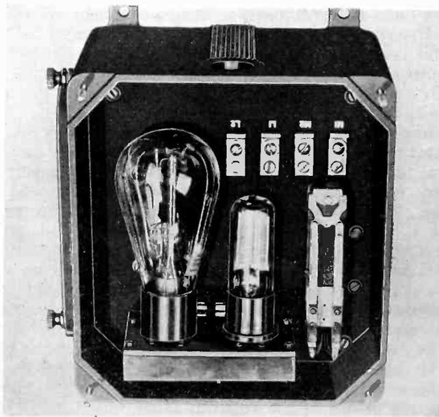
Westinghouse relay for the control of illumination or industrial processes
