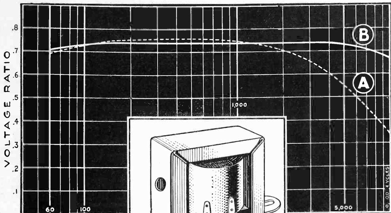
**A** This is the response curve of the audio-frequency transformer, shown on this page, wound with an ordinary layer winding. Note the sudden drop of the response curve at the higher frequencies. This was corrected by redesigning only the winding. See Curve B in the above diagram.
