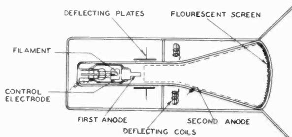
Cross-sectional view of the cathode-ray tube showing detail assembly
