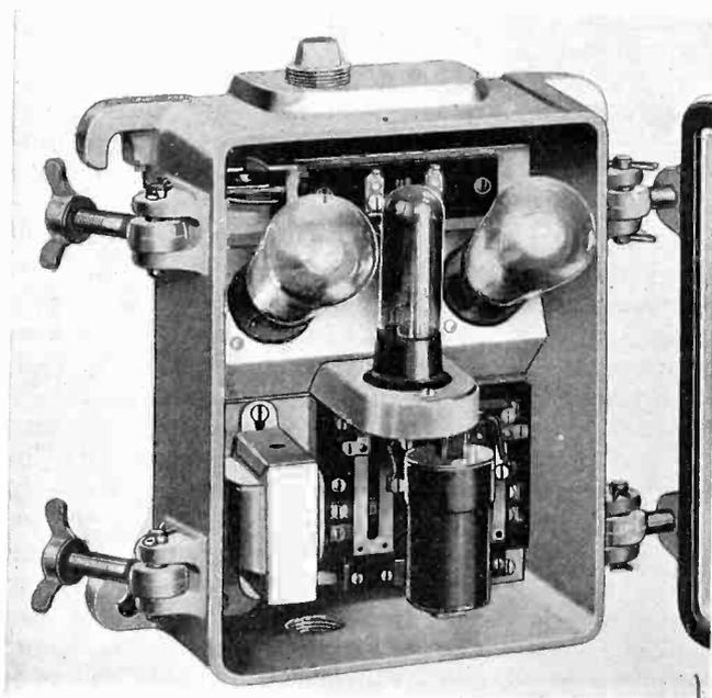
Allen-Bradley equipment in which phototube controls glow tubes
