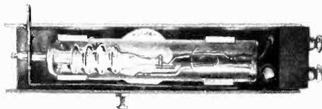
vacuum contact which in turn controls up to 6 amperes continuously or 8 amperes intermittently, at potentials up to 220 volts. The vacuum contact has innumerable possibilities in controlling power circuits by means of the most delicate actuating force.—*Electronics, November, 1931.*
