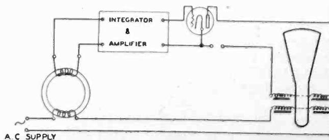
Elementary circuit adapted for the cathode tube used for hysteresiograph
