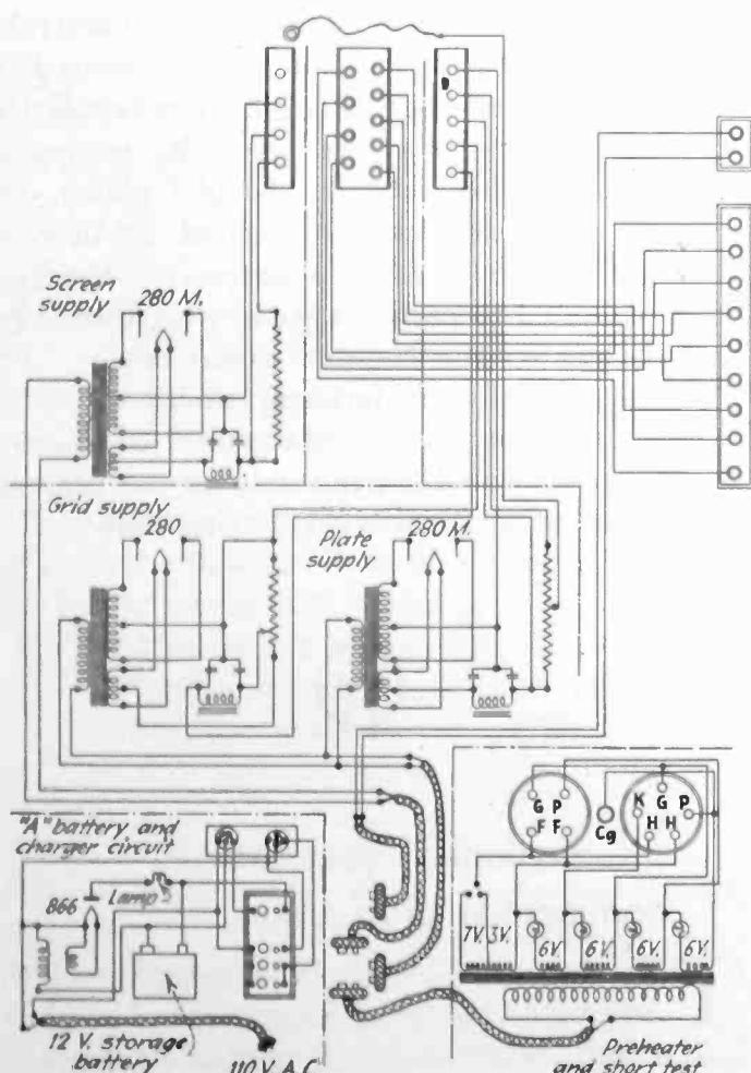
**Power supply equipment for the tube testing board.**
