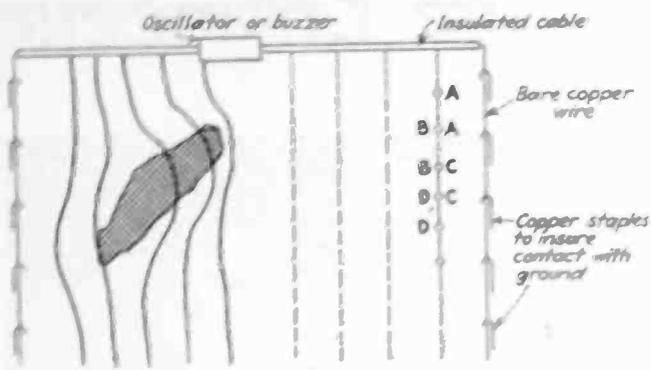
Fig. 1—Location of underground body by equipotential method
