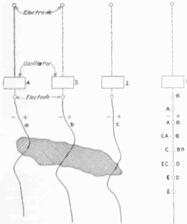
Fig. 2—Potential ratio method of prospecting electrically
