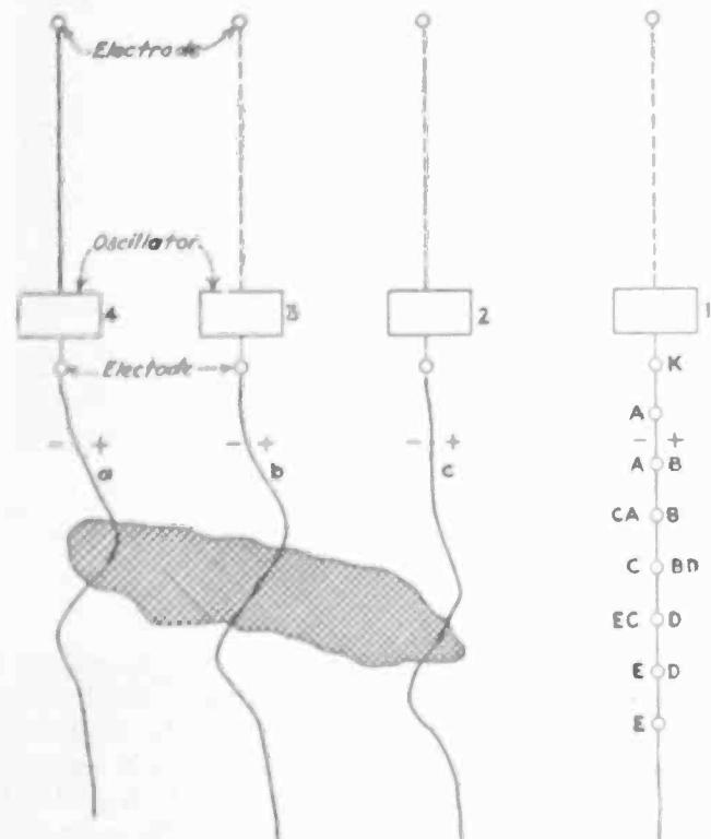
Fig. 2—Potential ratio method of prospecting electrically
