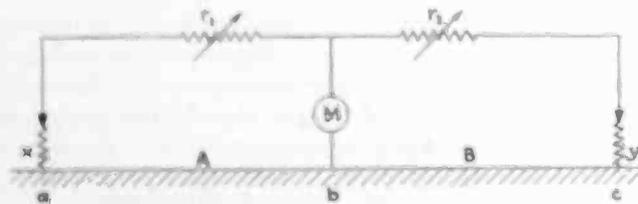
Fig. 3—Compensation for contact resistance in potential ratio method
