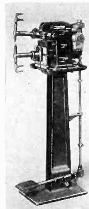
.0005 in. to  $\frac{1}{8}$  in. combined thickness of steel. The principal advantages claimed are: Speed in production, uniform welds, positive and smooth in action, simplicity of construction, few working parts, rugged and compact, wide range of heating steps and low maintenance cost. — *Electronics, November, 1931.*
