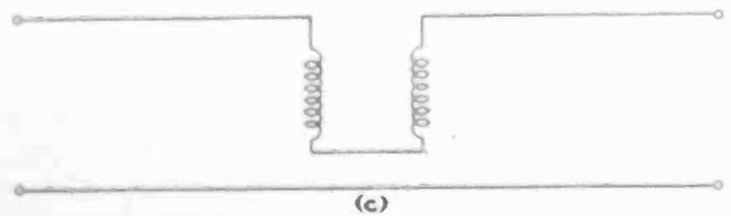
Fig. 8—Fundamental diagram of the phase balancer
