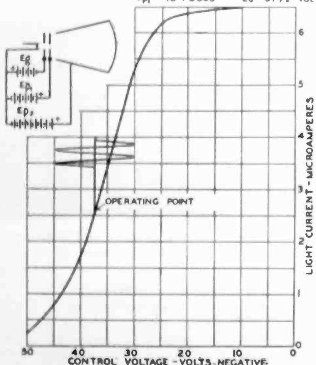
Modulation characteristics of the tube with operating voltage limits indicated
