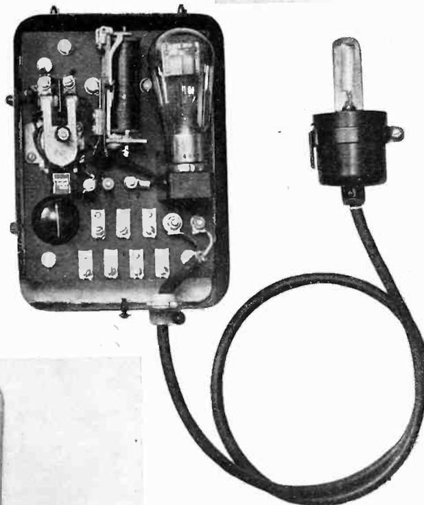
The General Electric unit has a portable phototube making it possible to house the relay and amplifier tube at some distance from the operation under control
