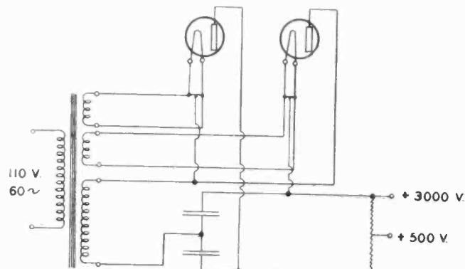
Arrangement of circuits for supplying necessary voltages for operating oscilloscope from a.c. mains
