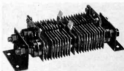
Washington Ave., St. Louis, Mo. It occupies a space of only 7½ in. by 2½ in. by 2½ in., and may be given a continuous output rating of 75 watts. It will operate directly from the 115-volt a.c. line.—*Electronics, November, 1931.*
