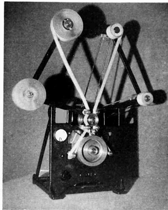
Sound-printer designed by J. S. Watson and R. V. Wood which automatically compensates for film shrinkage and reduces high-frequency losses
