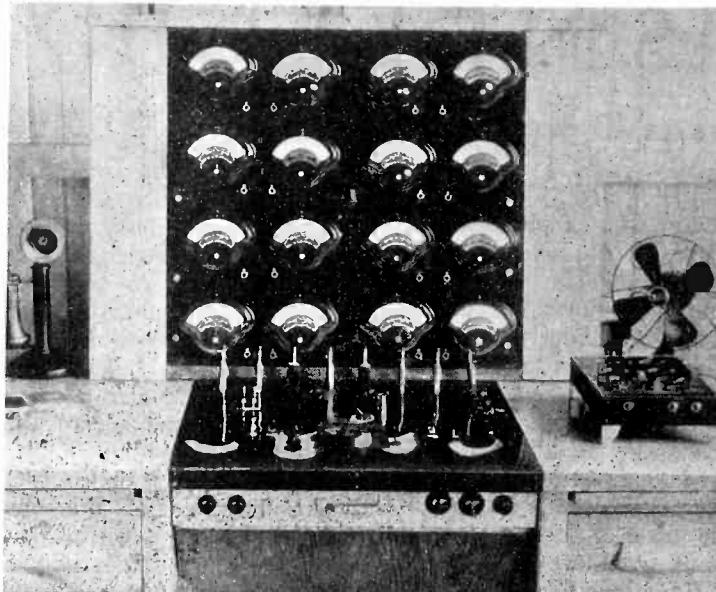
Entire tube test apparatus is installed in a standard office desk making an examination for defects a simple and time-saving procedure
