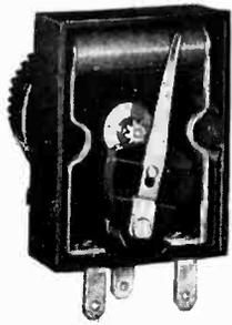
In the Bradleyometer approximately 50 solid resistance disks are interleaved between metal disks, forming a resistance column that will produce any form of resistance-rotation curve, as shown to the right.
