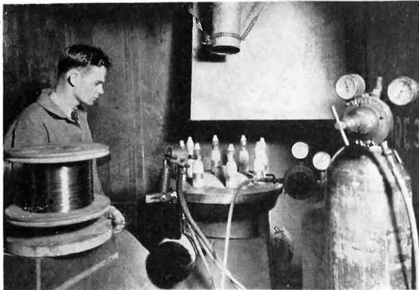
Spraying operation during the manufacture of spray shield tubes in the plant of Grigsby-Grunow Company. The machine is automatic and uses zinc wire for making metal spray
