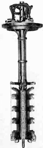
Support for the nine filament wires requiring 500 amperes of current and emitting 160 amperes
