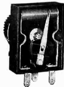
In the Bradleyometer approximately 50 solid resistance disks are interleaved between metal disks, forming a resistance column that will produce any form of resistance-rotation curve, as shown to the right.
