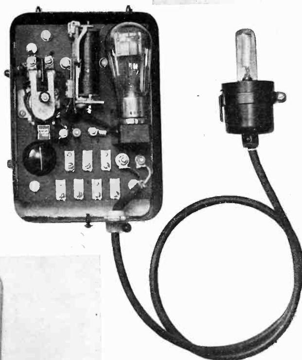
The General Electric unit has a portable phototube making it possible to house the relay and amplifier tube at some distance from the operation under control
