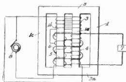
**Piezo-electric oscillator.** Crystals of opposite temperature coefficients connected in series to compensate temperature effects. R. A. Heising, B.T.L. No. 1,827,196.
