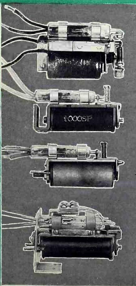
For utmost convenience, the vacuum contact is now available in a standard mounting as shown above. Heavy casting, nickel finished, protects glass mechanism. Link extends through slot and connects with actuating force. Adjustment screw regulates pressure applied on extension stem of vacuum contact. Mounted for normally open or normally closed circuit
