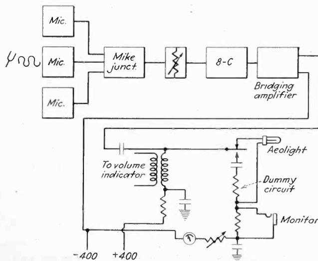
Fig 2—Typical glow-lamp recording circuit with associated equipment
