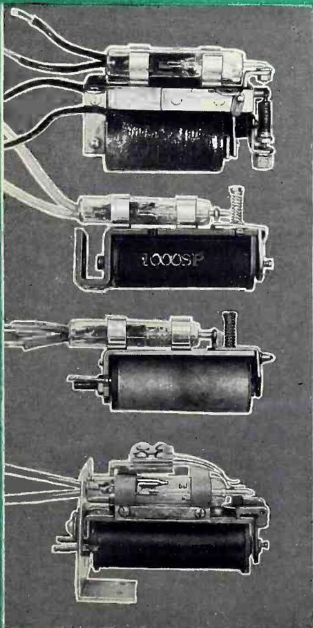
For utmost convenience, the vacuum contact is now available in a standard mounting as shown above. Heavy casing, nickel finished, protects glass mechanism. Link extends through slot and connects with actuating force. Adjustment screw regulates pressure applied on extension stem of vacuum contact. Mounted for normally open or normally closed circuit
