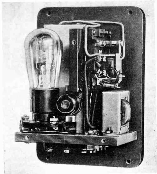
In the Struthers Dunn relay shown above the phototube is located at the lower center
