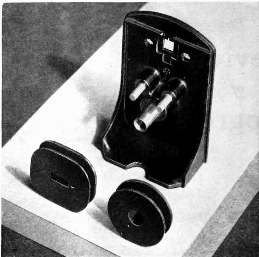
Bakelite Molded back plate and spools used in electric pick-up, made by Webster Electric Co., Racine, Wisc.
