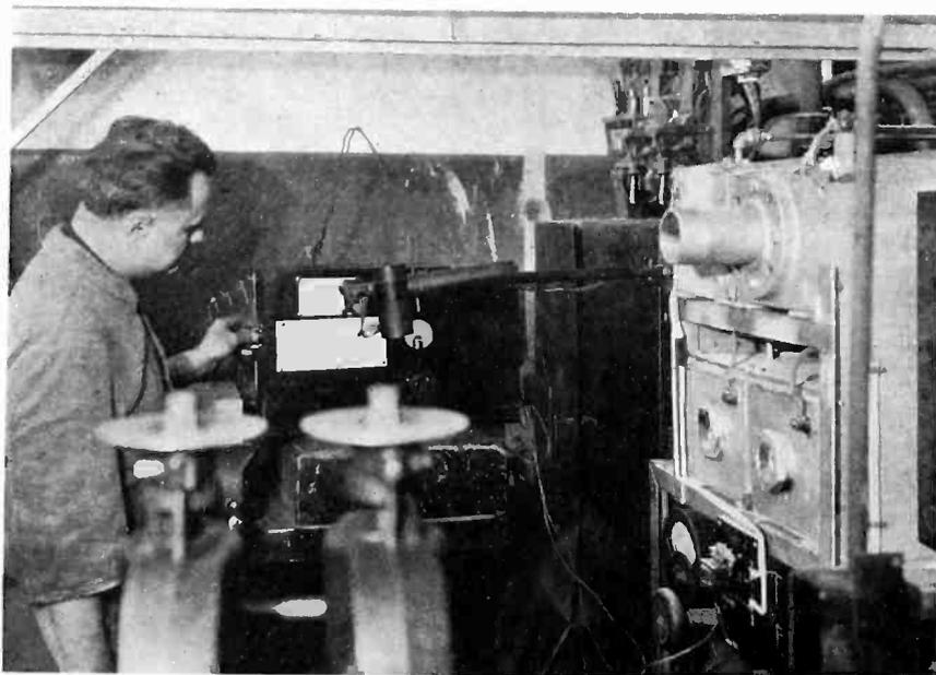
Apparatus developed by Dr. L. R. Koller uses a phototube and amplifier system for controlling furnace temperature
