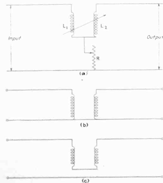
Fig. 8—Fundamental diagram of the phase balancer
