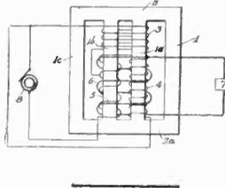
**Piezo-electric oscillator.** Crystals of opposite temperature coefficients connected in series to compensate temperature effects. R. A. Heising, B.T.L. No. 1,827,196.
