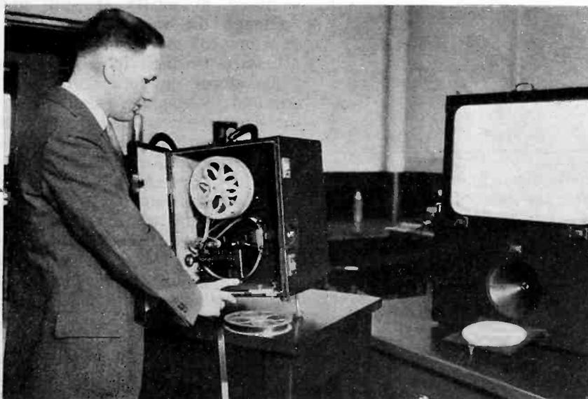
Projection equipment which uses 16 mm. sound-on-film with sprocket holes on one side only. Designed by the Westinghouse Research Laboratories and later turned over to RCA Victor for commercial development
