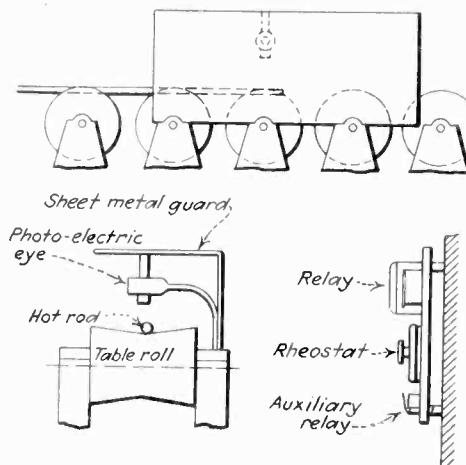
A photo-tube above the red-hot bar, operates relays and a cut-off saw, cutting bars in even lengths
