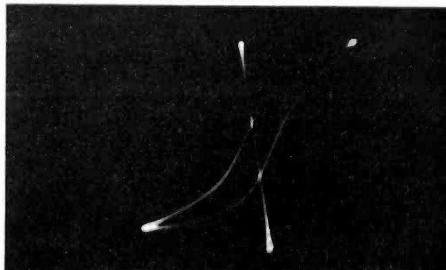
Sample of photographic recording of a hysteresis loop obtained by means of an outside camera
