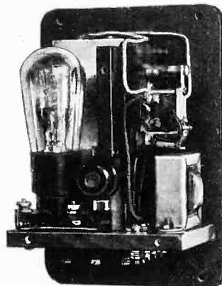
PRICED at \$30, the new light sensitive cell unit can now be put to thousands of uses, not possible before, because of much higher cost. The new unit operates on standard voltage—110 volt, 60 cycle. Special sets, both A.C. and D.C., can be built to order when other voltages are required. The set uses a standard UV 112-A tube and is housed in an aluminum finished case 6" x 5" x 3" overall. Circuit construction diagram and complete information will be sent promptly.
