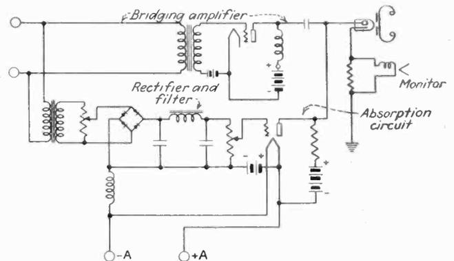
Fig. 5—Simplified circuit using a full wave contact rectifier in place of thermionic rectifier
