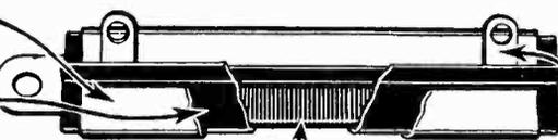
TERMINALS OF BEST GRADE COKE PLATE FOR EASY SOLDERING
