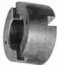
A coupling disc fabricated by National from a grade of Phenolite developed for the known requirements of this particular part—high tensile strength and resistance to wear; unaffected by oil, acid and moisture; highly shock absorbing.
