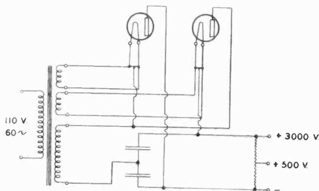
Arrangement of circuits for supplying necessary voltages for operating oscillograph from a.c. mains
