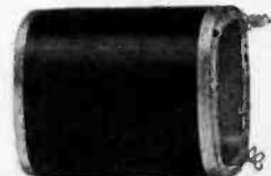
Power Amplifier Transformer Coil wound on No. 104 "Universal" Multi-Coil Winder.
