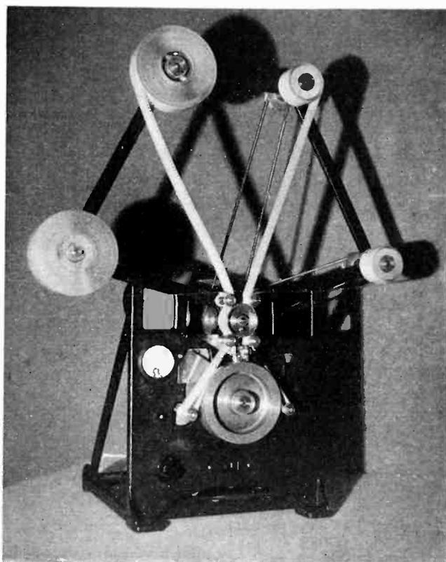
Sound-printer designed by J. S. Watson and R. V. Wood which automatically compensates for film shrinkage and reduces high-frequency losses
