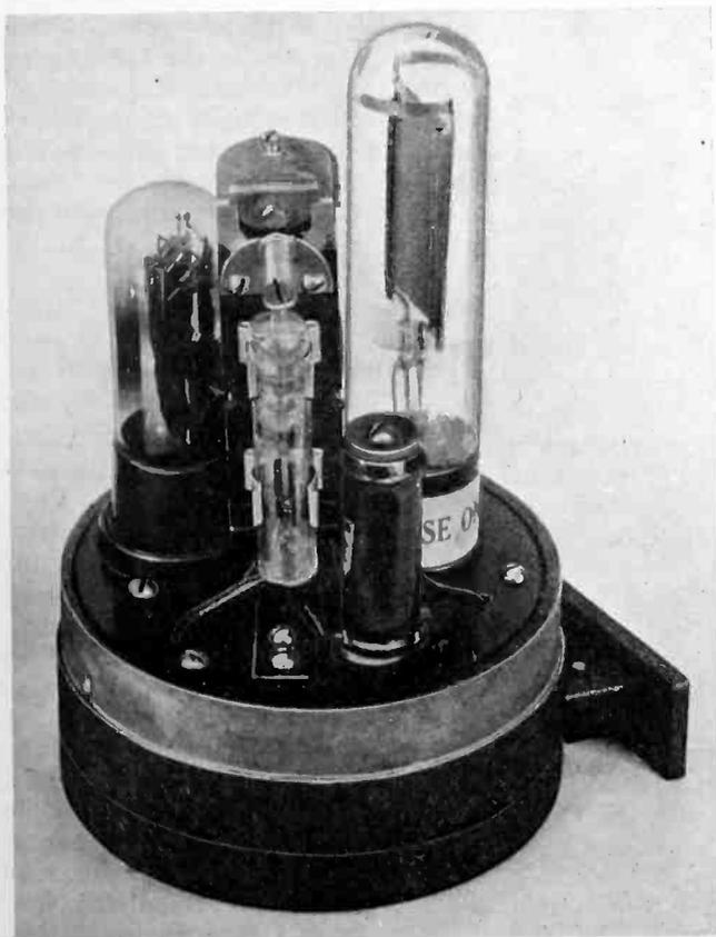
Burgess selenium bridge, triode and relay apparatus
