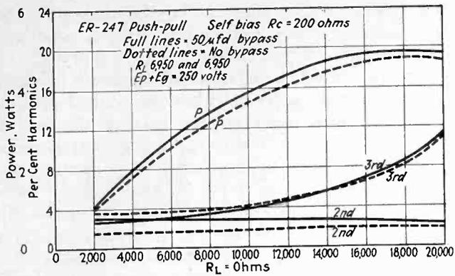
Fig. 4—Effect of by-passing self-bias resistance—push-pull pentodes
