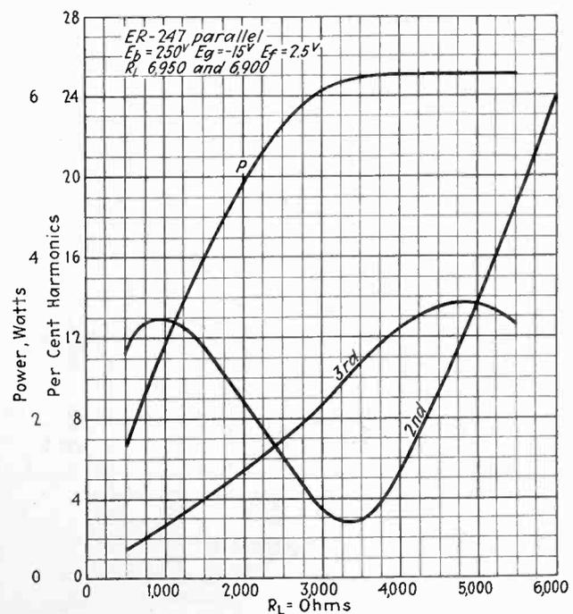
Fig. 3—Power output and distortion of pentodes in parallel
