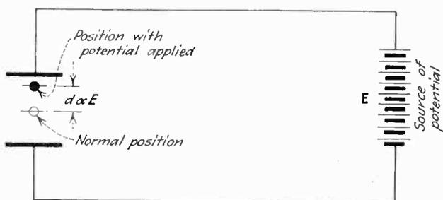
Fig. 1—Deflection is proportional to applied potential
