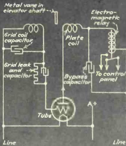
Tube control circuits for elevators in new McGraw-Hill building
