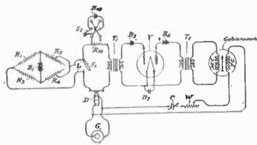
**High frequency generator.** A method of getting very high frequencies by a push-pull input stage, parallel output circuit in which the input capacity of the tube is in series with an output inductance. R. L. Davis, assigned to Westinghouse E. & M. Co. No. 1,832,621.
