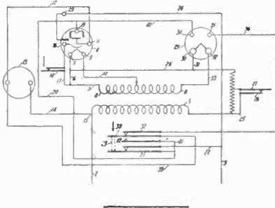
**Short wave antenna.** A radiation current meter is placed in the mid-point of an antenna, and the direct current leads from this meter are carried through a metallic tube to the transmitter room proper. D. K. Martin, assigned to A. T. & T. No. 1,831,921.
