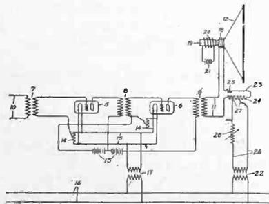
**Stabilizing circuit.** By means of an external circuit, two grid circuits of an amplifier are connected together in such a manner that undesired oscillations are prevented. T. H. Burns, Newark, N. J. No. 1,831,340.
