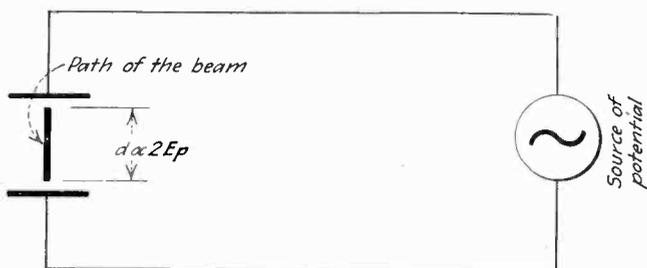
Fig. 2—Alternating e.m.f. produces straight line deflection
