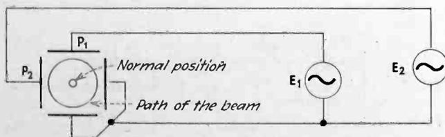
Fig. 4—Circular deflection produced by two alternating voltages of proper amplitude and phase
