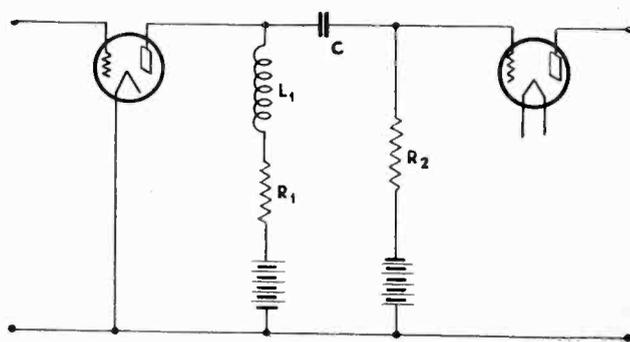
Fig. 2—A shunt circuit method of boosting high-frequency response
