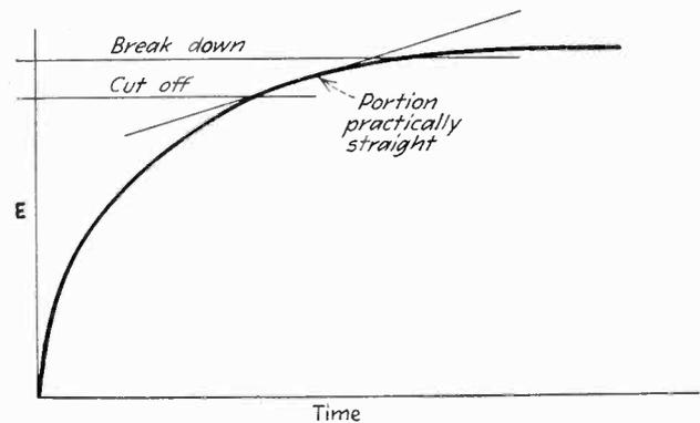
Fig. 6—Linear portion of charging rate of condenser used in timing scheme
