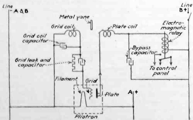
Simplified connection diagram of elevator-control system
