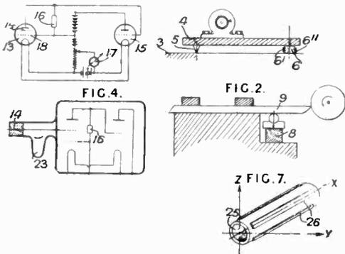
**Light and heat control apparatus.** Devices for automatically laying guns, etc., or for steering torpedoes, in which an image of the target is distributed on one or more light- or heat-sensitive cells connected in a balanced circuit. The out-of-balance current produced by this image actuates steering apparatus. K. Tihanyi, Budapest. No. 352,035.
