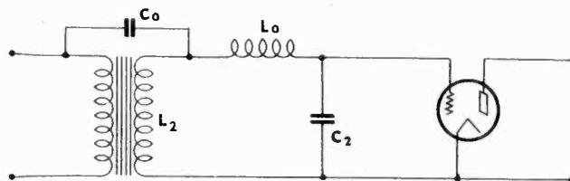
Fig. 1—Method of utilizing capacity between transformer windings
