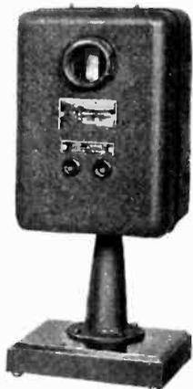
*Photometric relay unit CR7505-D3, indoor type, for the automatic control of factory, office, school, or residence lighting*
