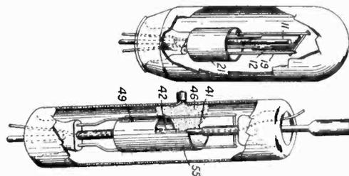
**Alkali cell.** Manufacturing patent dealing with method of manufacturing caesium type cells. Westinghouse Lamp Co. No. 345,043.
