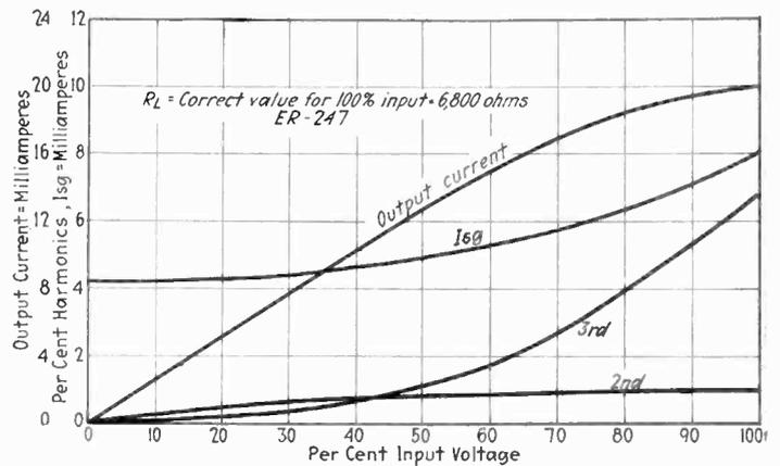
Fig. 2—Output current and harmonic content of power pentode
