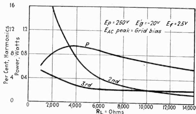
Fig. 5—Pentode used as triode; screen-grid tied to plate
