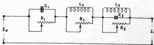
Fig. 3—Band suppression circuit consisting of a series of elements
