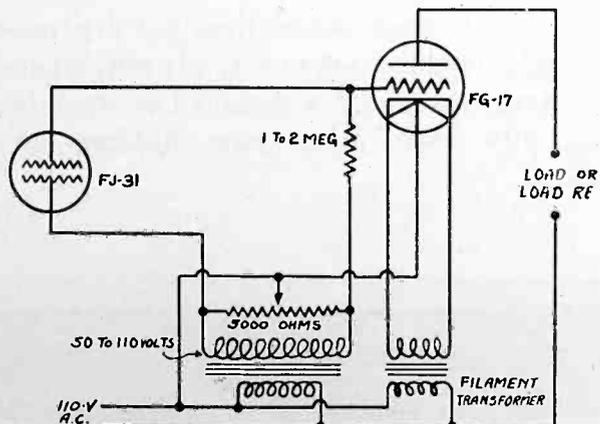
Use of selenium tube to control a Thyatron circuit
