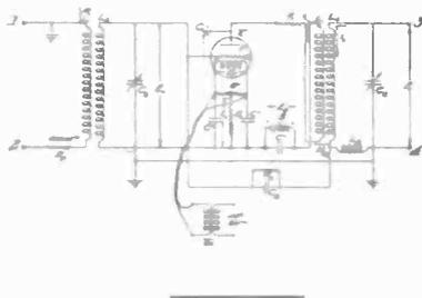
**Regenerative receiver.** Incoming oscillations set into oscillation a local circuit, low frequency oscillations controlling the oscillation of local circuit. Fritz Fischer, G. D. T. No. 1,833,323.
