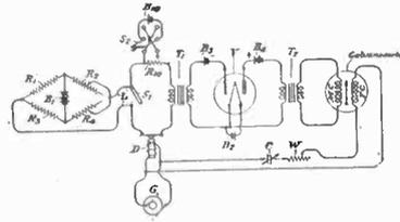
**High frequency generator.** A method of getting very high frequencies by a push-pull input stage, parallel output circuit in which the input capacity of the tube is in series with an output inductance. R. L. Davis, assigned to Westinghouse E. & M. Co. No. 1,832,621.
