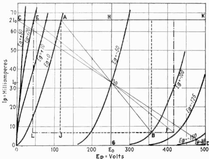
Fig. 1—Pentode characteristics; 247-type
