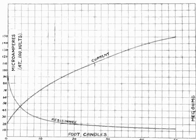
Light-current light-resistance characteristic of selenium tube
