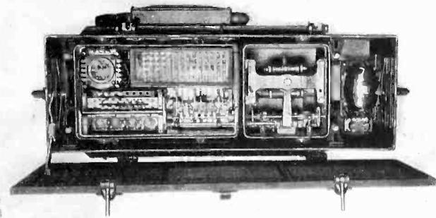
Detail view of the equipment box with dynamotor, governor, cams and four-tube amplifier
