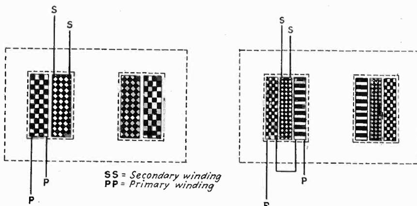
Fig. 1(a)—Standard transformer layer winding (left); (b) same transformer with interspaced winding (right)
