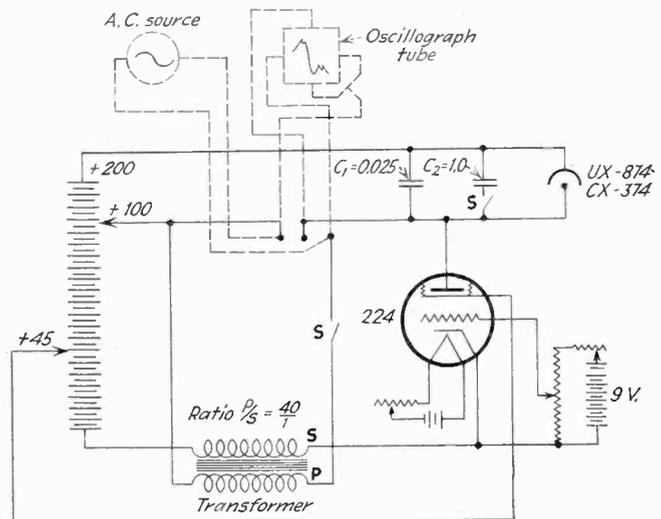
Fig. 5—Method of producing timing axis for cathode ray tube
