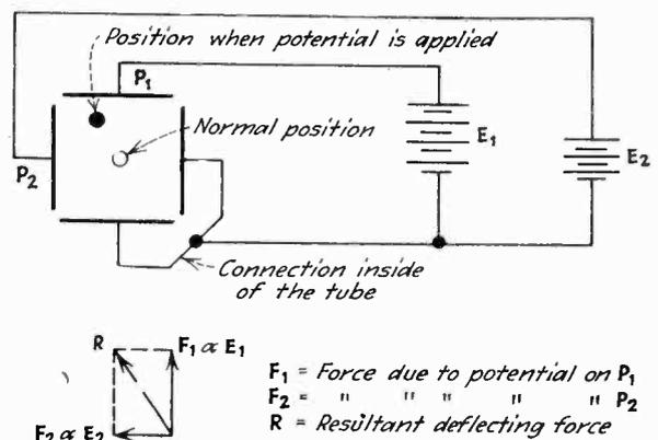
Fig. 3—Potentials applied to two sets of plates produce deflection proportioned to each
