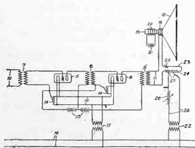
**Stabilizing circuit.** By means of an external circuit, two grid circuits of an amplifier are connected together in such a manner that undesired oscillations are prevented. T. H. Burns, Newark, N. J. No. 1,831,340.
