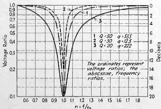
Fig. 5—Effect of varying circuits constants on sharpness and depth of suppression
