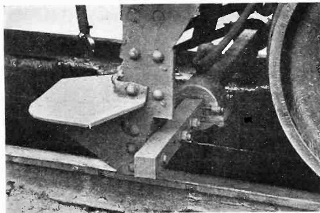
Close-up view of receiving coils mounted on cross-bar in front of the engine's forward wheels
