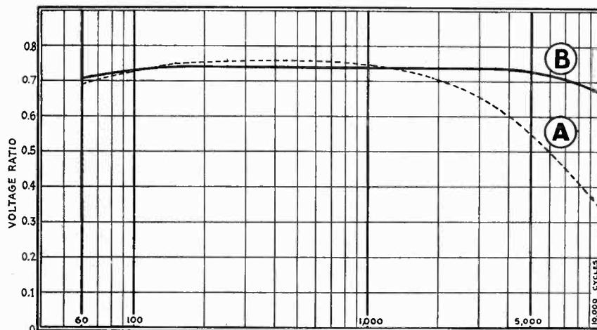
Fig. 2—Response curve (A) obtained with standard winding, (B) with interspaced winding
