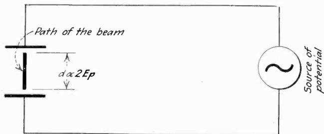
Fig. 2—Alternating e.m.f. produces straight line deflection
