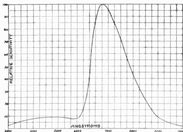
Spectral sensitivity of selenium showing high response in red
