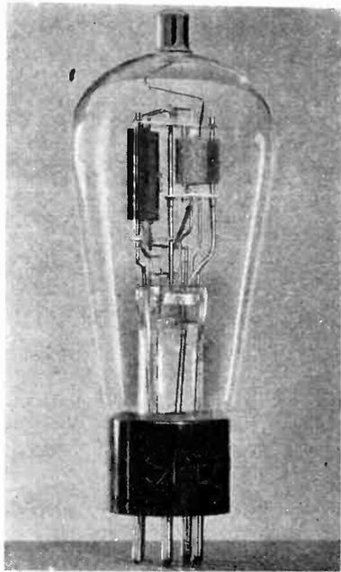
Voltage and power amplifier tubes directly connected, housed in one envelope
