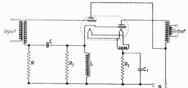
Method of connecting the double tube into the circuit
