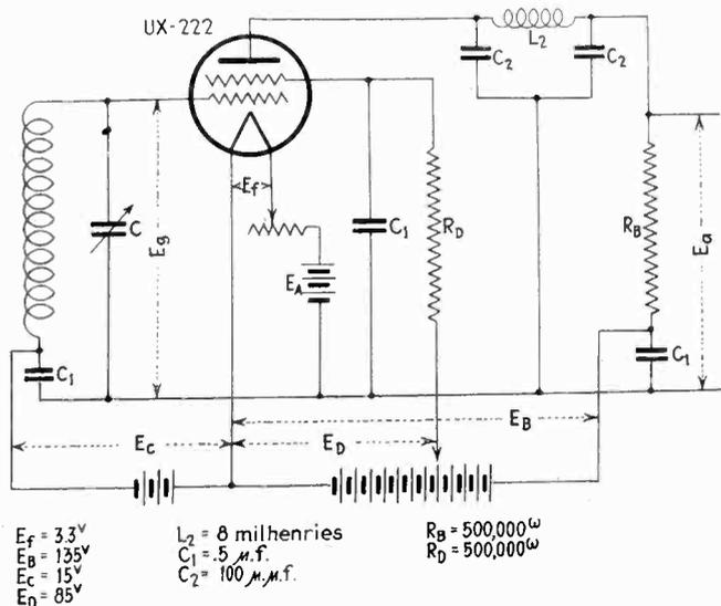
Circuit constants for the high overload limit detector
