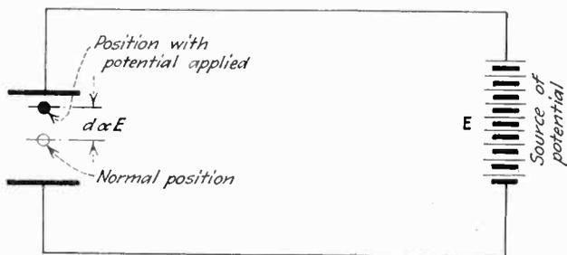
Fig. 1—Deflection is proportional to applied potential
