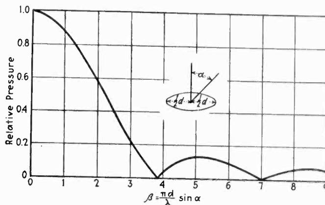
Fig. 2—Directional radiation characteristics of vibrating disc in infinite baffle
