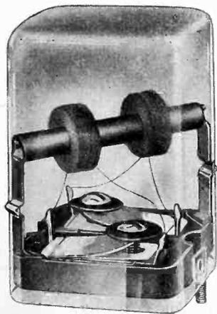
chassis, and held by two spade bolts. The coils are carried on a low-loss coil form and are extremely efficient in selectivity and gain. Compactly assembled, the coils are mounted on a newly developed material known as Learite and enclosed in a satin finished can.—*Electronics, February, 1932.*
