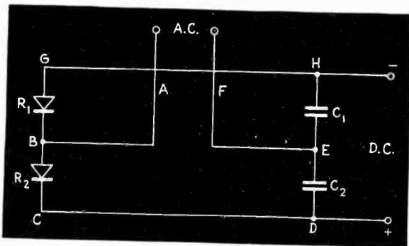
Fig. 1—Fundamental voltage doubler circuit
