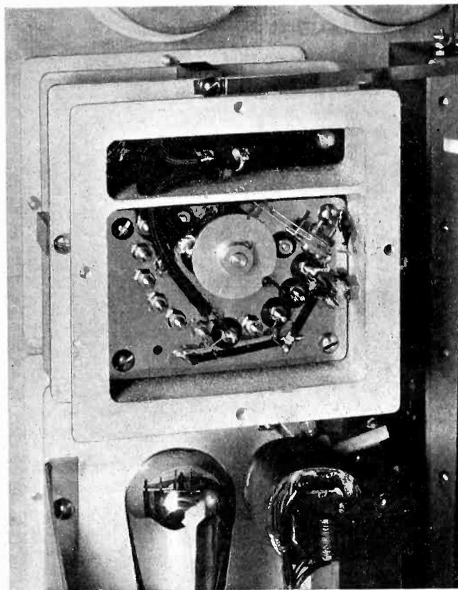
A 10-megacycle attenuator multiplier protected by a heavy aluminum case
