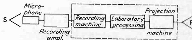
Fig. 1—Path followed by sound from source S to reproducer R
