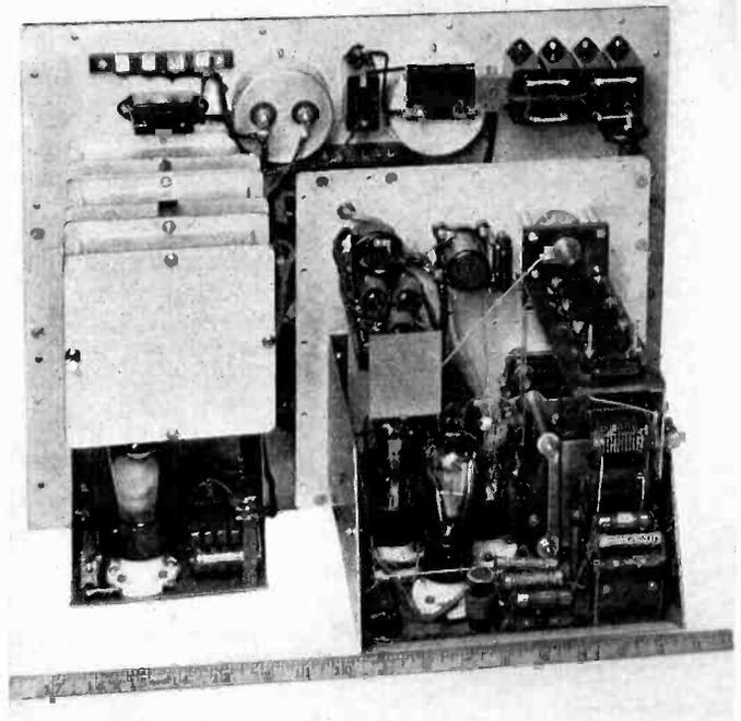
Interior of standard-signal generator with shield removed
