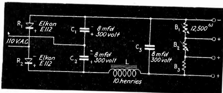
Fig. 2—Circuit constants of a modern commercial voltage-doubler
