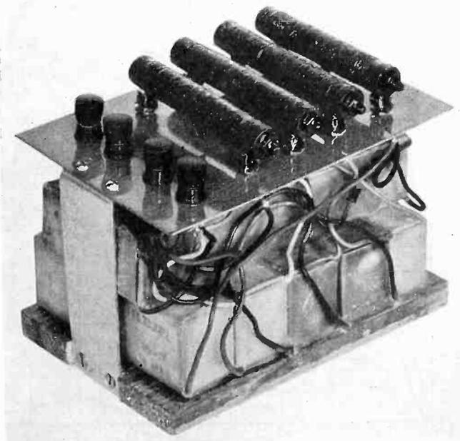
Fig. 6—Assembly of resistances, chokes, condensers, and rectifiers
