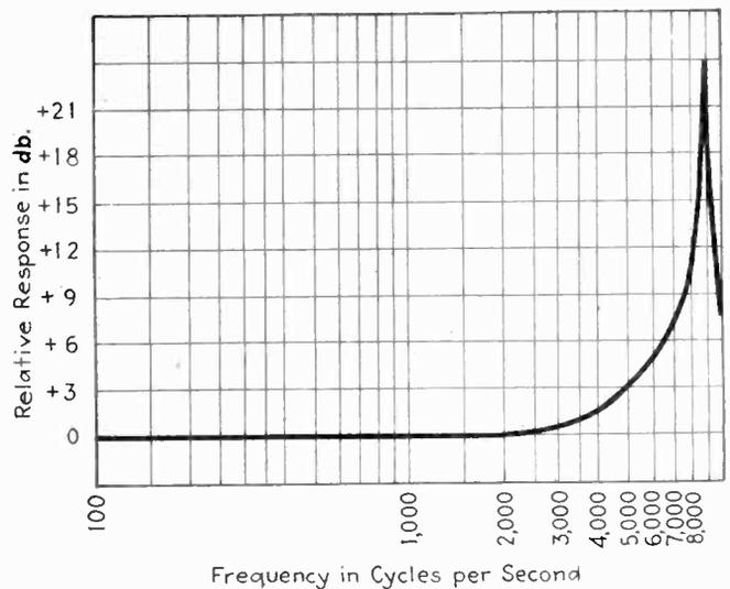
Fig. 3—Relative response characteristic of light valve tuned to 9,000 cycles
