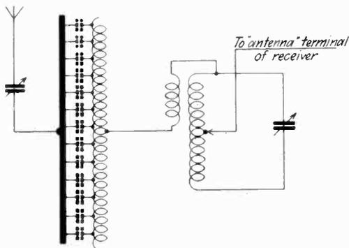
of fine wire are wound, so that close inductive and (distributed) capacitive couplings exist. It is claimed to produce very good band-filter effects and to possess many other advantages, the Editor confirms some of these.—*Radio B.F.f.A., Stuttgart, May, 1932.*
