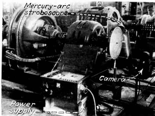
Sixty-cycle stroboscope and camera for photographing the angular transients of synchronous machines in the Electrical Laboratory M.I.T.
