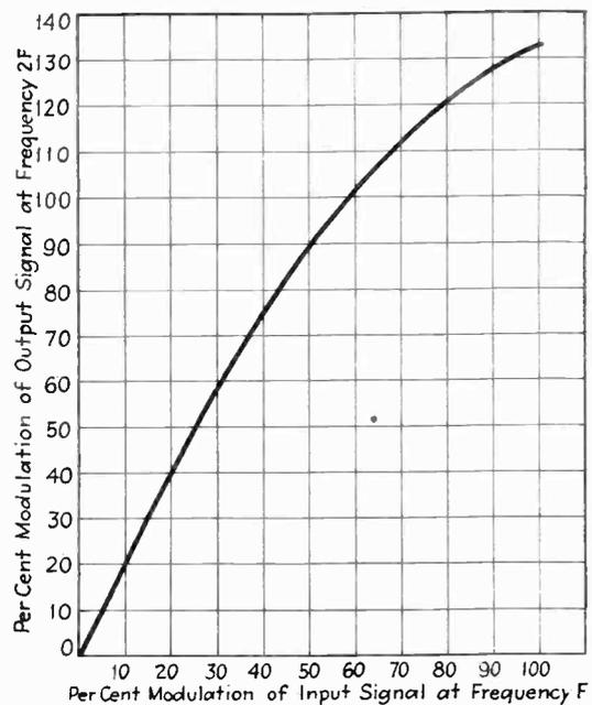
Fig. 4—Curve showing relation between input and output modulation
