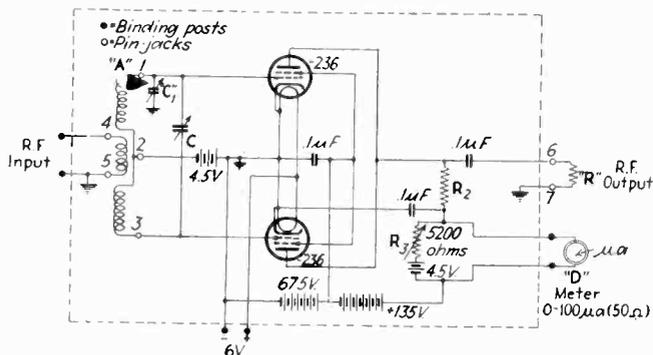
Fig. 1—Balanced circuit in which second harmonic is produced
