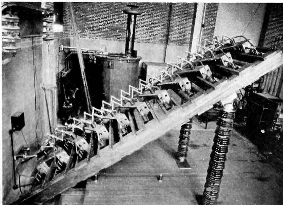
Kenetron chargers feed these condensers, in parallel; they can be discharged in series, while a cathode-ray oscillograph records the discharge
