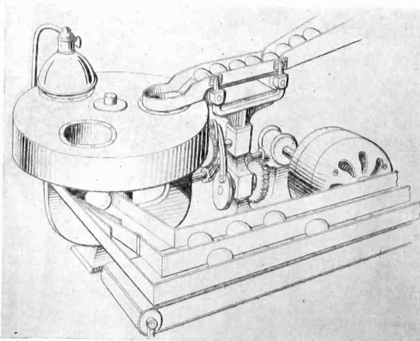
As the eggs reach the photocell, they are supported on a compressed-air cushion which is formed between a steel ring and a rubber ring
