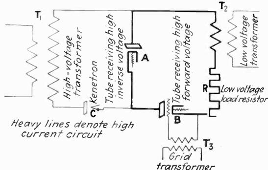
Simplified diagram of "cheater circuit" for testing power tubes
