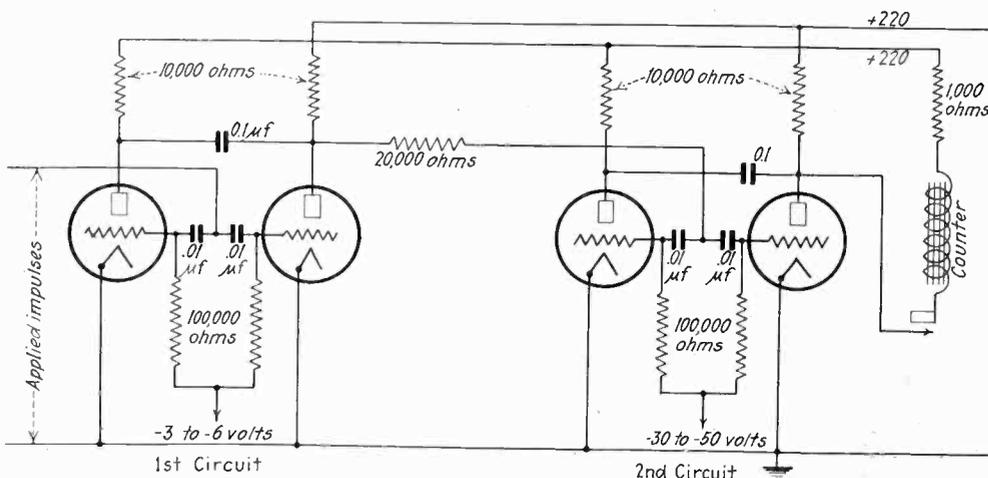
**High-speed counting circuit developed by Williams of the Cavendish Laboratory**
