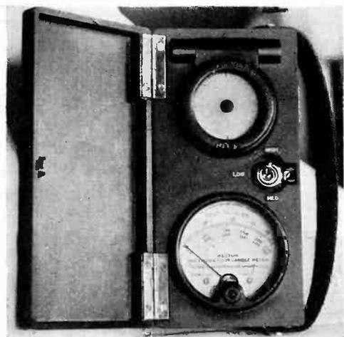
The latest of these is a pocket size photronic foot candle meter, built especially for salesmen's use, calibrated to read directly on three ranges—50, 250 or 500-foot candles.
