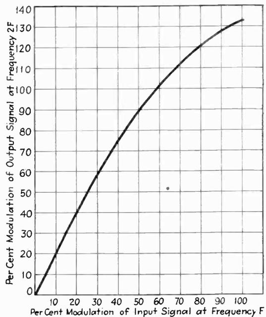
Fig. 4—Curve showing relation between input and output modulation
