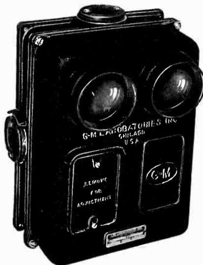
section of the relay entirely independent of front and back covers. The case is of cast aluminum and so designed that the entire unit may readily be weather-proofed for outdoor use. The unit is capable of operating at speeds as high as 600 light interruptions per minute.—*Electronics, July, 1932.*
