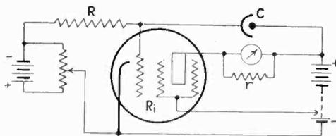
varying light flux. If  $C$  is kept very much larger than  $R$  and sufficient negative grid bias applied, the plate current is equal to  $R_i R (E_p + E_g/C)$ , where  $R_i$  is the internal resistance of the vacuum tube,  $E_p$  and  $E_g$  the plate and grid potentials.—*Canadian Journal of Research, April, 1932.*
