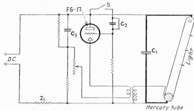
A circuit which produces stroboscopic light for photographic work
