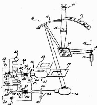
**Motor-generator regulator system.** A speed regulator system using vacuum tubes. W. T. Rea, assigned to A. T. & T. Co. No. 1,861,550.
