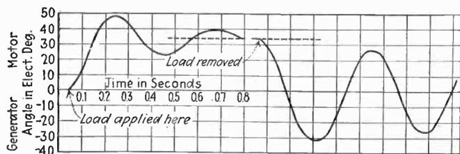
Curve showing the variation of the angular displacement when a sudden load is applied and then removed from a synchronous motor
