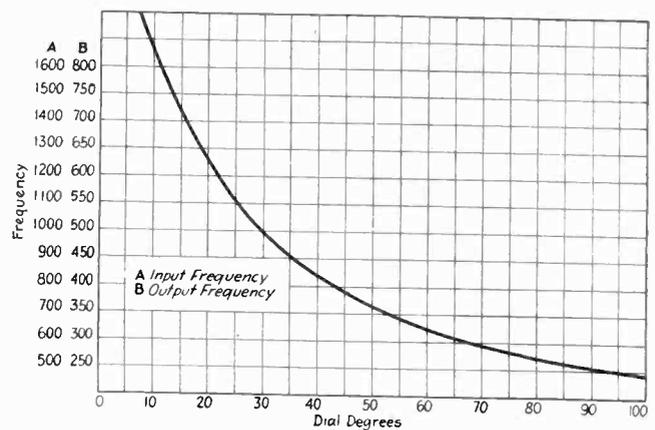
Fig. 2—Calibration of generator showing frequency doubling characteristic
