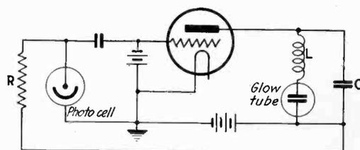
ments, the light produces sufficient feedback to maintain steady oscillations, their strength can be varied by screening part of the light. By using a sector disk or another variable diaphragm the oscillations can be modulated in many ways. A disadvantage of the device is the high resistance of the discharge tube and the distortion at frequencies above 10,000 cycles.—*Zeitschrift techn. Physik, April, 1932.*
