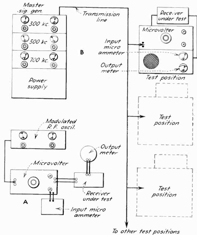
Fig. 6—Set-up for production testing of receivers
