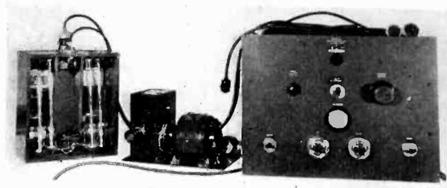
A 480-picture-per-second stroboscopic motion-picture camera
