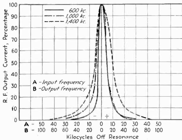
Fig. 3—Microvolter selectivity characteristic
