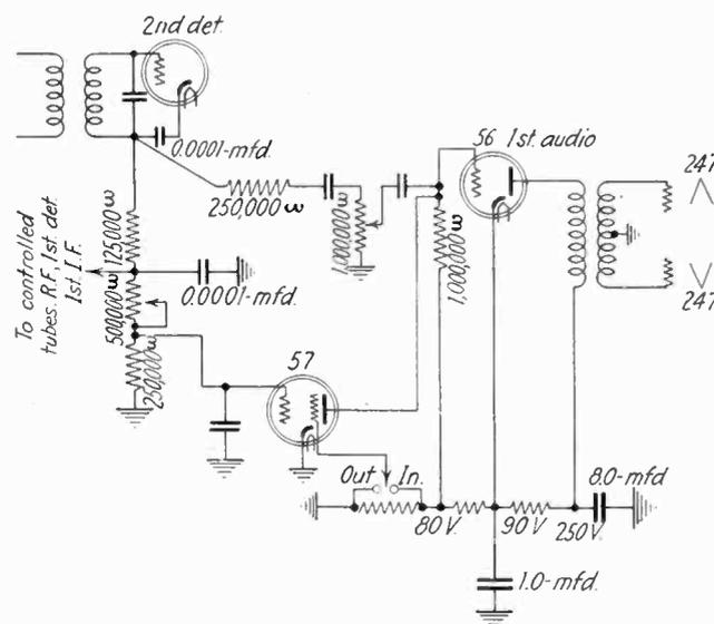
The Fada circuit for muting the audio amplifier between carriers thereby shutting out noise and static
