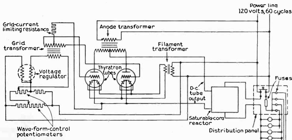
The diagram shows method of arranging Thyatron reactor control circuits for mobile color lighting of a show-window, fountain or other application of color flood-lighting. No moving parts carry load currents, and the dimming is smooth and without energy loss
