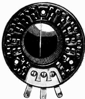
A  $2\frac{3}{4}$  in. circular refractory plate forms the base for the special resistance wire of low temperature coefficient of resistivity. The plate, wire, contacts and terminal connections are thoroughly protected against corrosion and damage by fused-on vitreous enamel.
