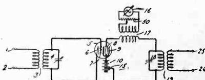
**Fire control.** A light-sensitive cell subjected to rays from a burning film and an electro-mechanical means acting upon the inflammation of the film. W. H. Dewitt. Filed May 5, 1931. No. 1,890,804.
