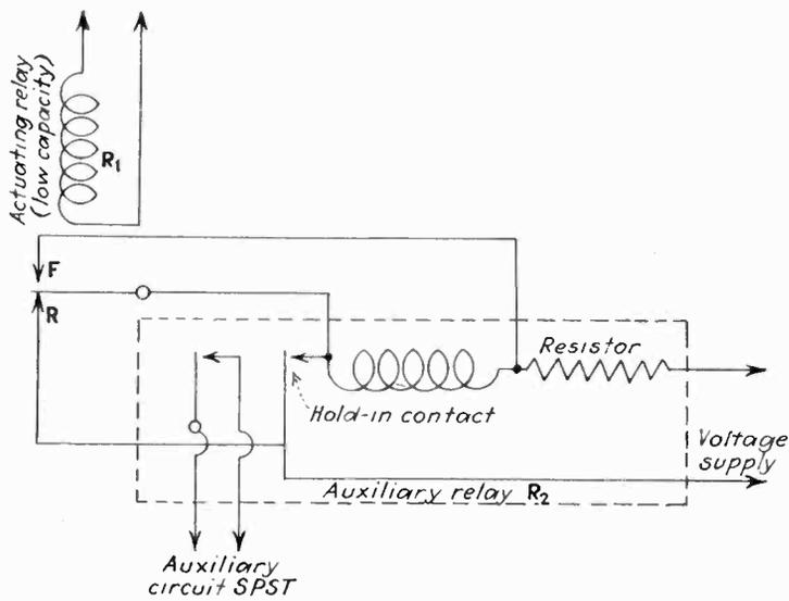
Fig. 3—Auxiliary relay circuit with lock-in feature
