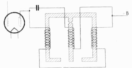
last anode and  $\pm B$ , and take only about  $\frac{1}{2}$  watt. They act as an effective choke for the audio frequencies. The armature coil is connected through a condenser, as shown in the figure.—*Funk Magazin, Berlin, December, 1932.*
