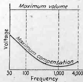
Right—Fig. 4—Voltage frequency characteristic of control
