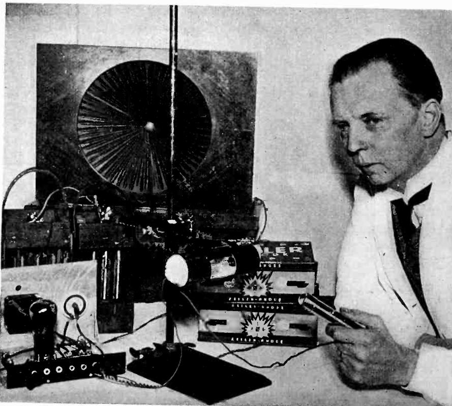
Joachim Winckelmann, Berlin, sends a continuous current through a selenium cell; when light falls on the cell a tone emitted by an oscillator varies in frequency with the intensity of illumination
