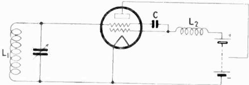
two coils. Other methods of stabilizing this circuit (a resistance in series with the tuning condenser, the division of  $L_1$  into two parts, one placed as now, the other in series with this condenser with no coupling existing between the two parts) are also discussed and experimental results given.—*L'Onde Electrique, Paris, September (published December 5) 1932.*
