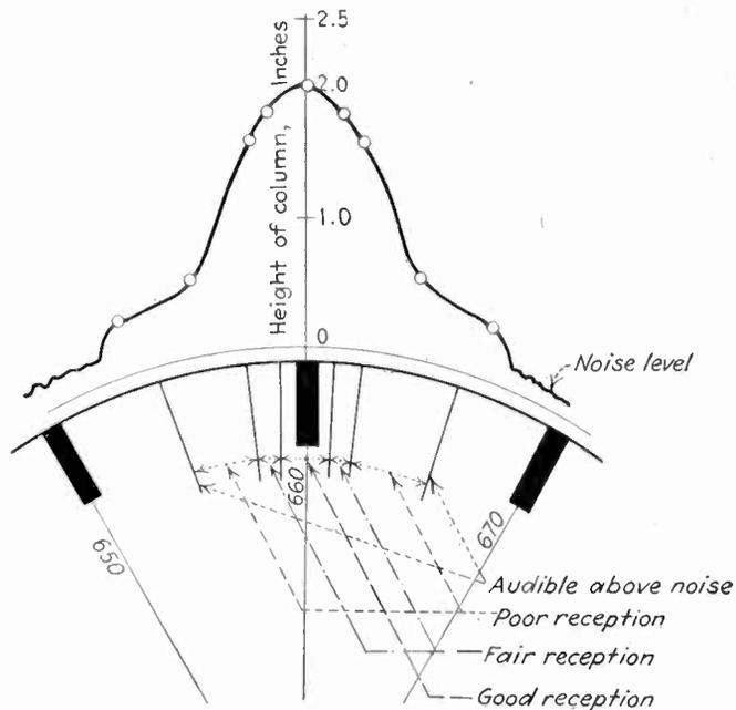
Fig. 3—Action of tuning-indicator on local signal
