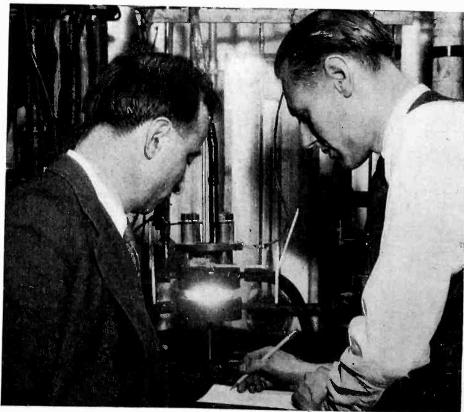
The new Slepian-Ludwig method of controlling a mercury arc by means of a high-resistance rod partly immersed in the mercury pool, was exhibited at the January convention, A. I. E. E.
