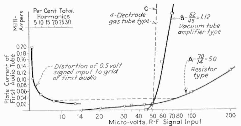
Fig. 6—Characteristics of three noise-gate systems
