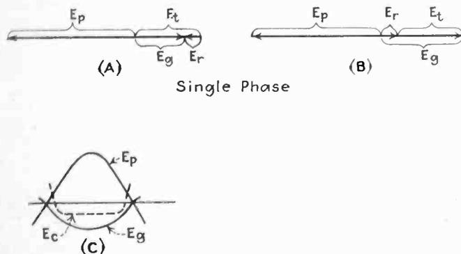
Fig. 4—Single phase circuit conditions preventing flow of current
