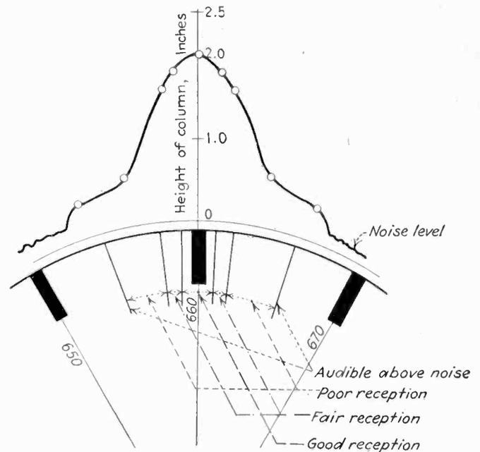
Fig. 3—Action of tuning-indicator on local signal
