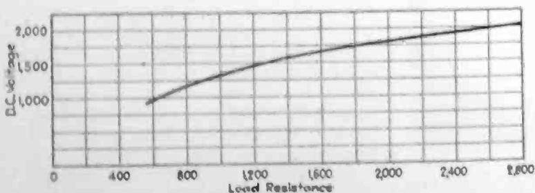
Fig. 2—Regulation curves for Thyratron-controlled rectifier
