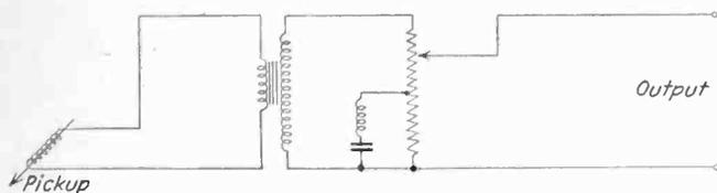
Fig. 5—Circuit diagram of control applied to phonograph
