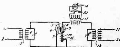
**Fire control.** A light-sensitive cell subjected to rays from a burning film and an electro-mechanical means acting upon the inflammation of the film. W. H. Dewitt. Filed May 5, 1931. No. 1,890,804.
