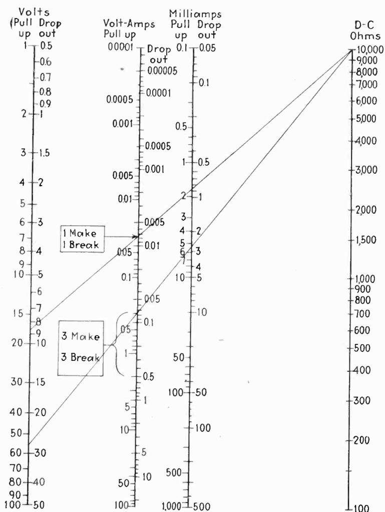
Fig. 1—Nomogram giving essential data on d.c. relays of telephone type. The most sensitive one-make, one-break relay is marked at 0.03; the average sensitivity of more complicated relays is noted. This chart is made on the assumption that the drop-out current or voltage is one half the pick-up, and one-quarter the volt-amperes
