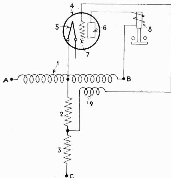
Fig. 1—Elementary diagram of the phase-failure relay
