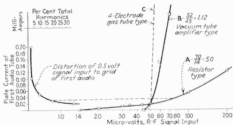
Fig. 6—Characteristics of three noise-gate systems
