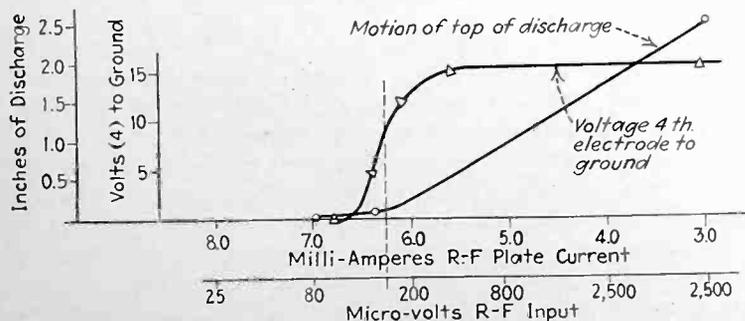
Fig. 5—Characteristics of indicator tube when adjusted to exclude signals below 200 microvolts
