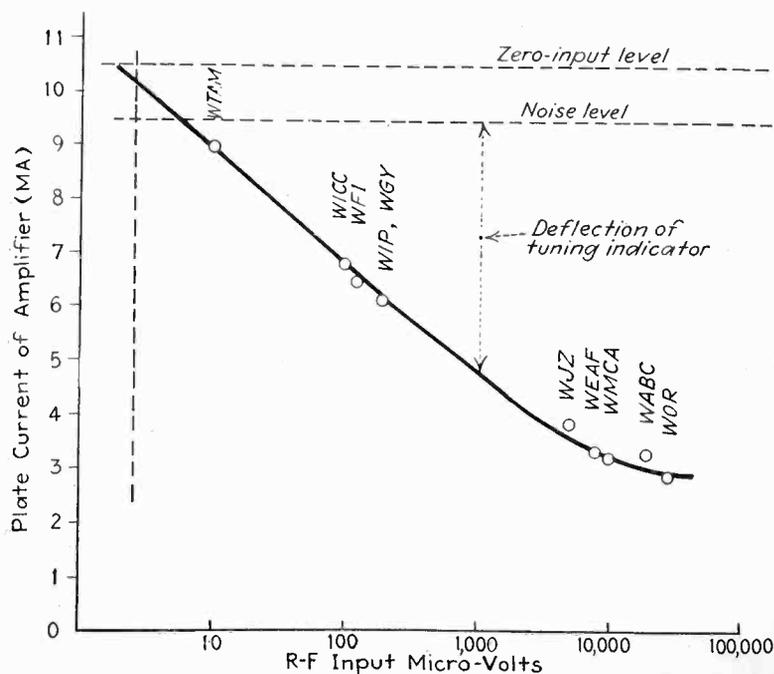
Fig. 1—Plate current variation in nine-tube super-heterodyne. Daytime signals in New York City
