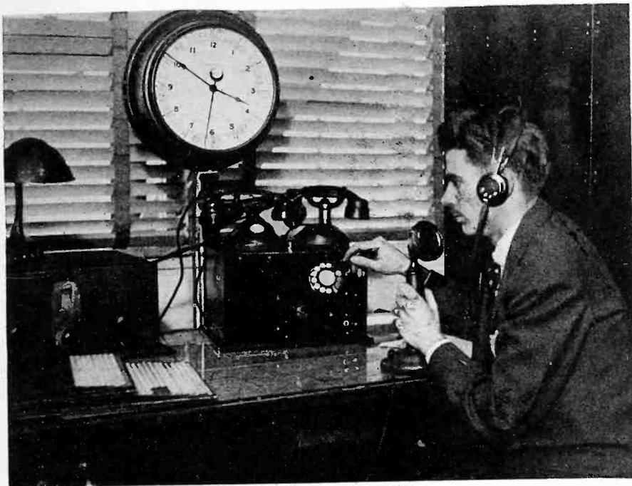
An "automatic dial" selects the wavelength wanted, in this new short-wave set used by the United Air Lines, Chicago. Any one of five or six planes can be reached by dialing its number
