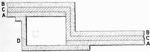
where *A, B* are the two conductors, *C* an insulator, *D* a bridge completing *A* and which can be moved to alter its inductance.—*Funk, Berlin, December 2, 1932.*
