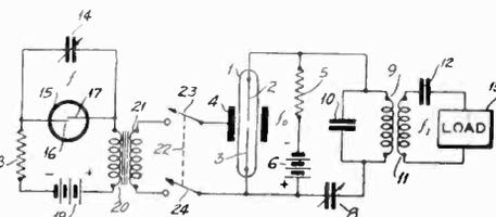
**High-gain amplifier.** A system for obtaining current amplification upward of 1,000,000 by negatively biasing the grid of the tube to such an extent that the positive ion current is predominant and using a resistance for the grid circuit having a magnitude of 1,000 megohms or above. Joseph Razek and P. J. Mulder, Drexel Hill, Pa. Filed Dec. 22, 1930. No. 1,890,750.
