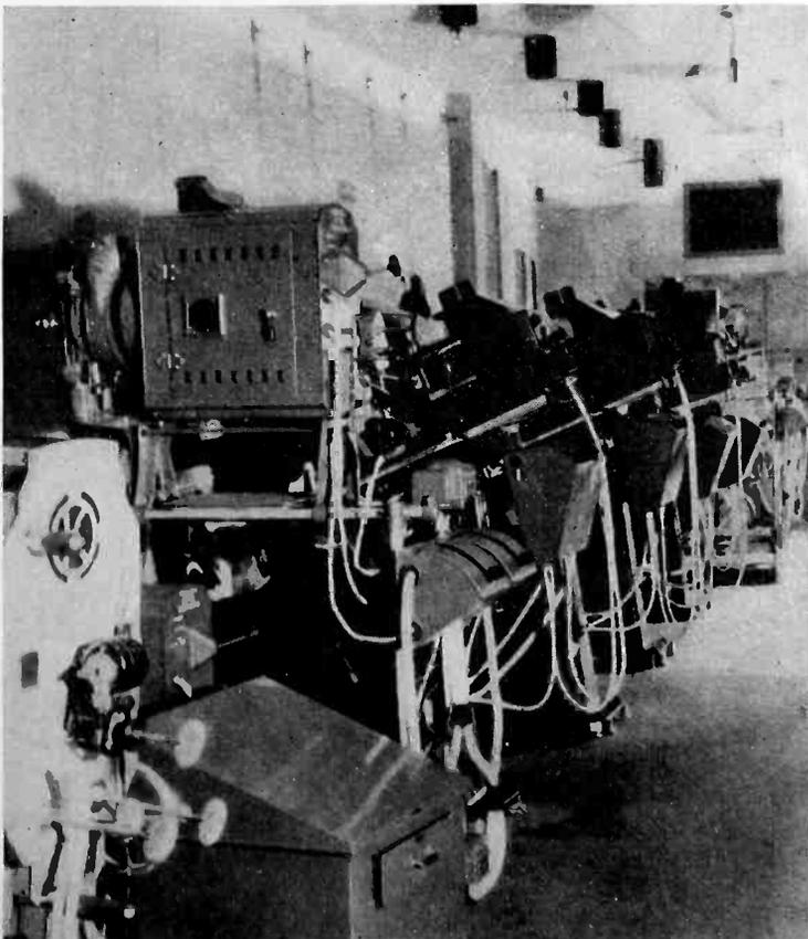
Four sound-picture projectors, with a throw of 180 ft., onto the largest screen ever used
