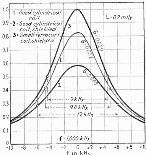
losses occurring in copper. However the new material possesses a considerably greater magnetic conductivity than air so that the amount of copper employed can be decreased and therefore the copper losses avoided.
