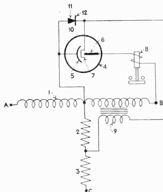
Fig. 5—Use of an auxiliary rectifier in phase-failure relay using cold-cathode tube
