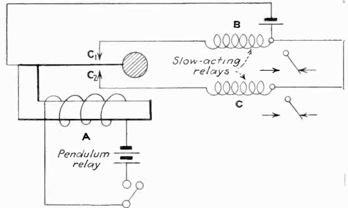
Fig. 2—Pendulum or vibrating reed relay
