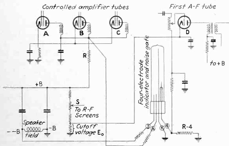
Fig. 4—Circuit of four electrode gaseous tube as tuning indicator and noise gate
