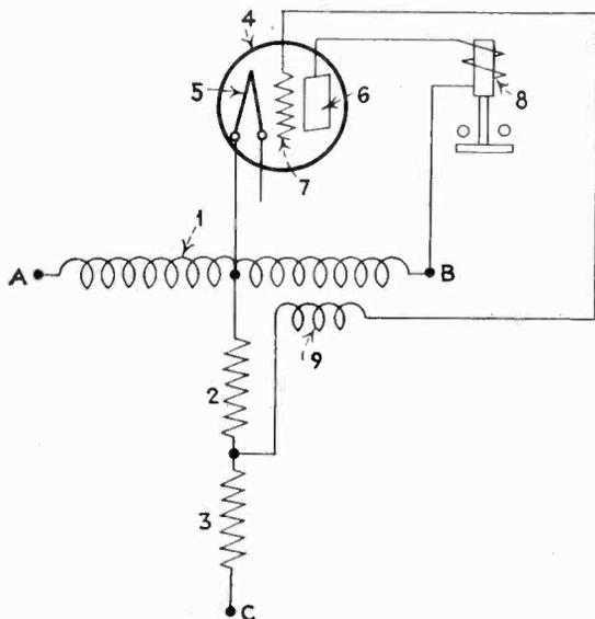
Fig. 1—Elementary diagram of the phase-failure relay
