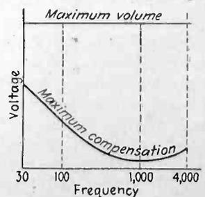
Right—Fig. 4—Voltage frequency characteristic of control
