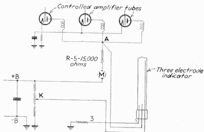
Fig. 2—Essential circuit elements of gaseous discharge tuning indicator
