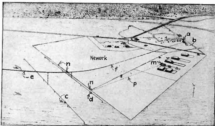
(a) Runway localizing beacon, (b) landing beam, (c) approach marker beacon, (d) boundary marker beacon, (e) spatial landing path followed by landing aircraft, (f) point of contact with the ground, (m) location of monitoring equipment and ground two-way communication set-up, (n) remote control stations for two-way equipment.
