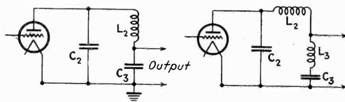
Fig. 4—Improved tank circuits for suppressing harmonic radiation
