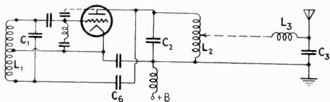
Fig. 3—Line termination effecting reduced harmonic radiation
