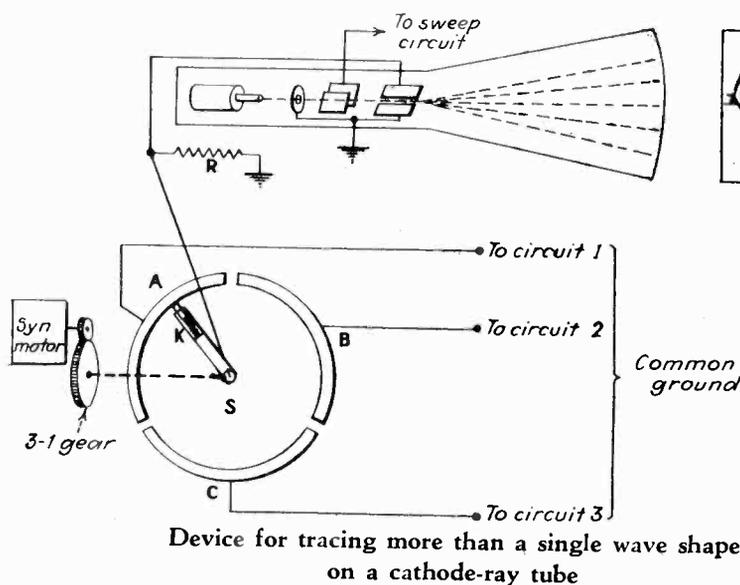
Device for tracing more than a single wave shape on a cathode-ray tube
