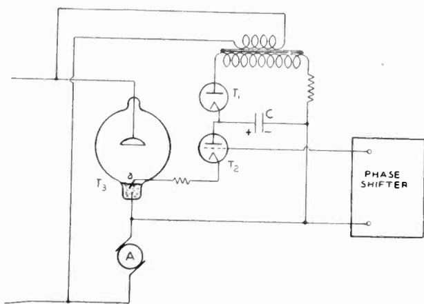
Fig. 4—Use of Ignitron for variable speed control
