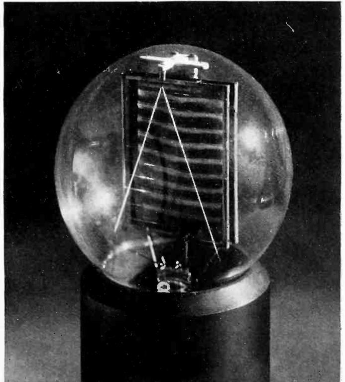
In this huge model of a three-element tube, exhibited by the Bell Telephone Laboratories, the plate is coated with a fluorescent material which glows proportionally to the number of electrons which come from the filament.
