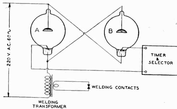
Fig. 5—High speed, high current spot welder controlled by the new tube
