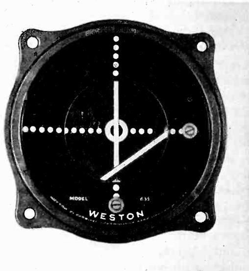
Fig. 2—Combined instrument used for securing lateral and vertical position of the landing aircraft
