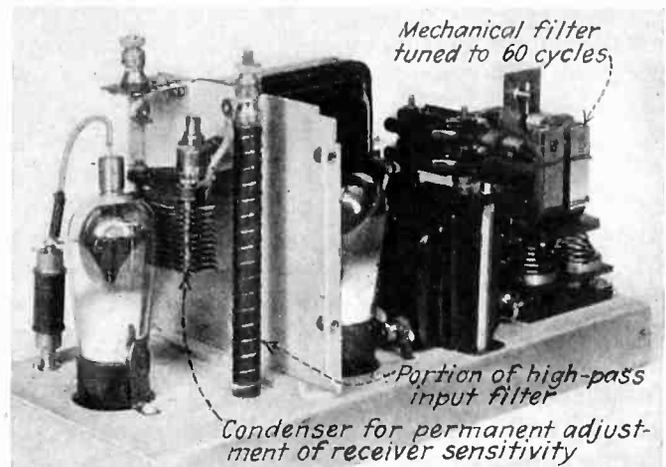
Fig. 4—Exposed view of landing beam receiving set
