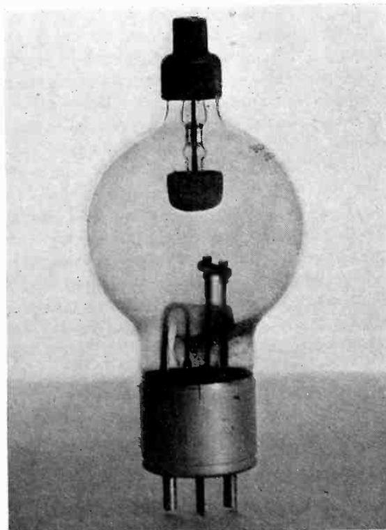
Fig. 3—The Ignitron, a new controlled rectifier
