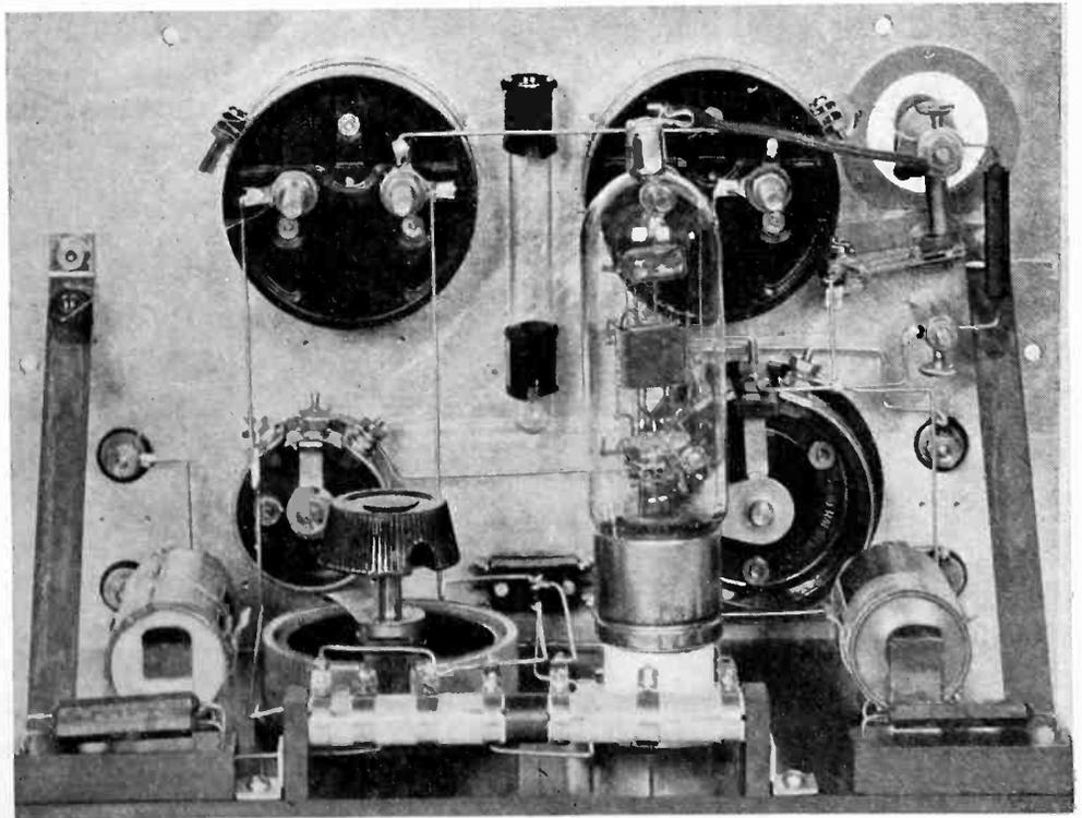
Rear view of an amplifier for measuring resistances up to a 1,000,000,000 ohms with only about one volt impressed
