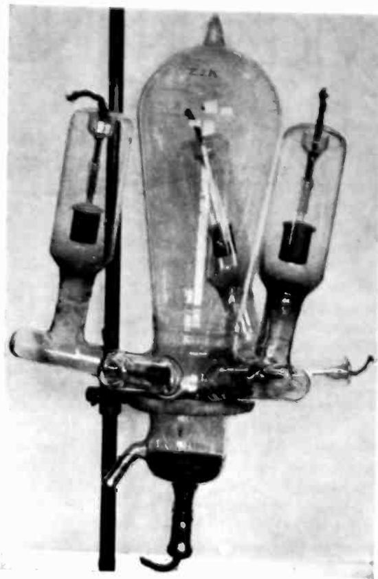
Fig. 2—A three-phase mercury pool rectifier of conventional type
