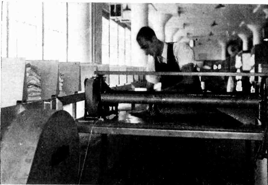
At the left is seen the conveyor belt with its compartments. A light-beam and photo-cell advance the conveyor, if nearest compartment is empty.
