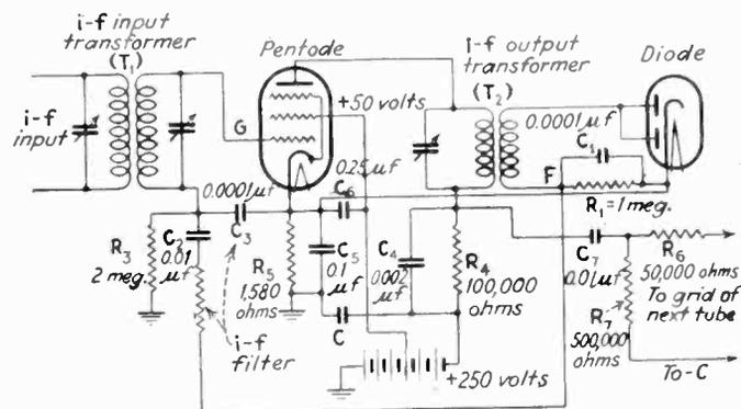
Fig. 1—Typical reflex circuit. In this case the diode and pentode are distinct; they may be combined in a single envelope, such as the 6B7
