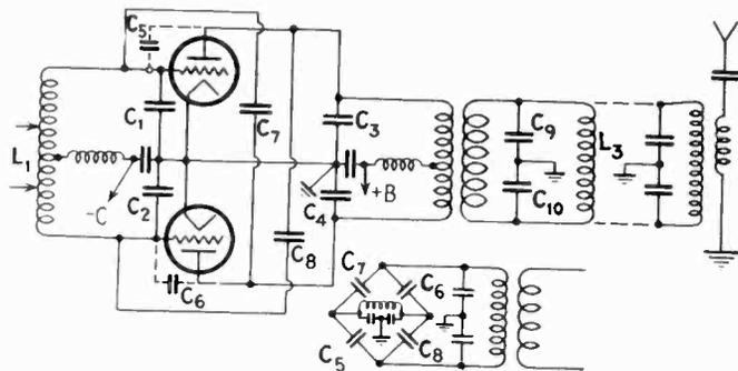
Fig. 2—Push-pull amplifier with high kva. tank circuit in transmission line
