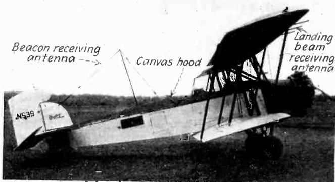
Fig. 5—Airplane used in hooded landings
