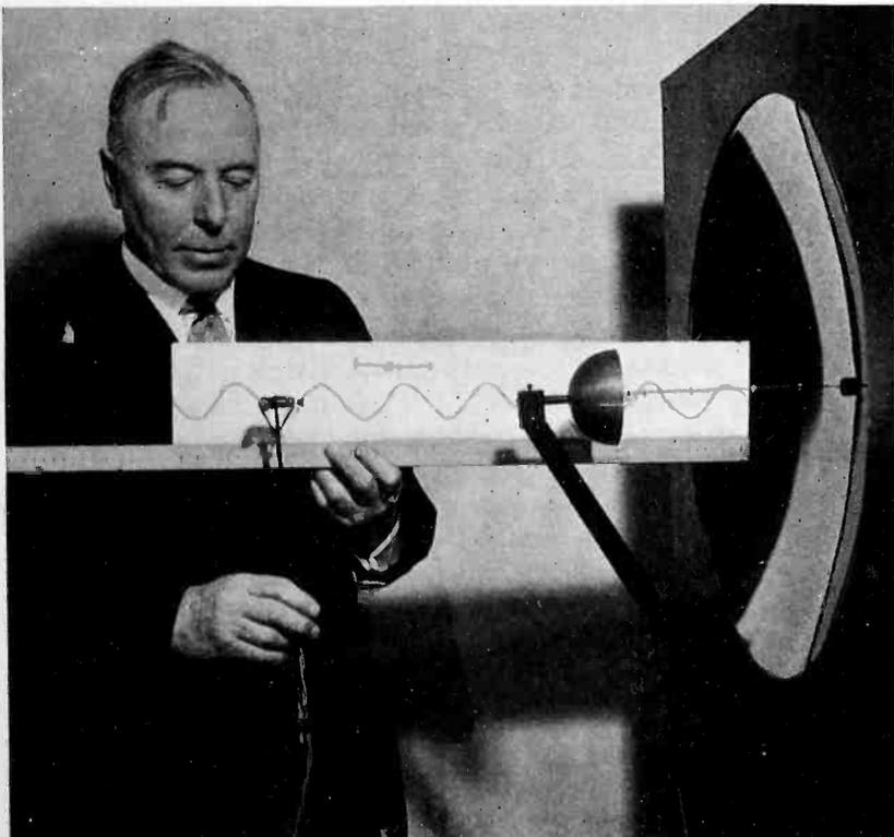
An ultra-shortwave generator producing 9-centimeter waves, is shown having its output measured by Dr. S. M. Kintner, vice-president and chief engineer Westinghouse company. The output of one watt of power can be reflected like light, but penetrates smoke and fog unimpeded.
