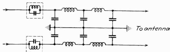
Fig. 7—Low pass filter combined with antiresonant circuits in transmission line
