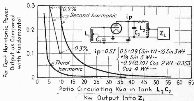
Fig. 5—Effectiveness of high kva.-kw. ratio in reducing harmonic output with constant power output at fundamental
