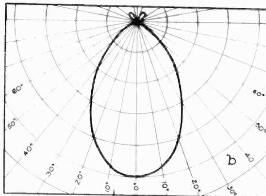
Fig. 6—Shape of landing beam (a) vertical directive pattern, (b) horizontal directive pattern
