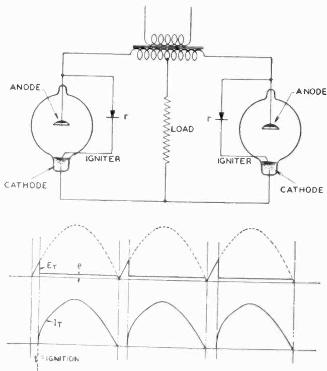
Fig. 1—Full wave single phase rectifier using the new tubes
