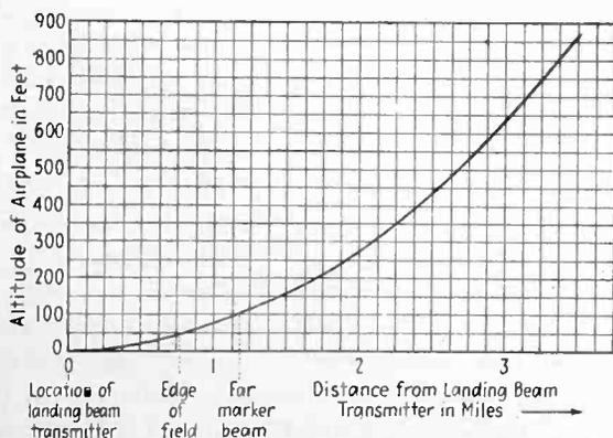
Fig. 3—Circuit of ultra-high frequency landing beam transmitter and landing path at the Newark Airport. No variations in this path have been noted during two months of intensive tests
