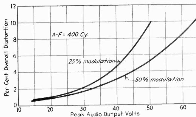
Fig. 3—Distortion from the reflex circuit and tube showing decrease at higher modulation due to weaker necessary i-f signal
