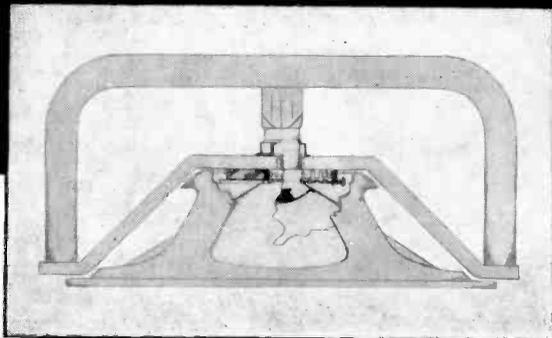
**W**ITH a domed center cap that completely shields the air-gap and voice-coil, and a radically new corrugated diaphragm type centering member, and acoustic filter assembly, Rola's new PM DYNAMIC speakers attest the skill of Rola technicians in pioneering new fields of loudspeaker engineering.
