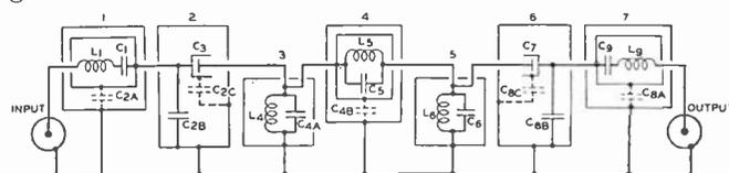
Fig. 8—Final filter circuit with desired characteristics
