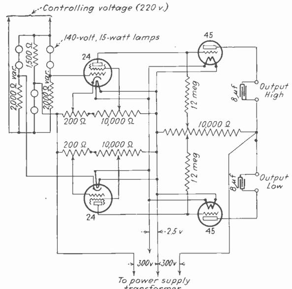
Fig. 6—Double-acting electronic voltage relay
