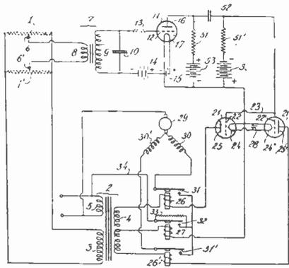
**Dual band system.** An amplifier system adapted for operation in more than one band of frequencies. C. J. Franks, assigned to R. F. L. No. 1,943,790.
