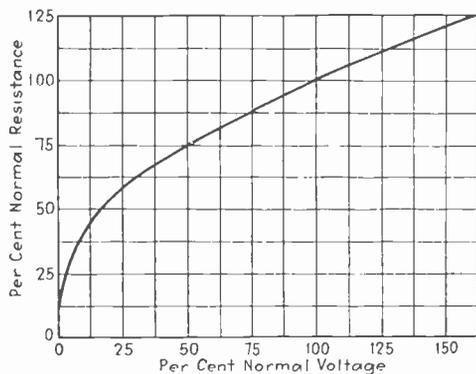
Fig. 2—Voltage-resistance curve—25 watt tungsten lamps
