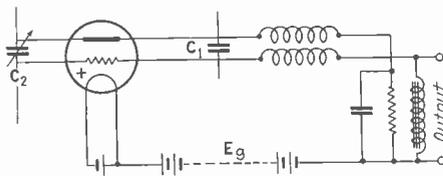
Ultra-short wave circuit with output in grid-filament path
