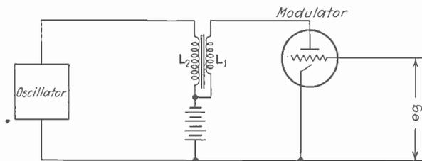
Fig. 3—Modified constant current system
