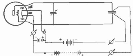
and grid inductance. The negative end of the A battery is joined to the negative of the B battery and the positive of A to the positive of C.—*H. F. Techn. El. Ak.* 43:12-15 January, 1934.
