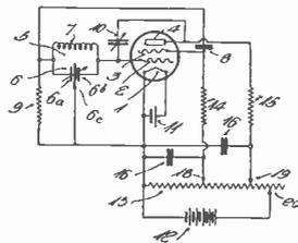
**Copper oxide rectifier.** Circuits for use in radio receivers. W. P. Place, assigned to Union Switch and Signal Co. No. 1,937,783 to 1,937,785, inclusive.
