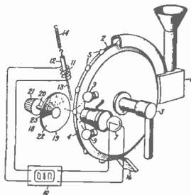
**Light control.** Photoelectric system for regulating the amount of illumination in a given area contributed by several light sources. F. W. Lyle, W. E. & M. Co. No. 1,944,751.
