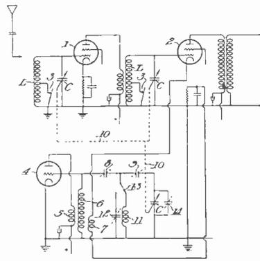
**Navigation system.** A radio system comprised of two co-planar coil antennas connected in series, an independent coil connected at right angles, electron tubes, etc. J. A. Willoughby, Washington, D. C. No. 1,942,526.
