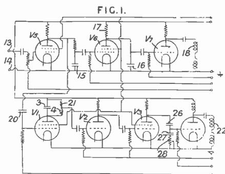
**Automatic tone control.** Combining manual tone compensation applied to the low-frequency stages of a receiver in combination with automatic volume control applied to the high-frequency stages, with the object of correcting the natural tendency of the ear to accentuate the middle frequencies as compared with the higher and lower notes, particularly at a low level of sound-output. L. E. Barton, Marconi Co. No. 397,763.
