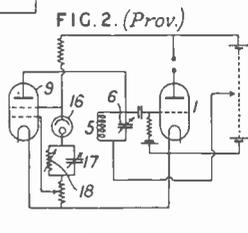
**Phase modulation.** Two components of the same carrier wave phase displaced by 90 deg. are radiated simultaneously from separate aerials after being modulated by signal currents in phase opposition. For reception it is necessary to supply a local oscillation of the same frequency, but de-phased from the incoming carrier so that the signals cause minimum interference with any normal type of receiver. G. W. Walton, London. No. 400,273.
