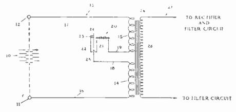
**Phase shifting device.** An electron tube method of continuously shifting the phase of an alternating current. W. A. Marrison, B. T. L., Inc. No. 1,942,483.
