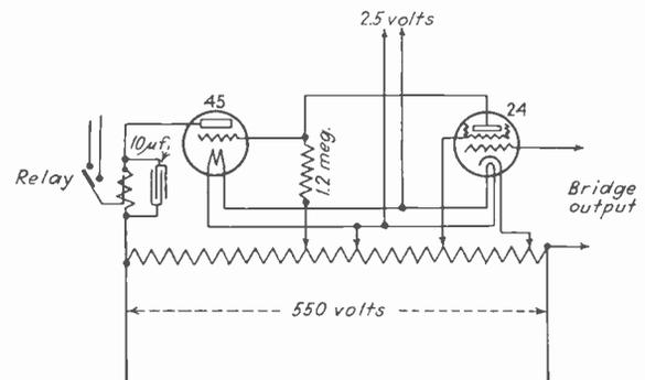
Fig. 4—Elementary diagram of voltage relay
