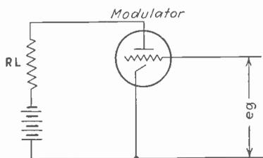
Fig. 2—Equivalent circuit of modulation circuit
