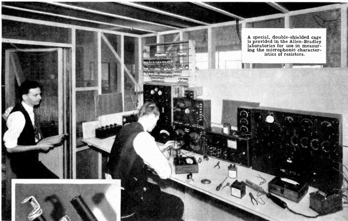
A special, double-shielded cage is provided in the Allen-Bradley laboratories for use in measuring the microphonic characteristics of resistors.
