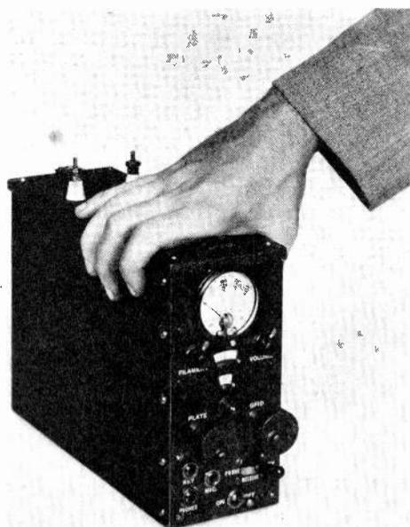
Compact 5-meter receiver-transmitter (RCA) for portable use
