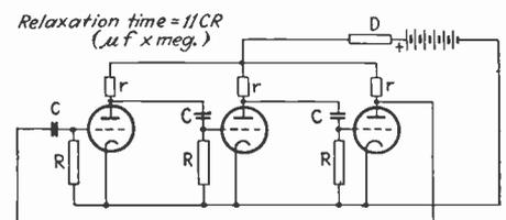
Source of sinusoidal oscillations.
