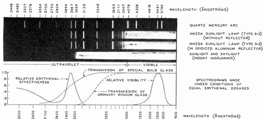
Wavelengths emitted by various light-sources; absorption by glass materials, and points of greatest eye and skin sensitivity.
