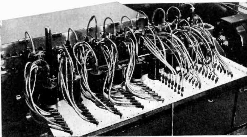
Over 150 Erie Suppressors are being continuously subjected to load tests under various conditions of temperature and humidity on this life testing equipment. With the exception of very short intervals when suppressors are inserted or removed, this machine has been running continuously day and night for an equivalent of over 650,000 miles.
