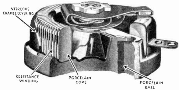
The cross-section picture shows several of the exclusive features of Ohmite all porcelain rheostats—solid porcelain core—vitreous enamel bond between winding, core, and base—no organic material to smoke or char—flat contact surface—large number of contact steps—shafts insulated against high voltage.
