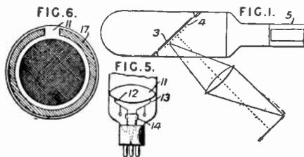
cooled by a surrounding layer of cotton wool on to which liquid air is poured. The helix and the screen are removed, and the tube is baked and evacuated and the silver deposits are then oxidized by passing a high-frequency discharge
