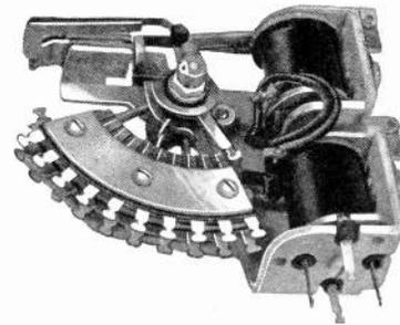
The Autelco Minor Switch can be used to select any desired contact of a group of ten, control being accomplished by push button, telephone dial, etc. Switch is operated and restored by electromagnets. One, two or three levels can be furnished, ten contacts per level, with one, two or three non-bridging double-spring wipers. Arrangements can be made for operation on from 6 volts up to 110 volts, D.C. Current-carrying capacity per wiper, at rest—3 amperes, D.C. or A.C.
