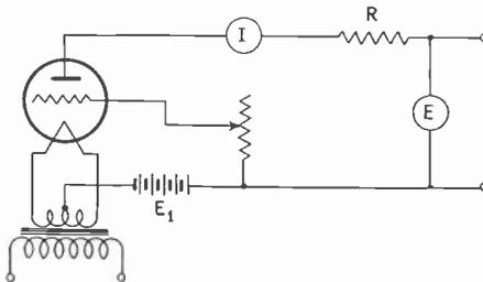
Fig. 3—"Holding-arc" circuit, using FG-57 thyatron.
