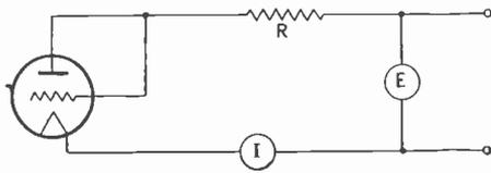
Fig. 1—Circuit for determining characteristics of rectifiers.
