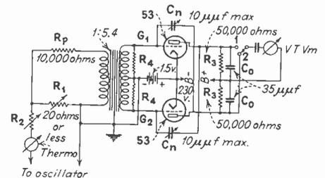
Fig. 1—Circuit diagram of neutralized push-pull audio amplifier.
