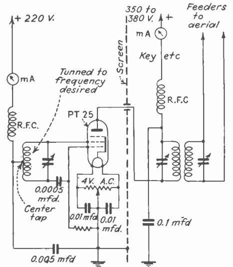
Electron-coupled oscillator for short-wave transmission.
