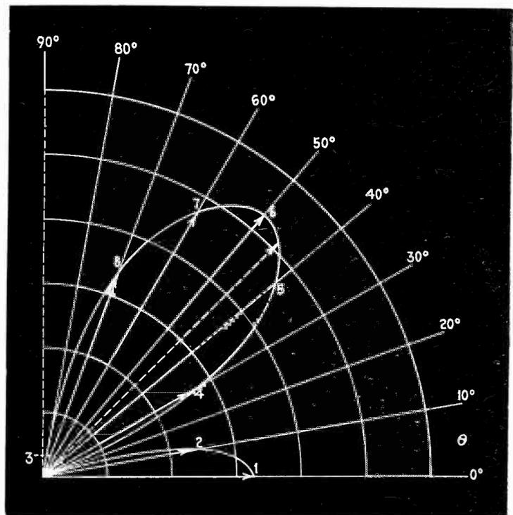
Fig. 8—The polar plot of field intensities for the case illustrated in Fig. 7, i. e., an antenna operated at its third harmonic. The large amount of high angle radiation in this case is clearly indicated
