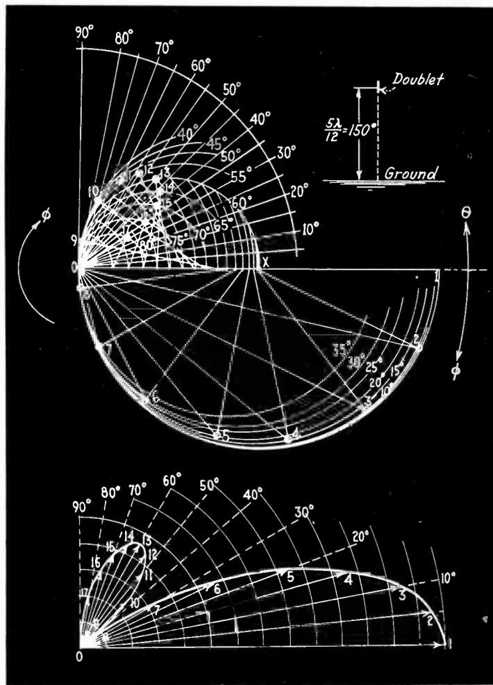
Fig. 6. Solution of a doublet located  $\frac{5}{12}$  wave-length above ground, in which a lobe of high angle radiation appears. The construction is the same as that of Fig. 5, except that  $\phi$  has values larger than  $180^\circ$
