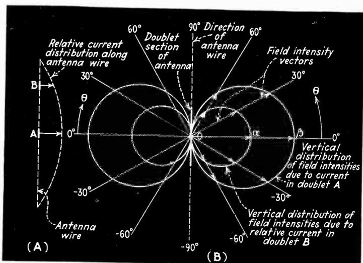
Fig. 1. (A) Typical vertical antenna, showing the current distribution and two doublets. (B) Field intensities radiated from doublets A and B at various angles above and below the horizon
