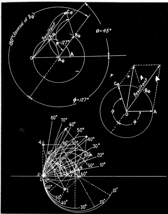
Fig. 7. Sample construction for the case of a vertical antenna operated at its third harmonic, described in text
