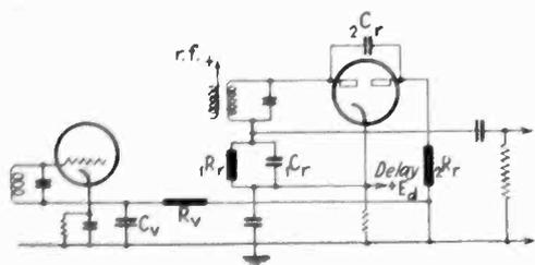
**Delayed a.v.c.** One plate of double diode is less negative than the other by the voltage across  $E_a$
