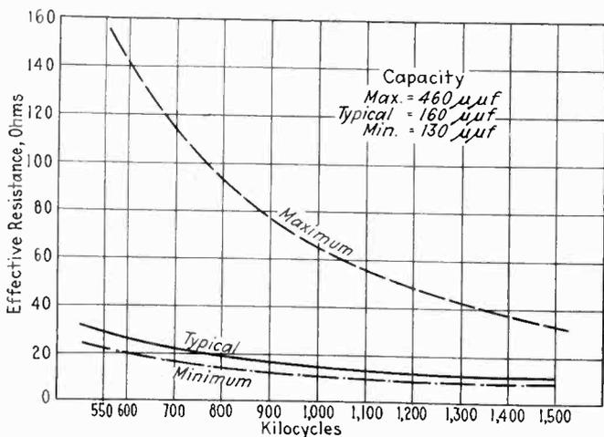
Fig. 3—Resistance characteristics of typical roof antennas
