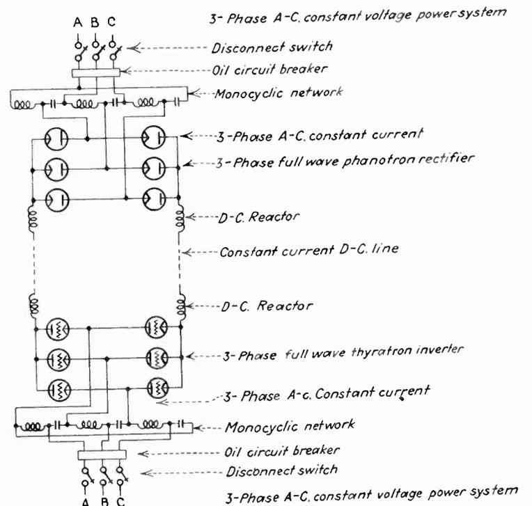
Block diagram of direct-current transmission system
