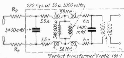
Equivalent network of modulation transformer
