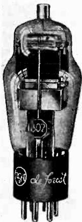
The plate lead is taken out at the top. The losses in the base are thus reduced to about 250 milliwatts at 5 meters. Following are typical operating characteristics:
