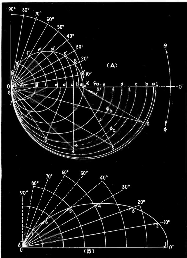
Fig. 5. Complete solution of the case shown in Fig. 4 (A), i. e. a doublet located one quarter wave above ground. (A) is the working diagram, whose construction is completely outlined in the text, while (B) is the polar plot of field intensities, the answer to the problem
