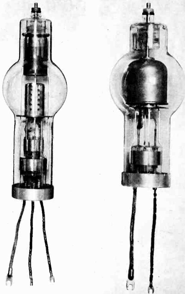
Types of Thyatron and Phanotron tubes used
