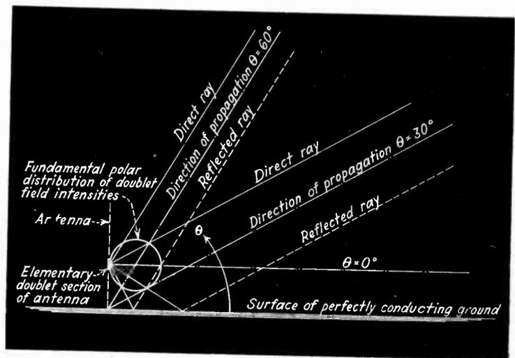
Fig. 2. A doublet located above a perfectly conducting ground. The reflections from the ground combine with the direct radiation, causing wave interference
