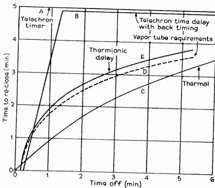
Fig. 1. Comparison of the re-closing characteristics of thermal, mechanical, and thermionic types of relay with the reheating characteristic of a vapor tube
