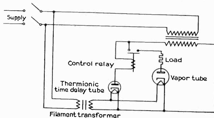
Fig. 2. Typical circuit diagram showing use of thermionic relay for cathode protection
