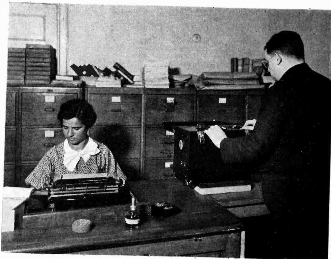
Analyzing office noise. Dr. E. E. Free, treasurer of the Acoustic Society of America, demonstrates how the noise of a standard typewriter can be measured by his portable noise-meter, for comparison with silent typewriter model
