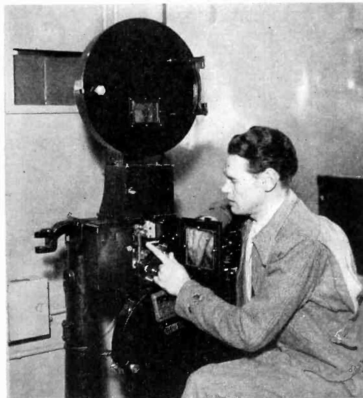
Station KFVB, Hollywood, Cal., has arranged this sound-picture projector element as a pick-up for broadcasting transcriptions from sound-on-film recordings. Music and voices from standard feature films are being broadcast. United Research Laboratories adapted the machine for the Warner Brothers station
