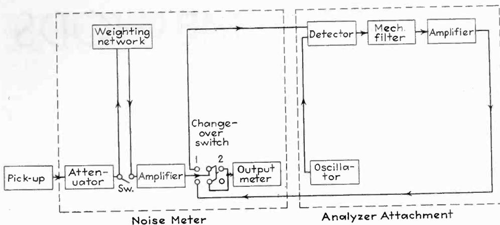
A typical noise meter and analyzer circuit diagram. With change-over switch in position 1, the noise can be analyzed. In position 2, total noise is measured
