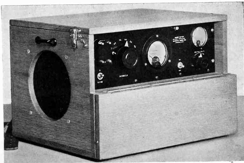
A typical noise meter intended for industrial use, developed by General Radio. The circular opening admits the sound to a magnetic microphone, the amplified output of which is indicated on the db meter
