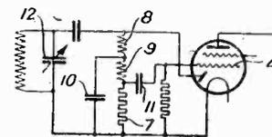
of a diode-triode, comprises a resistance in series with two equal but oppositely-wound chokes. This prevents damping of the input circuit. Philips. No. 420,476.
