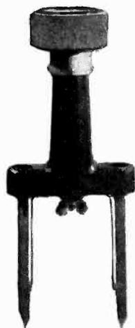
strument a double-purpose tester, is of the thumb-screw type and is located between the two cadmium-plated battery prods.
