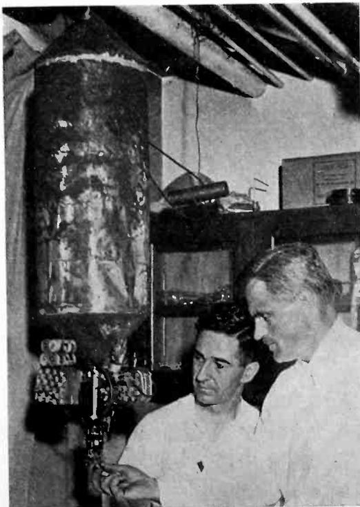
Ionization chamber with complete radio transmitter attached. Prof. J. M. Benade is assisting Dr. Compton
