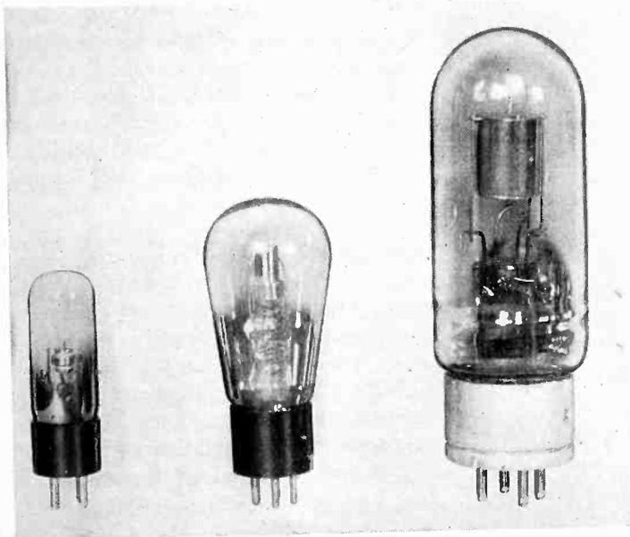
Fig. 3. Three types of thermionic relay tubes, for 5, 10, and 30 minute characteristics
