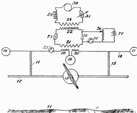
influenced by any change in distance between the aircraft and the earth and cause the oscillatory circuits to become non-resonant and produce a beat note, with means for measuring the beat note to calculate the change of capacity to measure the distance. R. A. Fessenden, Chestnut Hill, Mass. Application Jan. 18, 1922, 1 claim. No. 1,991,892.
