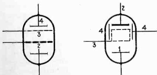
Head-on and wall type gas tubes
