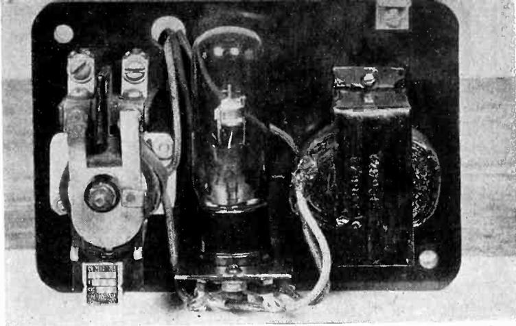
Fig. 4. Complete delay timer with thermionic tube in place
