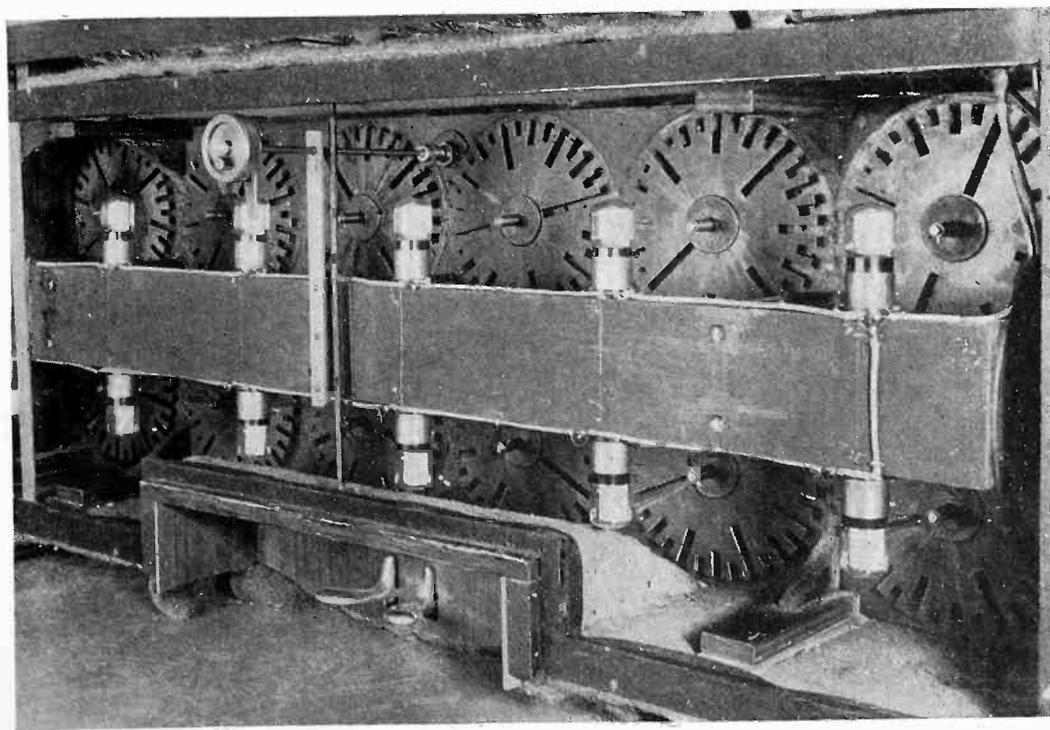
A front view of the WCAU Photona, showing the tone-shutter disks in complete detail. These disks revolve, and as the lights are switched on by the keys, the light beams flash through the shutters to the photo-electric cells and produce the tones of the instrument
