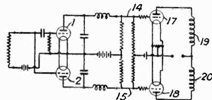
coupled so that the sign of the voltage difference between points 14 and 15 depends on the magnitude of the alternating voltage applied to their input. G. E. Co. No. 419,978.
