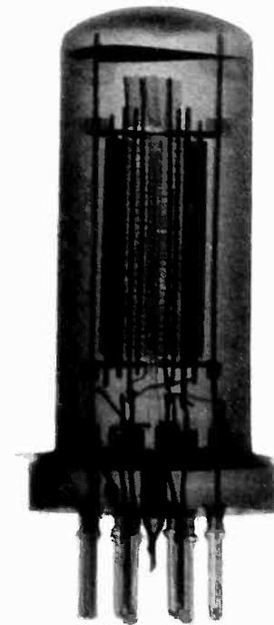
*X-ray examination has been extended to metal radio tubes, providing a non-destructive check on alignment of the elements after assembly, exhaust etc.*
