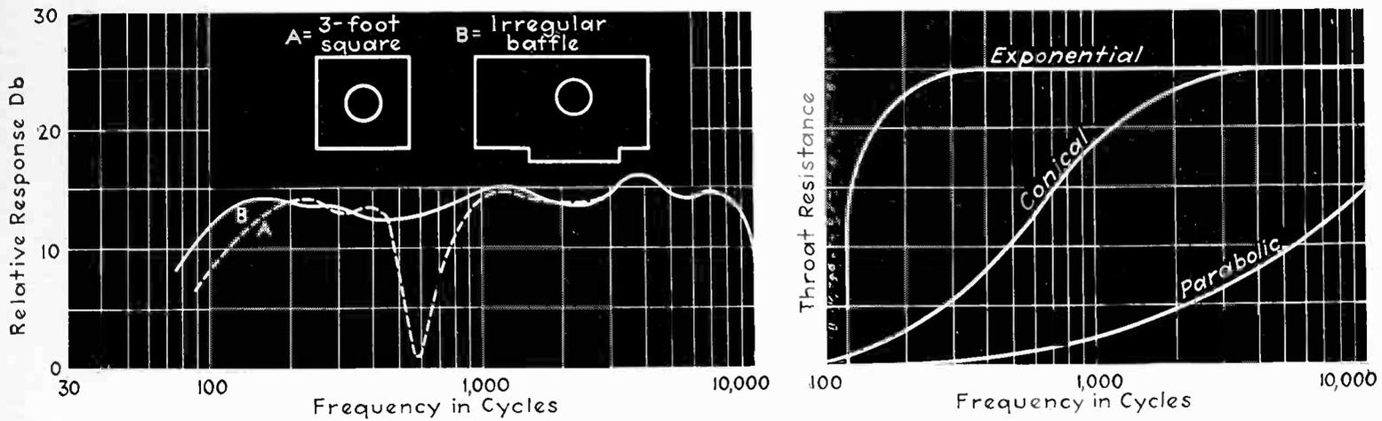
Fig. 4. Response curve of a double voice coil speaker taken at a distance of 10 feet. Figure 5 (right) Infinite horns having same throat areas and same areas at distances along their axes equal to 100 times the throat diameter
