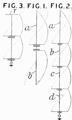
than half the working wavelength. The average overall current is at least 0.7 of the maximum current, while the current at all points of at least one element exceeds 0.5 and may reach 0.9 of the maximum current. H. L. Kirke, London. No. 436,254.
