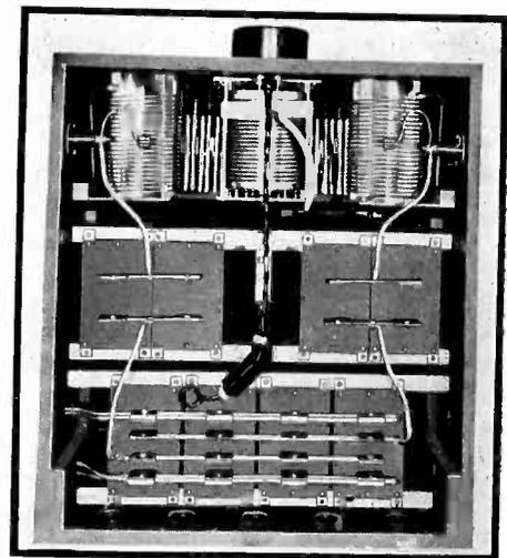
variable frequency, primary exciter circuit which is tuned and coupled to a low loss tank circuit. Its overall dimensions are 23½ in. front, 25½ in. deep and 37½ in. high.
