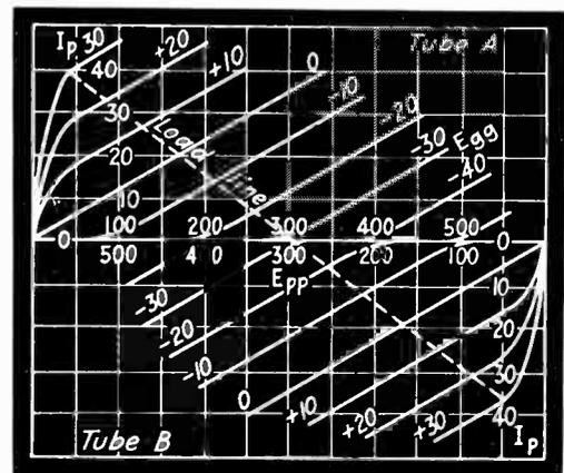
Fig. 3—Composite  $I_p$ - $E_p$  characteristics of Class B unit
