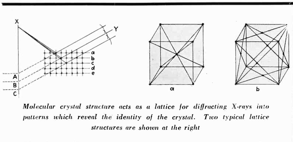
*Molecular crystal structure acts as a lattice for diffracting X-rays into patterns which reveal the identity of the crystal. Two typical lattice structures are shown at the right*
