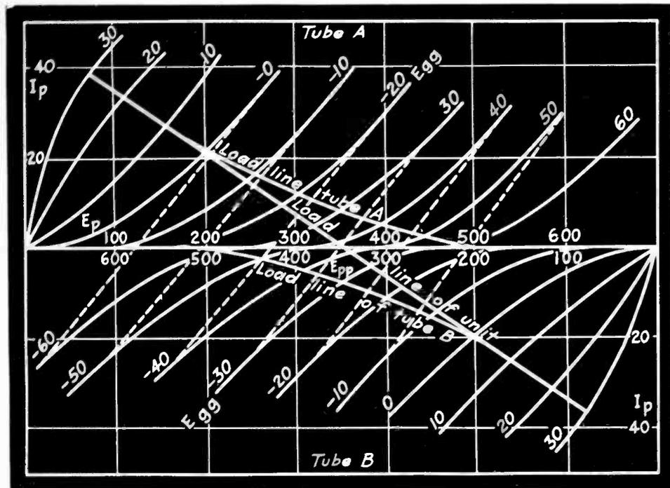
Fig. 4—Composite characteristics of Class AB amplifier
