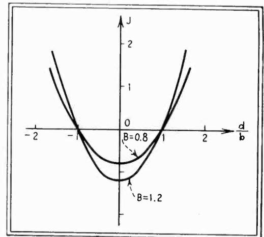
Master parabolas for the design of band-pass filters
