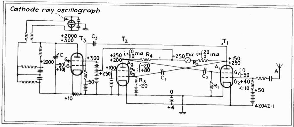
Electronic relay for tripping cathode-ray time sweep within 0.2 microseconds after the impulse is applied. The lower of the two figures given for plate and grid voltages is the value immediately after the impulse has appeared
