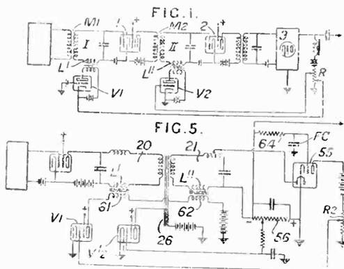
or more frequency-selective circuits. The d-c voltage may be applied to the grids of tubes the plate currents of which vary the degree of saturation of the iron cores of coils in the tuned circuits. R. A. Braden, Marconi Co. No. 436,482.
