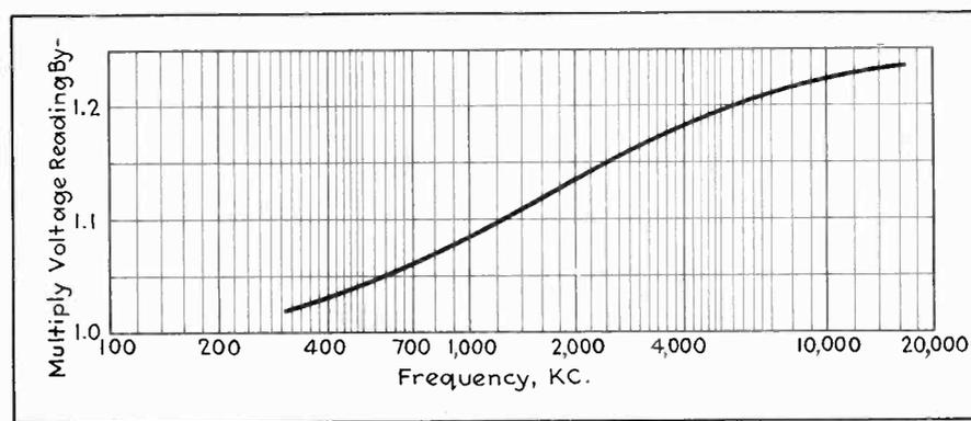
Fig. 2A—Calibration correction factor for peak-reading voltmeter
