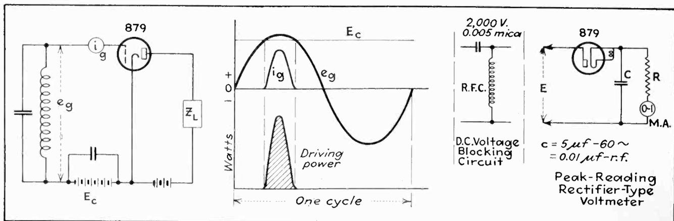
Fig. 1—Fundamentals of r-f power amplifier and details of rectifier voltmeter
