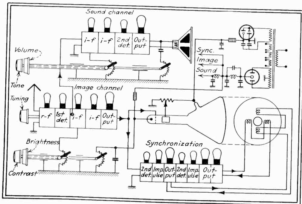
Schematic diagram of new Telefunken television receiver. Note separation of image and voice frequencies after first detector
