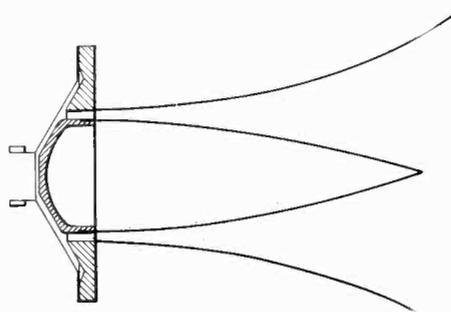
Fig. 8. Annular throat construction to reduce interference at the high frequencies
