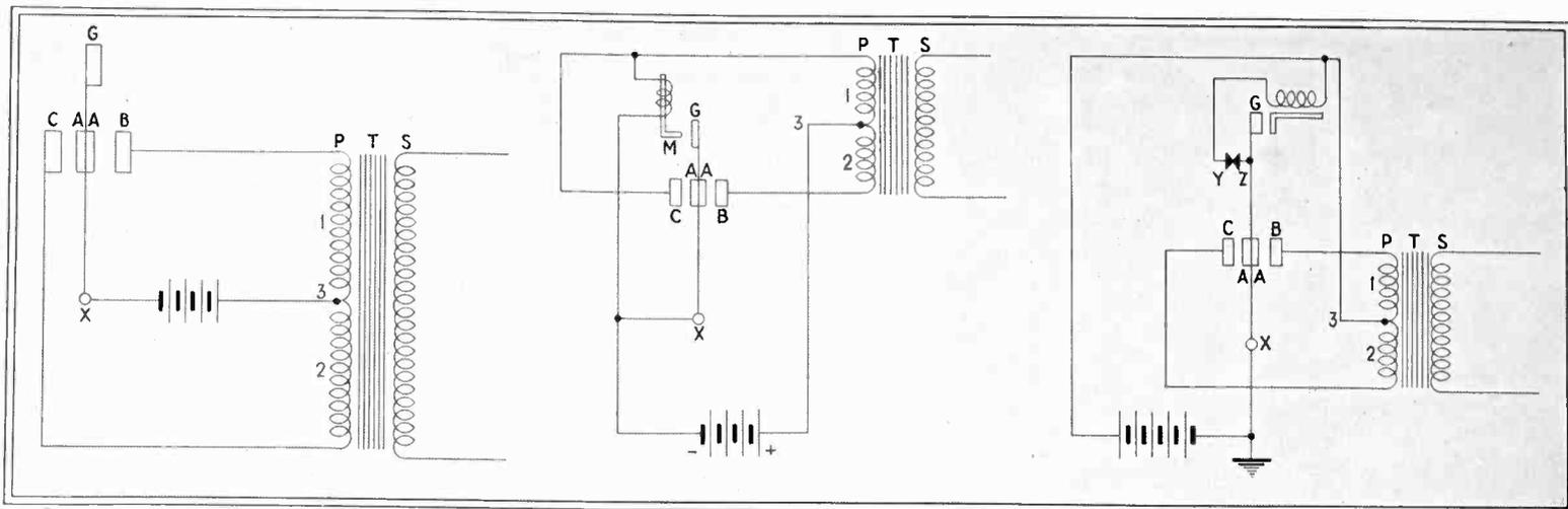
Fig. 1—Series type vibrator circuit. Figs. 2 and 3—Shunt circuits (Data from Radiart Service Course)
