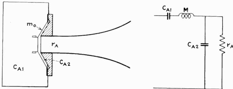
Fig. 6. Horn loud speaker and equivalent electrical circuit
