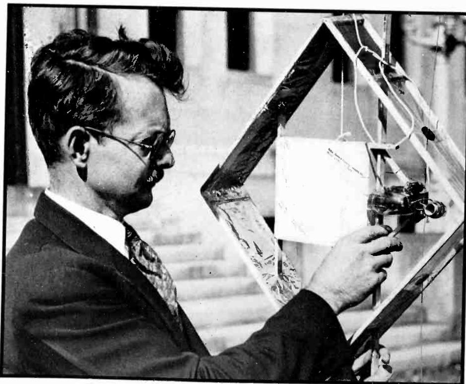
Dr. L. F. Curtis of the U. S. Bureau of Standards with a radio transmitter for attachment on meteorological balloons. A range of 80 miles at a height of 14 miles can be attained
