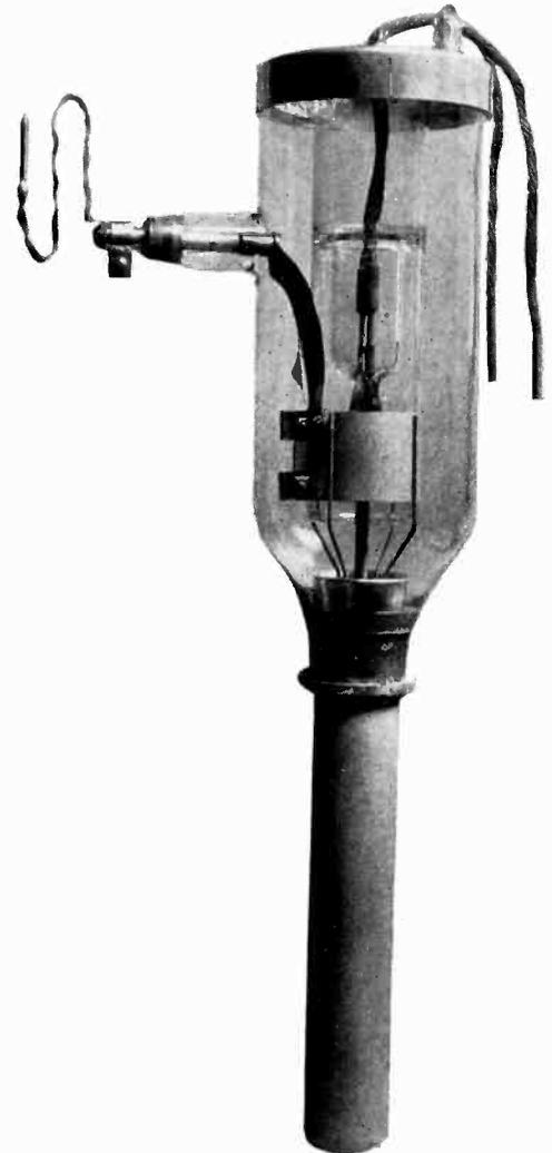
*Rigid control of materials and processing is necessary to insure tubes costing as much as \$500, such as this WL-207*
