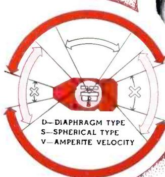
\* Diagram shows angle of pickup without frequency discrimination of various types microphones.
