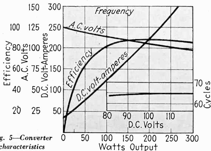
Fig. 5—Converter characteristics
