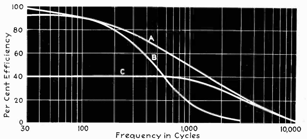
Fig. 7. Efficiency of horn type speaker driven by diaphragm having an effective mass of 2.5 grams and an area of 120 sq.cms.
