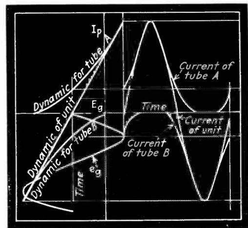
Fig. 5— $I_p-E_g$  dynamic characteristics of Class AB amplifier
