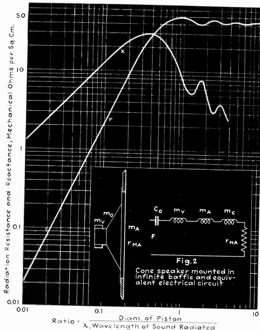
Fig. 1. Radiation resistance ( $r$ ) and reactance ( $x$ ) of a piston mounted in an infinite baffle
