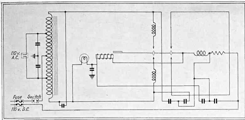
Fig. 4—Circuit of Electronic Laboratories d.c.-a.c. converter
