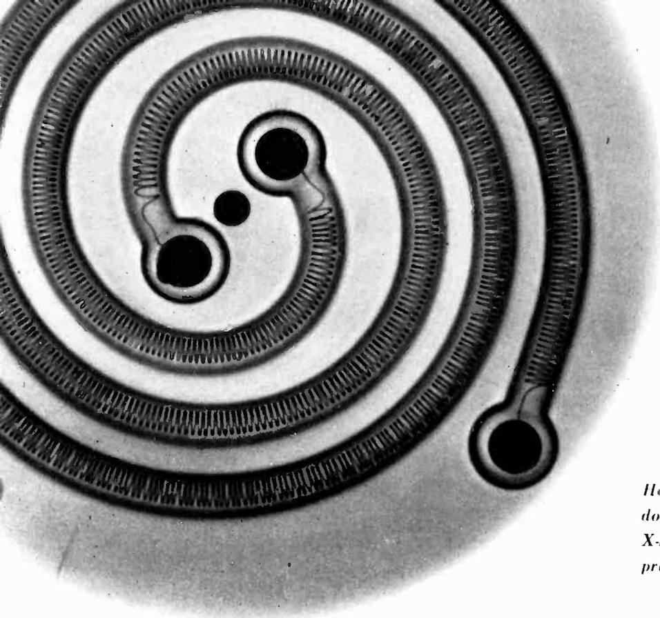
*Heater coils of a domestic appliance X-ray tested for proper spacing between turns*
