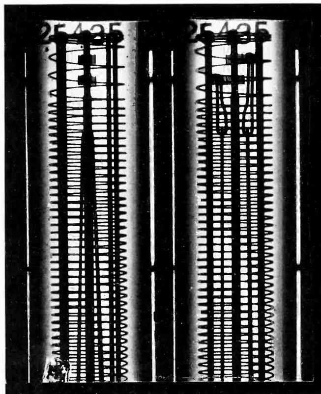
be properly aligned with respect to each other and to the surrounding copper anode. Anodes are X-rayed after the assembly has been sealed-in to reveal the exact position of the inner structure and to facilitate alignment measurements.
