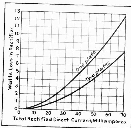
Fig. 6—80-type rectifier loss data
