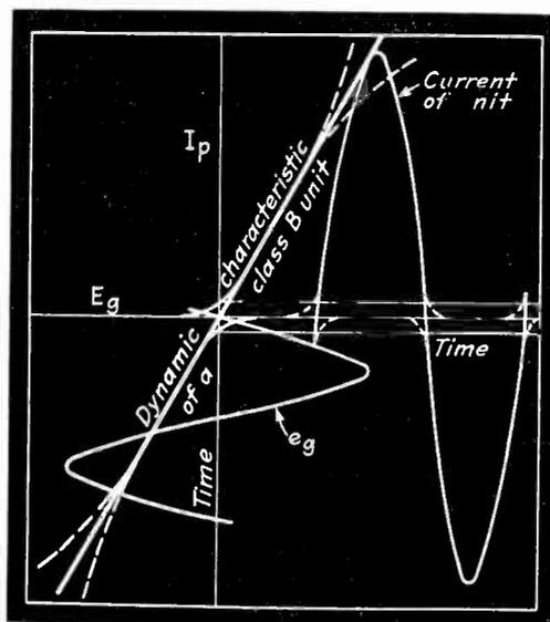
Fig. 2— $I_p$ - $E_g$  dynamic characteristics of Class B unit
