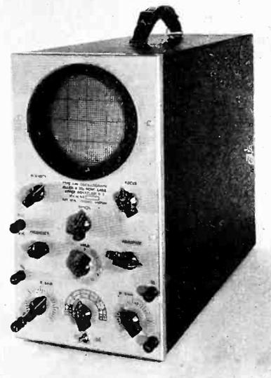
This instrument features a *basically new sweep* which allows waves from 10 to 500,000 cycles to be observed with improved linearity and exceptionally fast return trace.
