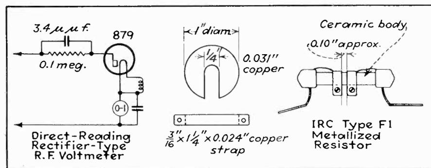
Fig. 3—R-f voltmeter and multiplier-equalizer details
