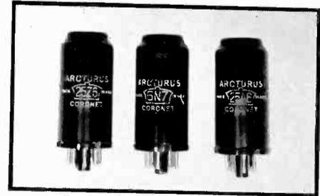
addition, be used in the driver stage as a Class "A" amplifier for driving the input circuit of a 6N7 operating as a Class "B" amplifier. The 25A6 is a 25.0 volt output tube, identical to the type 43, and is for use in ac-dc receivers. The 25Z6, identical in characteristics to the 25Z5, is a 25.0 volt full-wave rectifier for ac-dc operation.
