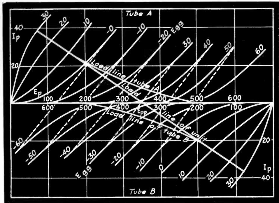
Fig. 4—Composite characteristics of Class AB amplifier
