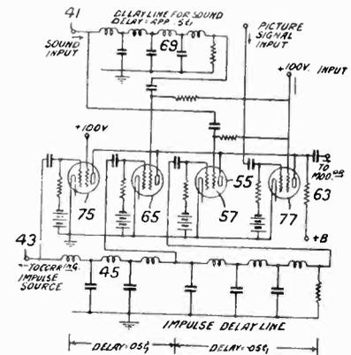
tion enables the time taken by the return of a scanning cathode-ray to the beginning of successive scanning lines to be used for sending accompanying sound. Also No. 434,891 to H. Branson, Marconi, on a similar subject.
