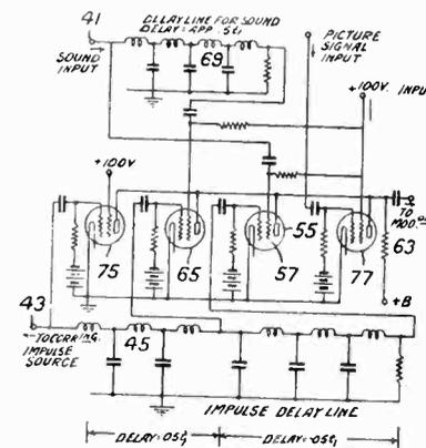
tion enables the time taken by the return of a scanning cathode-ray to the beginning of successive scanning lines to be used for sending accompanying sound. Also No. 434,891 to H. Branson, Marconi, on a similar subject.
