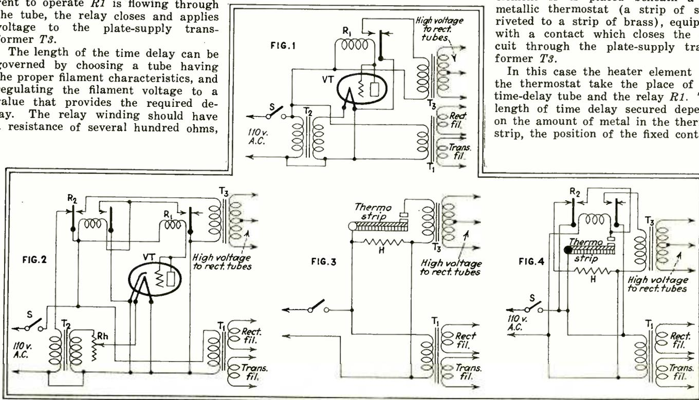
Circuits for introducing a time-delay in the application of high voltage to the plates of mercury-type rectifier tubes
