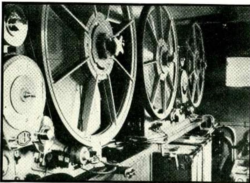
This self-contained steel-tape magnetic recorder, installed in a truck, is used in Berlin to gather opinions from the man in the street, news events, etc., which are later broadcast in an evening program called "The Echo of the Day"
