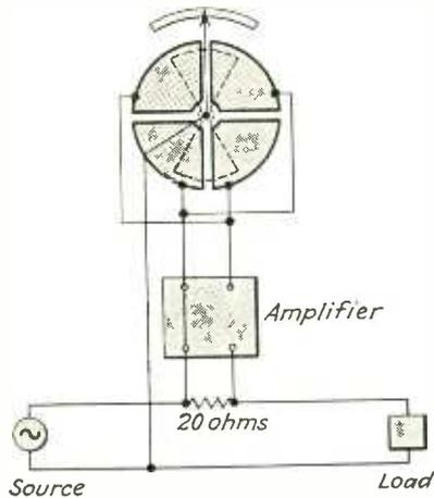
Fig. 1—Connections for measuring the power taken by a load
