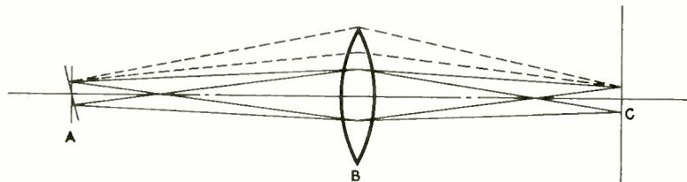
Fig. 1—Mirror, lens, screen to illustrate the "split-focus" systems
