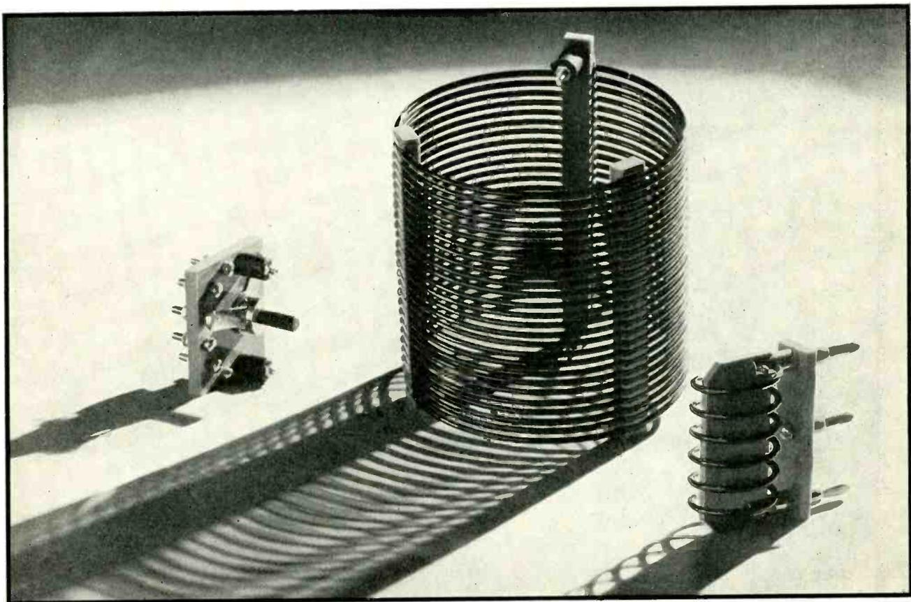
*Low-loss (Victron) parts made by Communication Products, Inc. The material is made opaque by a coloring matter to improve appearance and molding properties. It has no effect upon the dielectric properties*
