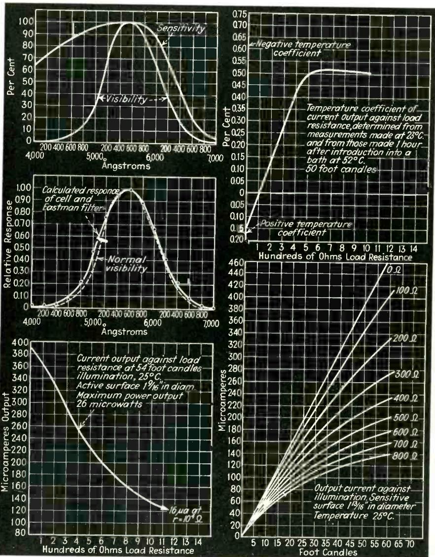
Quantitative data on the G. E. Blocking Layer selenium-platinum self-generating photocell
