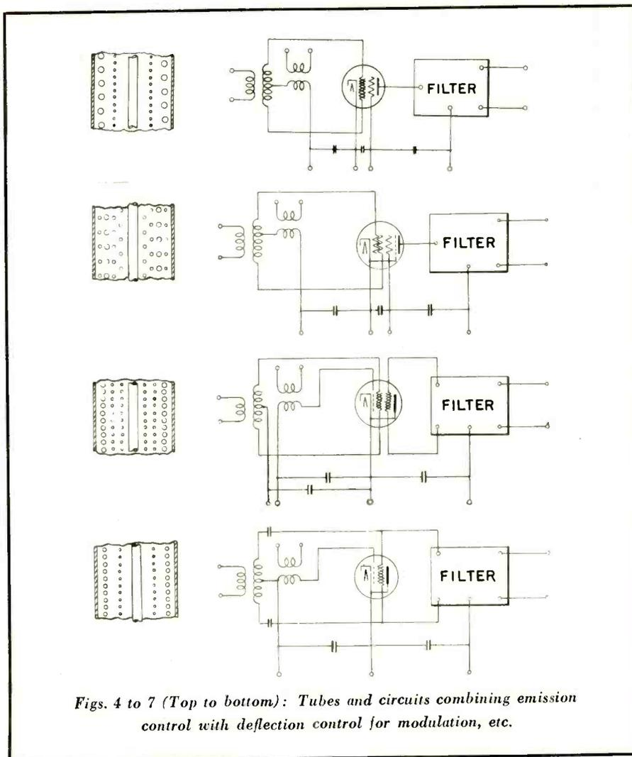
Figs. 4 to 7 (Top to bottom): Tubes and circuits combining emission control with deflection control for modulation, etc.
