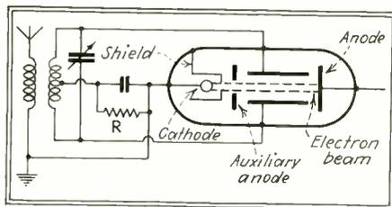
known as the concentrator is operated at a negative potential. Two plates running the length of the tube again correspond to cathode ray tube practice
