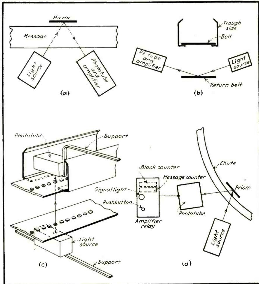
A and B—Light beams are projected through a belt—or across its surface. C—If the rate at which beam is interrupted decreases, an alarm sounds. D—How the phototube measures the ratio between messages successfully transmitted to those that stuck temporarily
