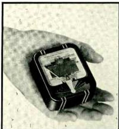
illumination levels are fully and legibly indicated. The scale is divided into five "seeing task" zones, set off by colored divisions. The back of the indicator contains an embossed metal plate classifying specific seeing tasks so completely that no assumptions need be made by the user.
