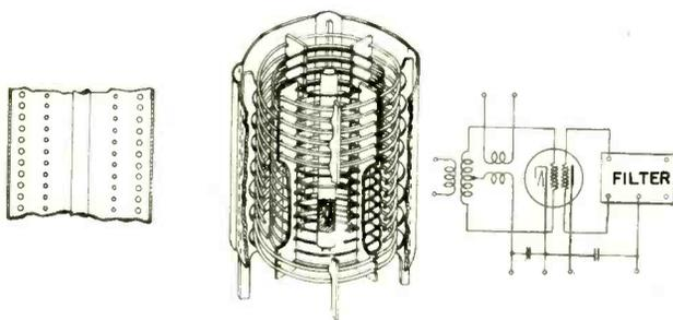
Fig. 1. The deflection tube and a typical amplification circuit
