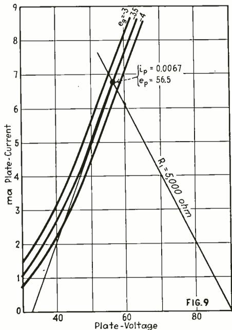
A 49 type tube connected as a triode provides a practical example of using the circuit of Fig. 8
