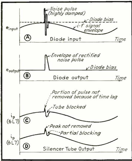
Fig. 2—(A) Diode input of signal envelope (only one edge shown) and noise. (B) Rectified envelope of noise peak applied to blocking grid of silencer. (C) Effect of blocking action on i-f envelope. (D) Incomplete blocking if noise is not sufficiently strong.
