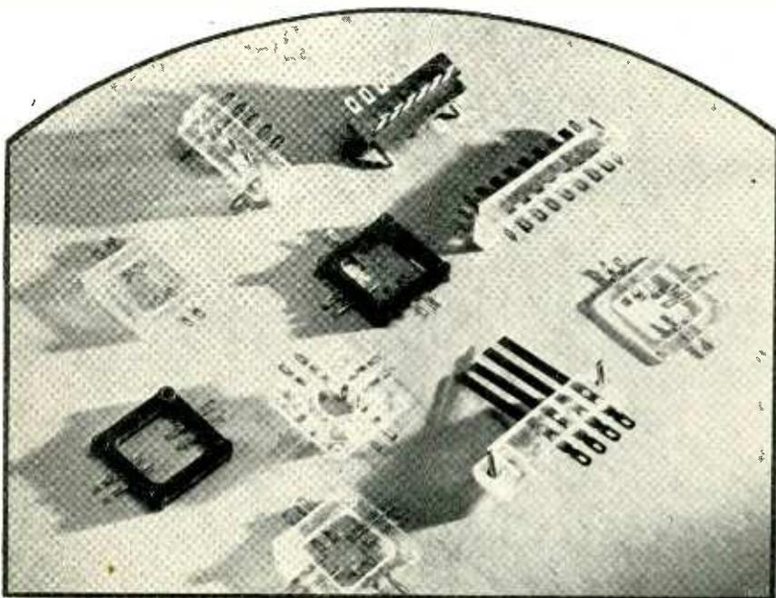
brittle and are quite difficult or impossible to machine. For this reason, if employed for coil forms with grooves for wires, the grooves should be molded into the form.
