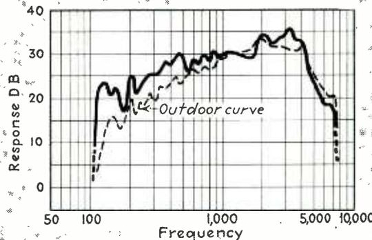
Fig. 5—Curve taken in a highly damped room at 12 feet with rotating condenser microphone. An outdoor curve is also shown. (After Bostwick)
