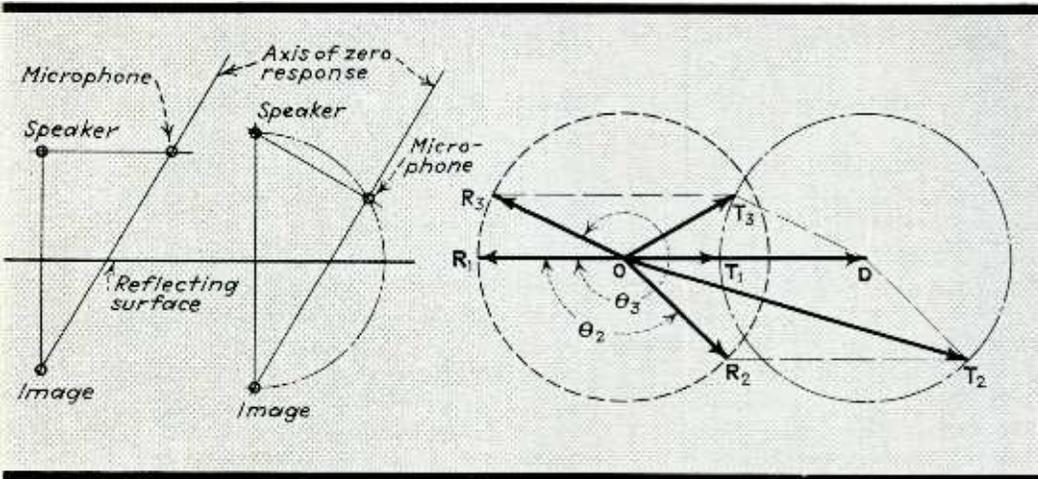
Fig. 6 — Directional microphone eliminates ground reflections
