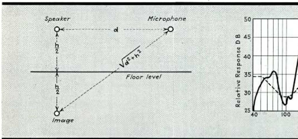
Fig. 2—Floor reflections in making loud speaker response measurements
