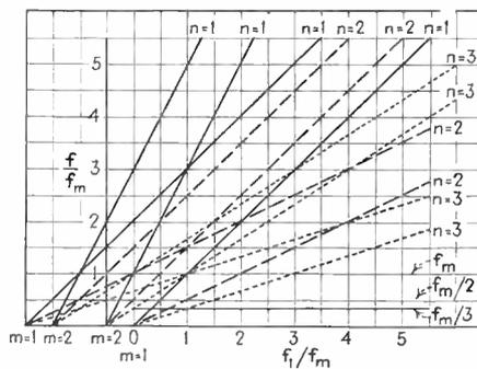
the stations are taken into account although in the particular example the interfering stations would have frequencies below 500 kc. Any station having a frequency  $f$  might be received together with the desired station  $f_1$  whenever
