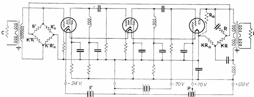
Above, representative amplifier circuit, with bridge-type feedback
