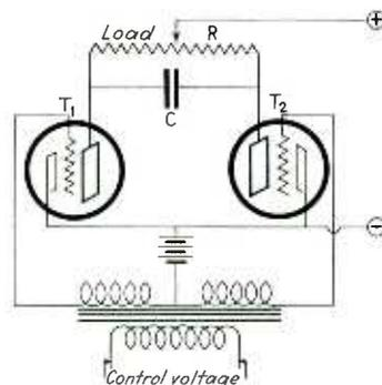
FIG. 3 - Use of one tube to control another
