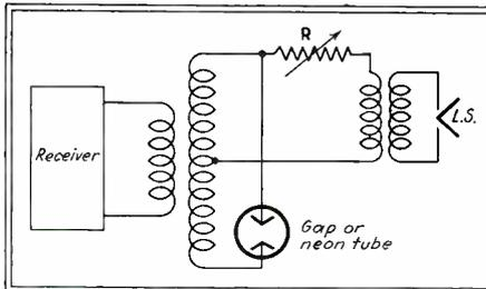
In this patent a circuit is shown involving an output transformer connecting the receiver to a loud speaker. A neon tube is substituted for the gap shown in the original patent and at a certain value of resistance, distinct noise limiting action occurs.
