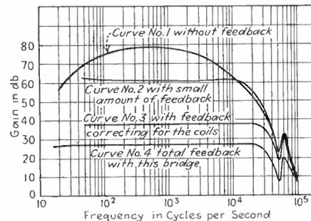
Typical feedback amplifier characteristics, gain vs. frequency and output current, effect on harmonics
