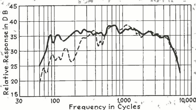
Fig. 4—Response curves taken on a cone loud speaker. Solid curve taken at one foot distance; dotted curve at three feet distance
