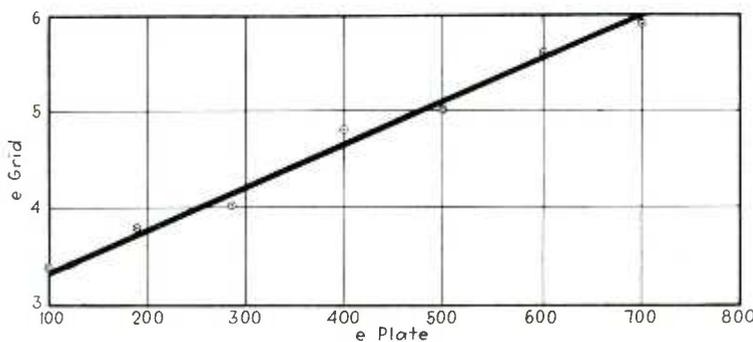
FIG. 1 - Grid-anode voltage regulation of F6-17 thyatron
