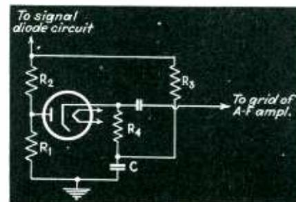
Static limiter circuit, described in the text (G. E.)
