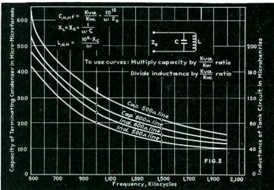
**2&3** Charts for calculating capacity and inductance of radio-frequency amplifier tank circuits
