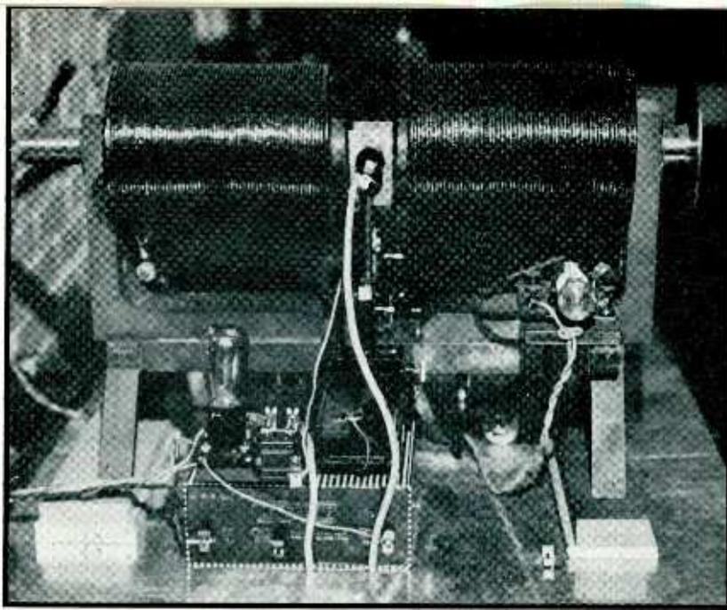
Chamber unit with Geiger counter mounted in an electromagnetic field for reflection of Alpha particles
