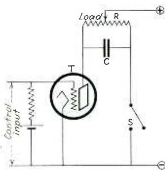
FIG. 2 - D-C operated controlled rectifier
