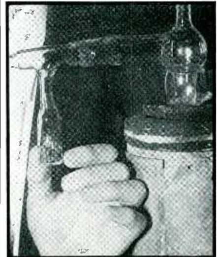
*What is claimed to be the smallest radio tube ever made has been constructed by Chao-Ying Meng, research fellow at California Institute of the Technology. The wavelength generated by it is about one centimeter long. The retarding field method is used, the plate (0.5 mm. inside diameter) being at zero or slightly negative bias while the grid (0.2 mm. diameter) is at high positive potential*
