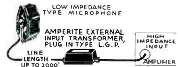
of the design eliminate hum pickup. Either a 50 or 200 ohm microphone can be fed into the standard input impedance of 200 ohms. Other impedances obtainable upon request. List price, \$5.00.
