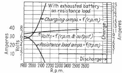
cooled and runs 14 to 16 hours on a gallon of gasoline. The generator maintains its voltage constant over a wide range of varying loads and permits the use of a resistance load across the batteries for lighting or power purposes. The list price is \$55 for the 6-volt unit and \$57 for the 12-volt unit, useful for boats and yachts.
