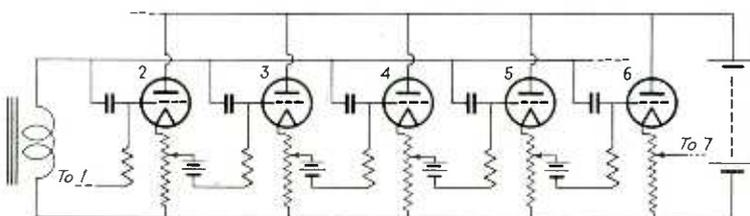
FIG. 4 - Multiple tube circuit increases ability to count speedily
