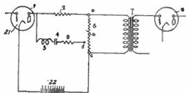
decreasing the attenuation of certain selective portions of the frequency band while maintaining the remainder of the band at the predetermined level. H. G. Tasker, United Research Corp. No. 2,037,285.
