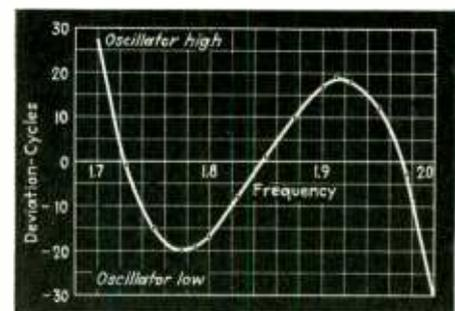
Fig. 2—Graph showing deviation from perfect tracking
