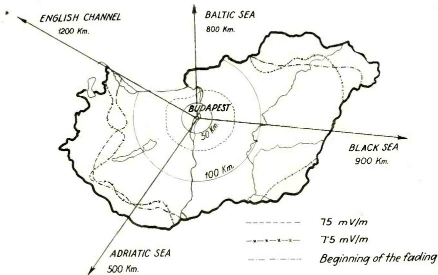
terferences. Budapest I. is working on 546 kc and with an antenna power of 120 kw, and it might be of interest to report the experiences and observations made with this transmitter, as conclusions can be drawn from them.
