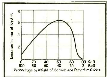
Fig. 3—Electron emission of oxide cathodes as a function of the relative percentages of barium and strontium oxides
