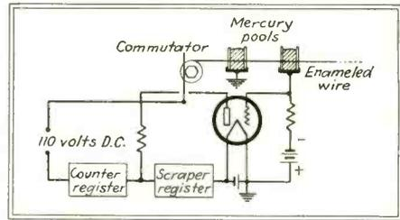
*Circuit for testing enamel wire*
