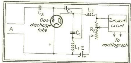
Gaseous discharge tube circuit for transient oscillograph
