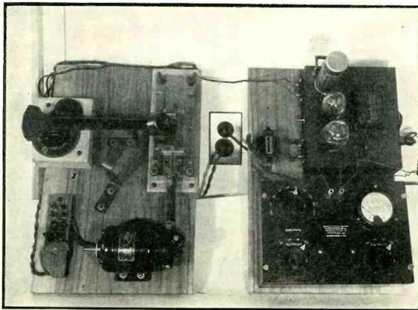
Fig. 1. Pick-up surface tester and amplifier
