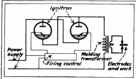
Two ignitrons connected for welding operation
