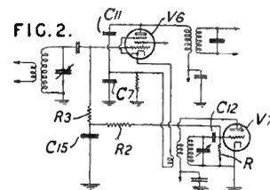
ceiver, a regenerative mixing tube has its regeneration varied by a biasing voltage derived from the oscillations. N. P. Case, Hazeltine Corp. No. 453,658.
