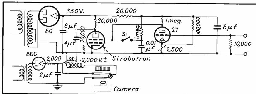
Fig. 5 Circuit diagram of a light-flashing apparatus for the photographic recording of spectral data
