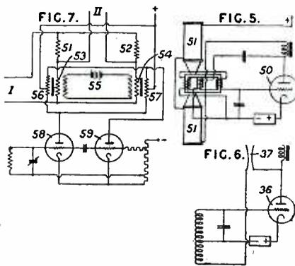
bias applied to capacities or inductances in circuits arranged to vary tuning, coupling or feed-back. Circuits are shown in which the band pass is a function of incoming signal strength. L. L. Kramolin, Berlin. No. 455,190.
