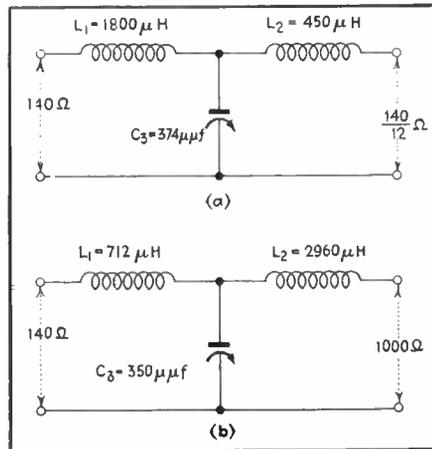
Fig. 4—Matching networks. A—Branch line to load. B—Line to attenuator
