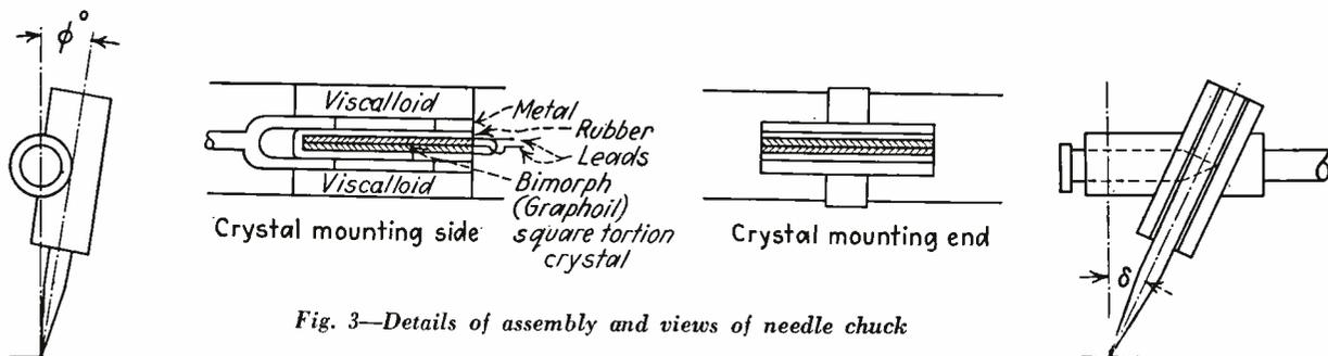
Fig. 3—Details of assembly and views of needle chuck
