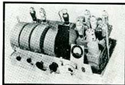
*Unusual layout and fine attention to mechanical detail characterize the newer German radio set chassis. The coils (inside the cylindrical water-tight cans) are moved between contacts, instead of being switched, for each waveband*
