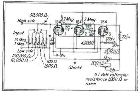
Schematic wiring diagram for instrument measuring  $10^{-3}$  to  $10^{-8}$  ampere, full scale
