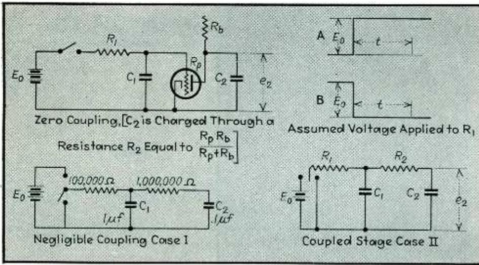
Fig. 5—Coupled and uncoupled two-stage filters
