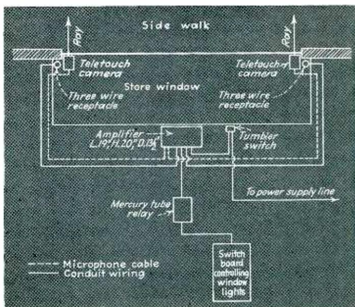
Set-up of Teletouch Ray for automatic window-lighting control
