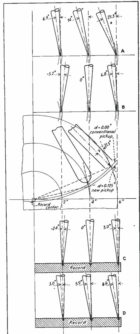
Fig. 2—Needle orientation, A and D, conventional pickup; B and C, new pickup
