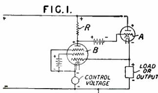
rived from a resistance connected across the supply in series with an auxiliary triode and a source of control voltage which is included in series with the load voltage or a part thereof in the grid circuit of the auxiliary tube. Philadelphia Storage Battery Co. No. 455,031.
