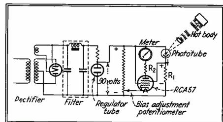
Schematic wiring diagram of the photoelectric pyrometer. A type 57 pentode is used to amplify the output of the phototube
