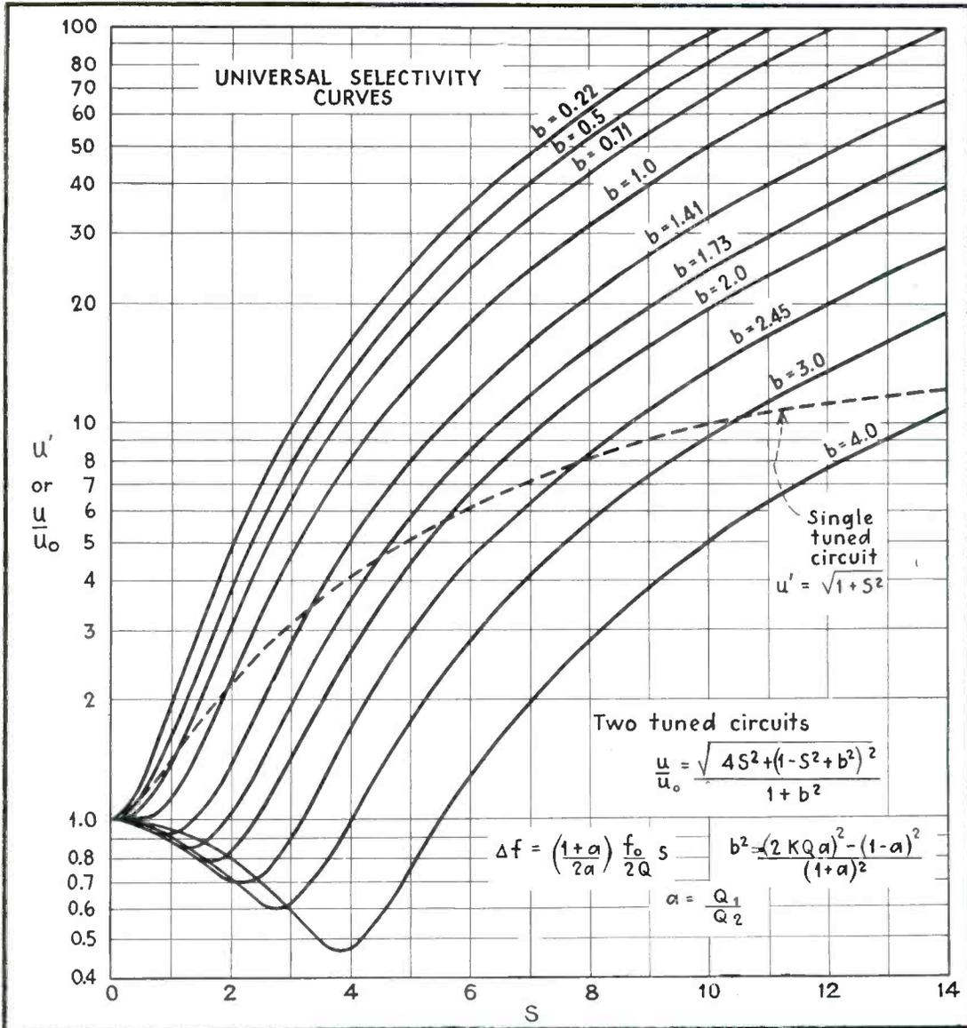
Solid curves for two tuned circuits show attenuation,  $u/u_0$ , and parameter,  $b$ , plotted against  $S$ . By interpolating, curves for other values of  $b$  may be determined. Dashed line shows similar information for single tuned circuit.
