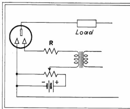
*Relay circuit using new tube*
