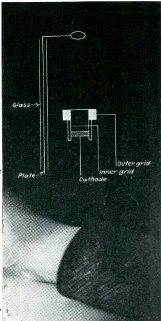
Fig. 1 Photograph and drawing of Strobotron showing arrangement of the elements
