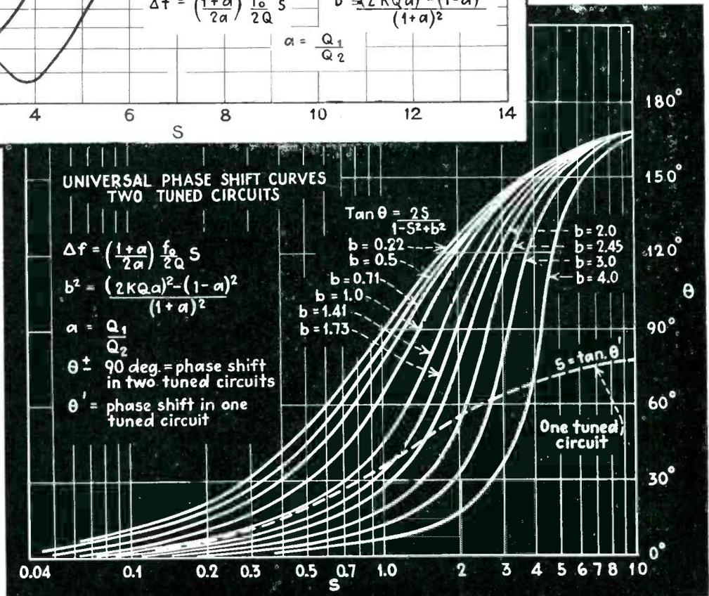
The equations for selectivity and phase shift for a single tuned circuit are given by
