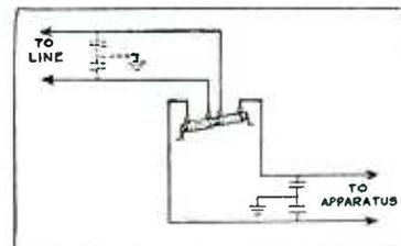
These power line chokes will not prevent interference of audio frequency and they are not recommended for that purpose.
