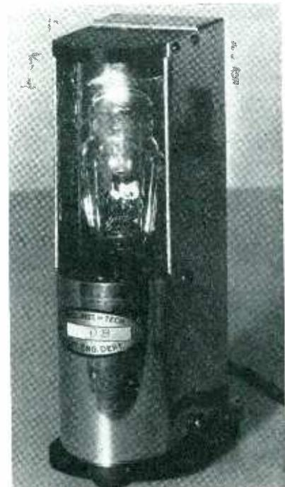
Completely assembled 60-cycle stroboscope in use at M.I.T.
