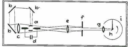
Combined shadow method and rotating camera technique for use with a spark discharge
