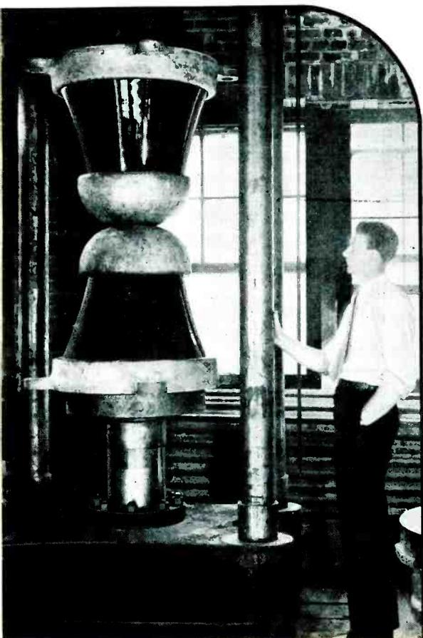
considerably lower loss, according to the claims of the manufacturer. Tests made by the National Physical Laboratory in England on the lead-less variety give values of dielectric constant of 6.1, power factor of 0.2 per cent. and loss-factor of 1.2. This loss factor compares favorably with the best steatite porcelain.
