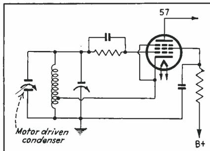
Fig. 2—Circuit of oscillator employed
