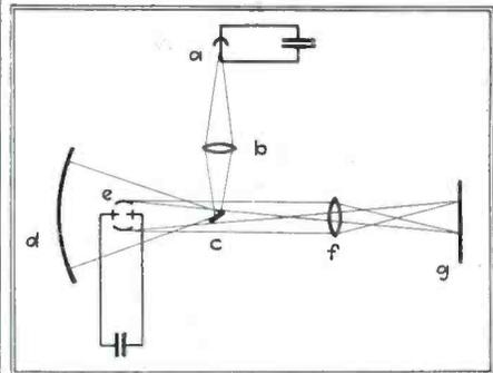
Diagram of the Schlieren method of photographing sound applied to a spark discharge
