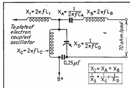
Fig. 3—Oscillator plate to line transformer
