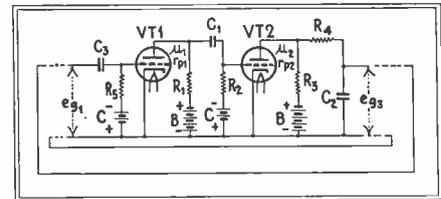
Schematic wiring diagram for the oscillator circuit using non-resonant circuit elements. By interchanging  $R_4$  and  $C_2$  the usual multivibrator circuit is obtained
