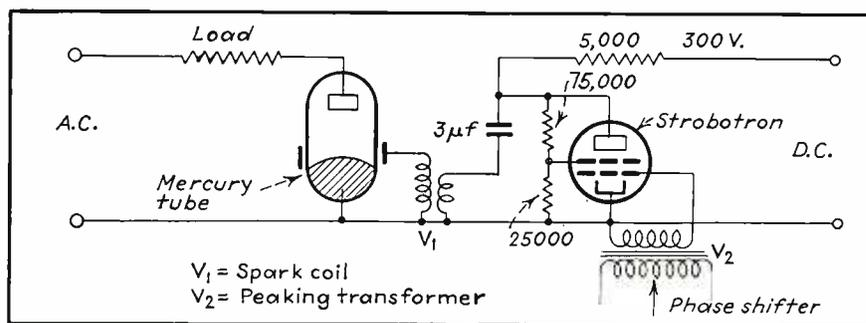
Fig. 6 Circuit showing the use of a Strobotron for starting a mercury pool rectifier used in a half-cycle welding circuit
