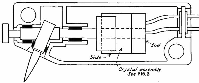
Fig. 4—Cross section of record-saving pickup
