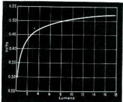
Fig. 3—Voltage output vs. illumination, high levels
