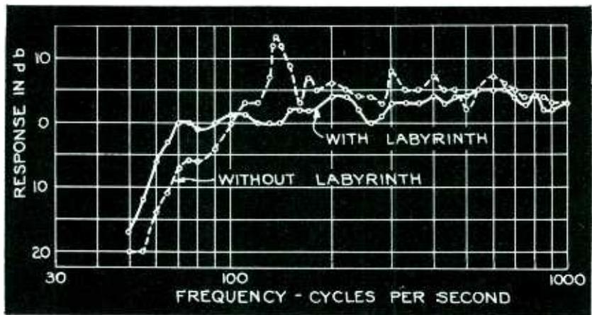
Fig. 4—Response of 8 in. cone loudspeaker in cabinet 2 ft. x 2 ft. x 1 ft. inside dimensions. Back of cabinet 2 in. from wall
