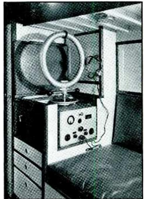
Two d-f installations on pleasure craft, both Bludworth models. The below-decks model (above) can be used inside wooden cabins. The model shown mounted on the cruiser (left) is completely waterproof and will operate readily when submerged in hot salt water.
