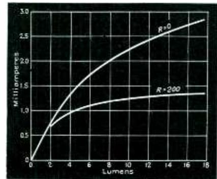
Fig. 1—Current output vs. illumination for low light levels
