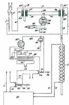
strip and a standard strip with means whereby the differences in permeability between the portion of the strip passing through the furnace compared to the permeability of the standard piece will cause operation of the furnace control means. A. R. Stargardter, Gillette Safety Razor Co., Boston. No. 2,059,976.
