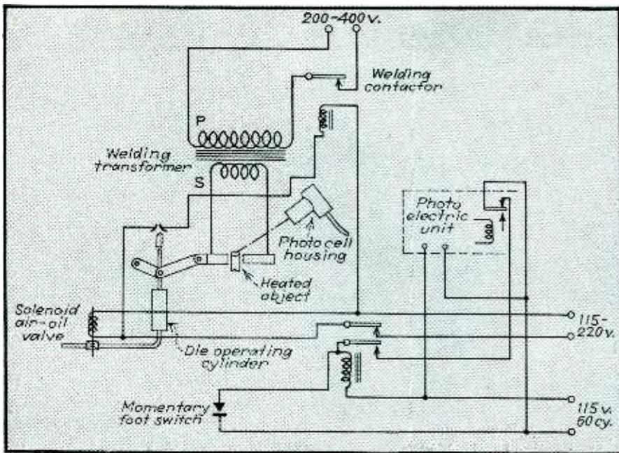
Typical phototube temperature control. Hydraulically driven dies may be eliminated in favor of a solenoid locking the work in proper position
