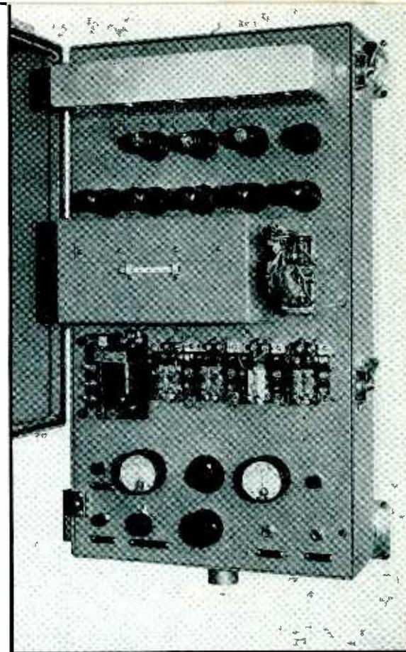
*The RCA-Radiomarine Corporation Auto Alarm. At the top is the superhet receiver. Below, a row of five timing tubes, which control relays in the box-like oven. These relays actuate the main contactors for counting and alarm-ringing*
