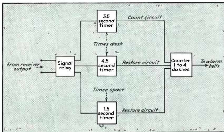
The auto-alarm receiver controls a relay which closes on each signal received. Three timers time the length of each signal and each space. If the signal is between 3.5 and 4.5 seconds long, and if the space is not longer than 1.5 seconds, a "count" is registered. Four counts actuate the alarm bells
