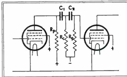
Fig. 2—By adding an additional blocking condenser and grid resistor, ordinary commercial condensers may be used in a stable resistance coupled amplifier
